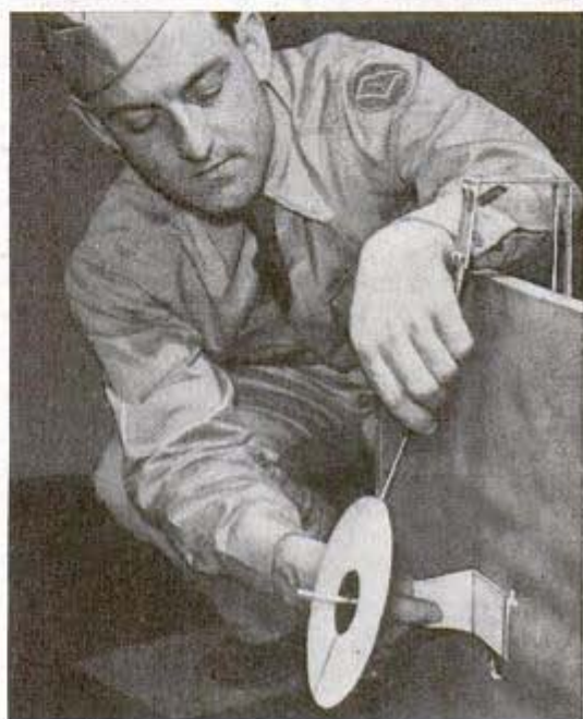
Lights in upper right hand corner on back of plywood target board tell operator direction in which to move target. Center mechanism consists of steel plate with cross pieces for suspending target and gears for moving it. Note roll of paper for marking. Right, Corp. Stanley J. Ketterer, Missouri State Guardsman, the inventor, shows paper used to record score
