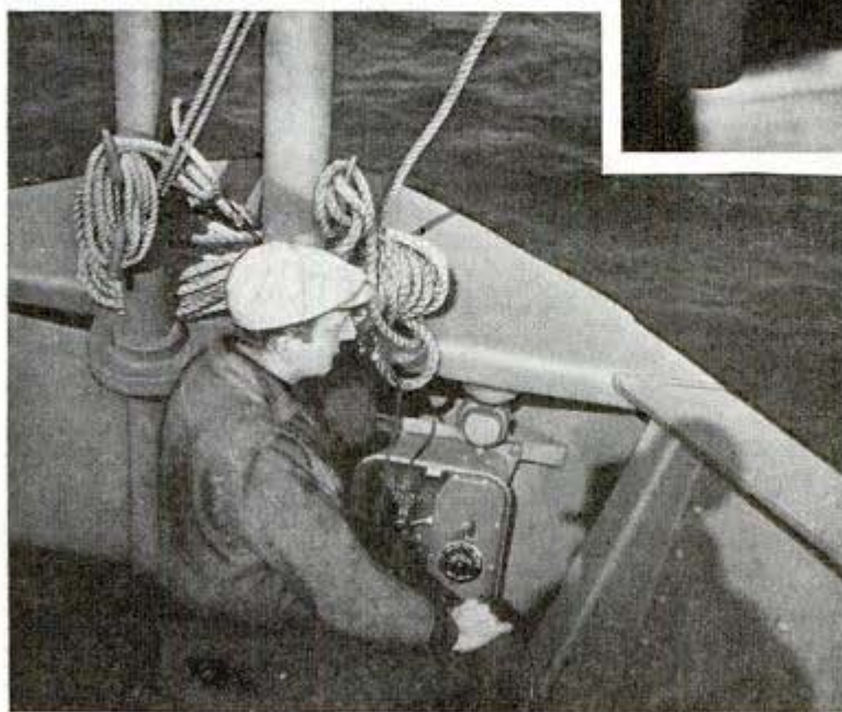
Waterproof telephone in station of bow lookout on Liberty ship
