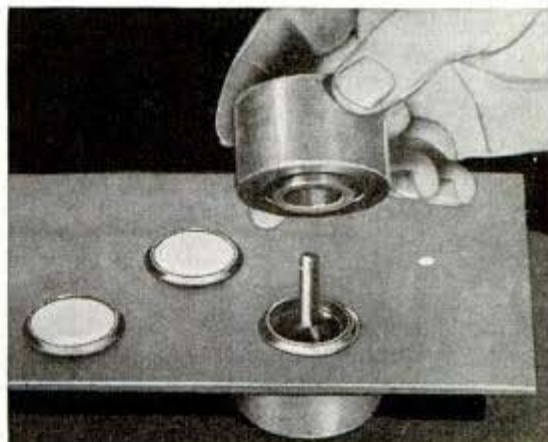
Tool cuts flanged holes in metal, straightens edges
