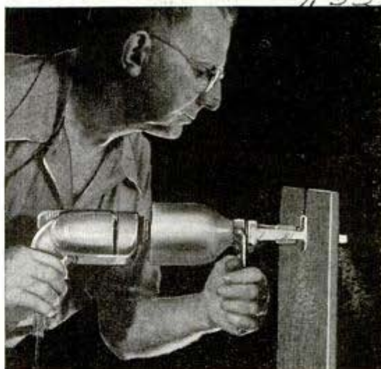
This "drill saw" can be used on either metal or wood
