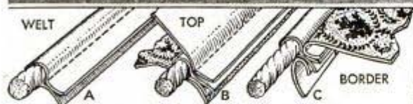
(15) CORRECT WAY TO SEW WELT CORD TO CUSHION TOP AND BORDER
