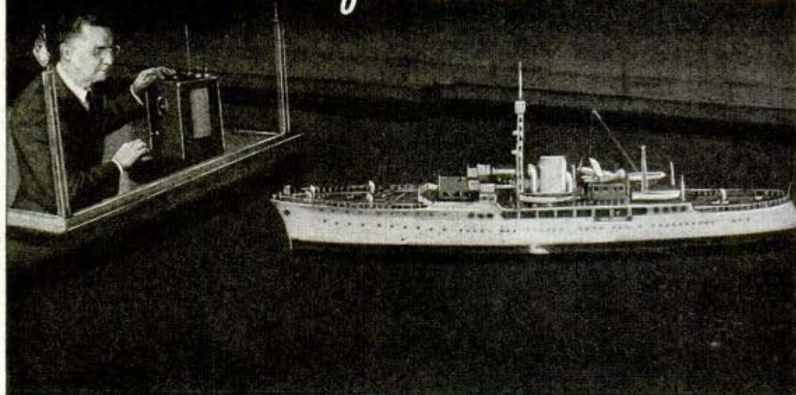
On a model yacht basin at Franklin Institute a radio-controlled ship maneuvers as operator dials transmitter
