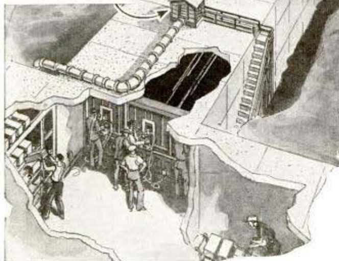
TWO BLOWERS, ONE AT EACH END, CLEAR RANGE OF GAS AND SMOKE
