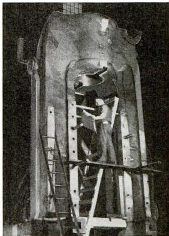
The manipulator above easily flips into any position the huge blank for bull gear of turbine-driven cargo ship, making welder's work easy. Below, the 97-ton metal monolith is a housing for steel rolling mill
