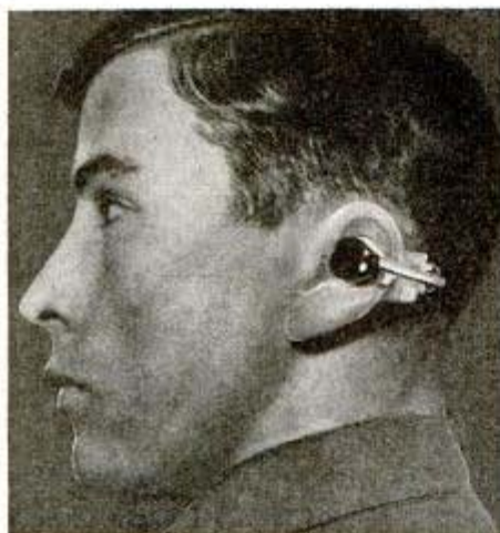
Top, electric current arcs sample of pure iron and spectrograph focuses radiation through prisms to record wavelength portrait of iron. Pilot's oxygen need is discerned (left) by watching blood color with phototube device. Below, welders work on turbo-generator, circled by frame for a huge motor
