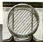
Straight lines through optical flat indicate perfect flatness.
