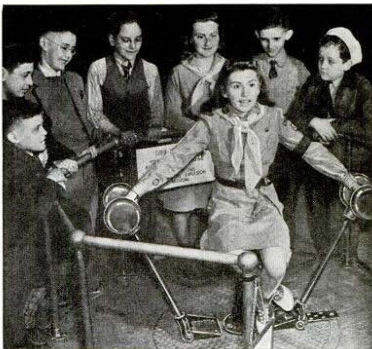
Spinning faster on rotating seat as she pulls weights in with her arms, this girl is demonstrating the law of conservation of angular momentum
