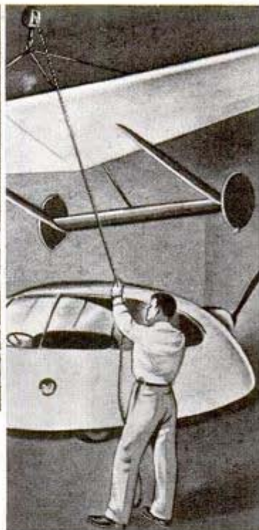
Stout's Aerocar, the flying family auto, is to be equipped with "hook-on" wings, shown being installed above. Shown below is the Aerocar in flight. Unlike the roadable plane, which is intended to be primarily a plane and secondarily a car, the Aerocar is, first, a good automobile
