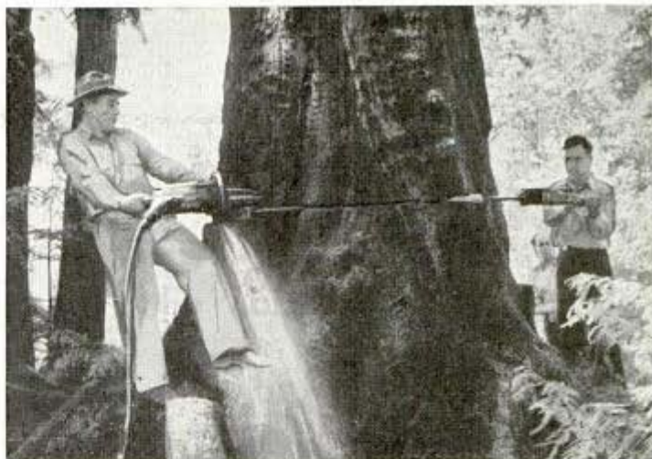
Above, felling a big tree with an electric saw powered by a generator on a Caterpillar Diesel tractor. The logging train below is hauling new-felled timber to a sawmill in the Redwood Empire
