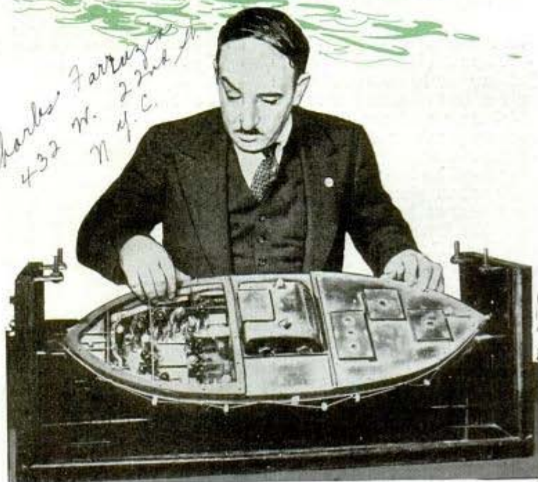
Below, inspecting model of an unsinkable lifeboat which has special compartments
