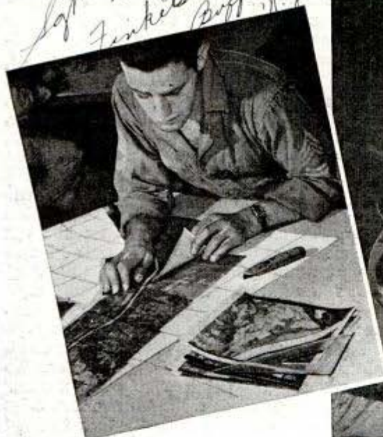
↑ Aerial photographs taken from various angles at high altitudes are matched into a large strip mosaic map. Sometimes three-dimensional maps are made, revealing the heights of objects seen under stereoscope
