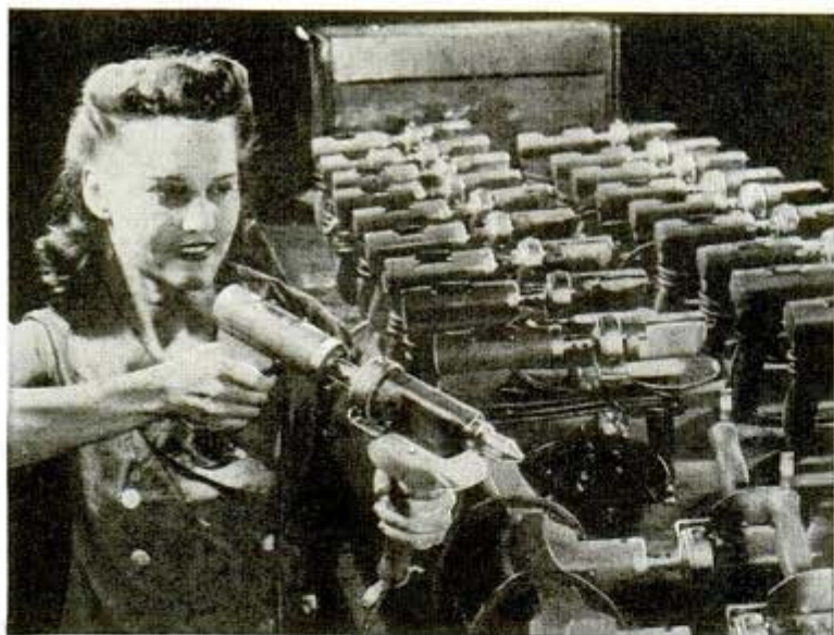
Heat guns firing explosive rivets used in aircraft manufacture incorporate the heater element from your electric stove, the thermostat from an ironer
