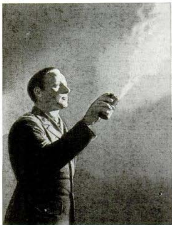
Canned death for malarial mosquitoes comes in containers first used to charge refrigerators with Freon
