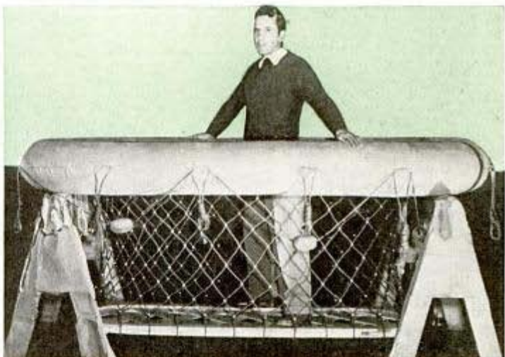
"Doughnut" life raft can sustain 15 men inside mesh on platform and hanging on outside ropes. Below, emergency flotation gear on wing of land plane will keep it afloat if it's forced down at sea
