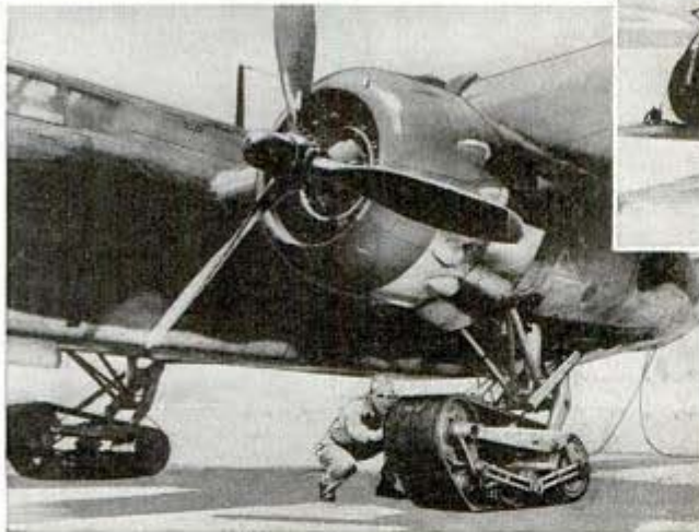
Caterpillar-type landing gear permits ship to land on unfavorable terrain at speeds as high as 120 miles per hour
