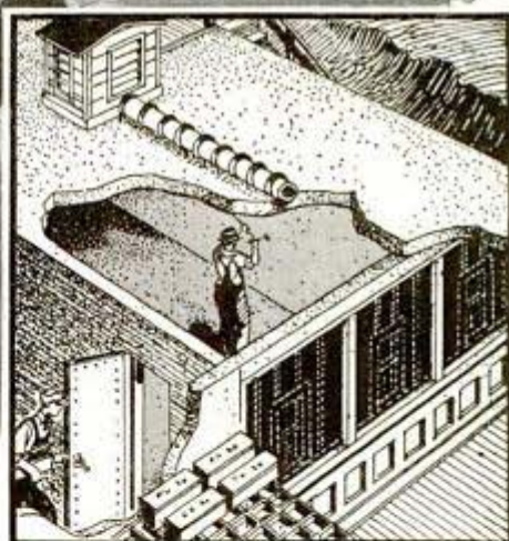
Built of concrete, the world's longest enclosed firing range is 1,800 feet in length. Above, firing ports close automatically when door leading into firing range is opened by maintenance men
