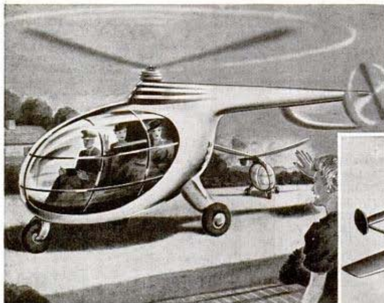
Stout's Aerocar would do 60 to 70 miles on the highway, and 100 miles an hour in the air with about the same gasoline consumption. Its air range would be about 250 miles. His roadable plane would be for use in the West, where distances are longer, and would have a range of 400 miles in the air, coming to the ground only if the weather is bad, and remaining on the road only until the storm area is passed. Its wings would fold for road driving. It would speed at 120 m.p.h. in the air, 35 m.p.h. on the ground. Above is a third of Stout's conceptions for postwar travel, a Helicab. He considers it most practical for use in congested cities, especially for home-to-office commuters. Stout says he foresees electronic controls to prevent collision and constant ground-air communication
