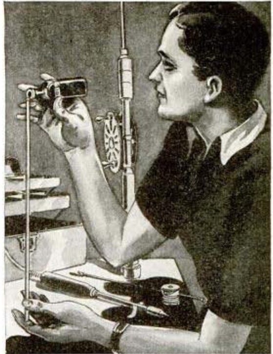
② USE OF LINSEED OIL INSIDE TUBULAR SECTIONS OF RODS WILL CHECK RUST
