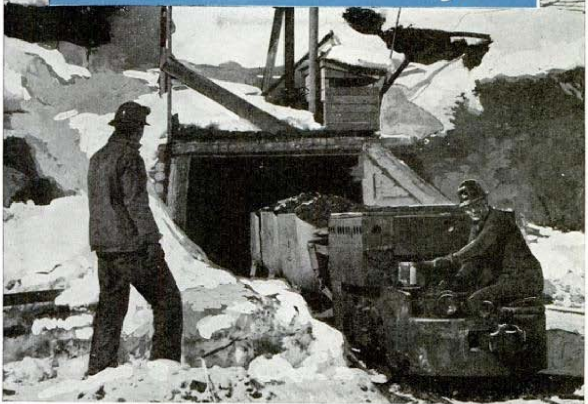
Dump cars laden with ore emerge from Benbow Mine, first of the chromite mines in the Beartooth range of Montana to begin war production. Ten cars are drawn by battery-driven locomotive
