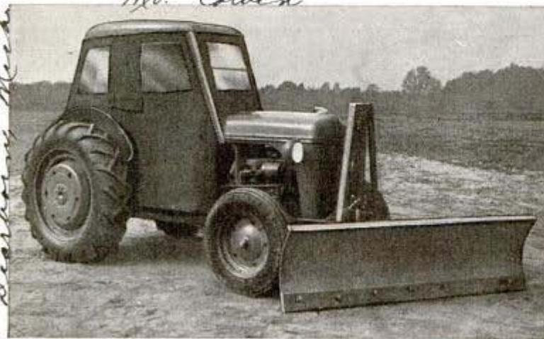
Angledozer on front of tractor is used to level runway or remove snow
