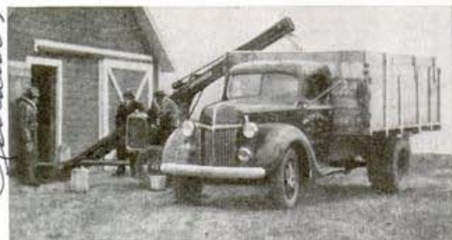
Parts of old farm machinery and of three different autos went into grain-loader (top), also pictured while at work (bottom)
