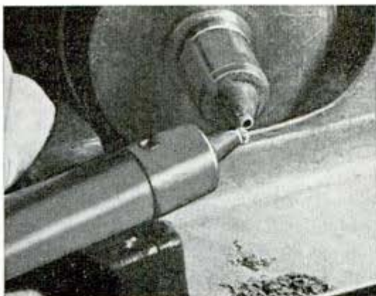
Closeup of girdling operation. Diamond dust dropping into bin is salvaged for use with olive oil for other cutting operations
