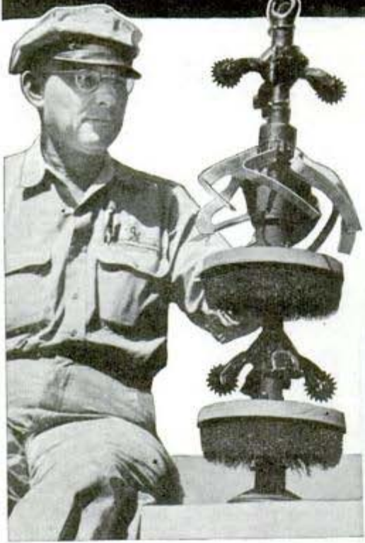
Engineer inspecting "go-devil" or "pig" used for cleaning pipeline and detecting wasteful leaks Right, a big ditcher rolling east preparing way for 24-inch pipe requiring 360,000 tons of steel
