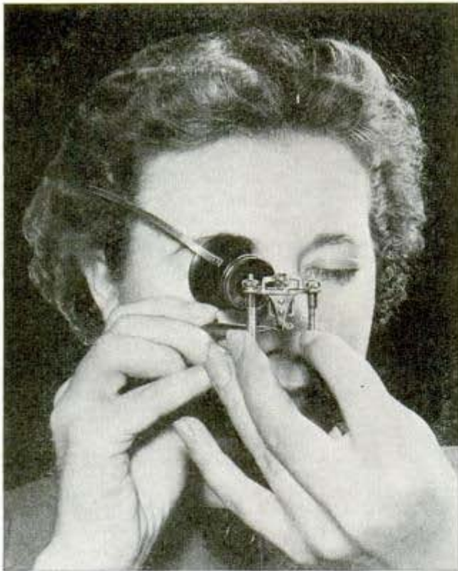
Magnifying eyepiece is used to inspect intricate parts of electric instruments (above). Below, what appear as stout bands of cable are really Westinghouse lamp-filament coils enlarged 65 times and pictured in a projection on a screen
