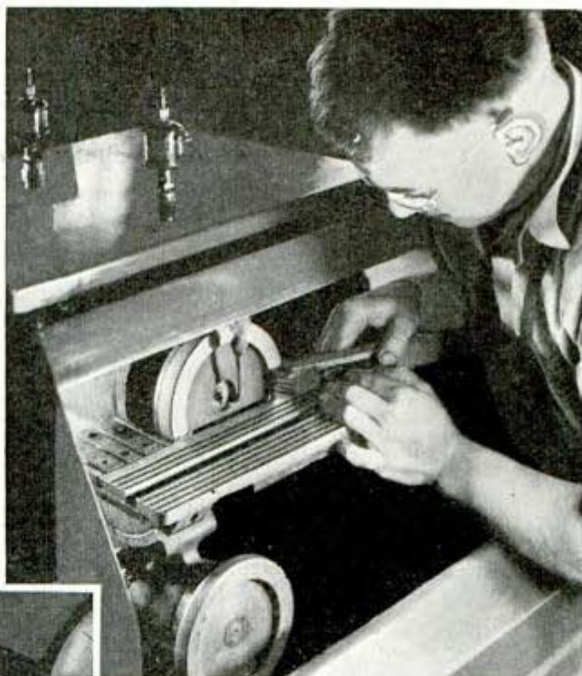
Norton Company photo Employing a diamond grinding wheel, the machinist above is sharpening a carbide tipped tool. There are several million dollars worth of diamonds in this pile; these jewels pay for the mining of cheaper industrial "diamonds in overalls"
