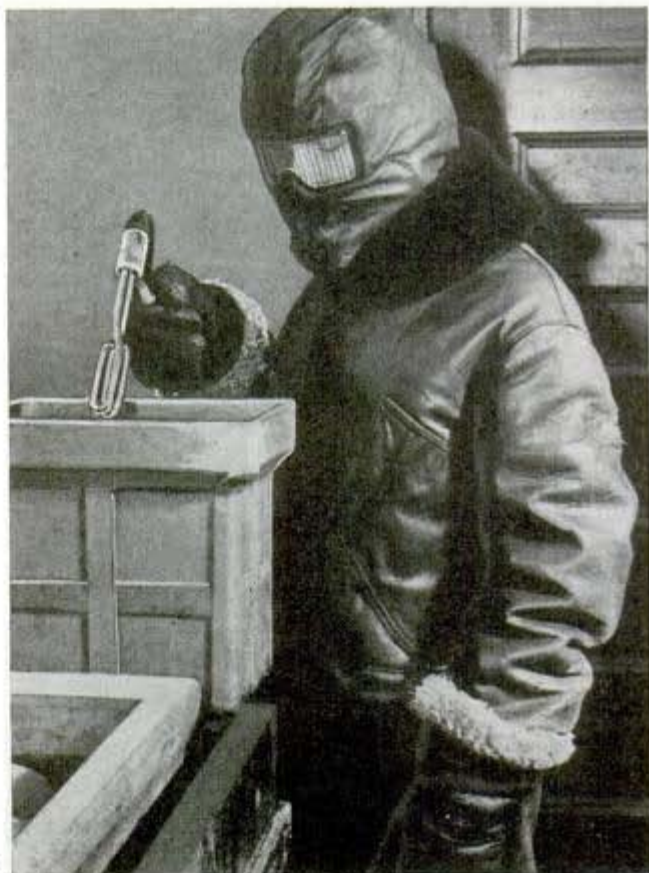
Immersion heater similar to heating unit in a kitchen range is used to warm developing solutions in Arctic photographic labs
