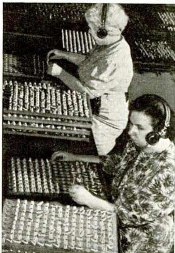
"Hear no evil" is the hope of inspectors at Stewart-Warner plant, who can detect by ear a defect in shell fuse heads
