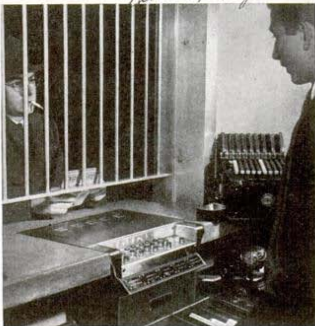
"Automatic ticket machine," used in an eastern railroad ticket office, can hold 24 different tickets, and 4,000 of every type
