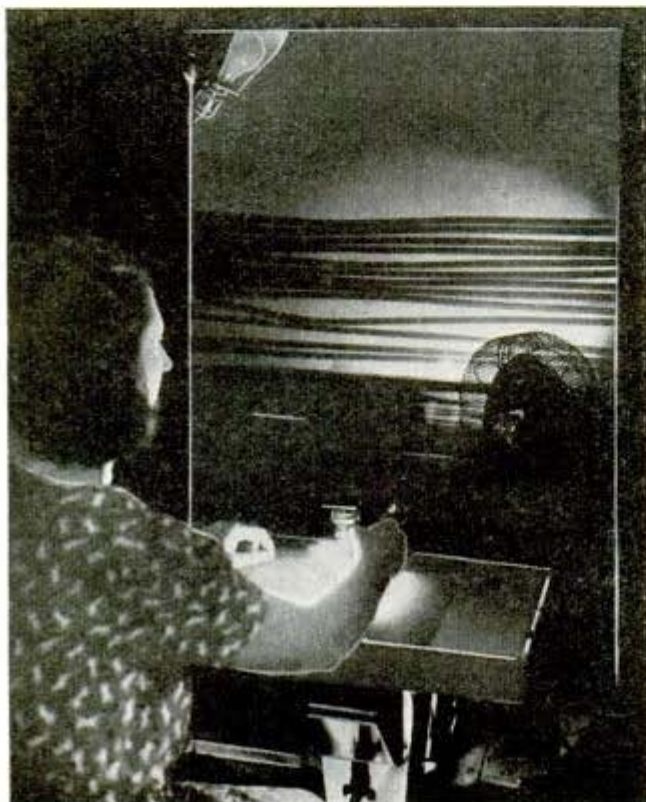
Magnifying eyepiece is used to inspect intricate parts of electric instruments (above). Below, what appear as stout bands of cable are really Westinghouse lamp-filament coils enlarged 65 times and pictured in a projection on a screen
