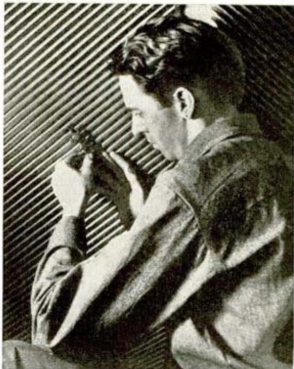
Allowable error in spacing of these gear teeth (above) is 1/10,000 inch, 1/50 the thickness of paper of this page
