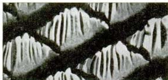
Micrograph enlargement of serrated teeth of coarse double-cut file.
