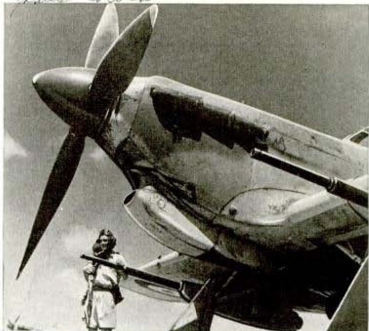
Hurricane used as anti-tank weapon mounts two 40 mm. cannon in wings
