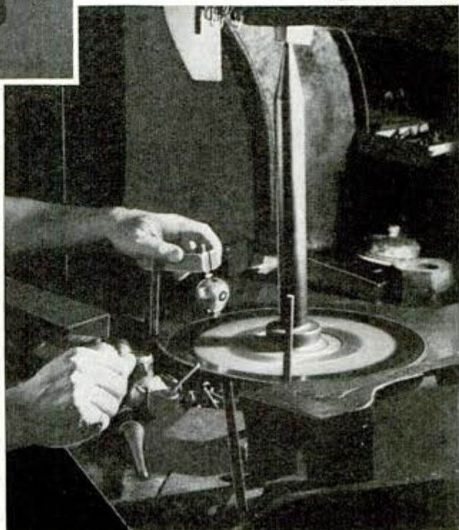
DeBeers photo Polishing a diamond with a steel wheel a foot in diameter, soaked in diamond powder and olive oil
