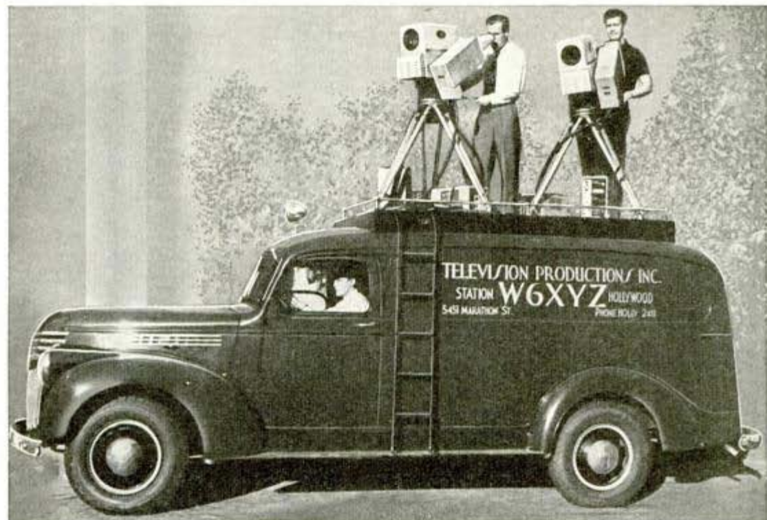
Mobile television unit mounts cameras on top of truck and beams picture to main transmitter for broadcast
