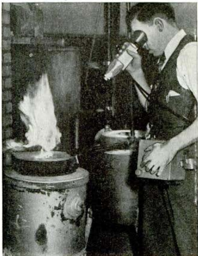
Visual thermometer—a gauge to measure the temperature of flame by matching color of fire with heated coil in 'scope
