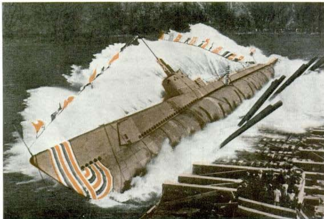
With a great splash the U.S.S. Puffer, fourth submarine to be built on the Great Lakes, is launched on its side at Manitowoc, Wis. Like all U. S. submersibles, it is named for a fish
