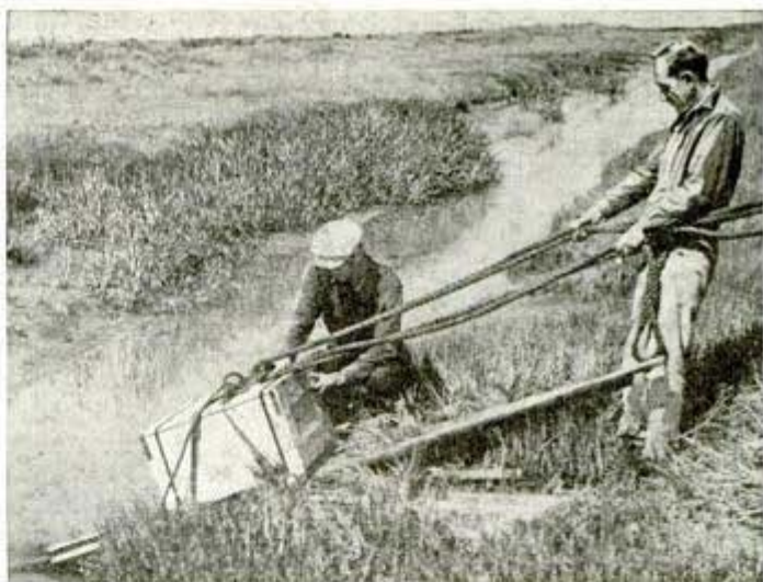
To test packing of replacement parts for army vehicles, box of the parts was sunk in San Francisco Bay. Here, workmen remove the box
