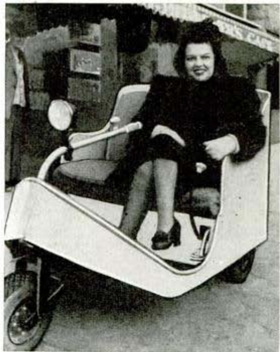
Levers control $60 car's speed, brakes and steering
