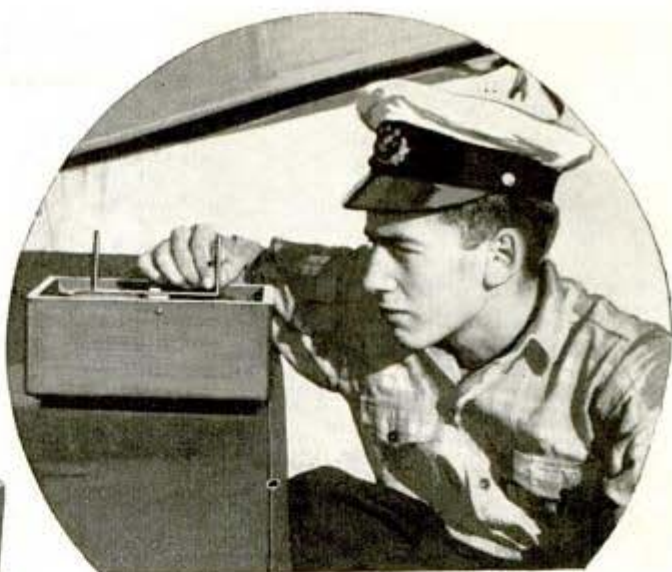
The photo above shows the pelorus used in a sailboat, the pelorus being placed even with the edge of the cabin, which is square with the fore-and-aft line of the boat
