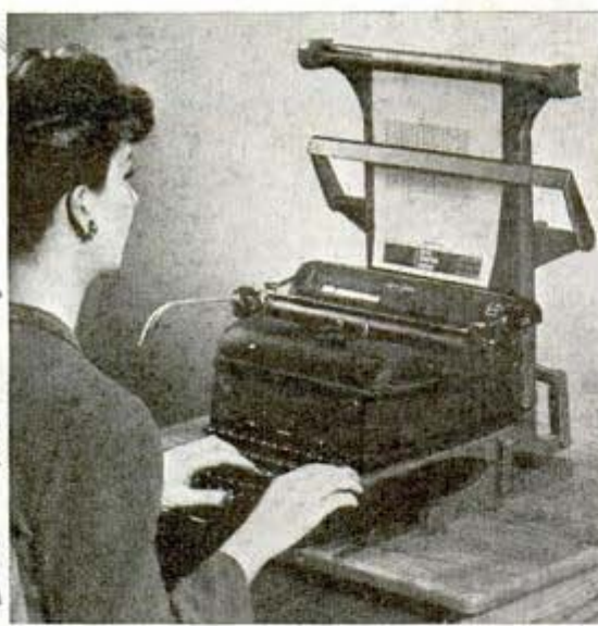
Fingertip pressure on lever keeps copy at eye level
