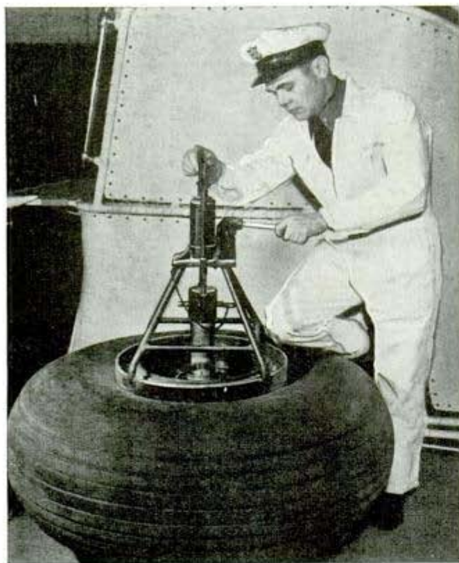
One-man hydraulic jack removes airplane's tire for inspection
