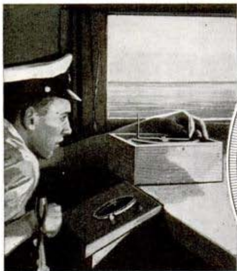
Here the pelorus is being used on a motor boat. In this case the box is aligned with the front edge of the chart table, which is at right angles to the fore-and-aft, or lubber line of the ship
