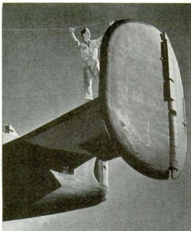
A mechanic checks the radio antenna wires on tail of Liberator
