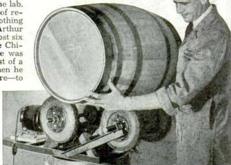
Ingenious mixer consists of four rollers turned by motor. Barrel contains substances to be mixed
