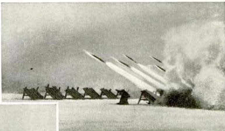
Operated by remote control and with lightweight mounts that can be moved easily, Russian rocket guns fire stream of shells
