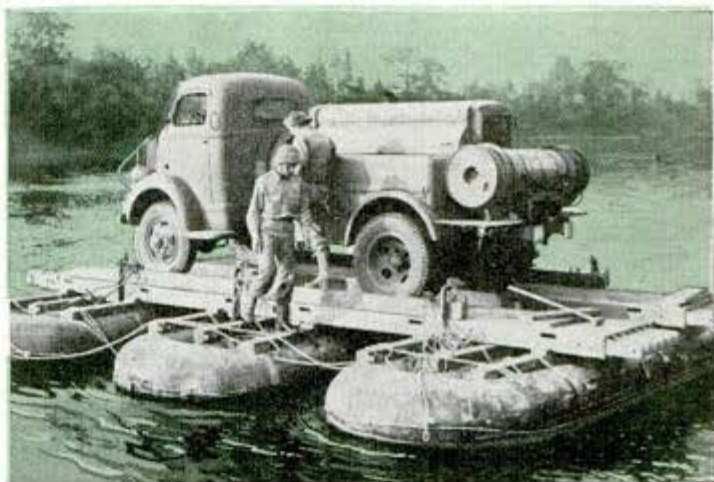
Cadets ferrying army truck on pontoon raft. Their laboratory for amphibious warfare is Lake Popolopen at the Point. Below, aiming one of the heavy field artillery pieces on the academy's new range
