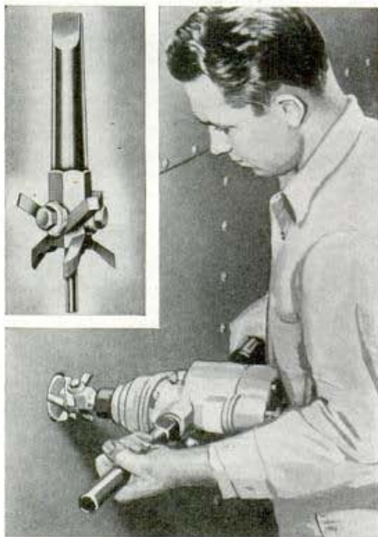
Cutter at work and, inset, three adjustable blades
