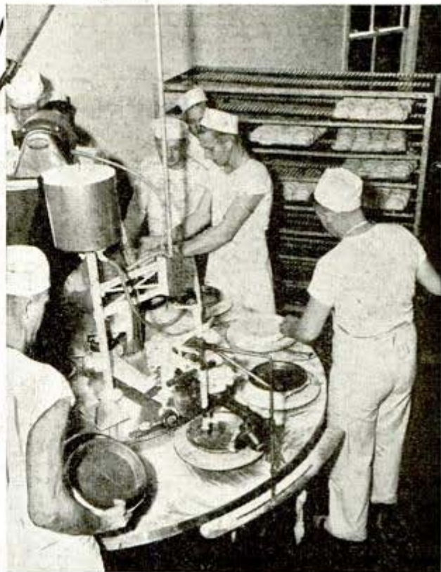
Pie-making machine above, operated by a seven-man baking team, multiplies production of one of the Navy's favorite desserts, turning out 900 pies an hour. Among the billion pounds of foods consumed by the Navy last year, 33,200,000 pounds were dried and canned fruits
