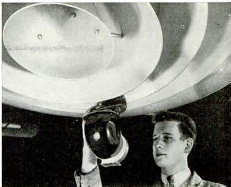
All the foundation's work aims at lessening industry's headaches. Here, expert measures the flow of air through the outlet of ventilating system
