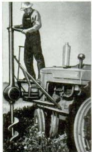
Holes up to 40 inches deep are made by tractor-driven digger
