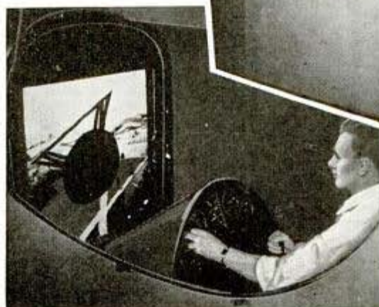
Picture strip with a plane's nose silhouetted, top, shows student craft's reaction to controls. Left, a student in cockpit
