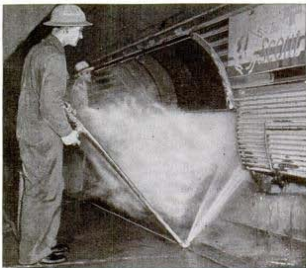
From cowcatcher to cab, the big steam locomotive (above) of the Santa Fe Railway gets a general washing and cleaning upon arrival at the Chicago roundhouse. On a special wash rack, road dirt and grease are removed with mixture of steam and cleaning solvent released from high pressure jet. Locomotives must be kept in tiptop shape these days to help carry the greatest tonnage of war goods in history—thousands of tons of tanks, guns, food, bombs
