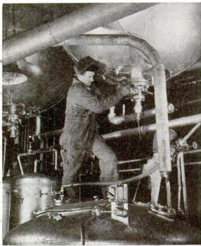
Sealing a radio transmitting tube with a gas "flame thrower" in Westinghouse plant. Below, tapping a tank in synthetic rubber factory; natural gas is converted into butadiene OWI photo
