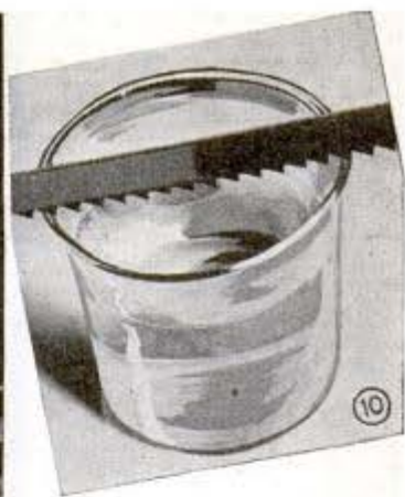
8—Teeth are milled in as many as forty saw bands at once, the bands being clamped side by side in an air-operated vise. 10—Acid test shows exact depth of flame-hardening on saw bands by discoloring hardened portions. 9—Tooth-setting machine that shows a magnified image of the teeth between limit lines so that operator can detect errors of set at a glance. The circular insert shows image as seen
