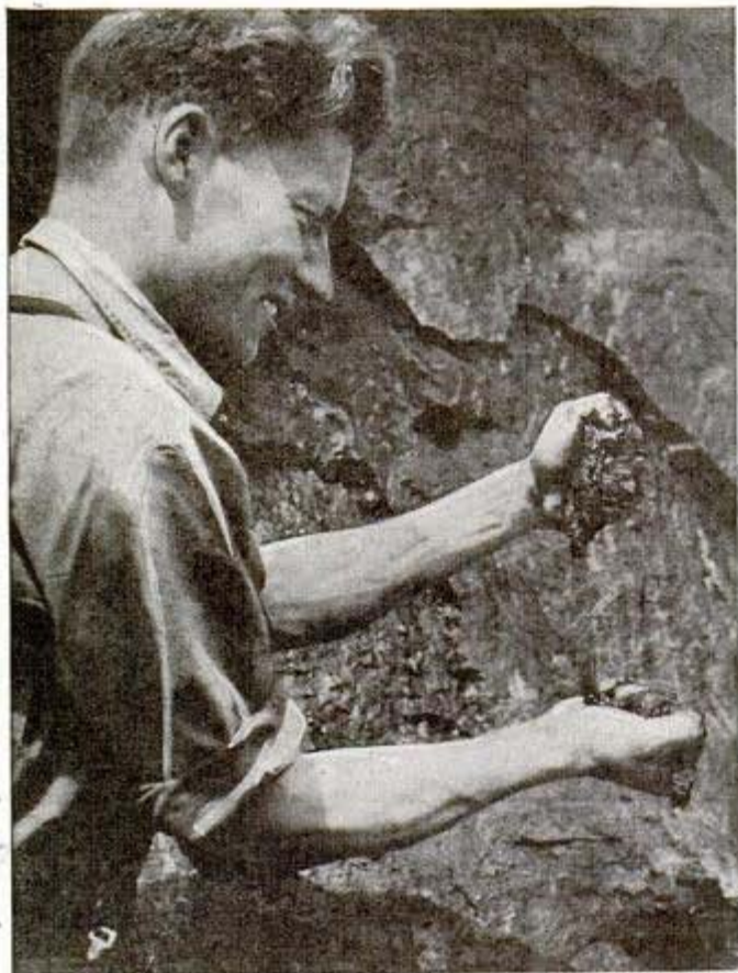
Left, squeezing oil from gummy oil sands deposit in Canada—world's oddest "mine"
