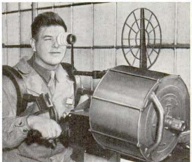
Redesign of the shoulder rests and sight of the Oerlikon ack-ack gun makes it easier for left-eyed, broad men to use it
