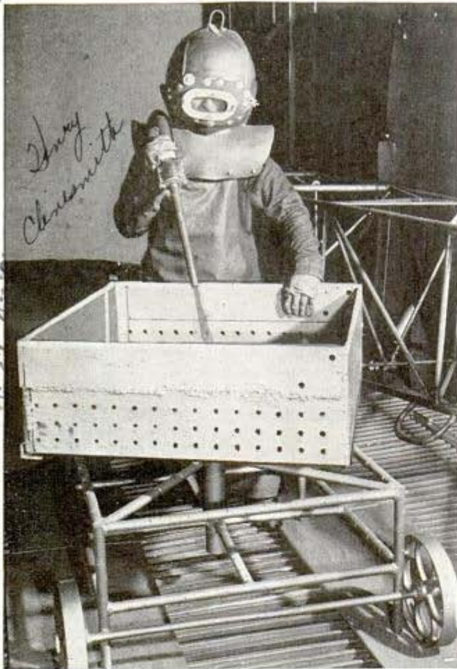
Looking like a deep-sea diver out of his element, this sandblaster cleans airplane parts held in a perforated metal box
