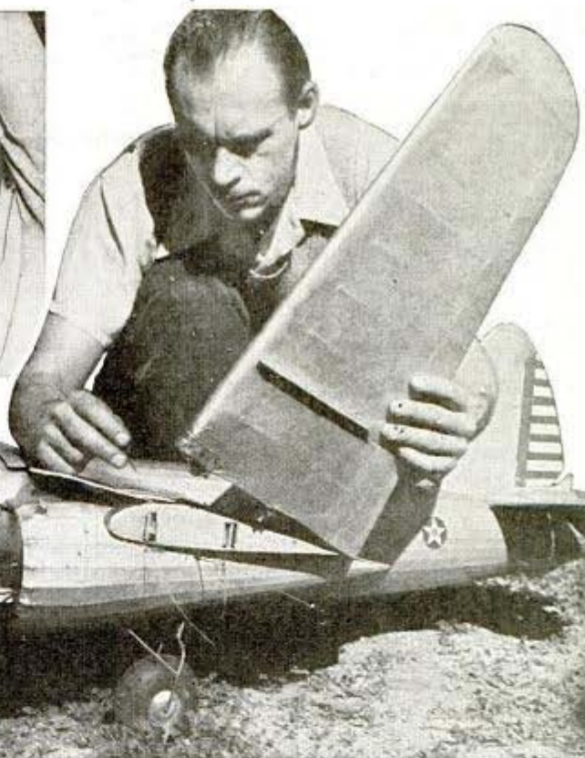
Models are controlled by lines that operate the midget plane's elevators, connected to the 100-foot guide lines (top). Above, attaching the wings of Martin bomber model. Planes can be made to zoom, loop, hedge-hop—to perform almost any plane maneuver except barrel rolls—during dogfights
