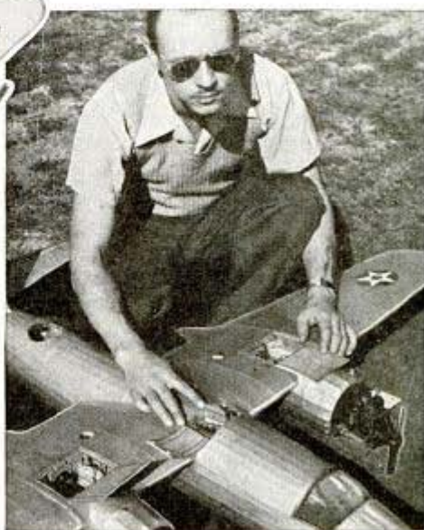
Open compartments above contain batteries and controls to kill motors during flight
