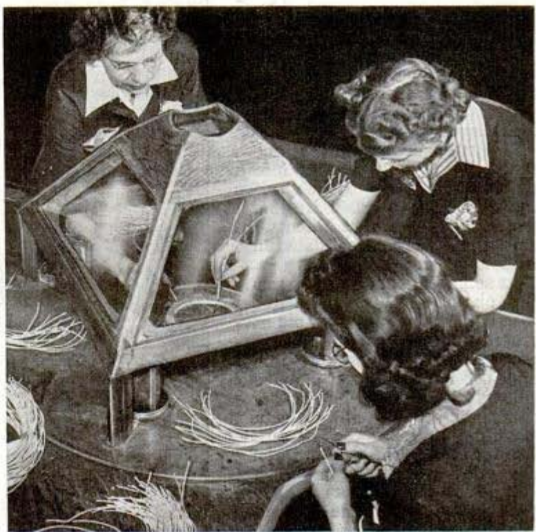
Glass shield protects workers tipping wires from flying bits of solder
