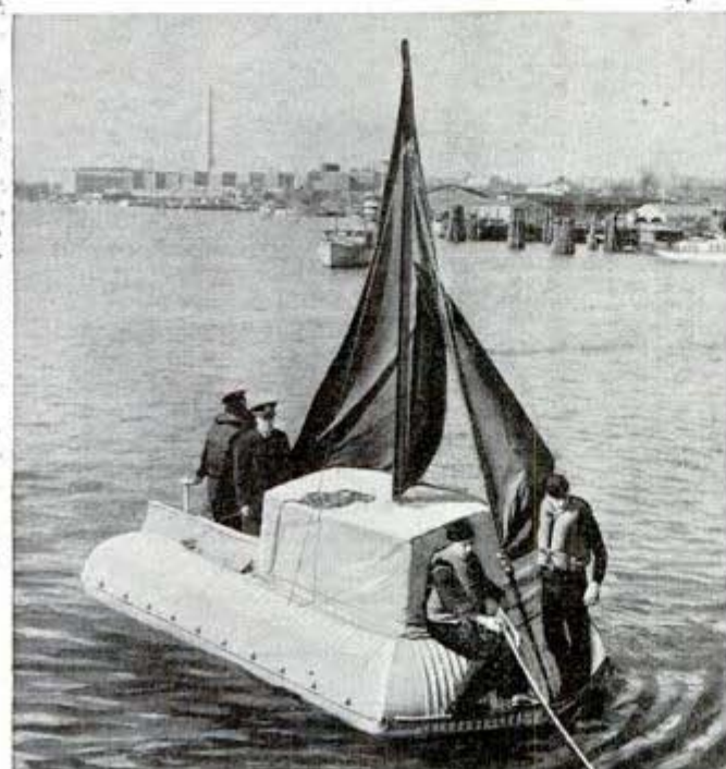
Metal sailing liferaft for merchantmen also has steering gear
