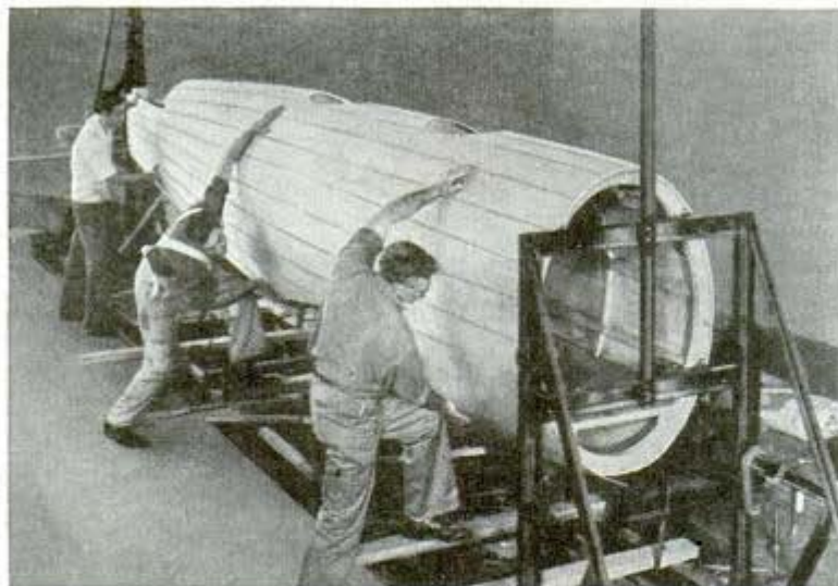
Joining the two halves of fuselage shell of Timm plastic-plywood trainer
