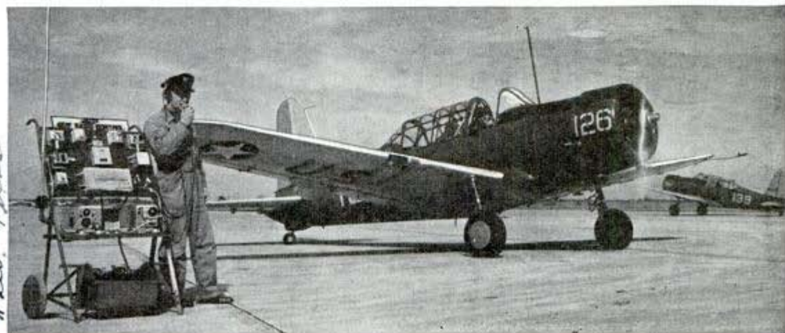
Carried in a jeep and ready for operation less than a minute after it arrives at an auxiliary field, this portable control tower saves grounding a plane merely to use its radio for messages
