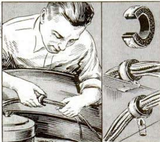
Wire harness attaches in place in a variety of ways
