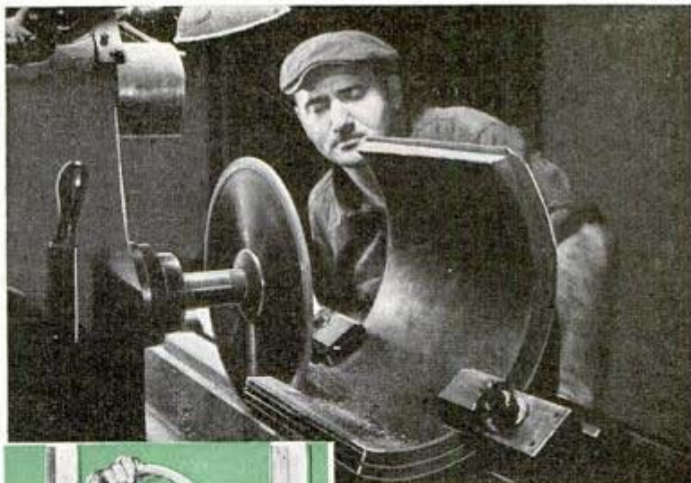
Top, machining a bearing made of Micarta, a Westinghouse laminated plastic, which will carry a million pound load in a steel mill. Micarta is molded under 6,000 lbs. pressure
