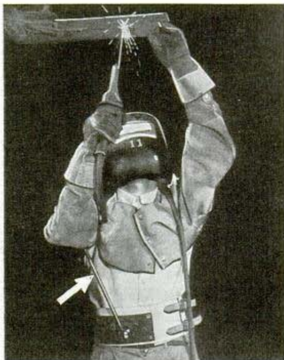
Upright (arrow) is adjustable to suit welder's height
