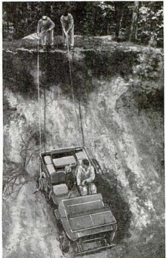
Oversized hub on jeep carries rope that is attached at top of gulley, and revolving wheel lifts machine
