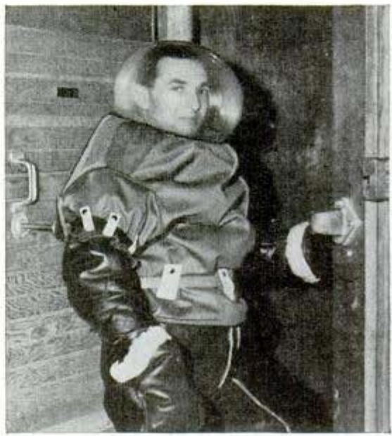
Lucite helmet permits clear vision in cold-test room
