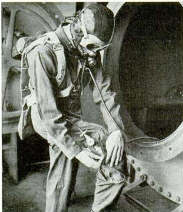
Entering the Boeing "stratosphere chamber," the pilot zips an emergency oxygen bottle into the leg of his flight suit
