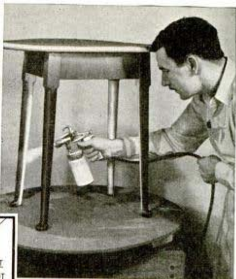
CHECK POSITION OF FLUID TUBE AND MAKE GUN ADJUSTMENTS
