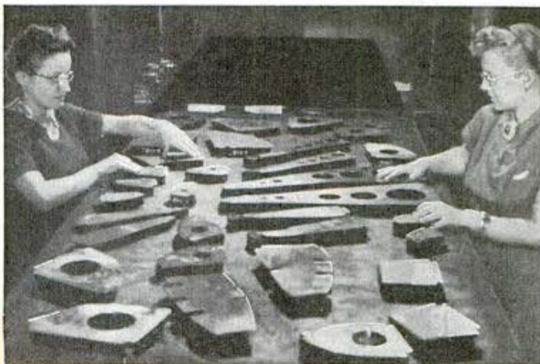
Photos courtesy Pullman-Standard Car Manufacturing Co. Placing templates (above) into which giant press will force aluminum alloy to form wing braces, ribs
