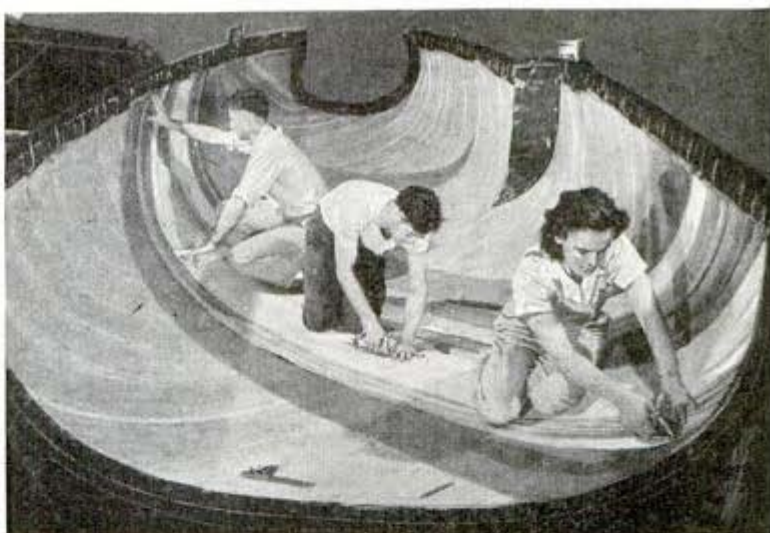
Alternate strips of veneer and adhesive are laid out in dies in the Duramold process, which uses fluid pressure applied through flexible platens in an autoclave, or huge tank—a variety of "bag molding." Workers above lay out strips to form the entire quarter section of training plane
