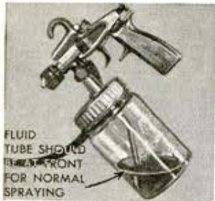
CHECK POSITION OF FLUID TUBE AND MAKE GUN ADJUSTMENTS
