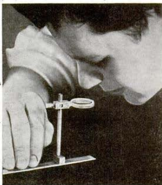
Plastic magnifying lens assures accurate scale reading
