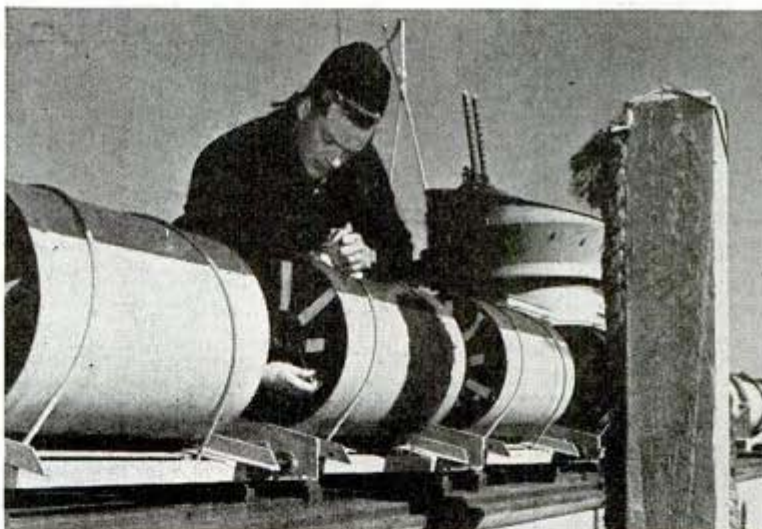
PT boat's "ashcans" may be set to explode at pre-determined depths, to assure maximum force of concussion is exerted close to submarine
