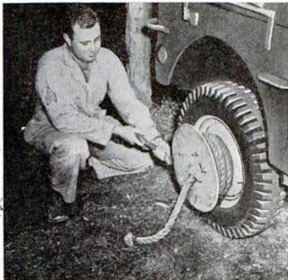
Oversized hub on jeep carries rope that is attached at top of gulley, and revolving wheel lifts machine
