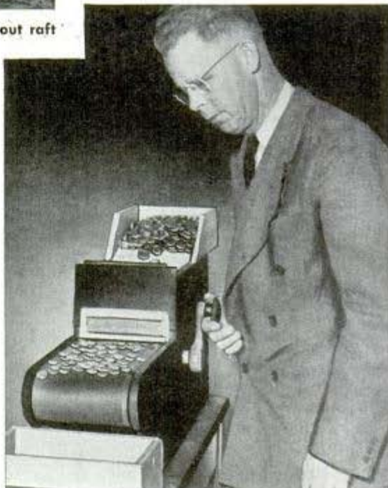
Hand-turned endless belt lets inspector reject slugs
