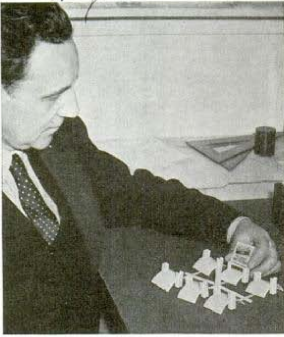
Plastic holders for book matches are cast six at a time. This half-dozen have not yet been separated
