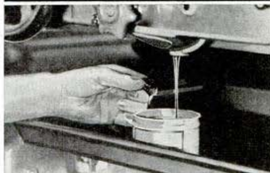
8 APRON OIL RESERVOIR IS DRAINED, FLUSHED WITH KEROSENE AND THEN REFILLED WITH SUITABLE OIL
