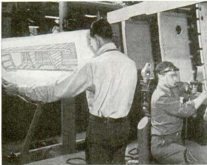
Design changes aim at more efficient use. The perspective sketch used in aircraft plant, above, is more easily read than blueprint. The table-top electrical cooking unit (below) has a separate oven
