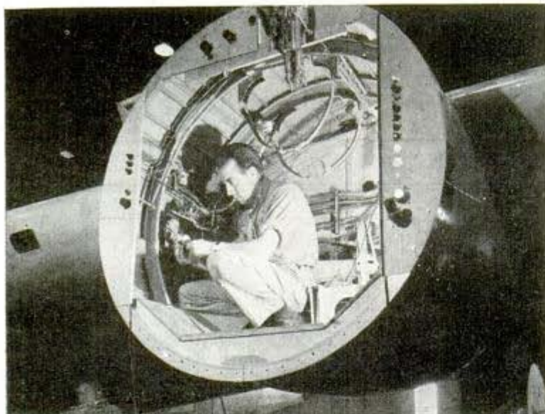
One engine can be removed and a new one installed in 45 minutes with these connections
