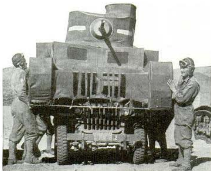
Placing a dummy tank made of pipes and canvas on a jeep's chassis
