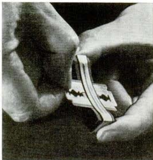
Clip keeps constant honing pressure on razor blade
