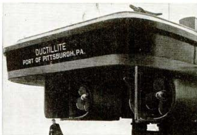
View of towboat above shows how Kort nozzle encircles propellers. Below, loading cars on a Commercial Barge Line 3-decker
