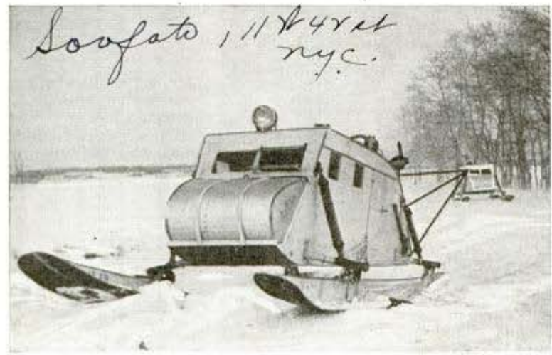
Driven by an airplane-type propeller, airsleighs are used on snowy terrain
