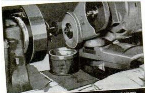
12 CATCHING EMERY PARTICLES FROM A GRINDING WHEEL IN A CAN OR CUP CONTAINING OIL OR WATER
