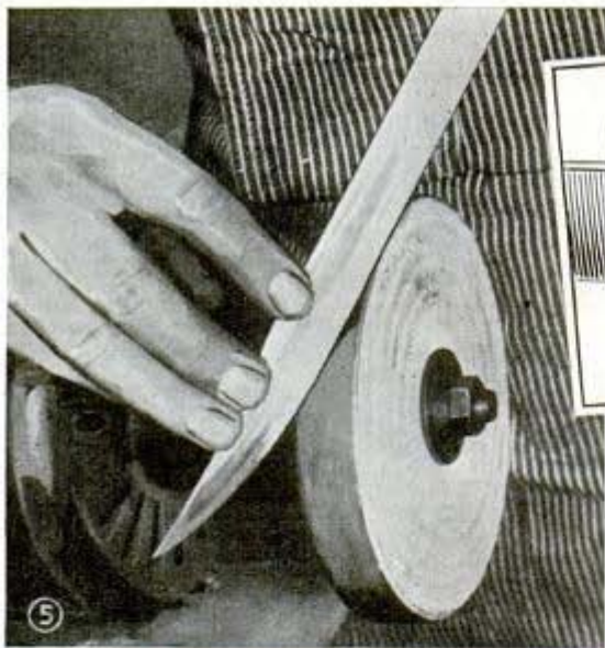
USE "GREASE WHEEL" TO REMOVE GRINDING MARKS
