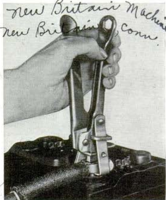
Pressure lifts corroded terminal from battery post
