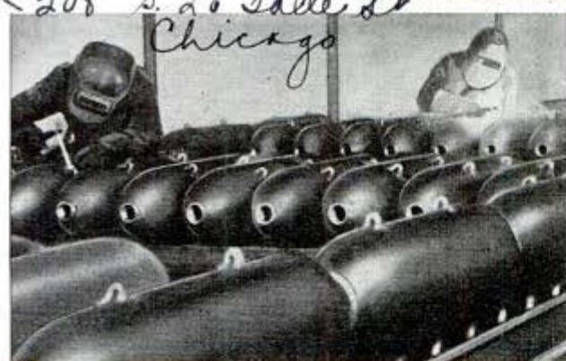
Glowing bomb casing above is shaped as a potter's finger shapes a vase. Below, carrying lugs are welded to casings
