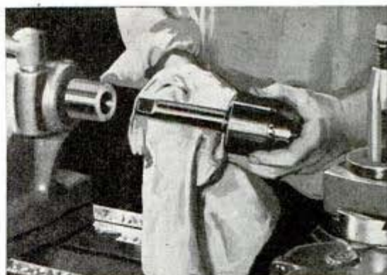
7 WIPING CLEAN THE TAPER SHANK OF A DRILL CHUCK BEFORE MOUNTING IT IN THE SPINDLE TAPER
