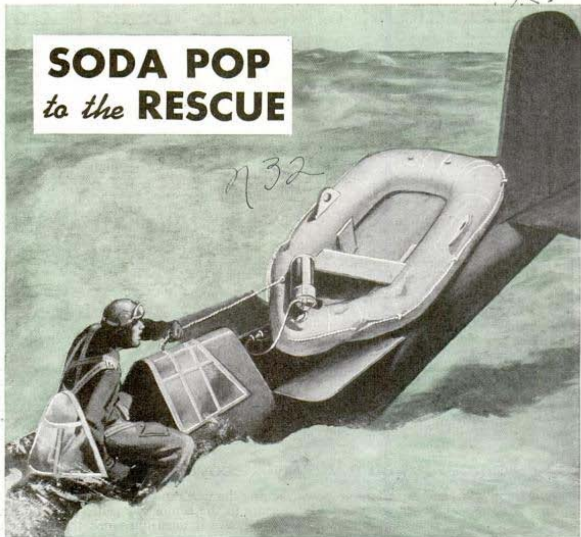
Life raft is automatically ejected from top of fuselage and inflated with carbon dioxide as plane hits water. Below, it takes about 30 seconds to snuff out gasoline fire this way Walter Kidde & Co. photos
