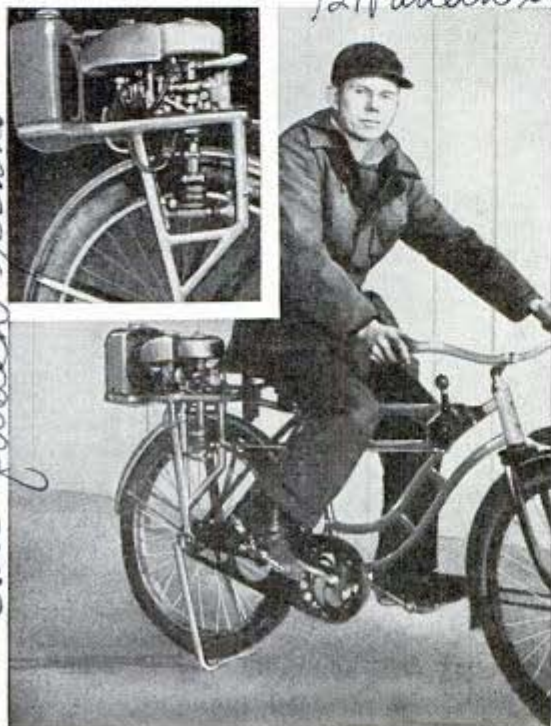
Outboard motor's water jacket is from an auto heater
