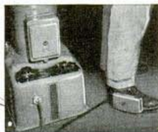
Control strapped like skate to his foot allows welder to move
