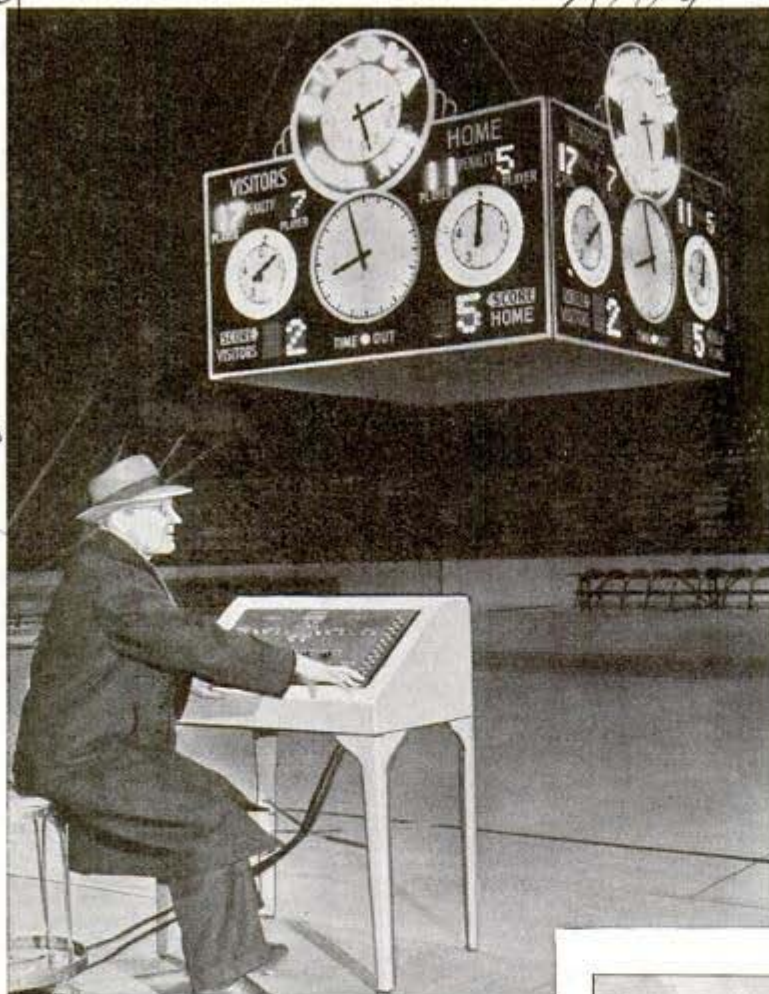
Lights, bells and sirens are controlled from board
