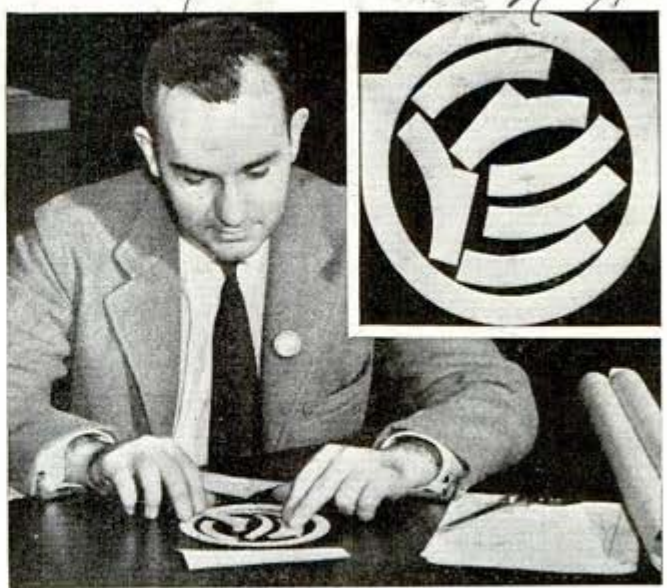
Pattern layout permits cutting of most parts from least metal
