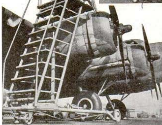
Mobile service platform, from which mechanics can reach all parts of an airplane, folds for towing behind an automobile
