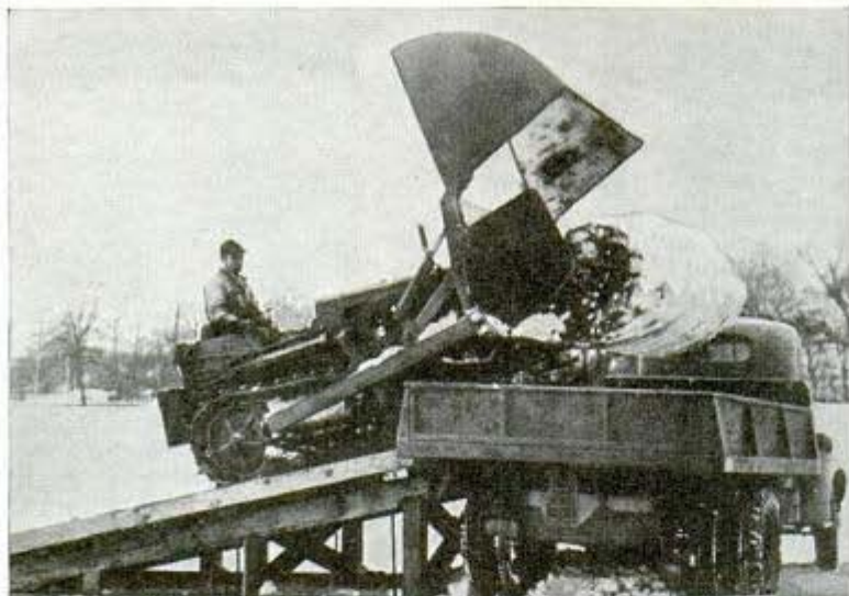
By packing it as it lifts, tractor-propelled clam shovel removes more snow
