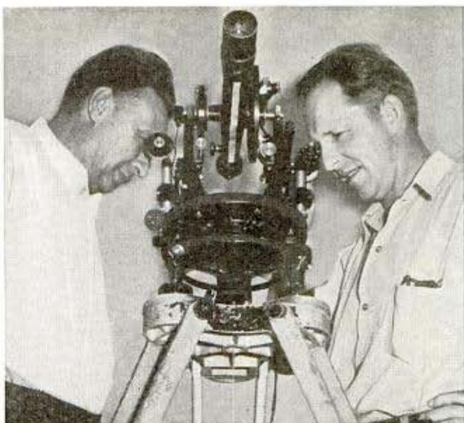
↑ Surveyors making readings simultaneously on theodolite to reduce errors
