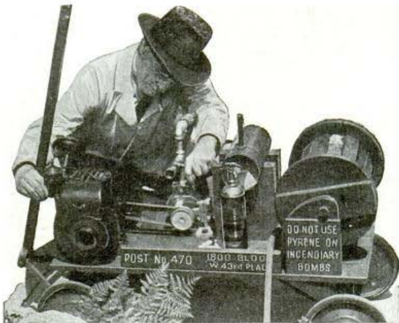
Air raid wardens, working in backyard workshops, constructed this portable pressure system for fighting fires as a safeguard against bombing
