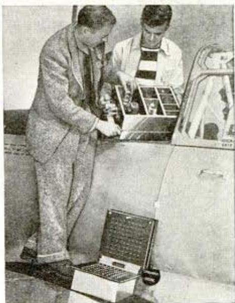
Recorder on ground (top) receives report of performance at 70 points on plane during test flight. Lower photo shows engineers installing transmitter in new plane
