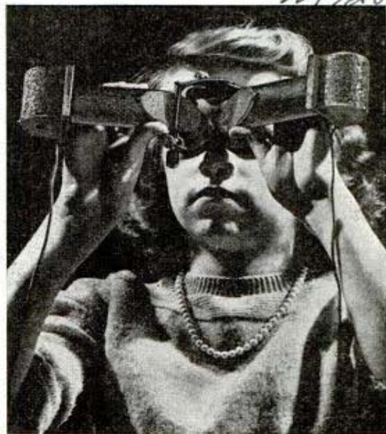
Double-tube optical instrument trains crossed eyes
