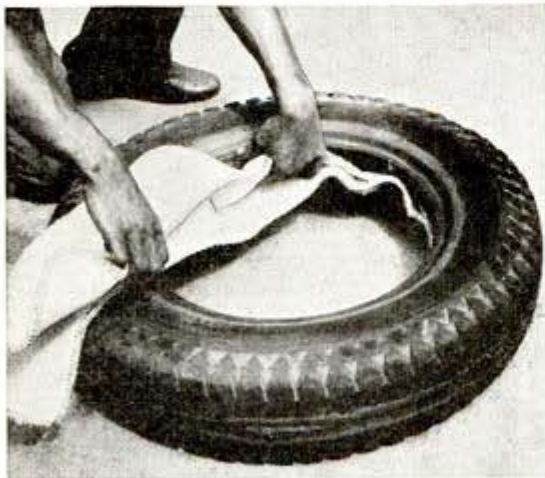
Liner goes between tube and casing, fits any size
