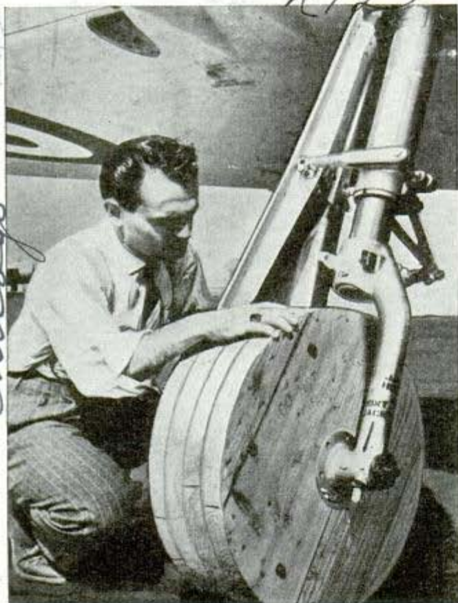
Fighter plane's wooden wheel saves rubber during ground tests
