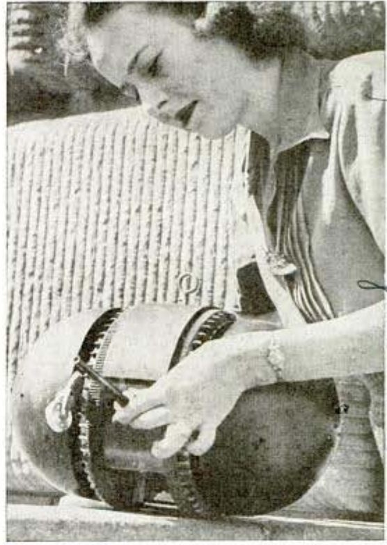
Model of roller tank shows end mounting of wheels
