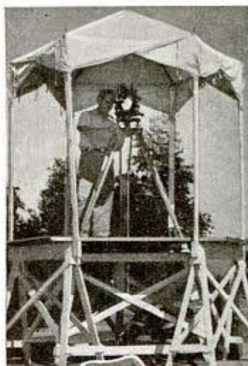
↑ Surveyors making readings simultaneously on theodolite to reduce errors
