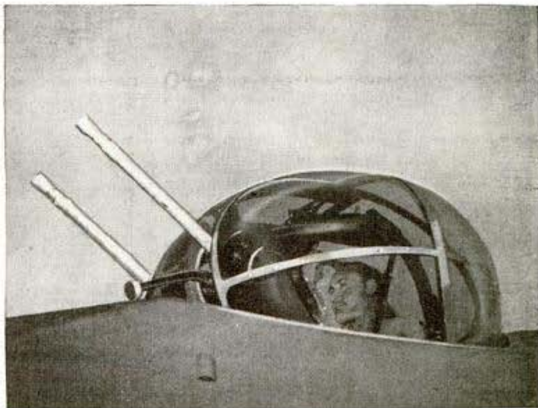
This is the upper gun turret of a 4-motored British "Lancaster" Douglas Aircraft Co. photo
