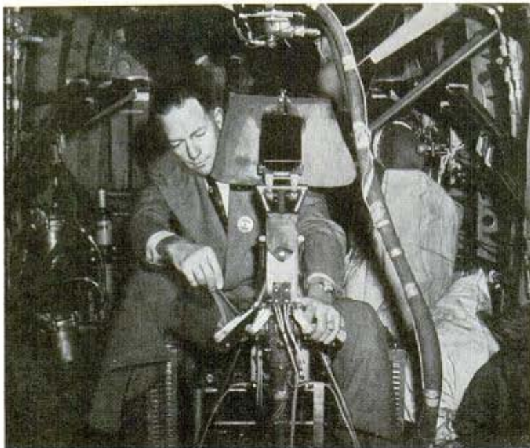
A Douglas engineer tests the controls of a "Lancaster's" belly guns, his left hand on trigger. He is leaning past periscope used for sighting guns
