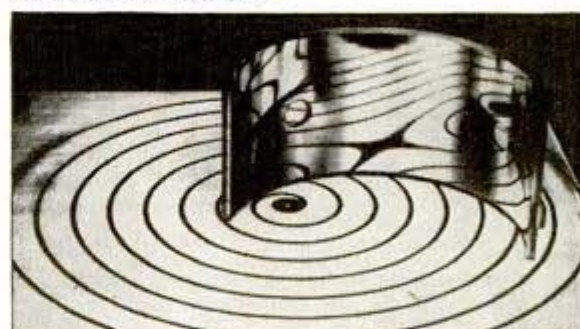
Tattle-tale. Inspecting a polished bearing surface is tough under ordinary light. But place it on a smoothly lighted diffusing glass with lines on it; clean-cut reflections say "OK", distortion says "roughness".
