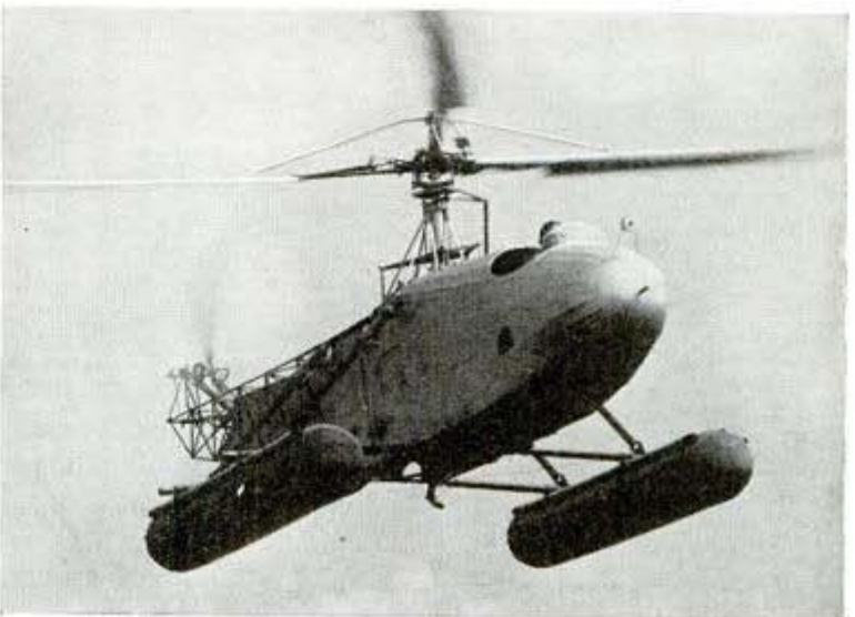
The outriggers were dropped in the first major revision and a tower over the tail substituted (above), carrying a single rotor. In the present version the tower has been scrapped, pontoons replace wheels
