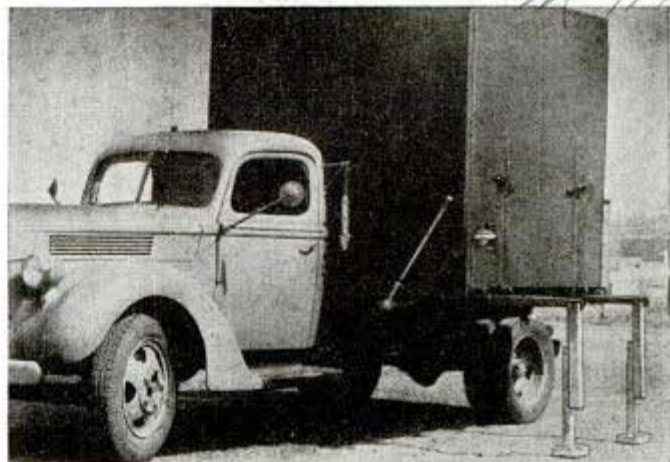
Demountable body is moved on or off truck chassis by one man
