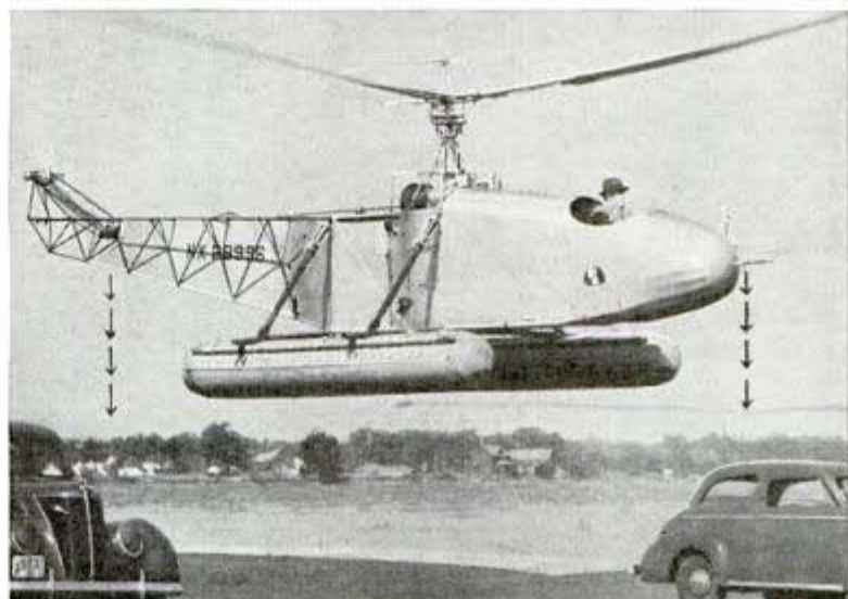
Mr. Sikorsky sets the VS-300 down between parked cars, in a space just wide enough to allow clearance of the fourteen-foot main rotor blades
