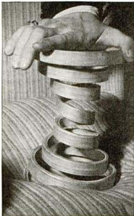
Foregoing use of steel springs to conserve metal, the furniture makers have devised substitutes of noncritical materials, chiefly wood. Above, a double-conical coil, collapsing within itself, made from thin, laminated wood strips
