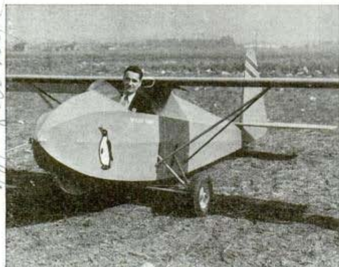
Student learns proper use of plane controls in pre-flight training glider which is towed around field by automobile
