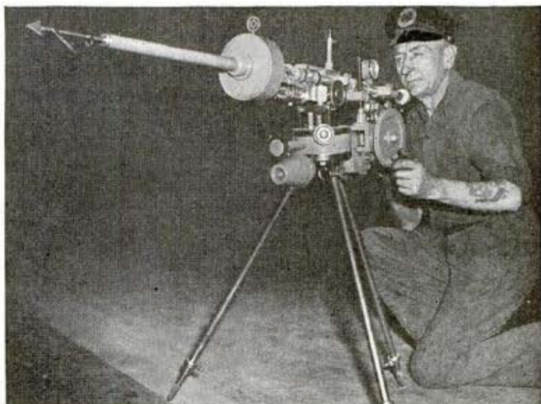
↑ Here is a compressed-air harpoon gun used for shark fishing. Air is discharged into barrel behind the harpoon by means of electromagnetic valve
