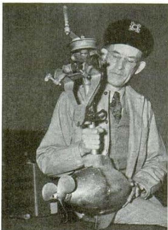
Battery-driven outboard engine has electric motor in streamline housing in front of screw. Crank is for slow speeds
