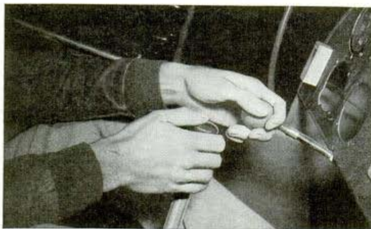
This is how a glider pilot cuts loose from his tractor plane, releasing the tow line when his craft is ready for a glide to earth. Below, beginners get the feel of parachute and harness before they start the rigorous aerial course at Fort Benning, Ga.
