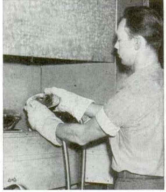
Low pressure hose extends into each asbestos glove with cool air to prevent burns on hands of worker
