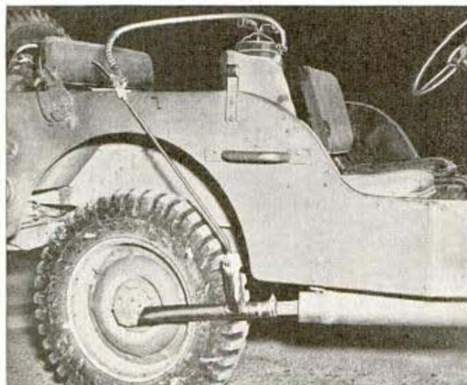
Pressing lever by seat sprays fluid into the hot exhaust pipe
