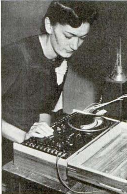
Left, multiple temperature indicator used to check temperatures of different parts of body in research on common colds. Right, attaching the leads for measuring temperatures at various points on a subject's arm
