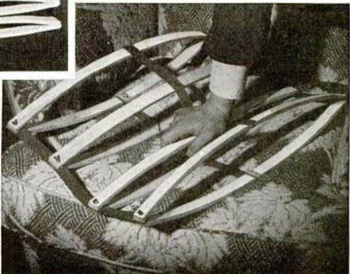
"Bouncy" foundations for innerspring mattresses still in dealers' hands, and for the cotton felt mattresses coming into use, are achieved by a base made of wooden slats held in a bowed position by round wood blocks, shown installed on bed above
