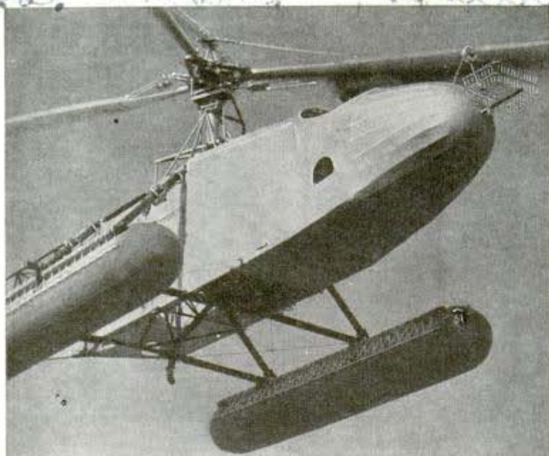
Ingenious controls in main rotor mast permit sidewise, backward, forward or vertical maneuvers
