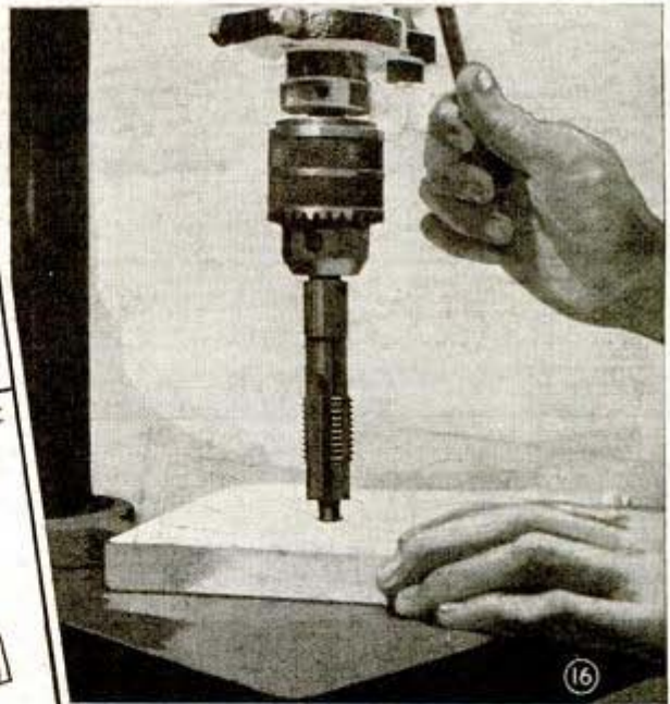
COUNTERBORE MADE FROM TAP
