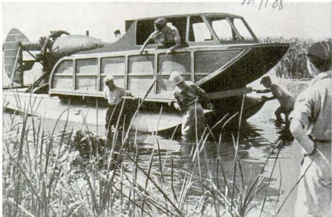
Driven by an air propeller and riding on pontoons, rescue boat is efficient in deep or shallow water
