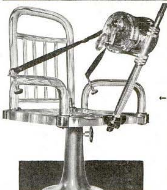
↑ Here is a compressed-air harpoon gun used for shark fishing. Air is discharged into barrel behind the harpoon by means of electromagnetic valve
