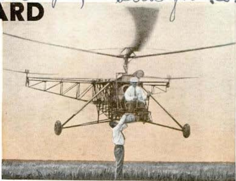
In this panel are the three stages of the experimental helicopter, first of its breed to fly successfully. The original model, above, had outrigger structures extending from the tail, with twin rotors
