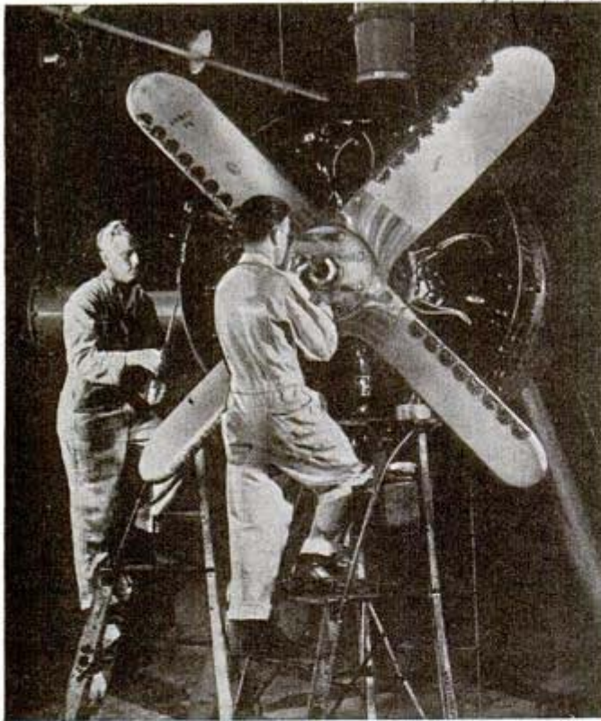
Airplane engine spins this heavy-bladed propeller during test run at the factory; its blades are shaped to cool the engine
