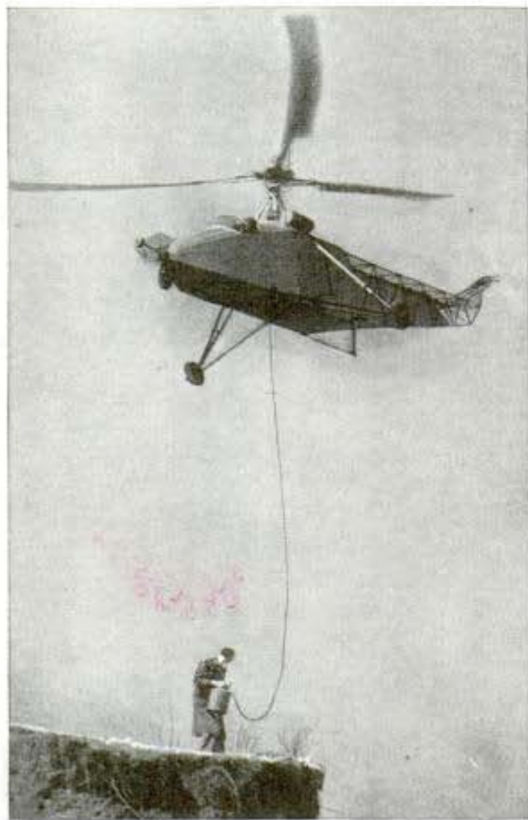
Its arms thrashing just enough to counteract gravity, the helicopter waits upstairs while its "ground crew" attaches a can of gasoline to line to refuel
