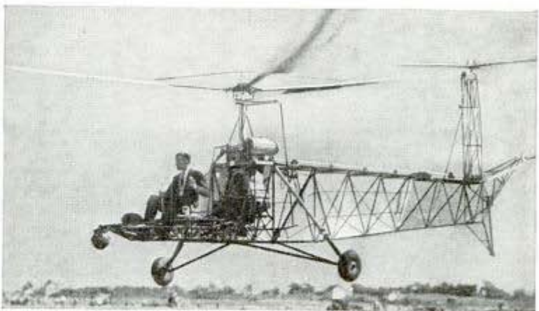
The outriggers were dropped in the first major revision and a tower over the tail substituted (above), carrying a single rotor. In the present version the tower has been scrapped, pontoons replace wheels
