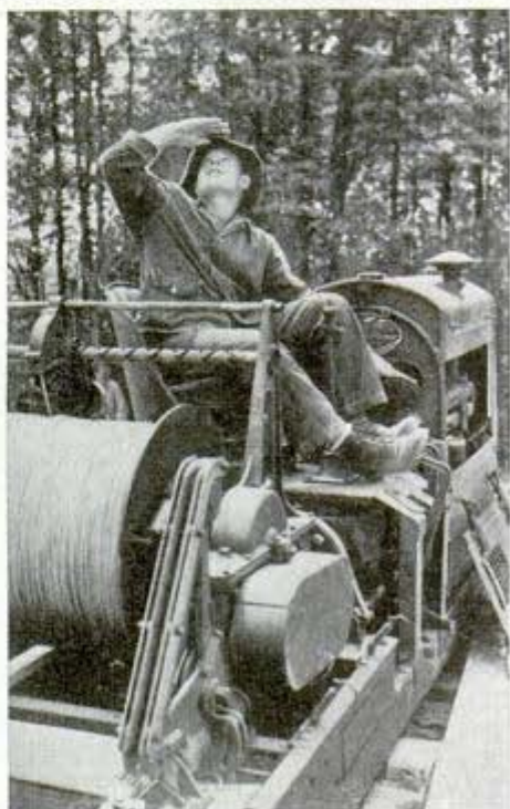
Down she comes, as a motor-driven winch winds in the steel cable holding balloon
