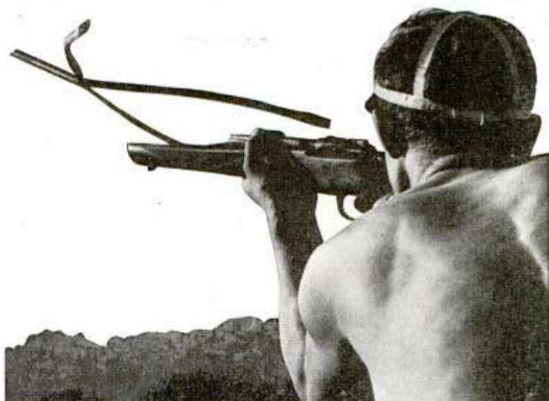
This rifle has a split barrel that burst because of stoppage. In this case the hunter was not injured, but proper care will prevent such mishaps
