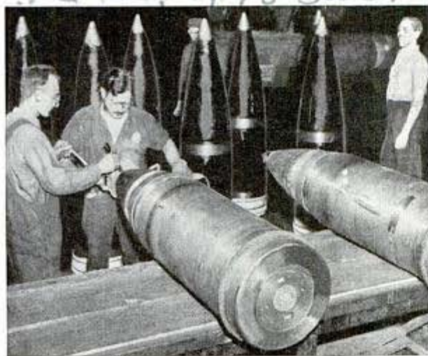
These giant armor-piercing shells carry load of TNT which is resistant to shock of impact
