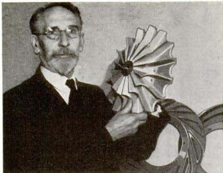
Dr. Sanford A. Moss of General Electric, who pioneered in developing the airplane supercharger for high-altitude flight, demonstrates the impeller
