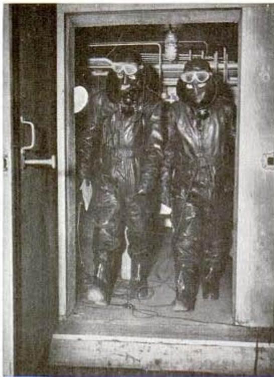
Pilot's reactions to extreme low temperatures above 30,000 feet are tested in Boeing Aircraft Company's cold room. Below, pilots in grotesque flying suits and masks emerge from sub-stratosphere laboratory
