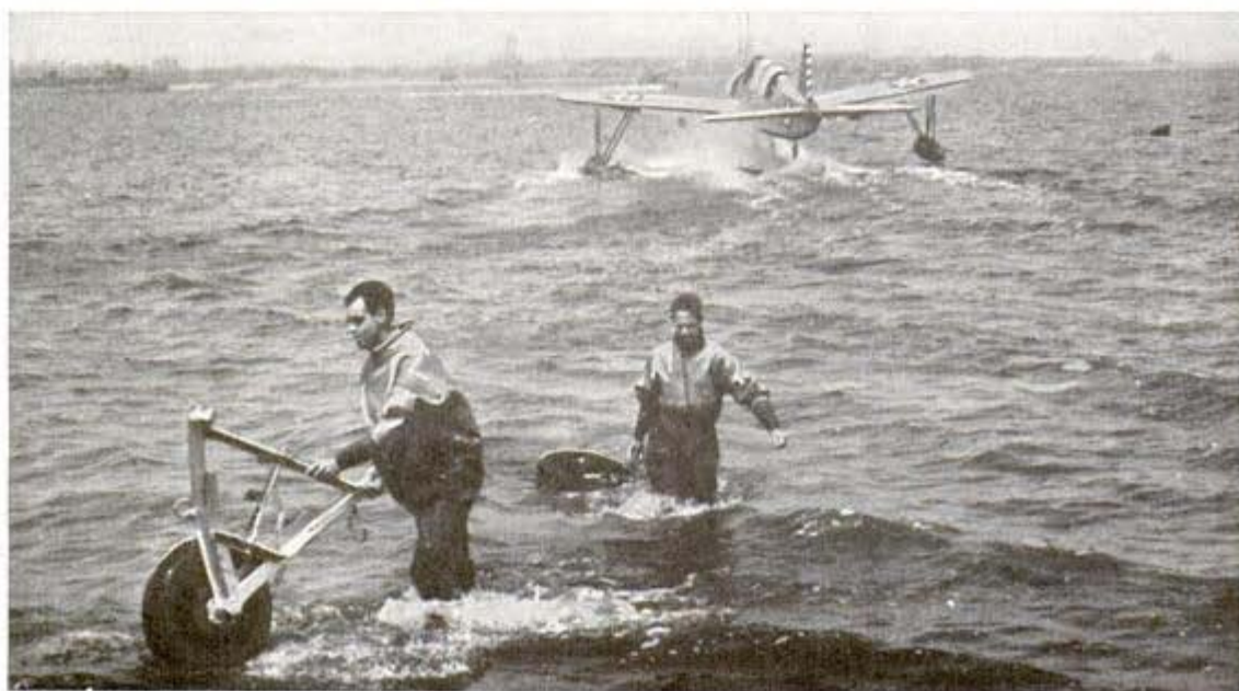
A seaplane is launched from shore in 60 seconds and the men bring back the wheels that rolled it into water
