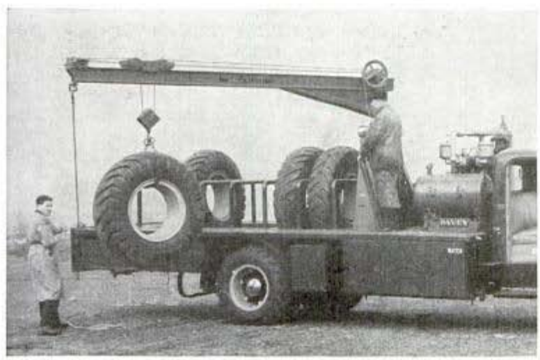
Tires too heavy for a man to lift are handled by crane mounted on truck
