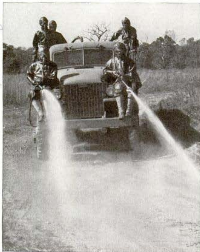
Spraying neutralizing chemicals on a gas-infested terrain from chemical warfare car Photo by A. G. MacNaull
