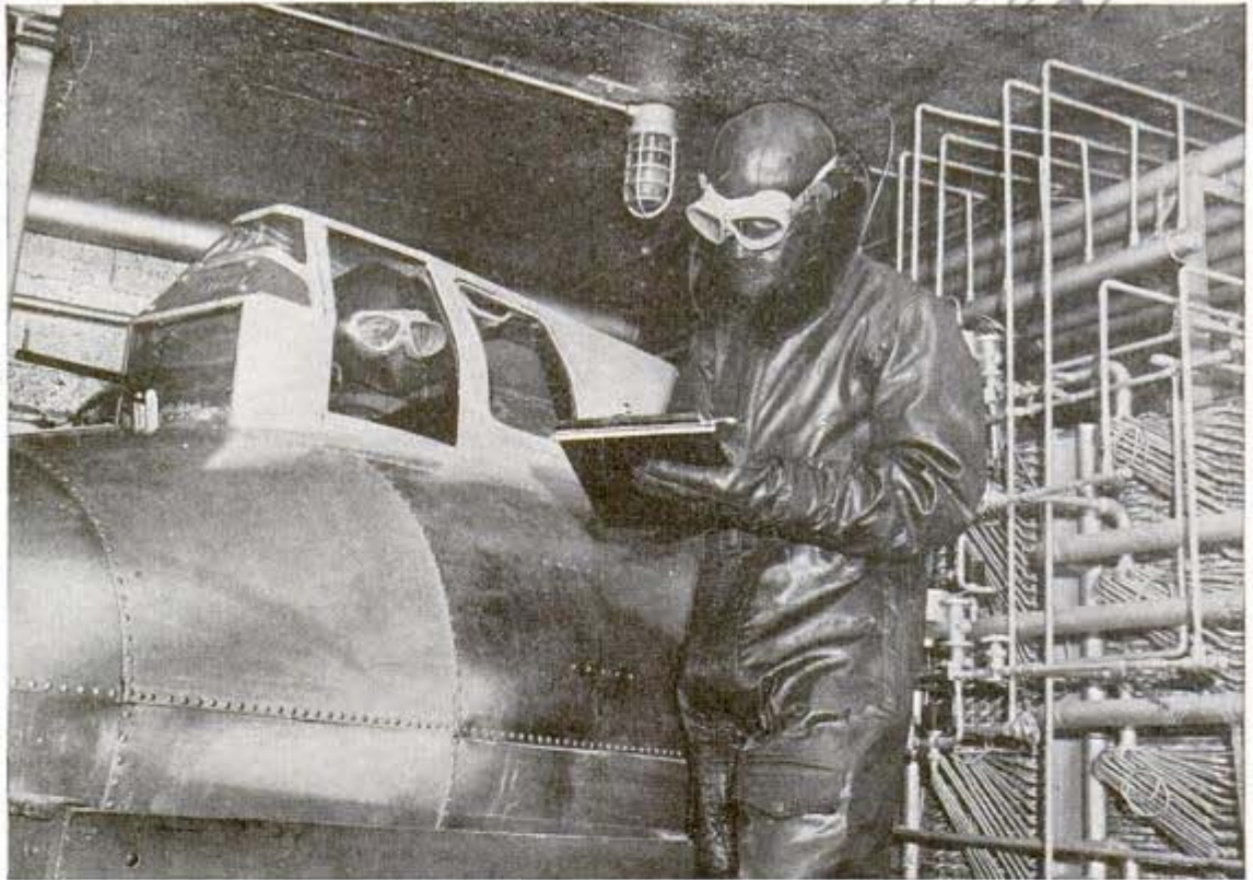
Pilot's reactions to extreme low temperatures above 30,000 feet are tested in Boeing Aircraft Company's cold room. Below, pilots in grotesque flying suits and masks emerge from sub-stratosphere laboratory
