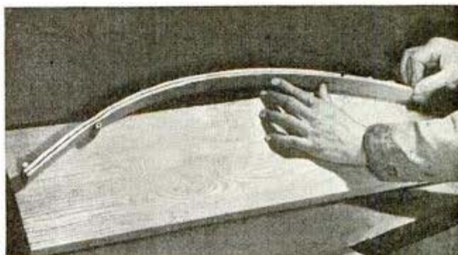
8 First, two glue-coated strips are sprung around dowels set in a flat board and left 24 hrs. to dry
