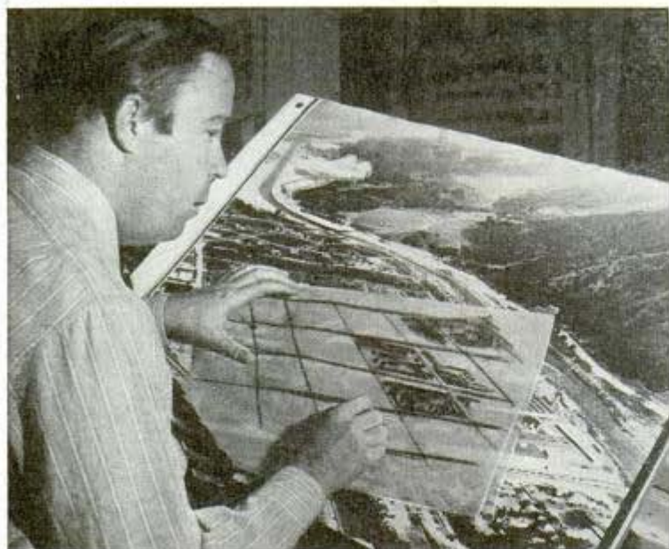
To plan a concealment scheme, the camoufler uses an aerial photo of the plant and sketches on tracing paper various patterns of "confusion"
