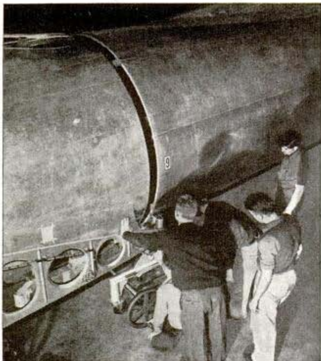
Fuselage sections of a Boeing Flying Fortress are assembled
