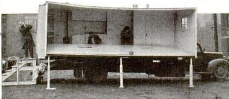
Any magician would be proud of this trick—transforming what appeared to be a big moving van into duplex house for war workers in 30 minutes
