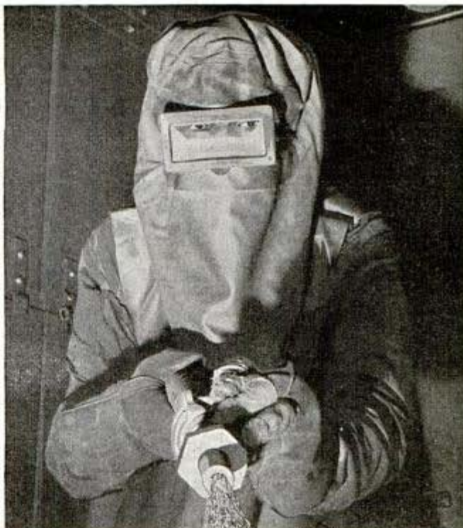
Hooded shot blaster in Westinghouse plant fires metal shot from nozzle to clean motor and other castings 6. Page
