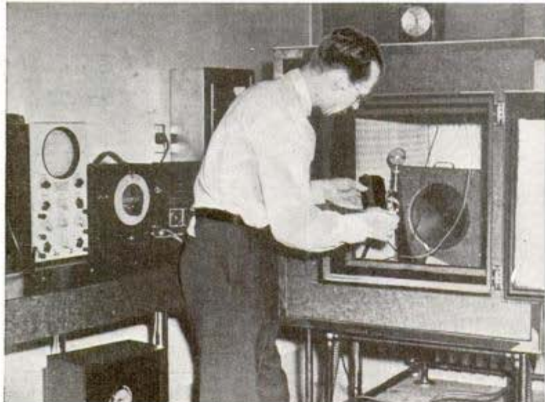
Testing sensitivity of microphone hidden inside a safe
