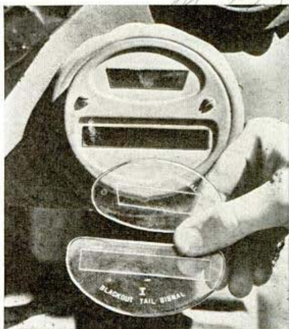
Shields make "jeep" lights invisible from the air
