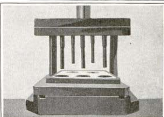
16 COMPLETED PUNCH AND DIE READY FOR SURFACE GRINDING ENDS OF PUNCHES AND DIE PLATE
