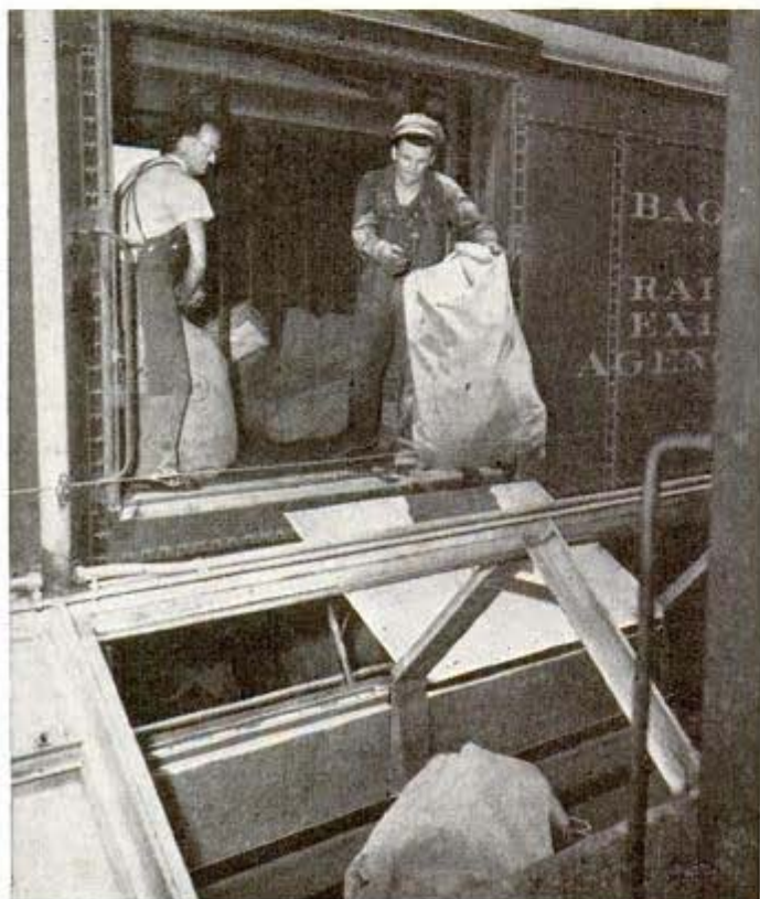
Unloading sacks of mail from a storage car to moving conveyor belt which takes it to sorting platforms inside the post office
