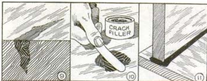
Checks in wood are first filled with wood putty, then top-dressed with stick shellac to match the finish, Fig. 9. Knotholes are filled with nonshrinking paste crack filler, Fig. 10. For sealing seams as at drawer bottoms, use caulking compound, Fig. 11
