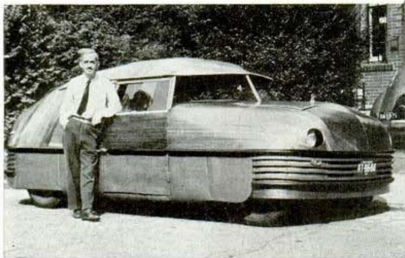
Car with plywood body weighs 600 pounds less than all-metal construction
