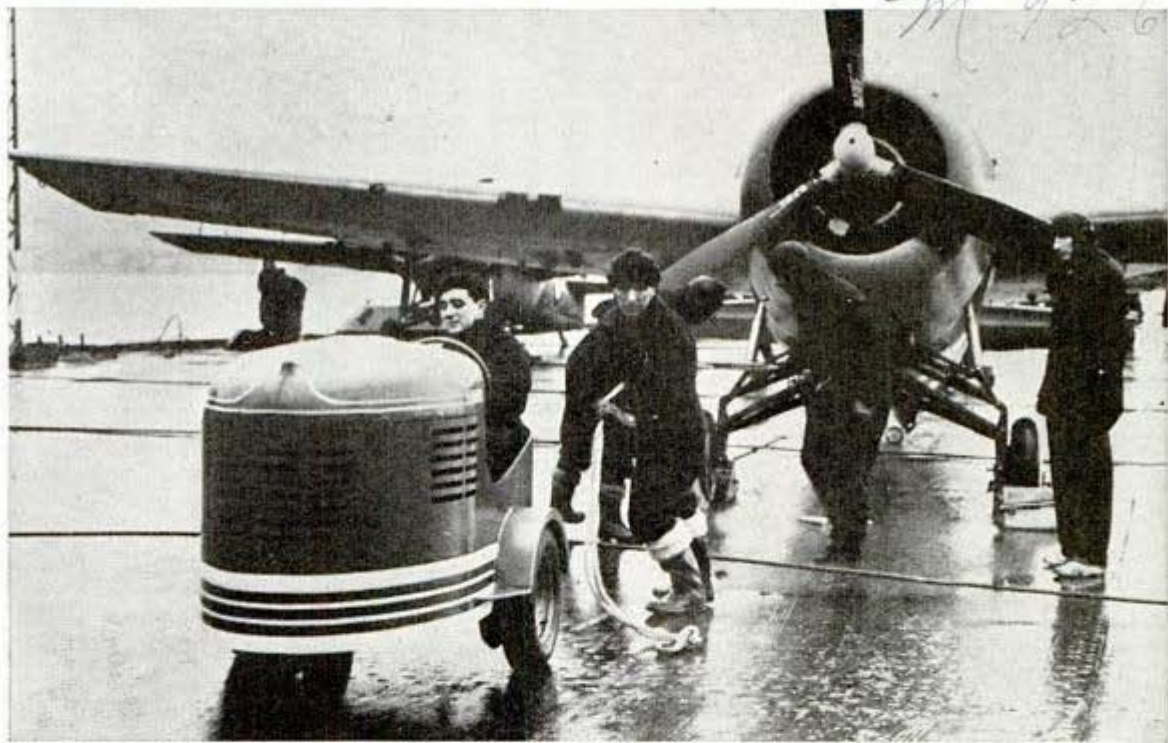
Midget car that "turns on a dime" backs into position to tow fighter plane across British carrier's deck
