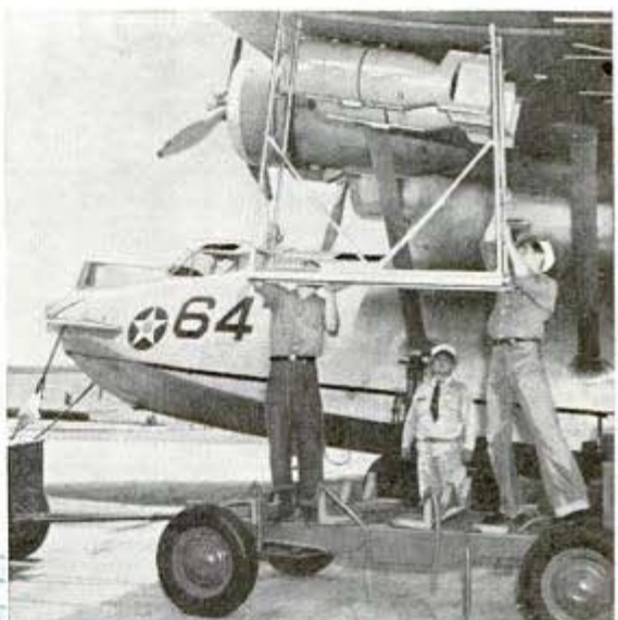
Two seamen (right) remove inspection platform under watchful eye of a chief petty officer. Bomb dolly, below, is pulled under wing of "Cat" with tractor. One man handles a 500-pound bomb with ingenious pulley
