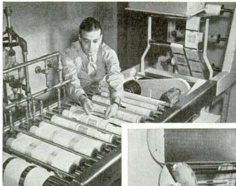
Right, developing and drying film; the lower reel is for developing, the upper for drying. Forty-five pounds of film, which would occupy the space of one mail sack, contain about 150,000 one-page letters. The unfilmed letters would fill some 37 mail bags weighing 2,575 pounds. Where apparatus for developing the microfilms is not available abroad the V-Mail is developed in the U. S. and then shipped, effecting a saving of about 1,000 pounds on 150,000 letters. Army officials laud the V-Mail as a great builder of morale—which can't be weighed
