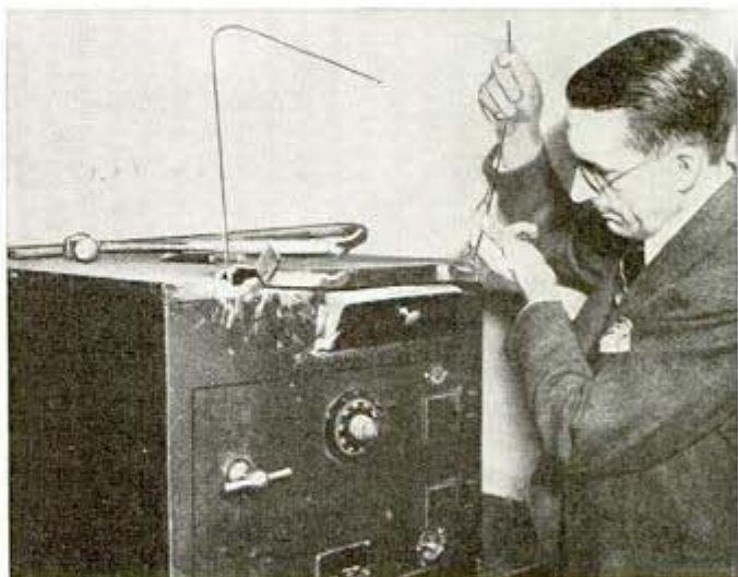
The locking mechanism of this money chest resisted "fishing expedition" with fine wire after hole had been cut in top. Below, oxyacetylene torch is used on steel panel in wall of vault to determine if microphone on other side of wall will "hear" the noise made by attack, thus causing instant alarm
