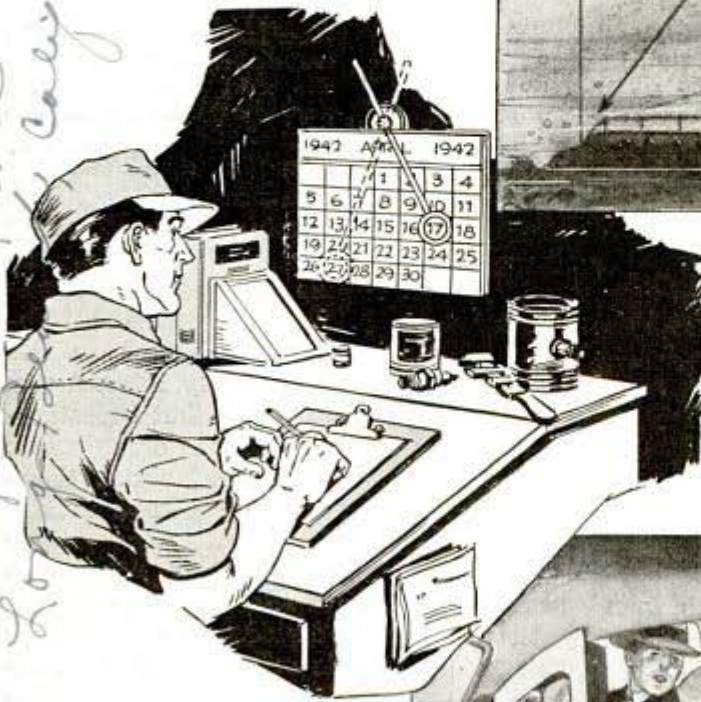
The date indicator, above, is adjusted to any average sized calendar. A rod with ring on the end swings back and forth or slides upward
