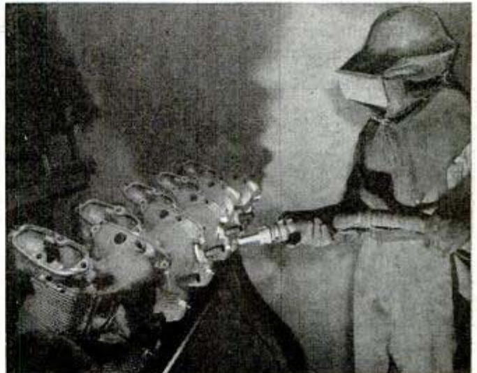
Dirt and fumes in the eyes, ears, nose and pulmonary tract would wear down and slow down the worker, so this American Airlines man is masked as he cleans motor parts with air gun
