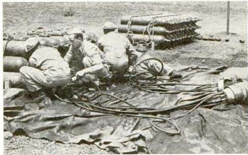
"Feeding the baby" is what crew members call the process of inflating giant barrage balloon → with hydrogen gas. Rubber hoses attached to cylinders carry gas to balloon's "appendix" in nose ↓
