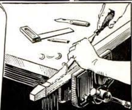
SPADE FOOT AND TAPER ARE FORMED WITH A CHISEL
