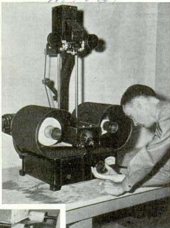
Making enlargements, above, from microfilm is one step in processing the new "V-Mail." Left, continuous rolls of prints pass through machine which develops, washes, and dries the letters which are then ready to be cut. V-Mail results in a tremendous saving in valuable cargo space. The two-way service handles millions of letters to and from men in armed forces
