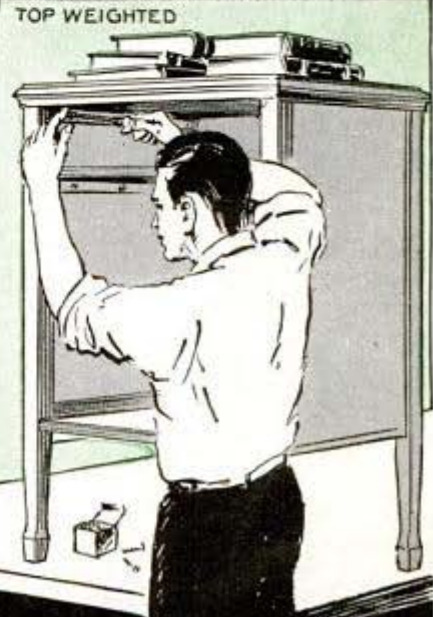
THE TOP ASSEMBLY IS SECURED WITH SCREWS
