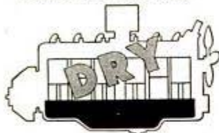
VITAL INNER PARTS OF AN ENGINE LEFT STANDING ARE DRAINED OF LUBRICATION
