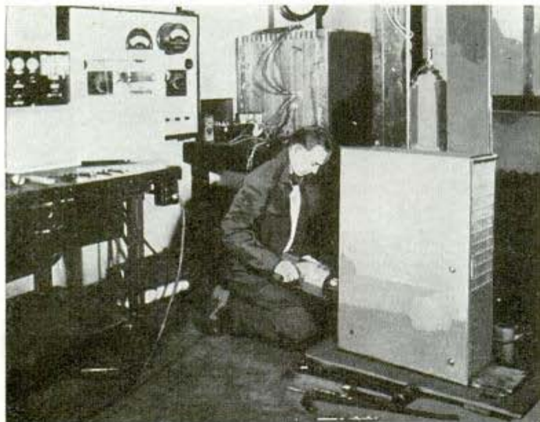
Attempting to "defeat" an electrically protected outdoor alarm box with an electric drill in one of testing rooms at Underwriters' Laboratories
