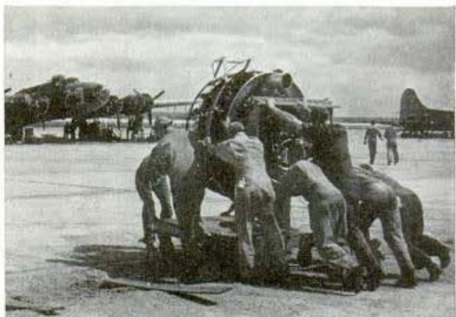
Keep 'em flying is a tough assignment if you mean keeping the Flying Fortresses equipped with efficient power plants. It takes a high degree of technical skill to adjust the four engines, as at left, and a liberal amount of muscular strength to replace "tired" engines with new ones, above, when the mammoth ships return from long bombing missions
