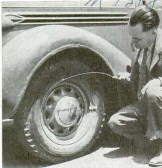
Special lock releases wire when air in tire is low
