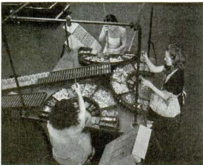
Handy material trays, electric screwdrivers suspended overhead, and conveyors eliminate waste motion and save effort
