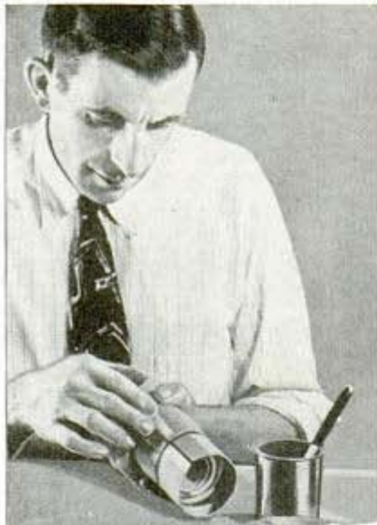
SOCKET ROLLED FROM GLUE- COATED CARDBOARD
