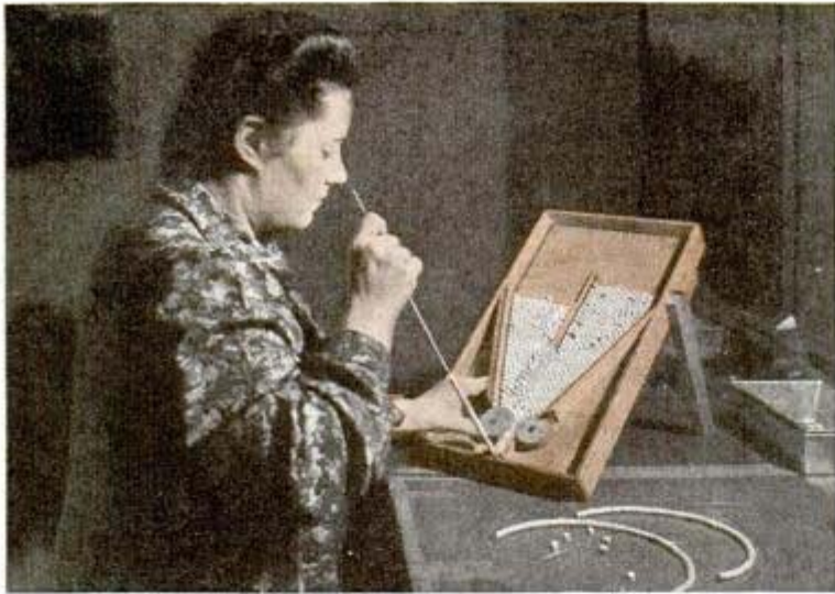
A few shakes of tray devised by Bell Aircraft worker turns antenna beads on end for stringing
