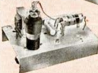
A.M. SIGNAL-GENERATOR (above) Build it yourself! Provide amplitude-modulated signals for test and experimental purposes. Gives valuable practice!
