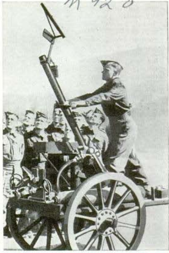
These rocket projectors send aloft parachutes from which wires dangle to ensnare enemy planes
