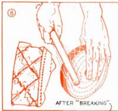
9 COATED SURFACE DRESSED WITH PIECE OF GRINDING WHEEL
