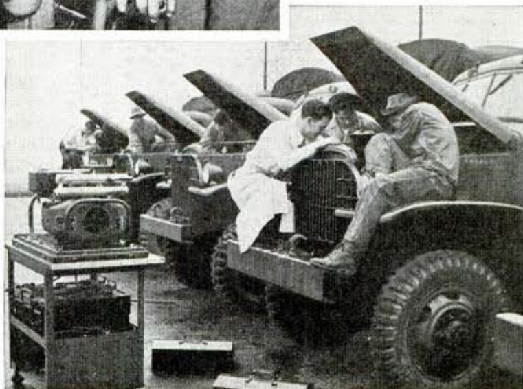
With truck bonnets up, the service class goes to work on engine repairs. Notice, at left, the gasoline-operated generator for charging batteries in field
