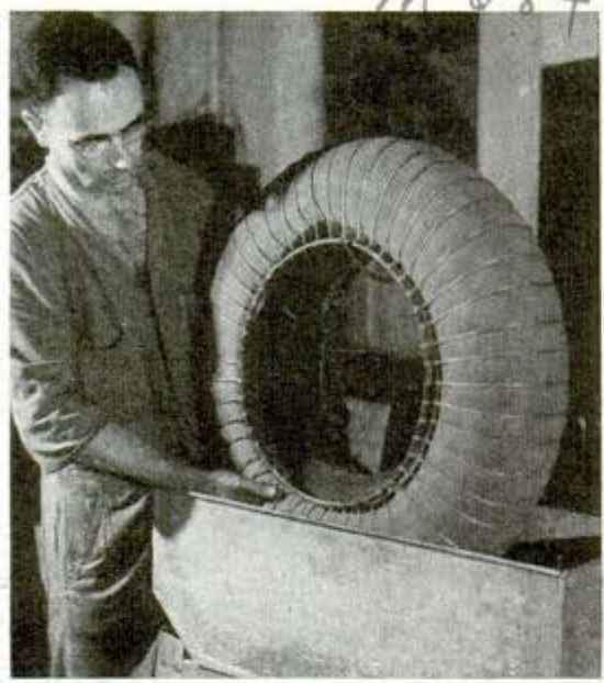
"Caged" inner tube safely withstands high pressure
