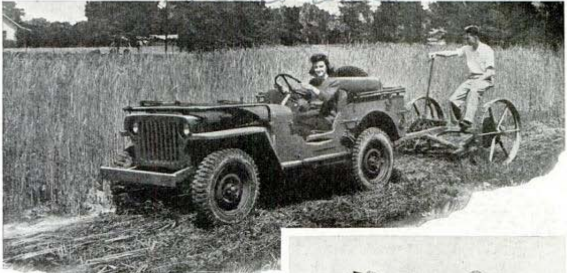
↑ Trying out the jeep's talents on a mowing job. Government experts say the jeep could be highly useful as supplemental power for light plowing, road use, and general field work, but it is too low and narrow for most row-crop cultivation jobs
