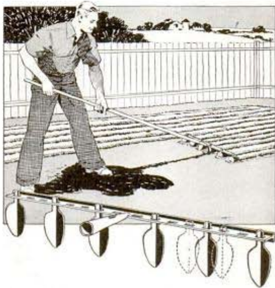
Digging six furrows at one time with hand plow that is pulled like a rake. V-shaped teeth fit in slots
