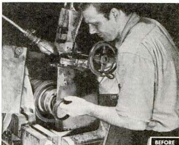
By installing a loading arbor, several pieces can now be loaded on centerless grinder, vastly increasing production
