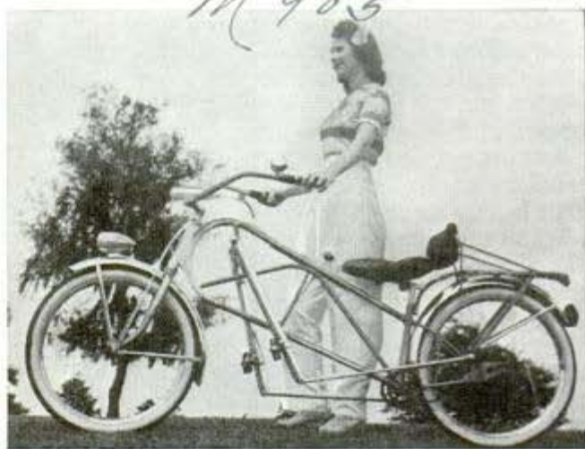
Dual chains driven by two levers apply continuous overlapping power, giving almost equal force the full length of each stroke
