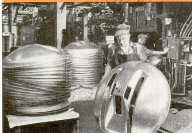
Aluminum machine-gun turrets for bombing planes are now formed by a powerful press formerly used to stamp out halves of aluminum beer barrels
