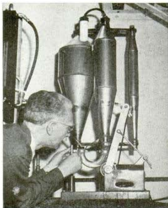
Determining amounts of particles of different sizes contained in chimney gases with a special apparatus
