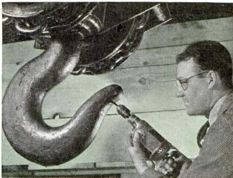
Instead of sawing off a piece for microscopic analysis, a tubular drill bores out a sample from tip of 50-ton crane
