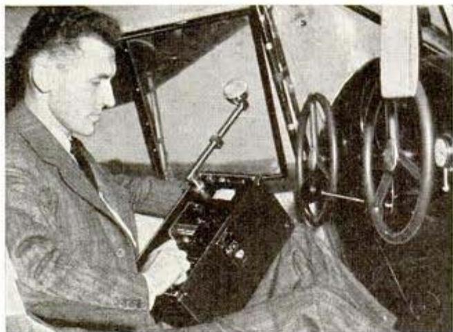
Portable sound-level meter built by General Electric engineers tests the noise of airplane propeller and engine in cockpit
