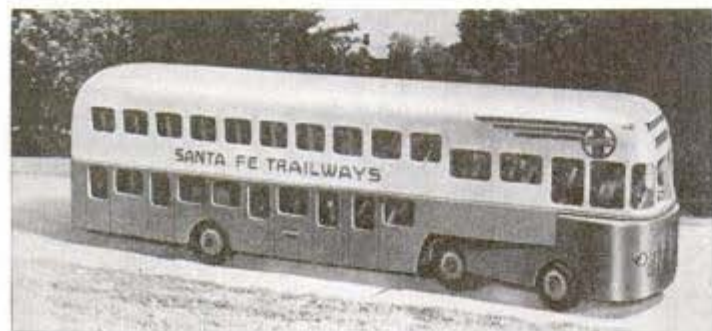
Pivoted tractor under front of big bus makes sharp turns possible
