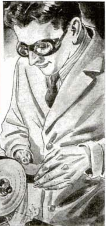
9 COATED SURFACE DRESSED WITH PIECE OF GRINDING WHEEL
