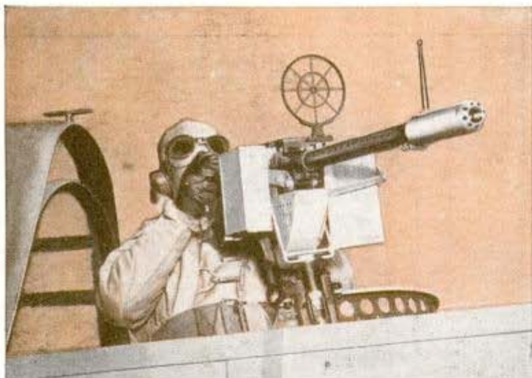
The bright tube on nose of this navy fighter plane's machine gun conceals powder flashes U. S. Navy photo
