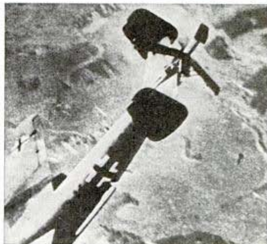
As bomber noses into dive, top, "umbrella" brake starts opening. At end of the dive it is open fully
