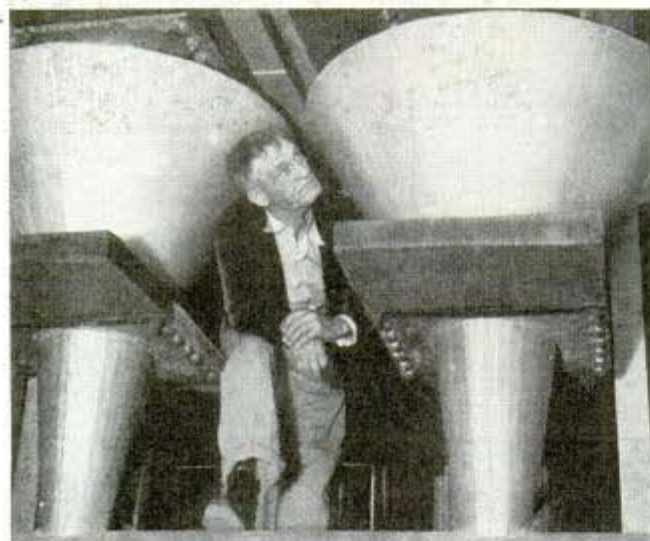
Left, "batching" bins at gold smelter for measuring amounts of ores and chemicals
