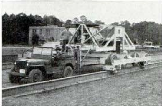
↑ Trying out the jeep's talents on a mowing job. Government experts say the jeep could be highly useful as supplemental power for light plowing, road use, and general field work, but it is too low and narrow for most row-crop cultivation jobs
