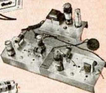
SUPERHETERODYNE CIRCUIT (above) Pres-selector, oscillator-mixer-first detector, i.f. stage, diode-detector-a.v.c. stage, audio stage. Bring in local and distant stations on this circuit you build yourself!
