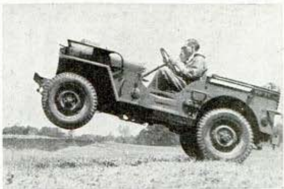
This bucking bronco of the army is tough enough for the rough work encountered on the farm (above). It could "ride herd" like a cow pony, pull like a draft horse. The tests included power pulls against a dynamometer (left), during which the jeep developed a 1,300-pound pull with almost no wheel slippage. The four-wheel drive with six forward and two reverse speeds offers plenty of pull for field operations, and the front wheel drive can be disconnected for road work. The jeep's engine develops 60 horsepower
