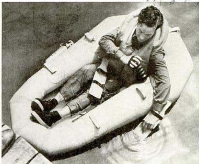
Boat pack, left, tilts scale at 12 pounds. Right, inflated, it cradles pilot and a few needed items
