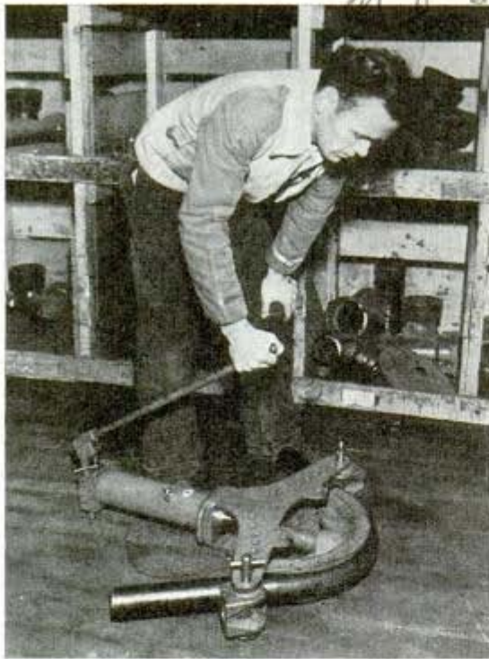
Portable pipe bender eliminates elbows and fittings
