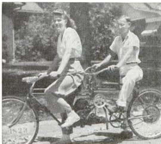
Work of pedaling this homemade tandem is taken over by washing-machine engine using little gasoline
