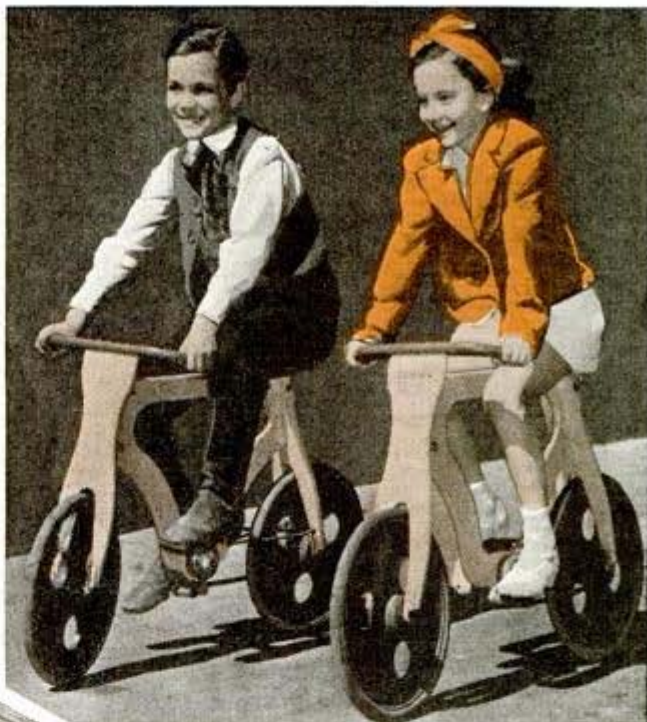
Off to school on bikes made of wood except for metal fittings and tires. Below, fan blade for cooling tower made of plastic-impregnated wood
