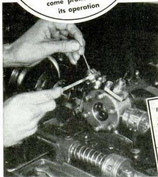
The turret replaces the tailstock of an ordinary lathe. It holds a number of tools used successively in machining operations, each tool being brought into position quickly yet accurately
