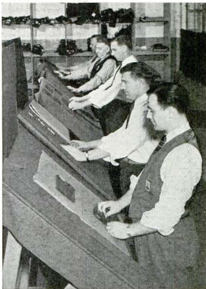
Examining samples of fabric to assure uniformity of shade is one of many analytical tests performed by a staff of experts
