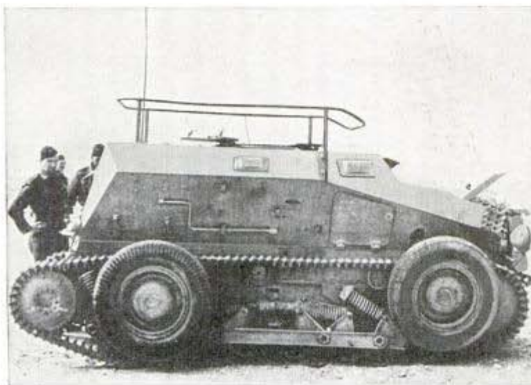
Captured while on scout duty in Egypt, this German car rides either on four wheels or a pair of "tracks" as required by the changeable terrain.
