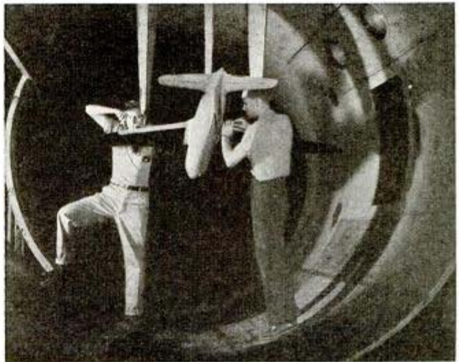
Douglas transport model is mounted upside down for special tests at California Tech
