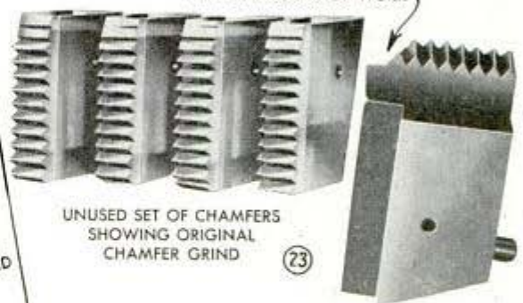
CHASER DAMAGED BY RUNNING INTO SHOULDER OF WORK
