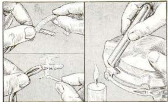
Tape solder, left, and bar solder, right, need no more heat than the flame of a candle or match
