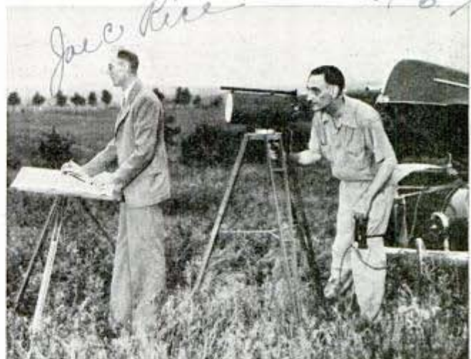
Charting angles at which light signals will be used (left) while (right) keyboard fastened at the knee taps out the messages
