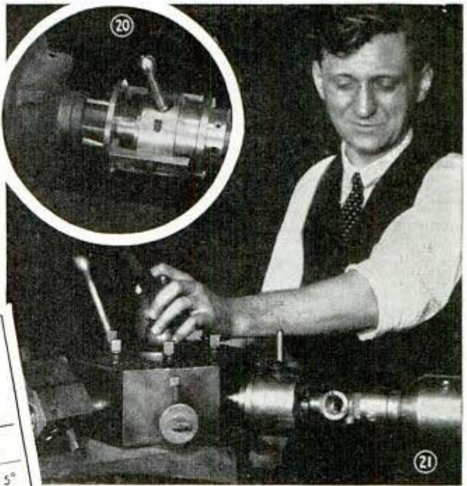
CHASER DAMAGED BY RUNNING INTO SHOULDER OF WORK
