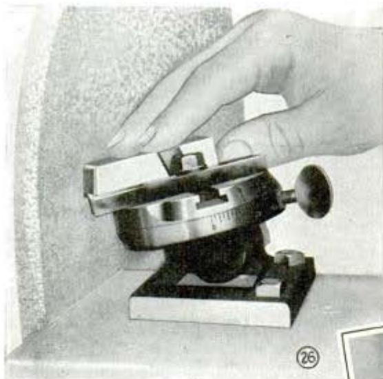
CHASER CHAMFER SHARPENED ON SIDE
