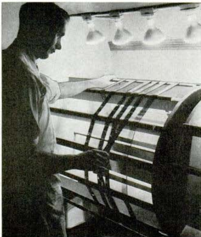
The dark bands encircling reel are newly developed microfilms being dried under heat lamps, a final step in the processing
