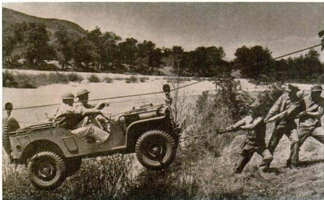
One way to get a jeep across a river—ferrying it on a cable with pulleys, ropes and chains. This mechanical pet of the armed forces is being pulled by prospective officer candidates
