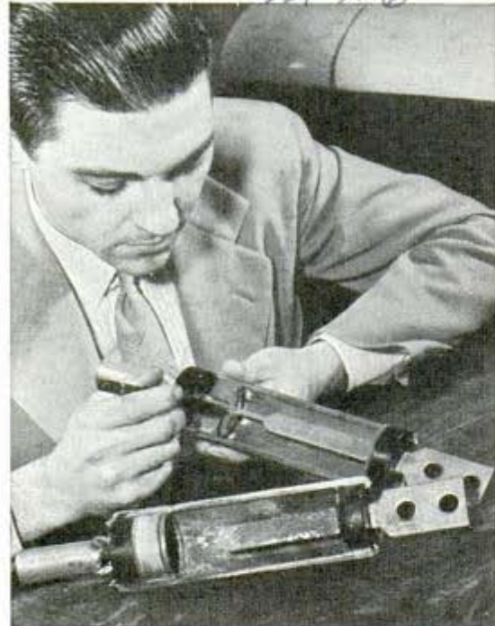
Cutaways of blown (foreground) and unblown limiter
