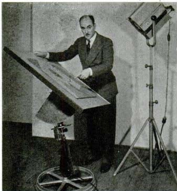
James C. Boudreau, head of Pratt Institute Art School, operates machine which duplicates sun-shadow conditions at any given moment of year
