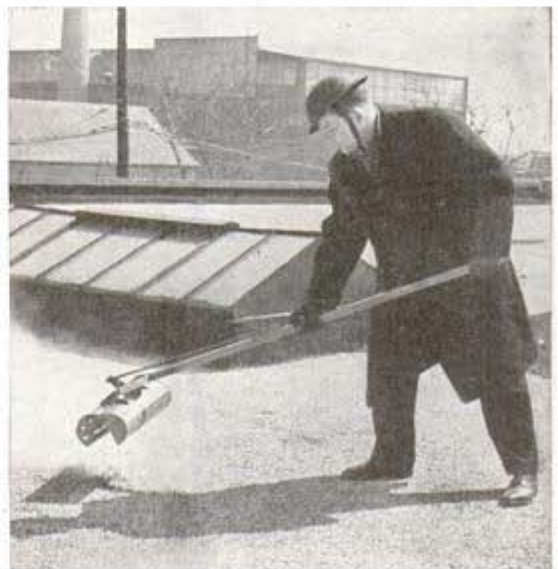
Split cylinder picks up bomb and holds it safely
