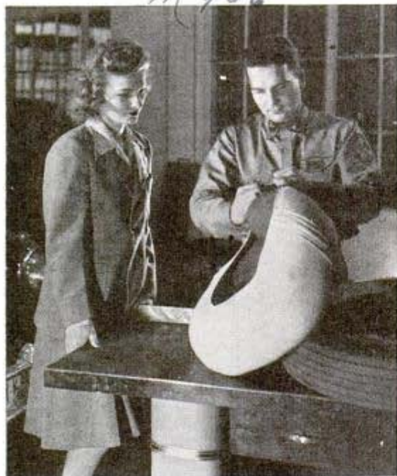
Jacket slips over inner tube before going into casing
