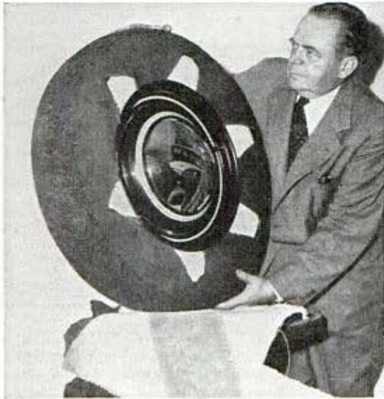
Sandal wraps around tire and points tuck in at rim
