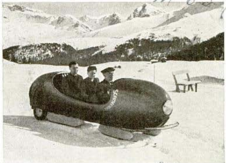
To run on bare ground this sled lowers its front wheels; rear wheels carry the driving force
