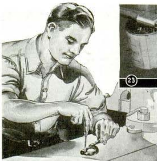
SQUARING WORN CONTACT OF MICROMETER SPINDLE
