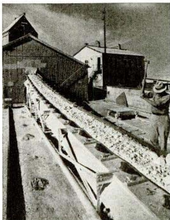
Hot molten sulphur flowing from mine into six-acre vat to form solid "cliffs" like those in background
