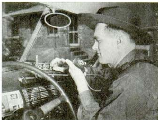
Telegraph key on patrol-car instrument board is used for radio communication when car is too far from station for voice radio
