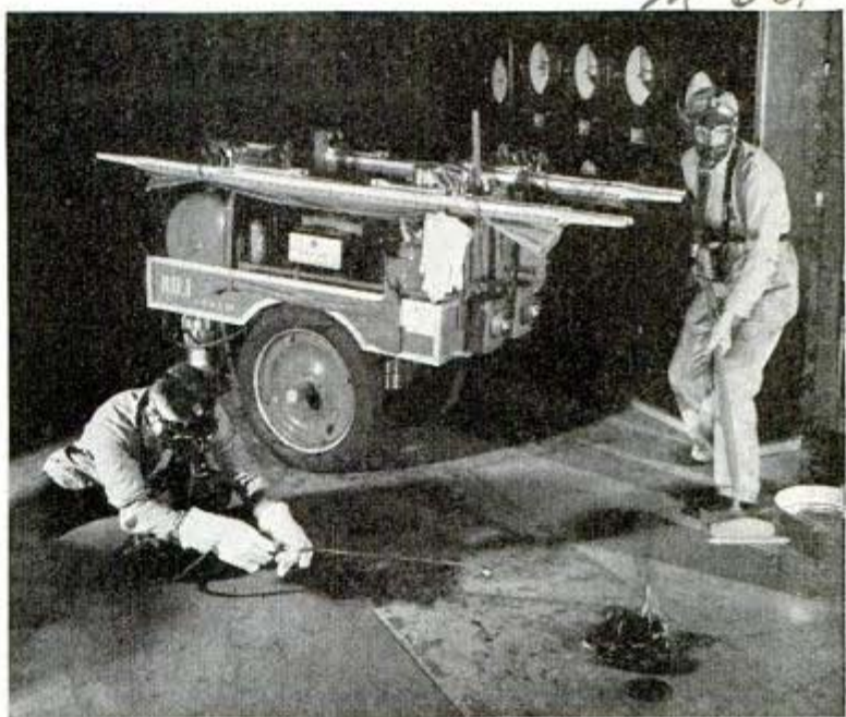
Two wheeled cart completely equipped to fight fires and aid the injured
