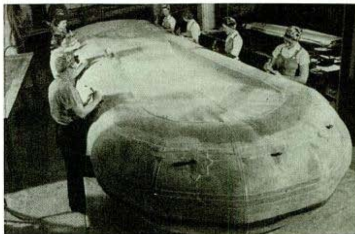
Check and double check—this huge rubber pontoon float made for the U. S. Army must be flawless for its future role under hail of shells Workmen removing a "cake" of Chemigum, synthetic developed by the Goodyear Co., from a press. Cakes are converted into war materials
