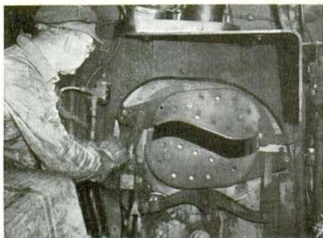
Engineer opening the inspection door of fire box in cab of steam locomotive boasting 132,000 pounds of tractive effort
