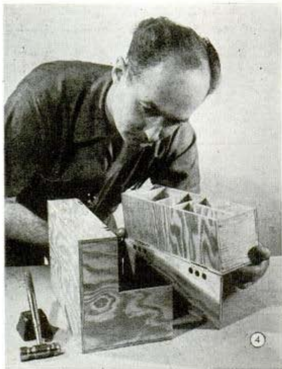
As the dimensions of your kit may vary, depending on the equipment available, it is advisable to get these first. The adjustable clip enables the worker to direct the flashlight in any direction and it can be left in the clip when the case is closed
