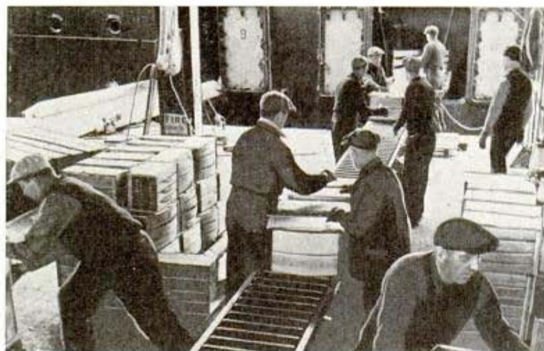
Crates of fruit from tropical America roll down the conveyor at New York, speeding a ship's turn-around
