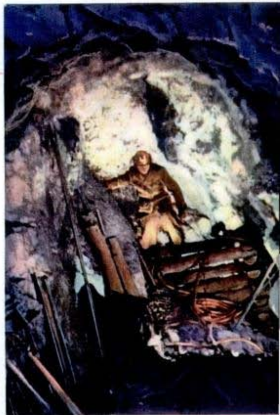
† Mining radium-bearing ore 500 feet under the earth, a stope in the Eldorado Mine on the edge of the Canadian Arctic. The ore vein which contains the radium is pitchblende—a dull heavy, black and brittle rock
