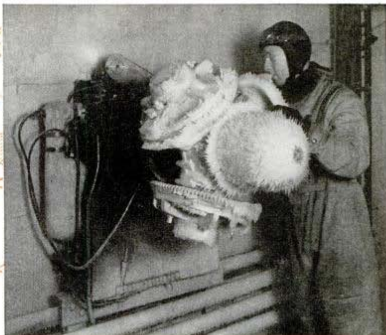
That's frost on the propeller mechanism being tested for 50 degrees below zero
