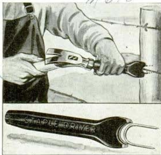
Grooved end prevents driver slipping from staple
