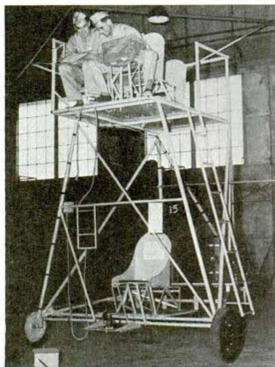
This animated "high chair" is used for practicing aim with bombsight on mobile ship silhouettes on floor
