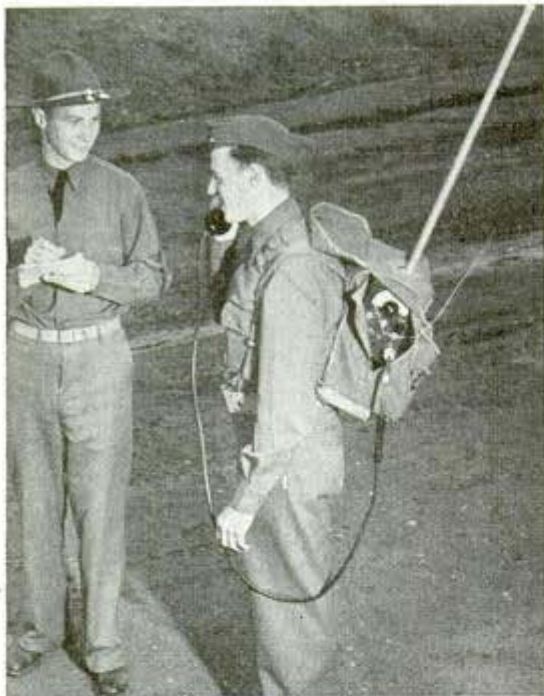
Army's famed "walkie-talkie"—portable two-way radio set—weighs less than regular infantry pack
