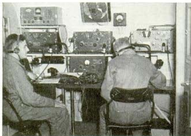
Above, interior view of the "broadcasting station on wheels" (below) used by the Signal Corps. Trailer carries radio receiver, also motors to supply power for a transmitter in the tractor
