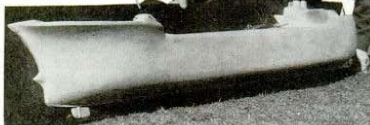
Model of wooden ship designed to ride low and carry warplanes
