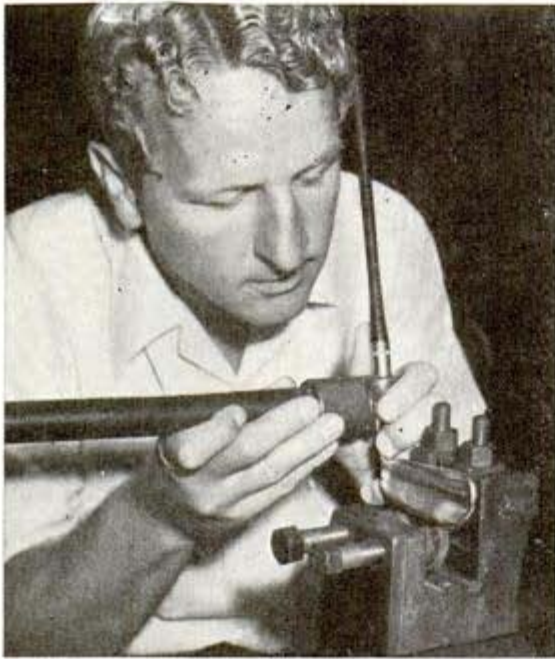
Measuring angle between blade and shaft of a putter
