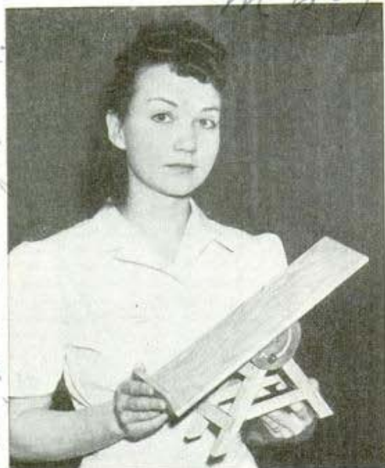
Balanced at the center, the table locks at any angle
