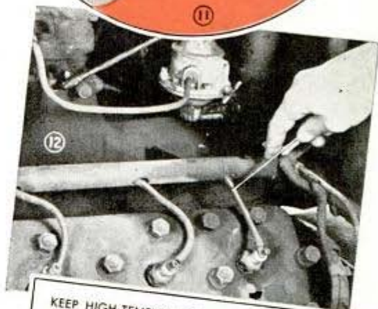
KEEP HIGH-TENSION CABLES CLEAN AND CHECK CONDITION OF TERMINALS IN DISTRIBUTOR CAP
