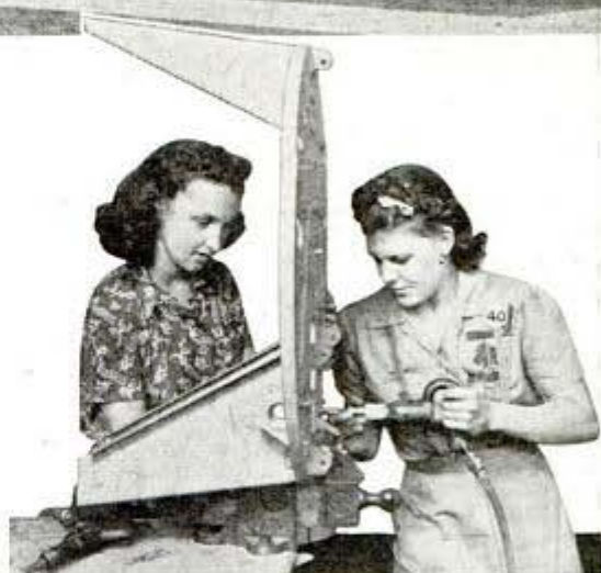
Girl at left bucks rivets driven by gun at right in assembling fuselage bulkhead for a Vultee plane
