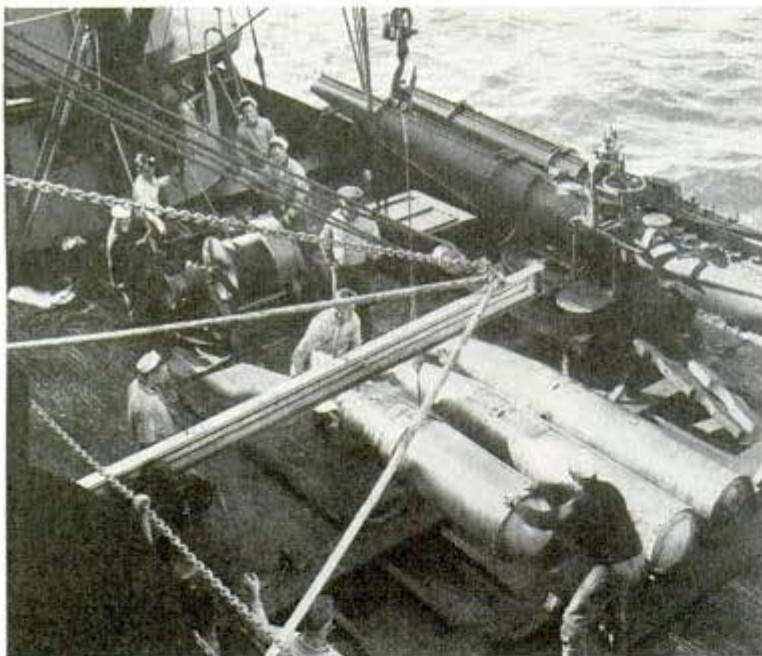
Loading torpedoes with "dummy" heads filled with water on a testing barge where they will be fired to check propellers, rudders and gyroscopes
