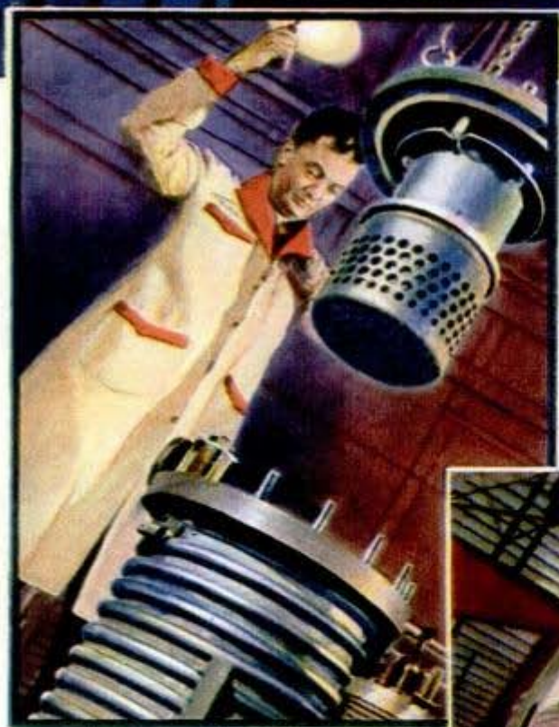
→ Another big machine for changing alternating current into one-directional flow is this rotary converter, used by a chemical company in producing an important element in the gasoline that powers American war planes, tanks and jeeps. The process is electrolytic, and this converter is capable of supplying 5,400 kilowatts of electric power—enough to drive an electric railway train
