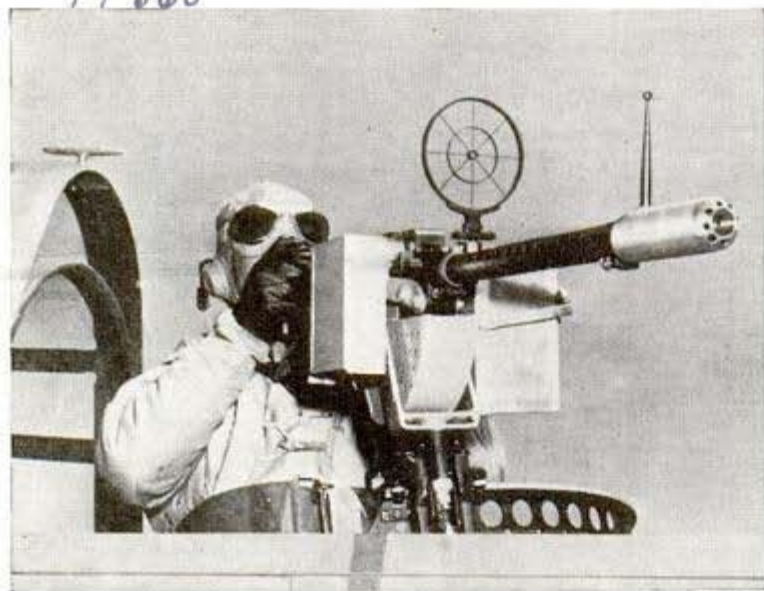
Tubular extension at nose of machine gun hides the flashes that might otherwise aid hostile gunners in spotting the airplane's exact position
