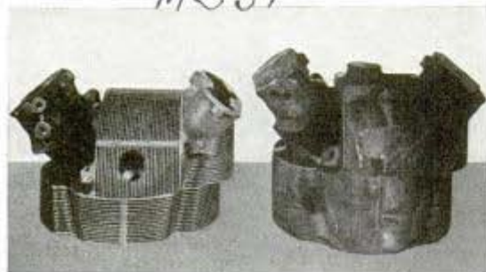
Cooling fins, left, are cut into forged head at right
