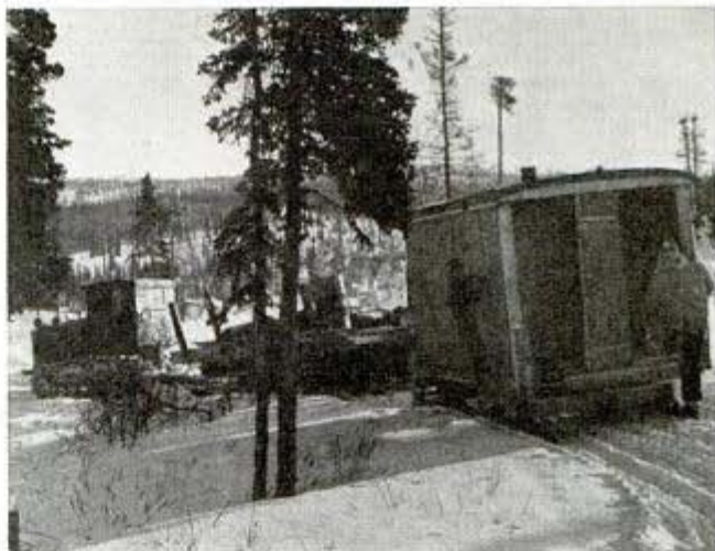
Crawling Diesels haul the "snow trains" laden with supplies. Usually there is a "caboose" serving as cookshed and dormitory
