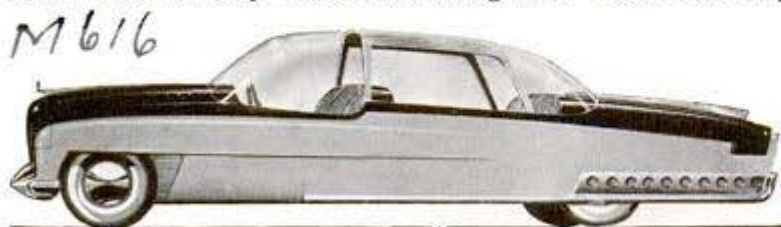
Designer's conception of automobile built from plastics and lightweight metals now being developed for use in construction of airplanes and tanks
