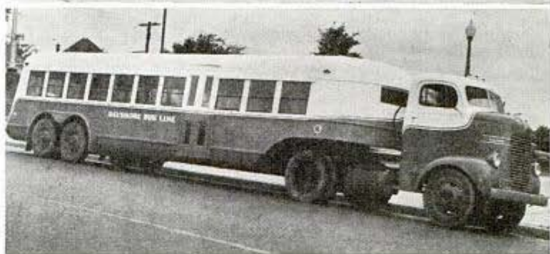
Bus, bottom, was converted from an auto transport trailer like the one above, opening a useful life for trailer that had lost its regular job
