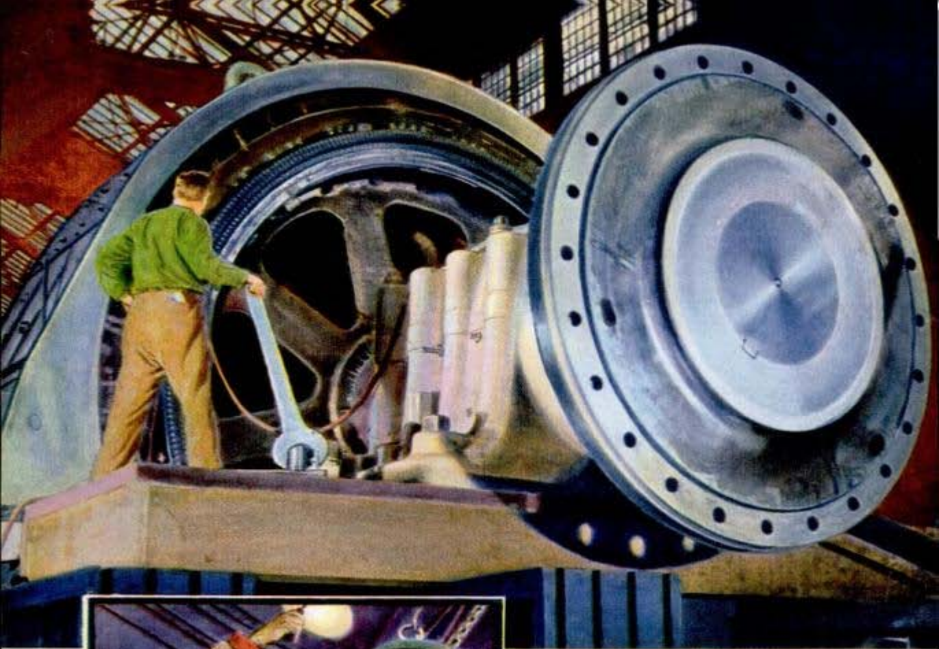
↑ Biggest of their kind are the two 5,000-horse-power electric motors built to power a plant producing aluminum for fighting planes. One of these powerful twins is shown here on test at a Westinghouse factory where it was completed months ahead of schedule as rush job for war program
