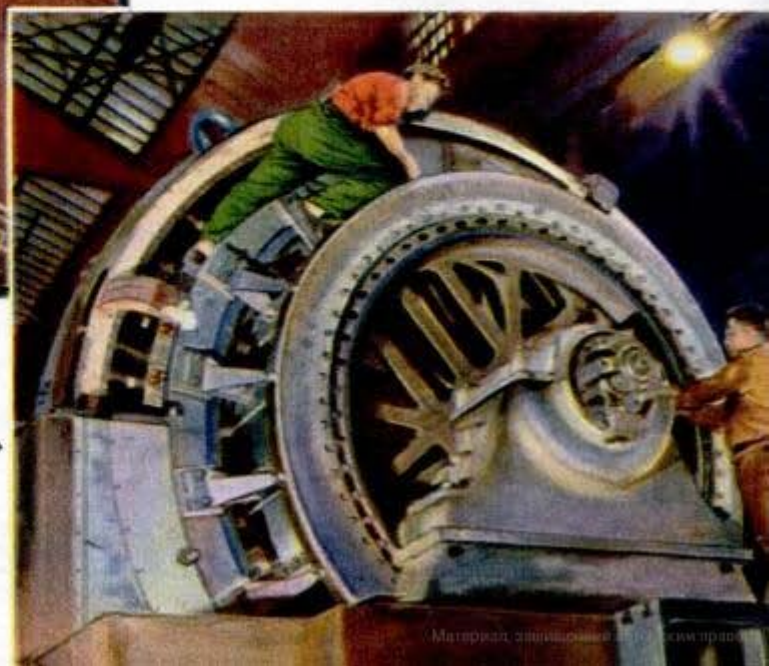
→ Another big machine for changing alternating current into one-directional flow is this rotary converter, used by a chemical company in producing an important element in the gasoline that powers American war planes, tanks and jeeps. The process is electrolytic, and this converter is capable of supplying 5,400 kilowatts of electric power—enough to drive an electric railway train
