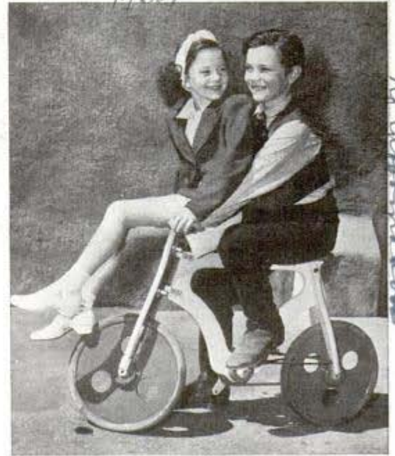
Bicycle frame made of wood saves metal for war uses
