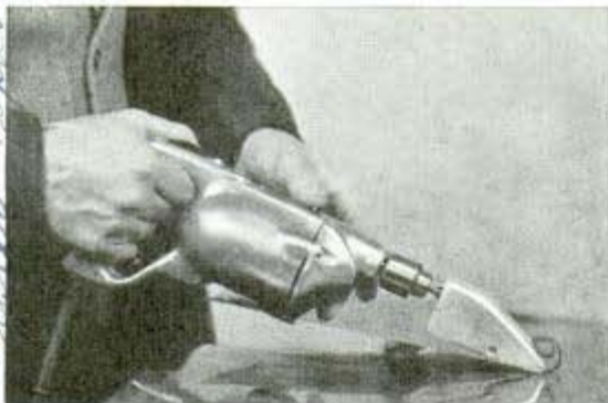
Drill attachment nibbles strip of metal as it cuts
