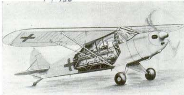
Two patients can be carried on stretchers in fuselage of light plane
