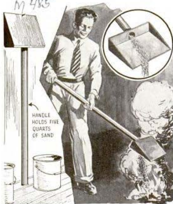
Shovel weighs only 19 pounds when loaded with sand
