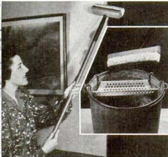
Drainer on bucket, inset, squeezes water from sponge
