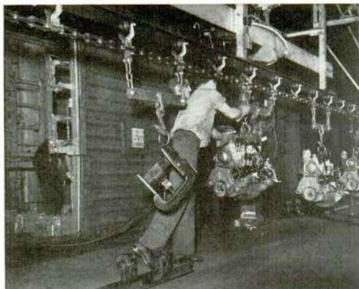
Chain conveyor in specially fitted boxcar facilitates loading of engines with minimum packing
