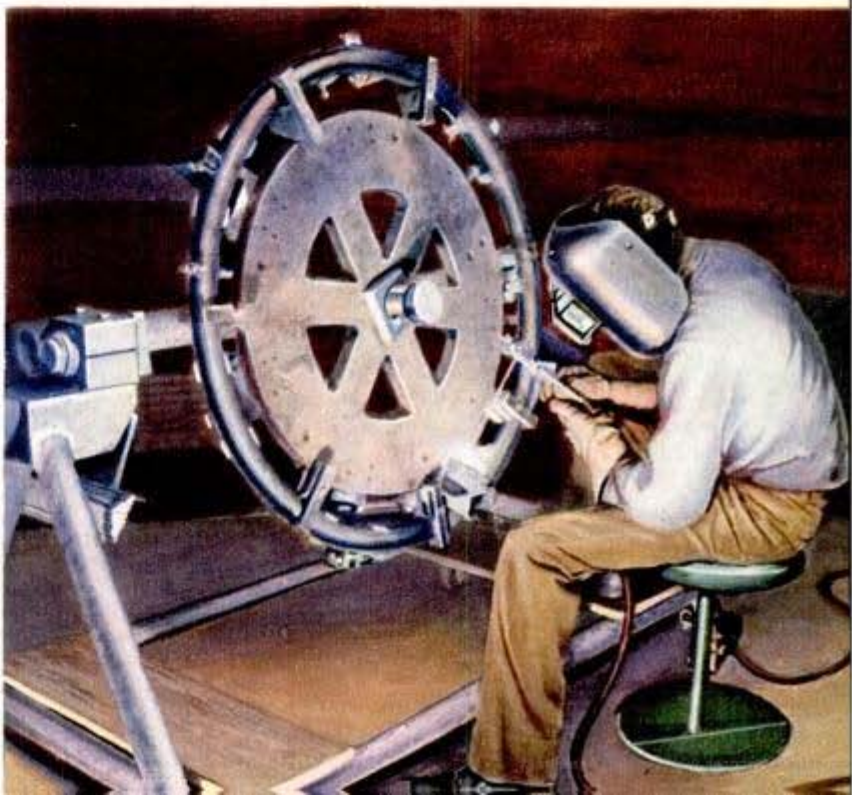
This tubular mount will hold a heavy airplane engine secure
