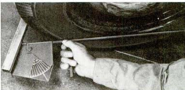
Dial, above, indicates both camber and caster. Right, top, toe-in trammel bar and gauge; bottom, angle gauge shows up bent radius rod. All parts are easy to handle
