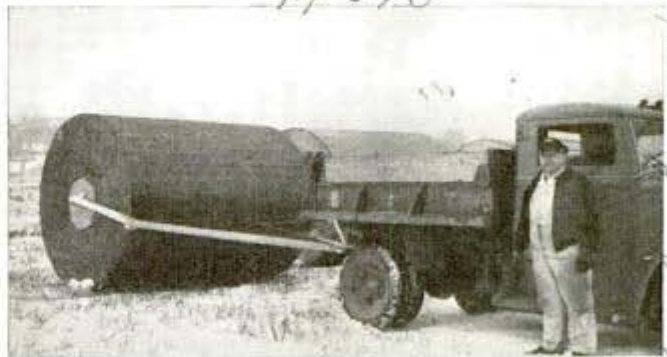
Snow roller, instead of plowing snow from the airport runways, packs it down so plane may use them soon after heavy snowfall
