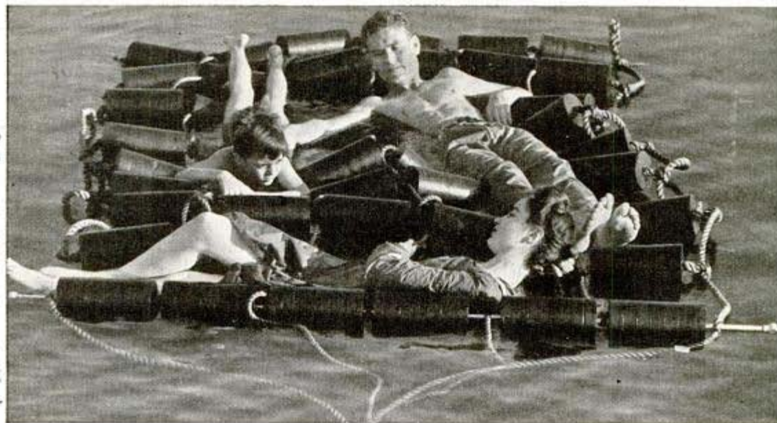
Discs made of a new rubber filled with nitrogen gas are roped together to form a raft lighter than cork
