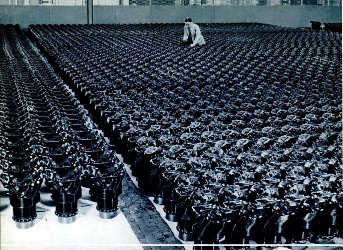
Cylinder heads are fitted with barrels of alloy steel
