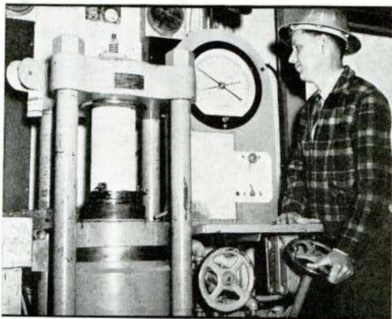
Measuring the crushing strength of a core of concrete taken from a dam
