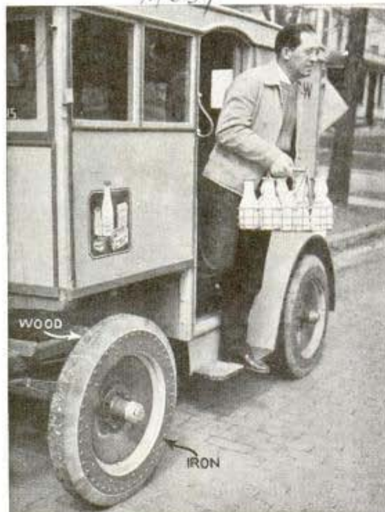
Milk truck equipped with wooden tires on iron rims
