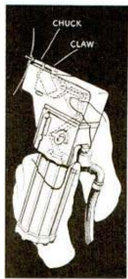
Tubular rivet slips over nail. Diagram shows double action of squeezer
