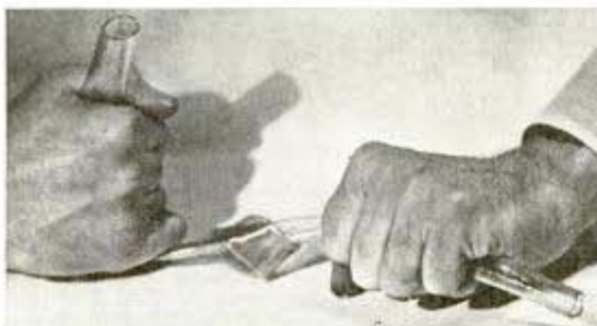
Tubing covers wires without hiding them from view
