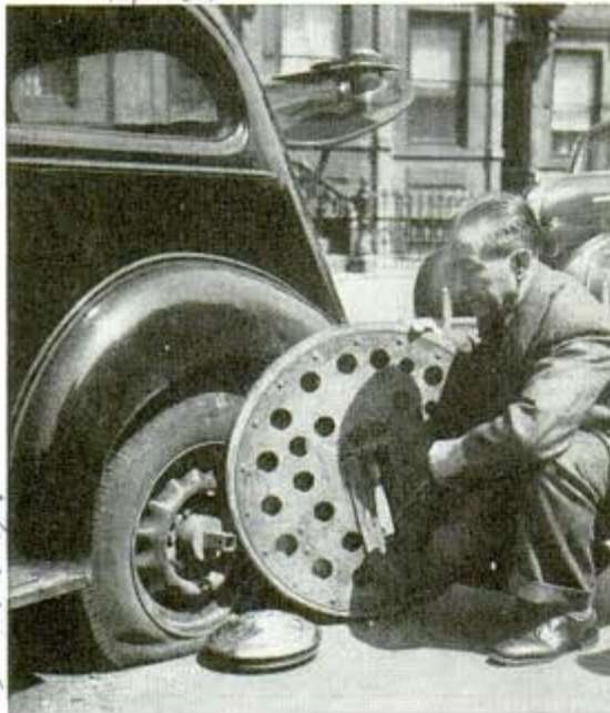
Emergency wheel fits on square extension of the hub
