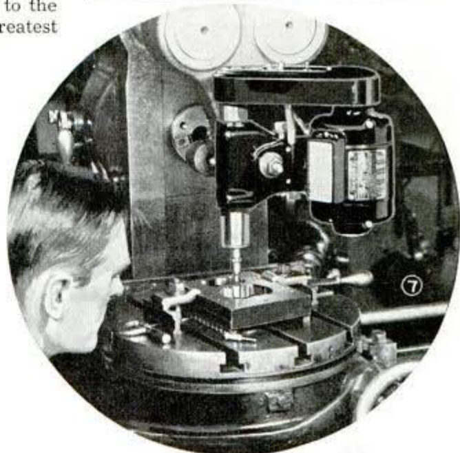
Upper photo shows how thread grinding is done in a screw-cutting lathe by means of an attachment on a tool-post grinder, which corrects threading-tool errors and heat-treating distortion. Lower photo shows how a tool-post grinder is set up for use on a milling machine
