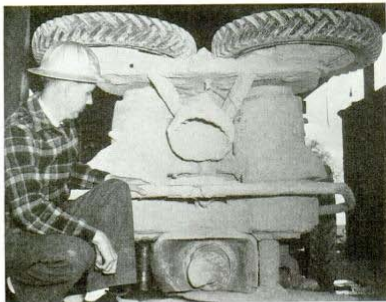
Odd-shaped auger (above) is at the end of an air suction line which is used for the transportation of bulk cement from box cars to silos
