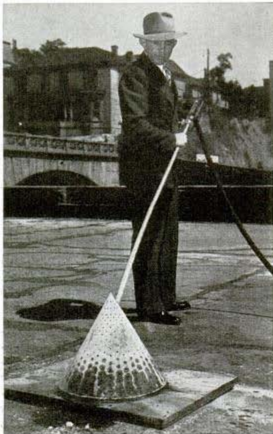
Spray causes bomb to burn itself out under sieve
