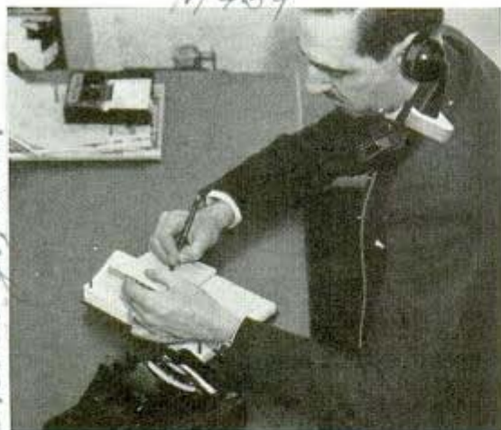
Telephone holder supports instrument on shoulder
