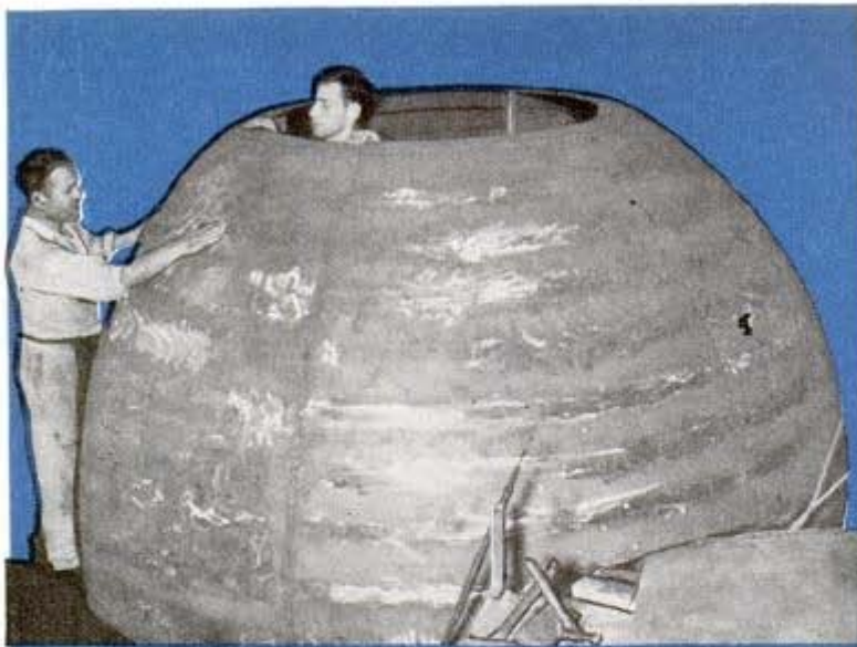
Resembling a new type of air raid shelter, the lower part of the largest bottle ever made for a sign awaits the neck. It will be 35 feet high
