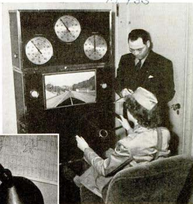
The driver faces a moving picture of road
