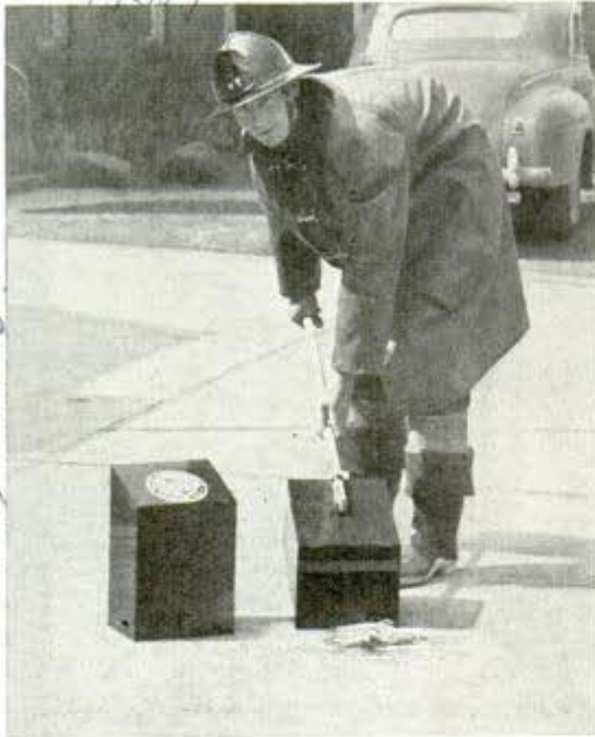
Views show bucket closed and opened to form scoop
