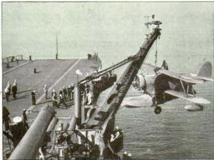
Hauling the observation plane aboard the Lexington; in the foreground is one of the carrier's guns. These planes scout ahead and alongside a "task force" on watch for enemy vessels
