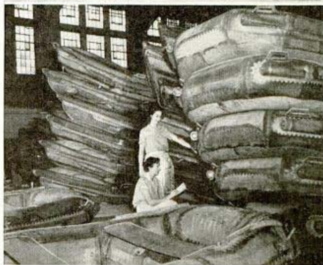
Two views of rubber assault boats being completed for United States forces. Deflated, the boats can be rolled into bundles
