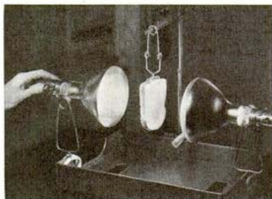
Heat lamps toasted bread in less than ten minutes 1,000 and 65-watt lamps with gold-plated reflectors
