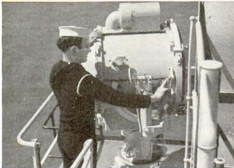
The blinker is the recognition light at night and is used for transmitting messages whenever it can be employed without detection by the enemy
