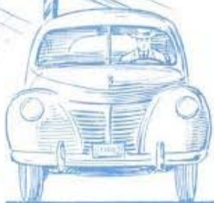
PIGEON-TOED WHEELS GRIND OFF RUBBER
