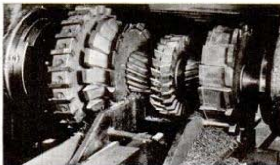
TWELVE SURFACES MILLED AT ONE TIME
