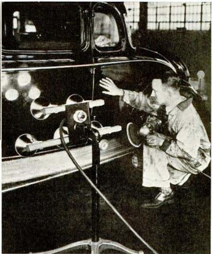
A battery of infrared lamps bakes enamel on an auto in repair shop
