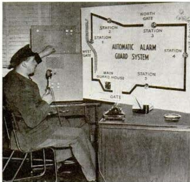
Master control board for acoustic fence, left. Dog crawling under fence, right, would sound alarm
