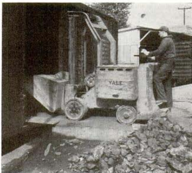
Scoop truck runs in and out of freight car to load or unload
