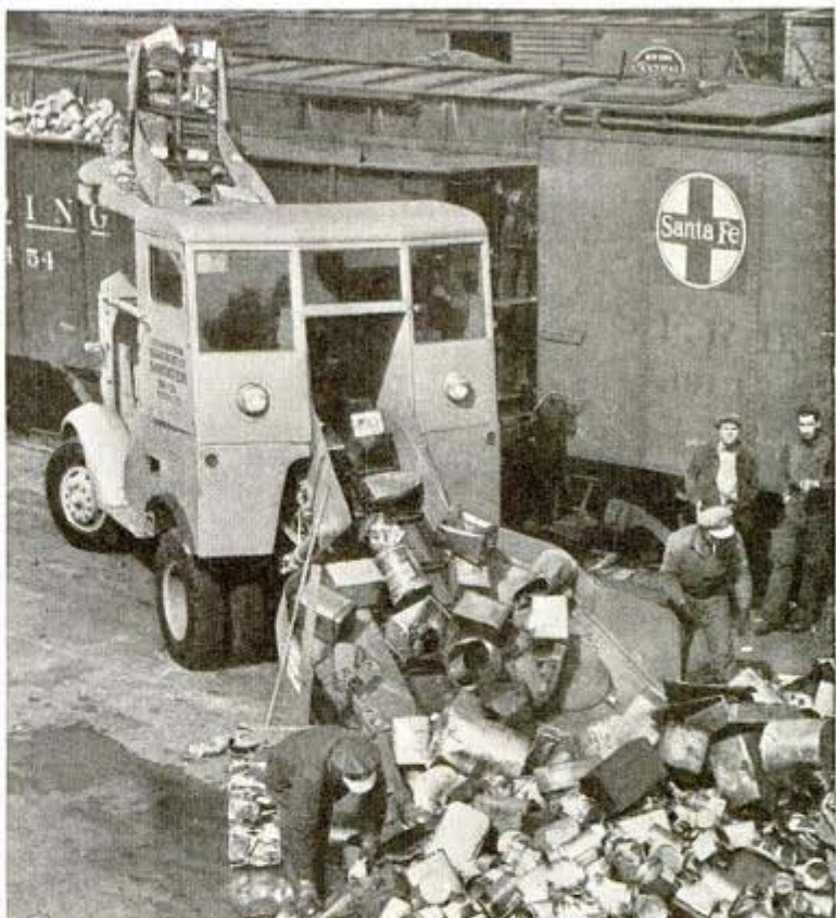
Snow loader fills freight car quickly. Tin cans pushed onto the scoop are hoisted in a steady stream over side of the car by means of conveyor
