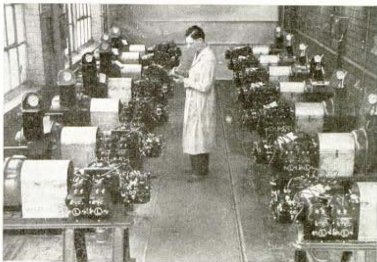
Lycoming engines, standard on several lightplanes, are given their first "run-in" electrically
