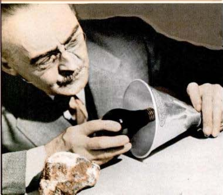
This is a $2 ultraviolet lamp made in special black glass which can be placed in any suitable reflector and used by the amateur experimenter
