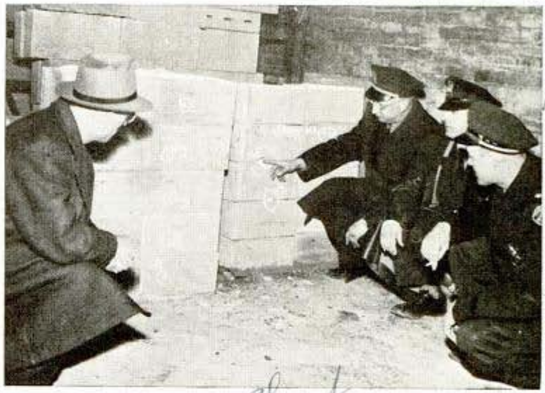
Policemen, top, lined up to fire into concrete blocks made by mixing slag with cement. Bottom, examining the bullet-resisting blocks after the test
