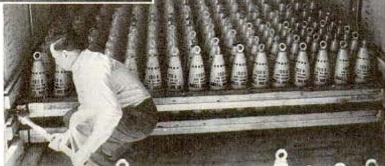
Tightening a load of 155-milimeter shells in a utility loader box car at U. S. arsenal →
