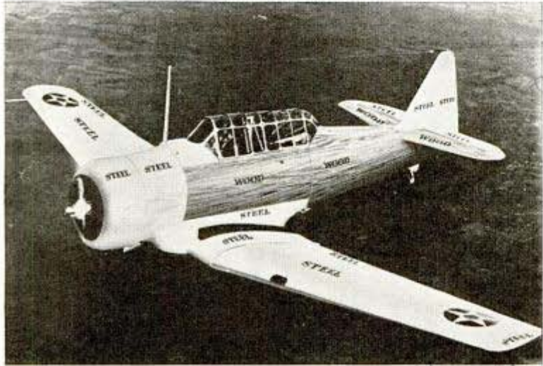
Surface of training plane is marked to indicate parts that will be covered with wood and steel instead of aluminum, to save the metal for fighters
