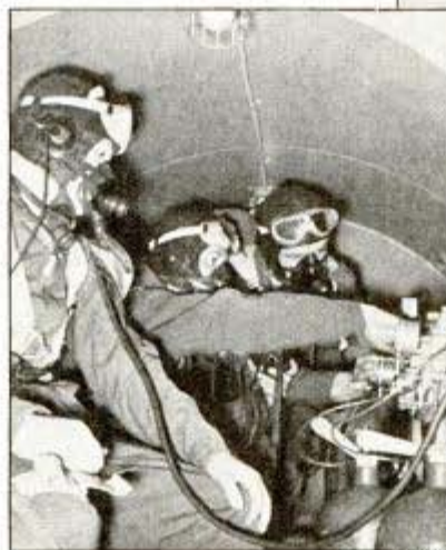
Test crew checking oxygen equipment in strato-chamber. Right, sketch of present-day fighting levels and those of tomorrow
