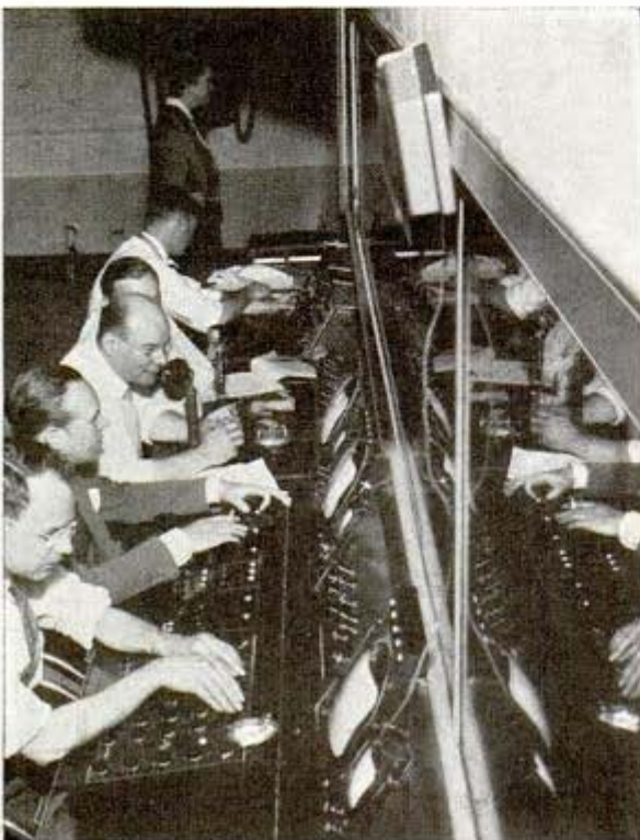
From this panel, CBS program director and staff guide action on studio floor and control the transmitted image
