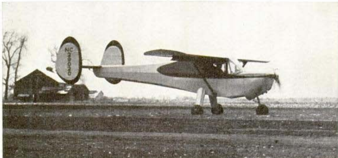
The rudderless "Skyfarer," top, rides level on the ground with its tricycle wheel arrangement
