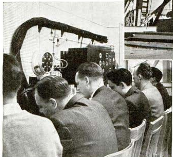
Rotating stand for testing engine, above, rolls on a circular track. Left, the "flight crew" is watching result of a test
