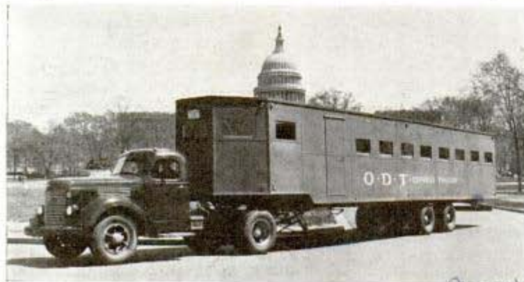
This 45-foot trailer for war workers is built of noncritical materials
