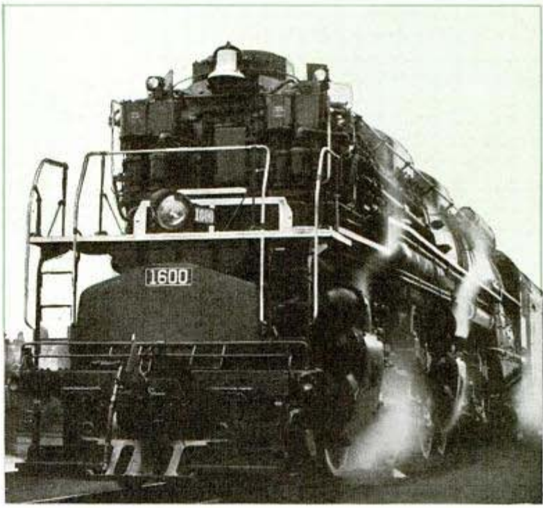
"Allegheny" type engine of the Chesapeake & Ohio, with unique 2-6-6-6 wheel arrangement, hauls heavy coal trains over eastern mountains. Below, armored division puts aboard a trainload of track-laying trucks
