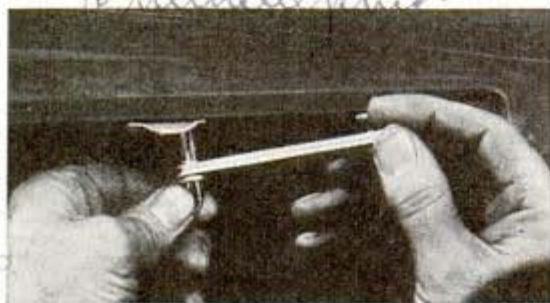
Offset ratchet screwdriver reaches into close places
