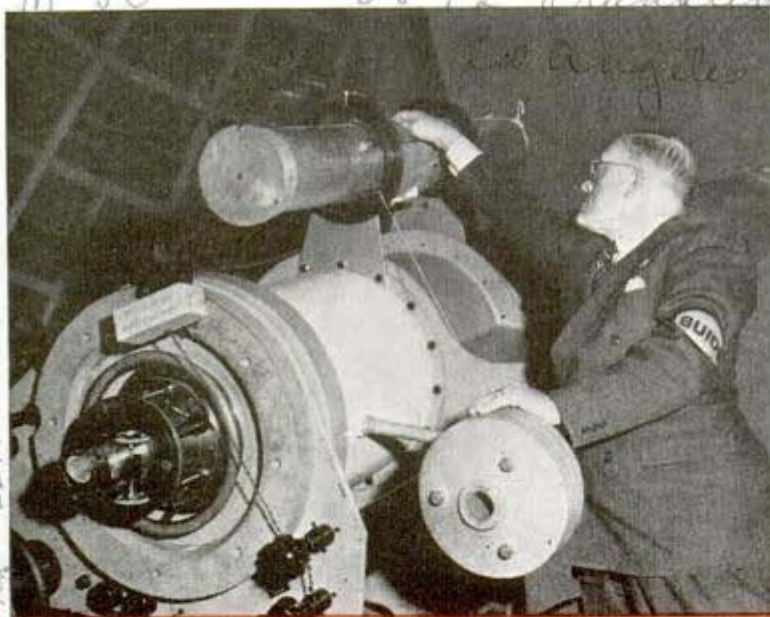
Inspecting the barrel of a small Schmidt telescope camera mounted on larger telescope at Griffith Observatory, Los Angeles
