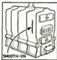
Boiler and Furnace Leaks
