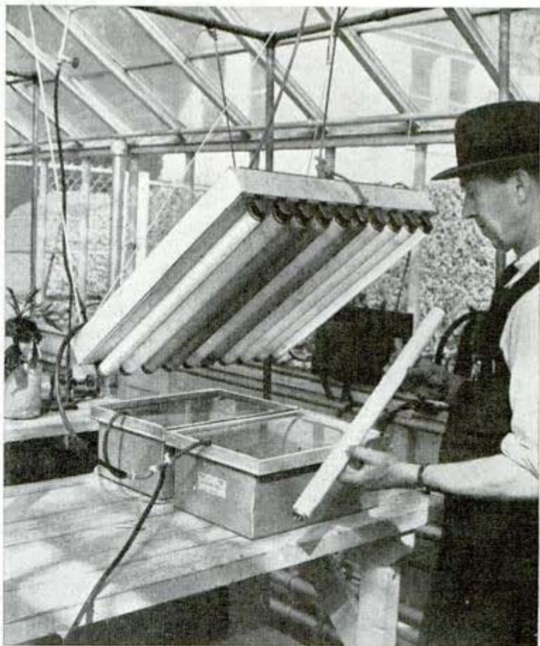
Apparatus which makes possible the determination of effect of various light spectra on plants; note the fluorescent light tubes
