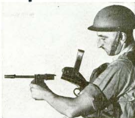
Pressure on button releases machine-gun barrel
