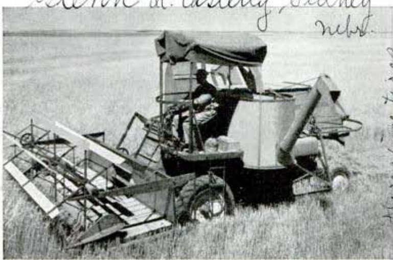
Combine driven by its own engine can be operated by one man as all controls are placed within easy reach of anyone in the driver's seat
