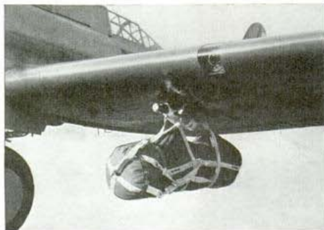
Rolled in felt pads, some kinds of supplies, including guns and ammunition can be parachuted safely to the ground
