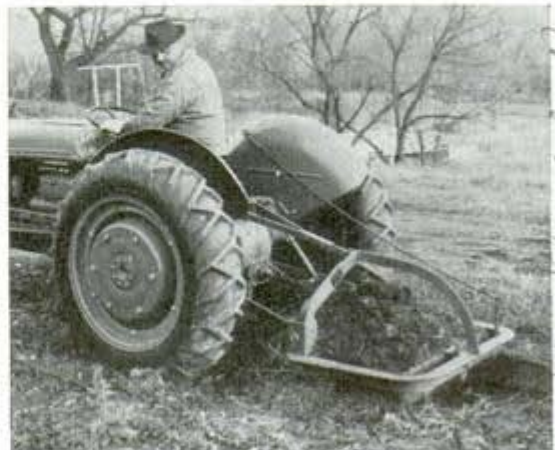
Scoop can raise load above ground and cart it away
