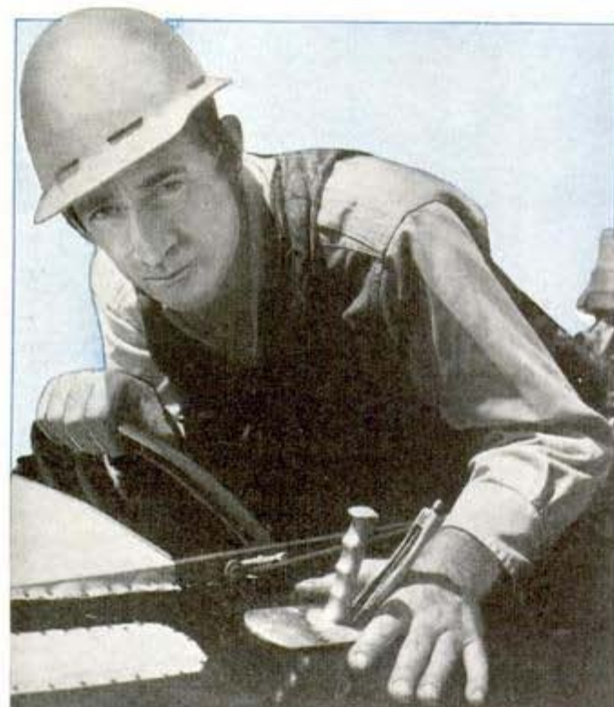
Left hand of driver is at the automatic throttle he must grip throughout race to keep motor going
