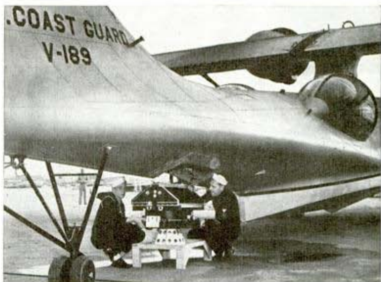
Nine-lens camera for flying boat will cover 300 square miles at 20,000 feet
