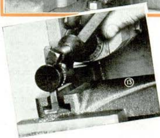
To cut a T-slot, the center section is grooved first; then the wider bottom portion is cut with a specially formed T-shaped bit
