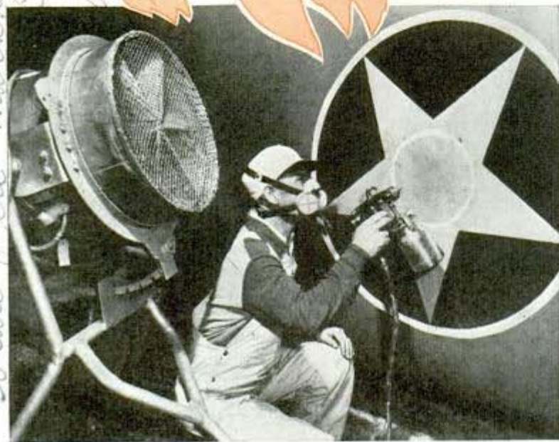
Painter at Douglas plant working on wing insignia. Big fan behind him carries spray vapors to exhaust system of paint room
