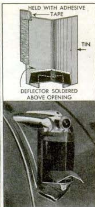
(5) Taillights can be blacked out from above yet continue to serve their usual purpose, or the taillights can be turned off entirely if a blackout lamp that throws light on the ground, is provided
