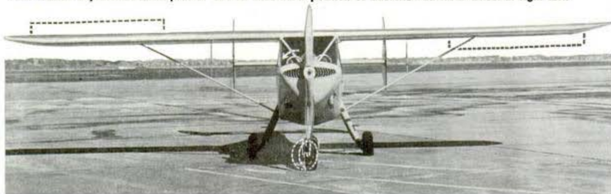
Here is the "Skyfarer's" clean profile. Dotted lines show position of ailerons and front wheel in right turn
