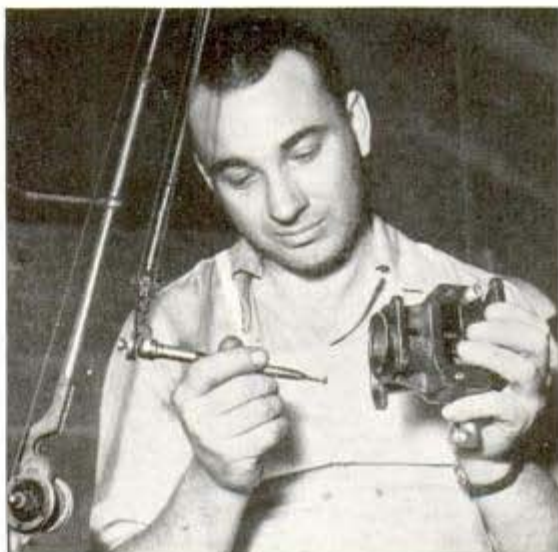
Below, buffing surfaces of cylinder head with a tool mounted on a dentist's drill
