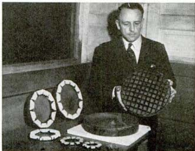
Some of the special grinding tools used in shaping a 12-inch Schmidt reflecting mirror; mirror glass rests on white slab
