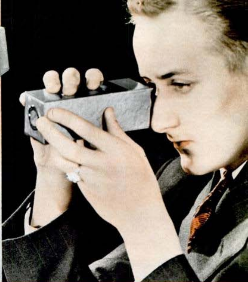
23 Right, using the Vuescope, an instrument for viewing Kodachromes. Drawings at left show that this is accomplished by employing a small light bulb drawing current from dry batteries
