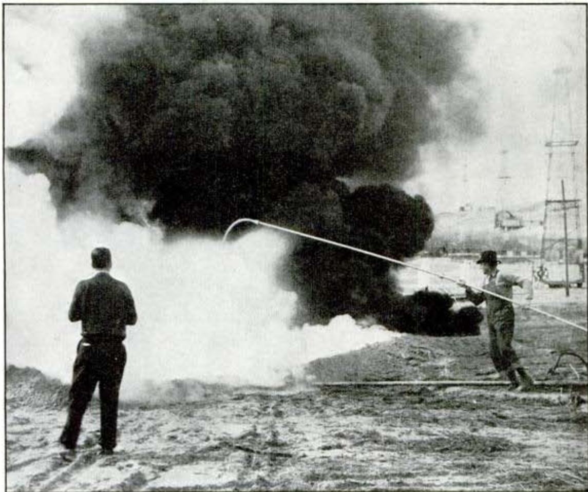
Extinguishing gasoline fire with fine water spray that cools gasoline below ignition temperature
