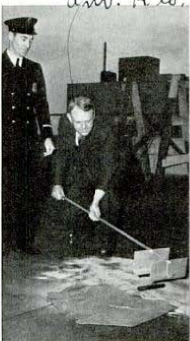
Demonstrating with fuses, left, how jaws of pickup device, operated from distance, can grab incendiary bomb and, right, drop it into pail of sand
