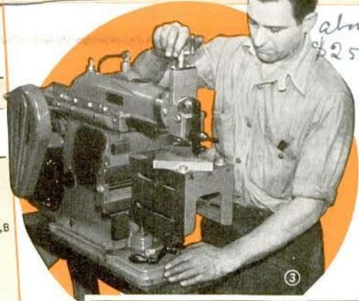
In shaping the male part of a dovetail, a long, sharply pointed tool bit is needed for clearing the metal in the angular cut
