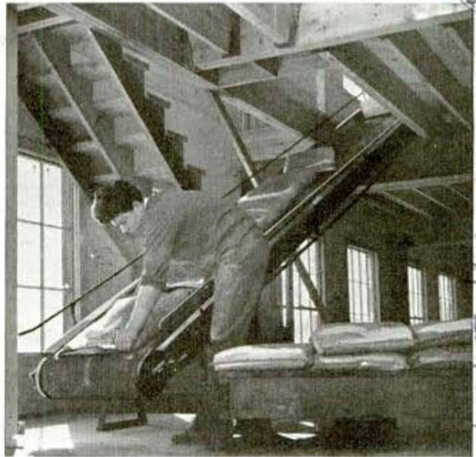
This belt conveyor is ready for immediate use, needing only a convenient floor opening and connection to an electric outlet
