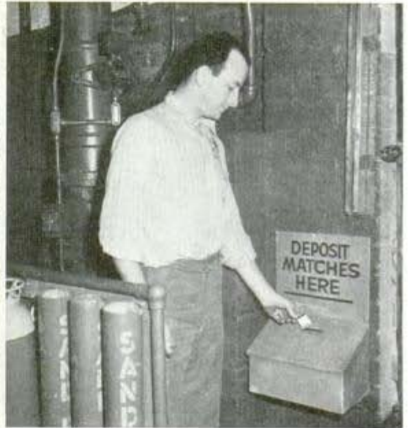
"Dope room" worker at Douglas plant depositing matches as he enters working quarters
