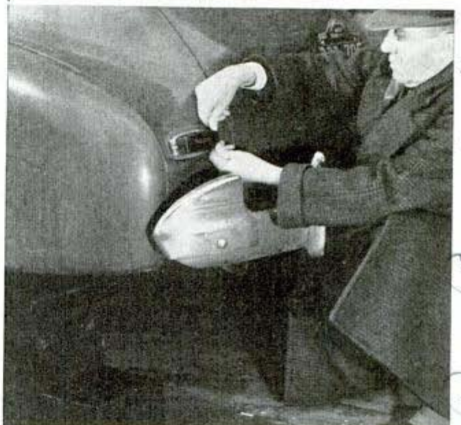
Top, fitting blackout hoods over the headlamps. These slip on easily without special attachments. Below, the taillight mask
