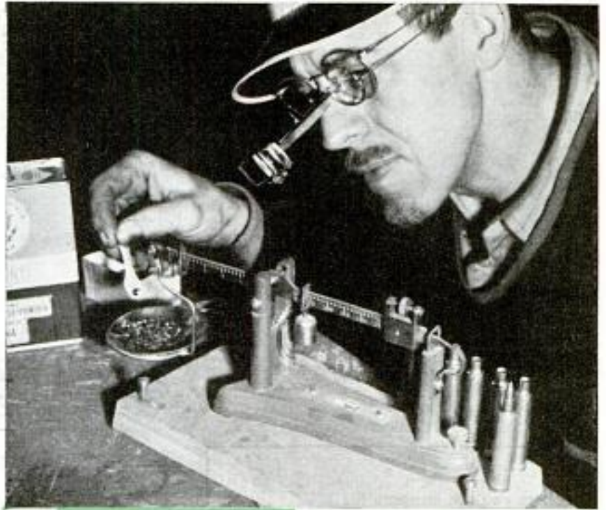
↑ Weighing out the big powder charge for hand-loading super-high velocity .22 magnum cartridge
