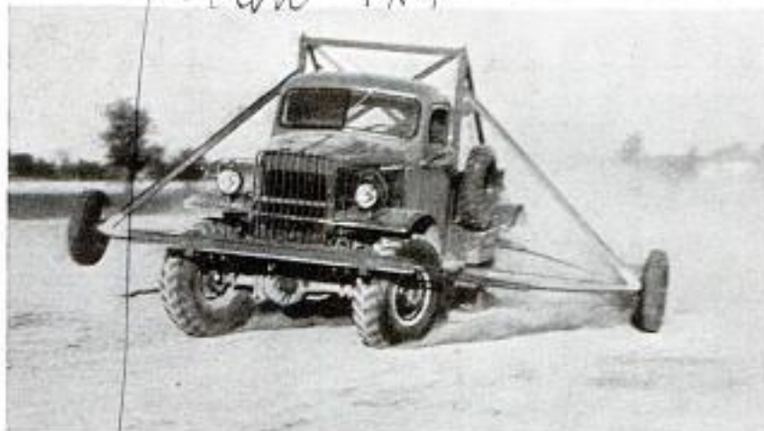
Outrigger keeps truck from tipping over on sharp turns like this one
