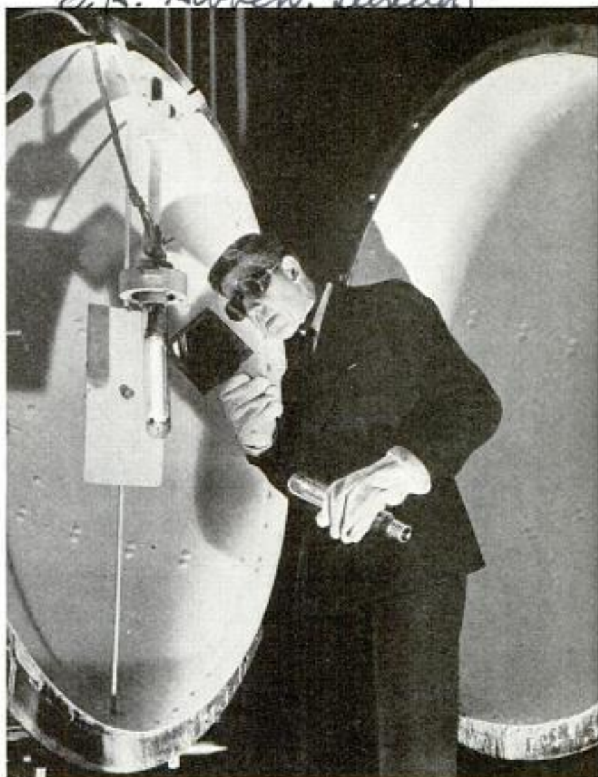
Examining the glass capsule of a powerful mercury-vapor lamp mounted in photometer. Goggles and a special filter shield the eyes when peering directly into the light source
