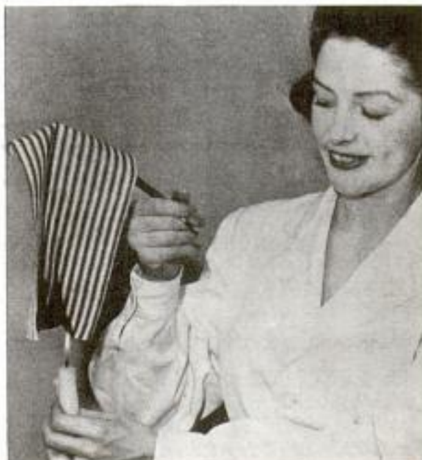
This candle test proves that fabric treated with ammonium sulfamate may char, but it will not flame
