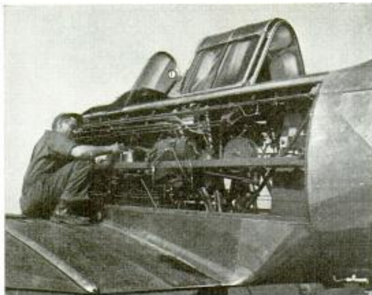
With the skin of its fuselage stripped away, construction and maze of controls of a training plane are exposed. Familiarity with these is an essential part of training
