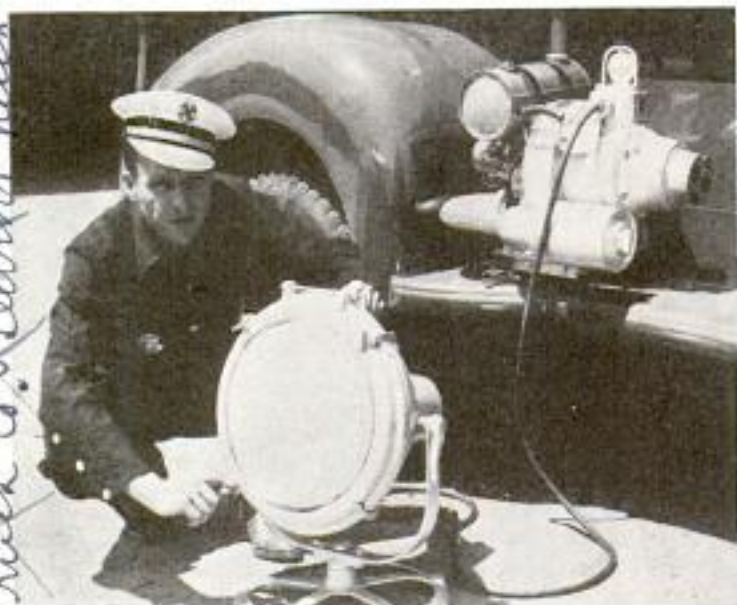
Spotlight run by portable generator helps fight fires at night
