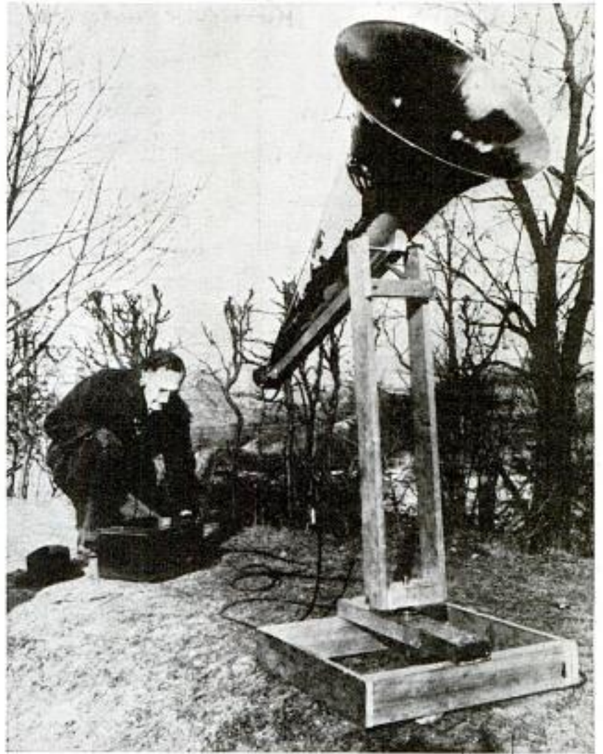
Planes 10 miles away can be spotted with horn and amplifier hookup
