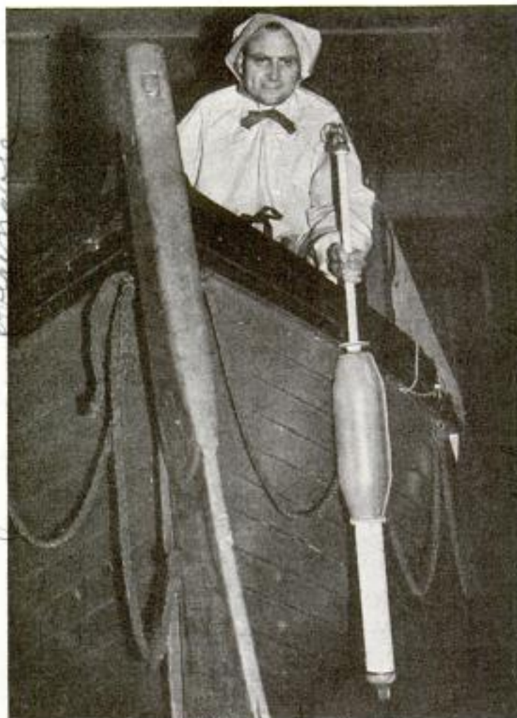
Cast into the sea from a lifeboat, this buoy stays afloat for 60 hours sending S O S signals. Note seaman's hood and cloak
