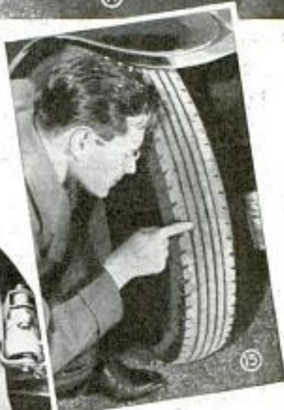
If the tires have been regrooved, check to see if grooves have been cut too deeply into the fabric. Also, be on the alert for a frame that has been repaired as the car may have been in a bad wreck
