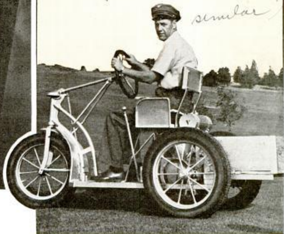
Lightweight car, built by a greenskeeper for traveling around golf course on inspection trips, prevents damage to course
