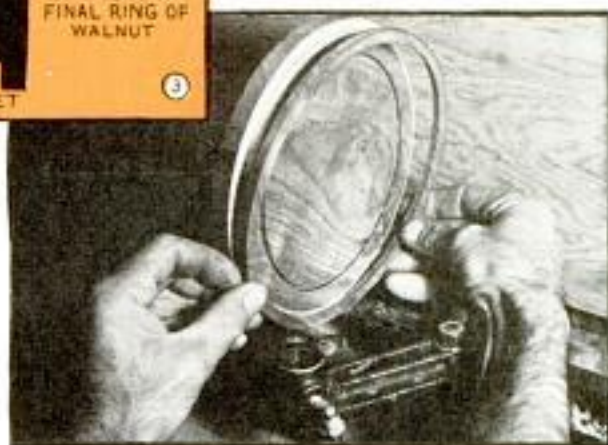
Inlaying is done by turning off one edge to take a maple ring, which is rabbeted to take a narrow walnut ring
