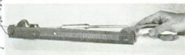
Filings pass through spaces between crosswise blades
