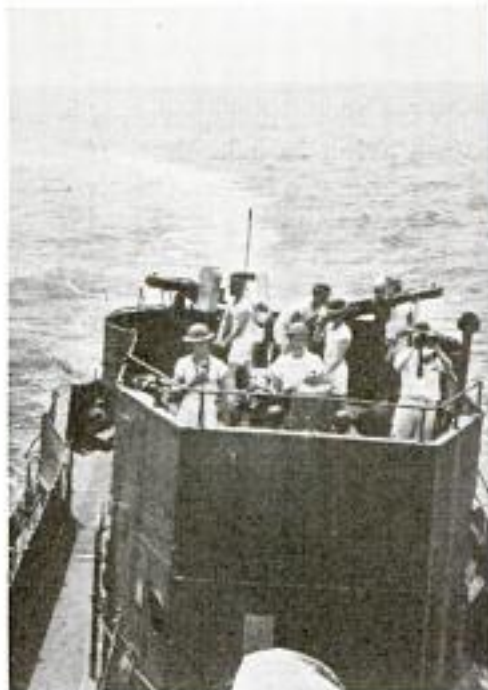
Crew manning secondary or emergency controls of destroyer. These controls are duplicates of those in the pilot house and would be manned in case the pilot house were damaged
