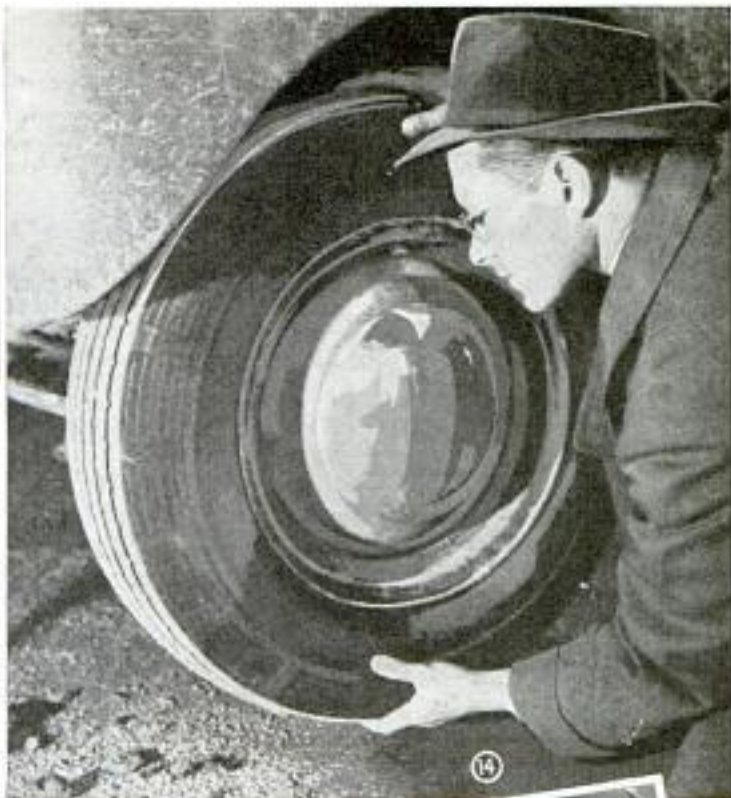
Rocking the front wheel when the car is on a jack will give you an idea of the condition of the spindle bushings
