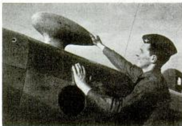
On the fuselage of a "flying classroom" a student inspects the streamline housing of a radio compass
