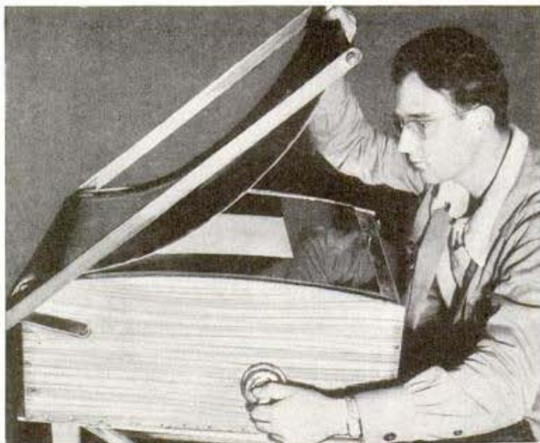
Four 100-watt bulbs inside this homemade print drier provide heat; canvas holds drying tin in place against curved metal top. Below, a film drier is sketched
