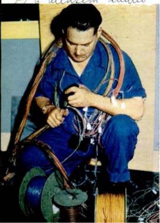
Insulated wires are colored differently to distinguish one circuit from another
