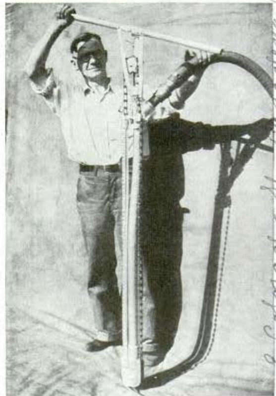
Hollow tube dredge lifts sand and gravel from river
