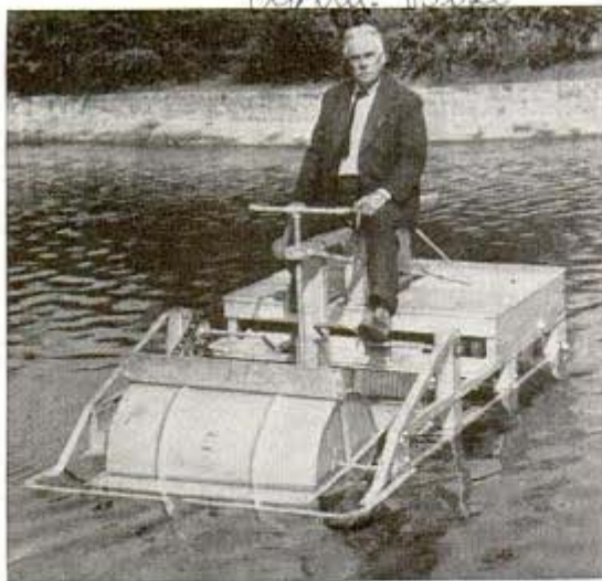
Treadles turn paddle-drum to propel odd fishing craft
