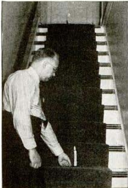
Double candle test, with candle at bottom and another at top of the stairs, indicates drafts; constant, draftless heat is efficient
