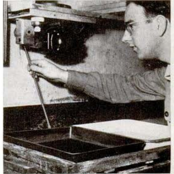
Eccentric arm from electric motor is rigged up to rock developing and fixing trays for quick results
