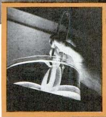
↑ Case-hardened Bausch & Lomb goggles for industrial workers are tested by a barrage of steel balls from an air gun
