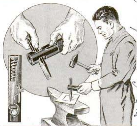
Spring grip for chisel keeps hand from danger zone
