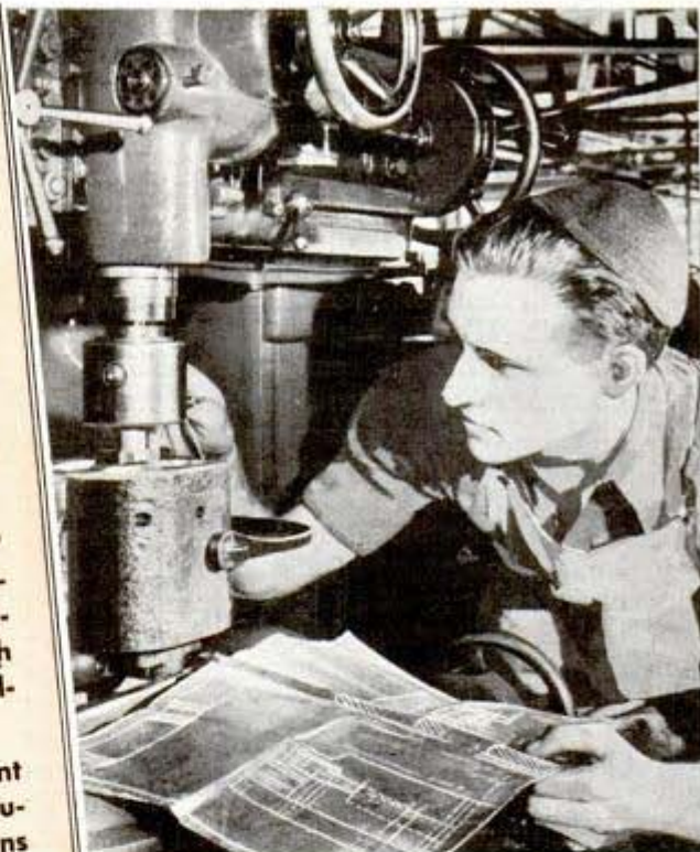
Above: This craftsman in the making is working at a boring mill, which often requires accuracy to .0001 in. Lower left: Men being trained to take charge of groups of operators in a large machine-gun plant
