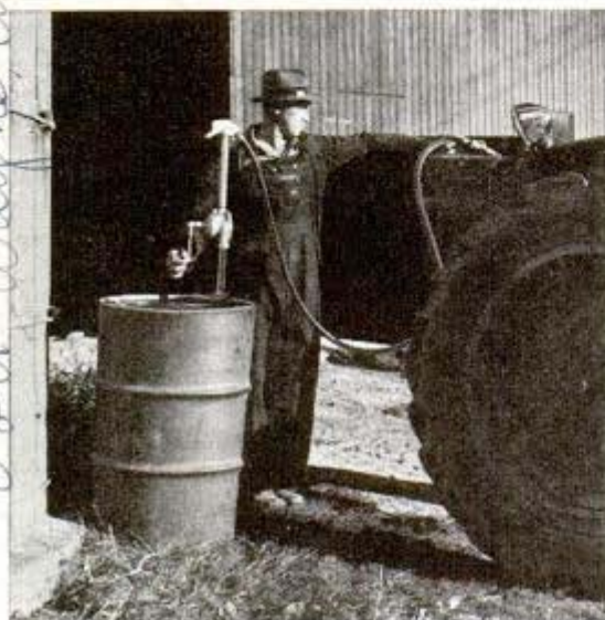
Hand pump makes filling station out of gasoline drum
