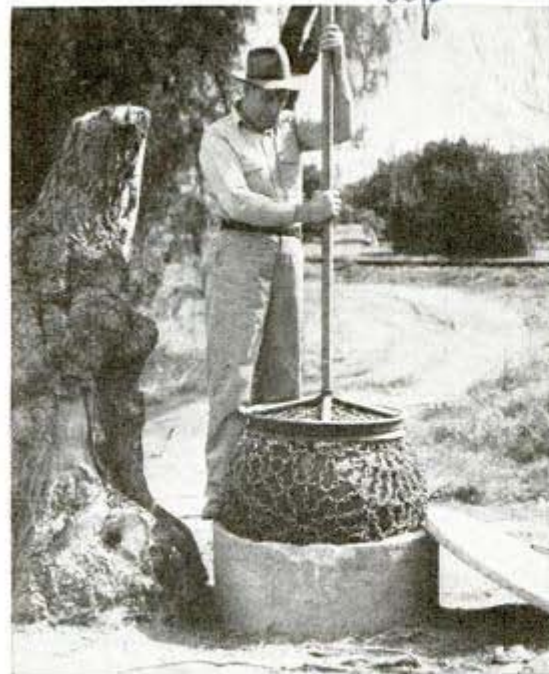
This Rotary Crawler, a chain-covered inflated ball, scours pipes clean; it can be adapted to oil lines
