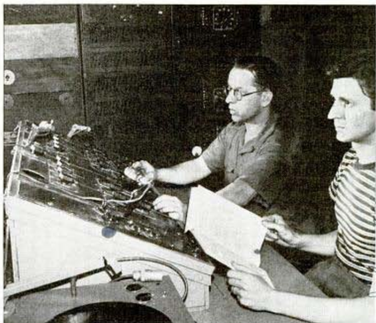
Sunk in ground near stage is this control board for sound amplifiers
