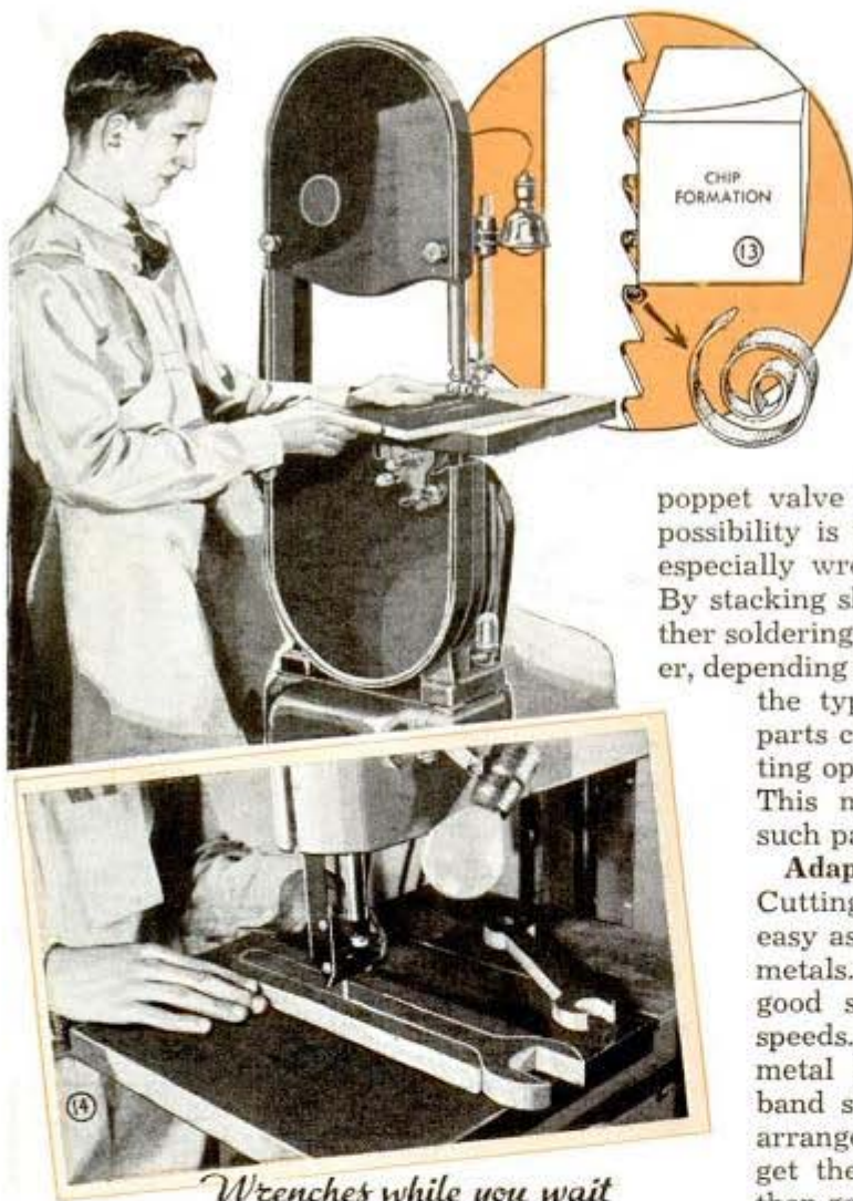
Sharp band-saw blades produce chips of the formation shown in Fig. 13. Simple tools such as wrenches shown in Fig. 14 are cut out in record time and later hardened
