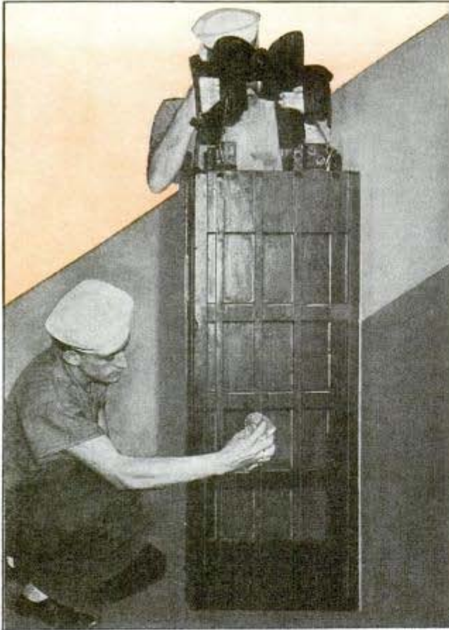
This is single cell of submarine battery; it weighs about 1,600 pounds
