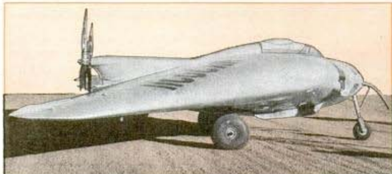
Side view, above, shows tips rebuilt horizontally into the wing; notice extreme thickness of the center section. Spear projecting from apex of wing in the photograph below is the air-speed indicator tube
