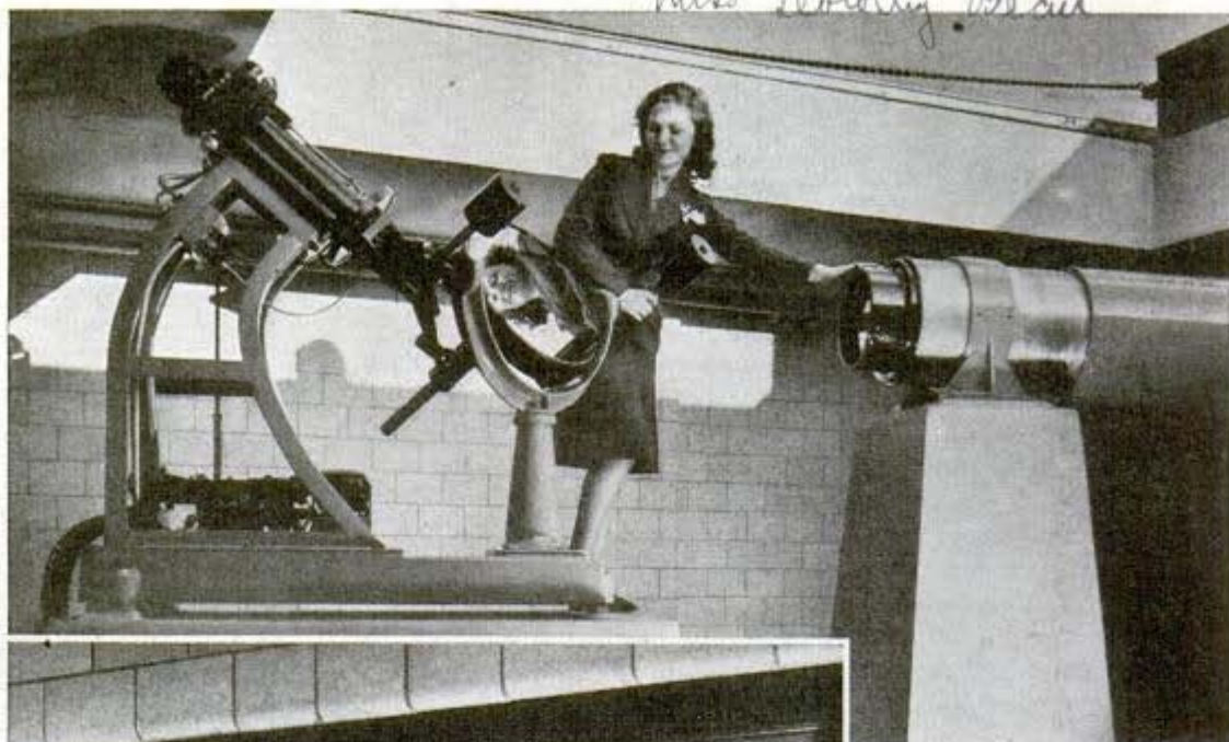
↑ Mirror, center, may be turned to bend ray from any star into ten-inch lens of telescope ← "Seeing end" of telescope. Dials, left and right of eyepiece, control movement of mirror
