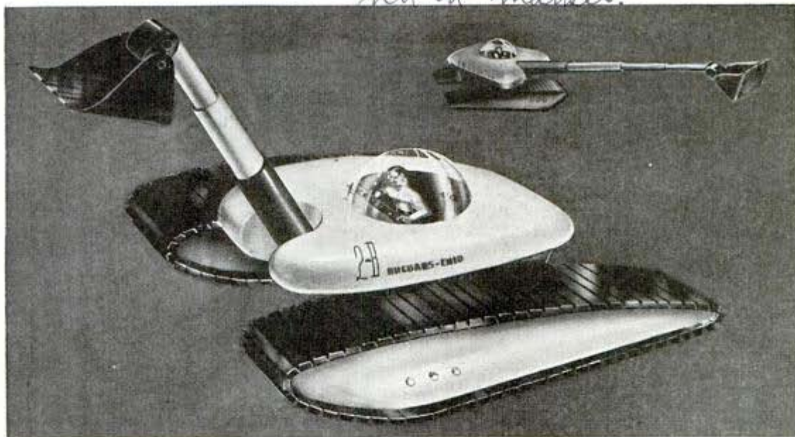
Plastic bodied power shovel, with transparent cab, will have telescoping arm as shown in sketches
