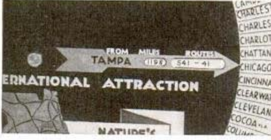
To find mileage, motorist turns outer dial (top) until name of the city appears opposite arrow (bottom)
