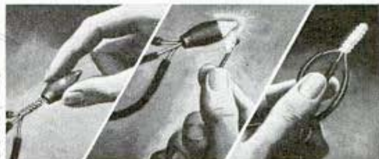
Slip shell on wires, light it, and splice is soldered
