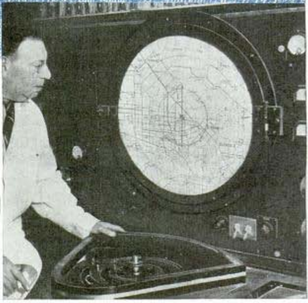
Landing map of flight recorder enables ground watcher to guide oncoming plane directly to the airport
