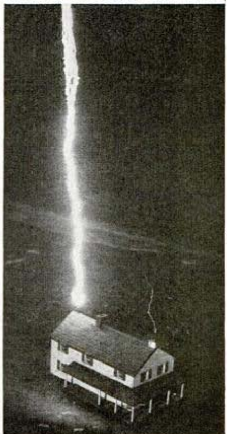
Model house protected by miniature lightning rod → withstands bolt of man-made lightning
