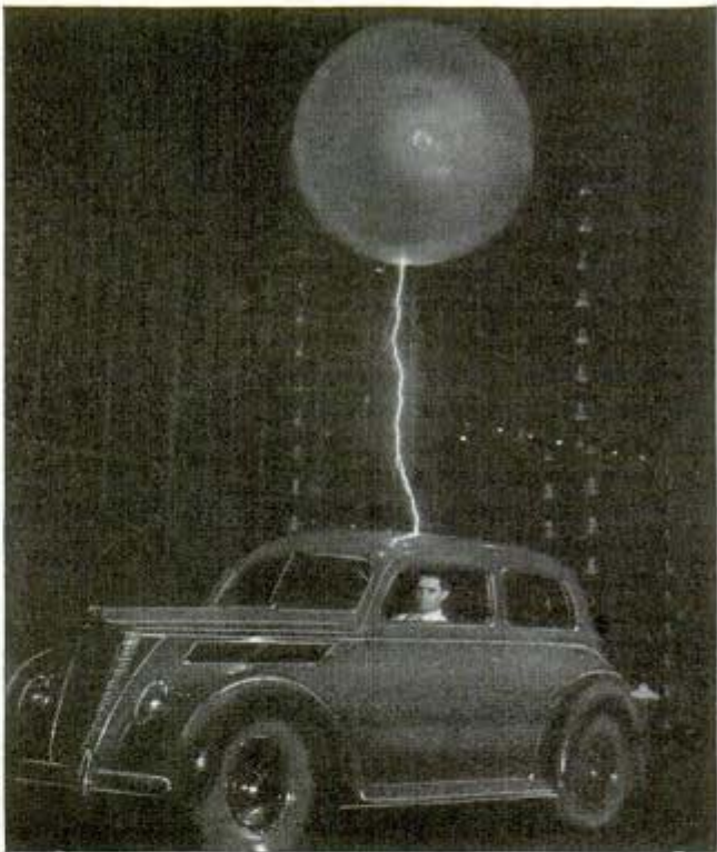
Three million volts of man-made lightning hits car while author sits at wheel
