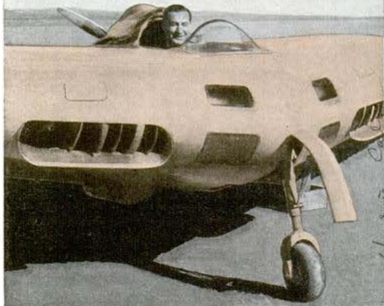
Above, a closeup of center section of the flying-wing plane with Northrop in cockpit. Openings admit air to carburetor and to cool engines
