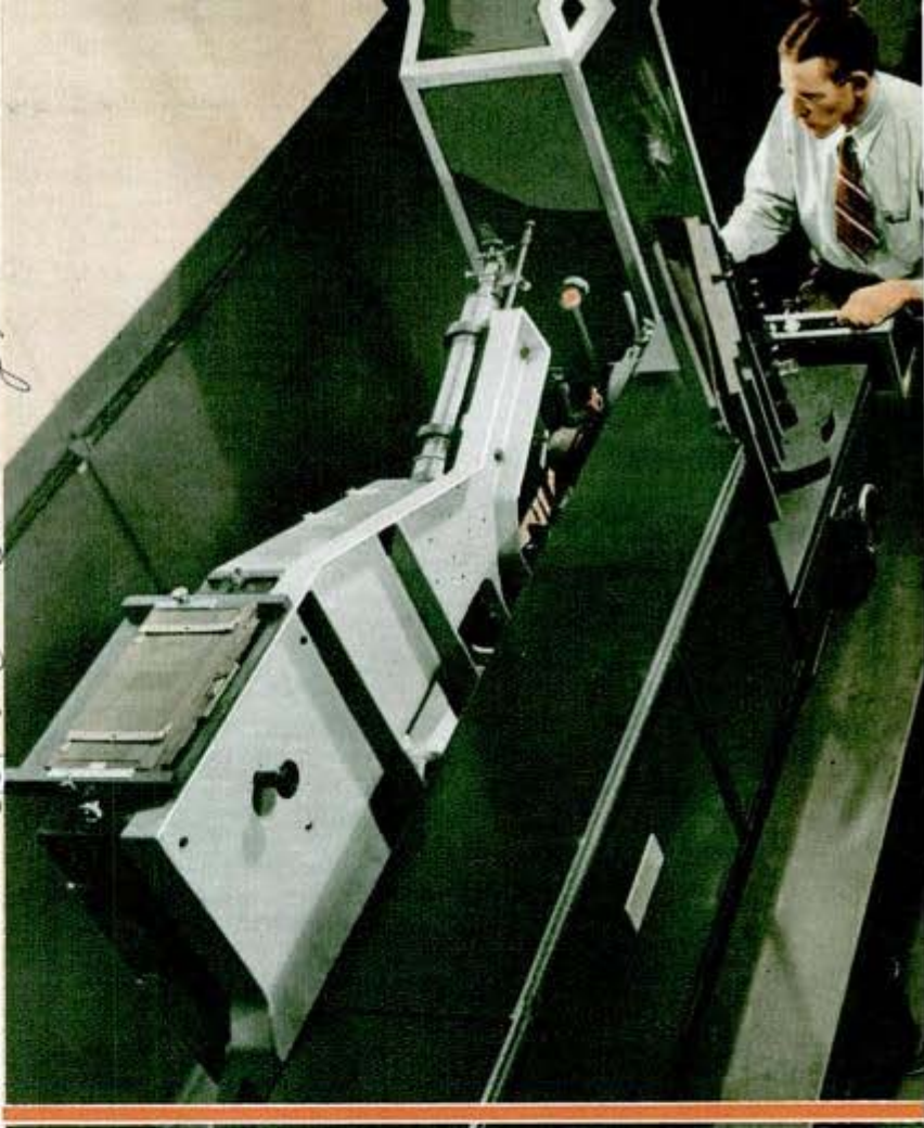
Westinghouse Spectrograph uses photographic film in analyses of unknown materials
