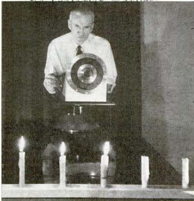
Fast whirling rings of air, shot from gun in background, snuff out candle flames. Idea some day may be applied to city smoke
