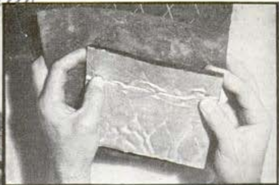
Three kinds of rubber made from milkweed are used in three layers of self-sealing aircraft fuel tank
