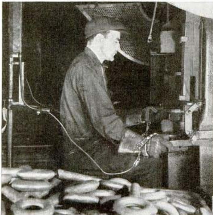
Flexible wire cords attached to wristlets of Bethlehem Steel worker shut off trimmer if his hands are in danger
