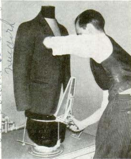
Fin-type heater dries coat after it is pressed
