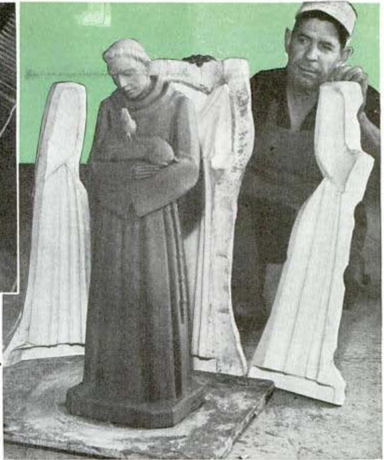
Workman removing plaster of Paris form from terra cotta statue →
