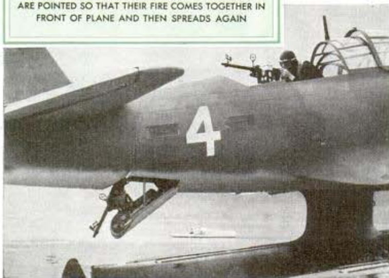
Northrup seaplane fighter with two machine guns. Lower gunner lies on stomach to fire
