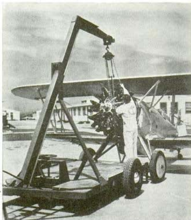
Trailer crane eases and quickens removal of airplane engines
