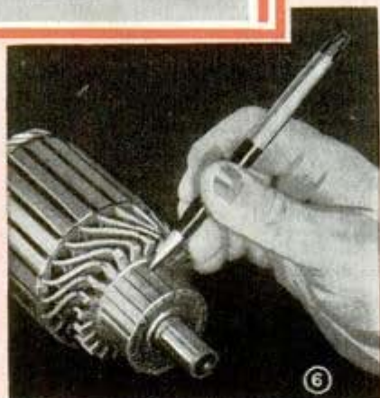
Mica on a starter commutator is not usually undercut as dust would collect in the grooves and cause short-circuits
