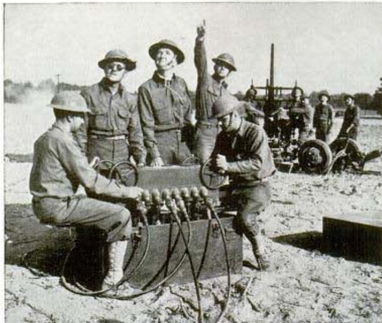
Tracer control box aims antiaircraft gun at "predicted" position of plane
