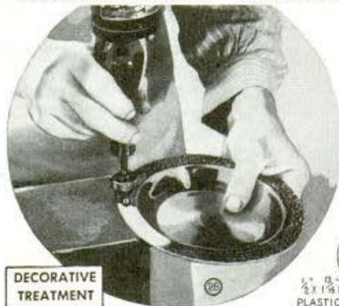
SPINNING SHALLOW TRAY SHAPE ON INTERNAL CHUCK
