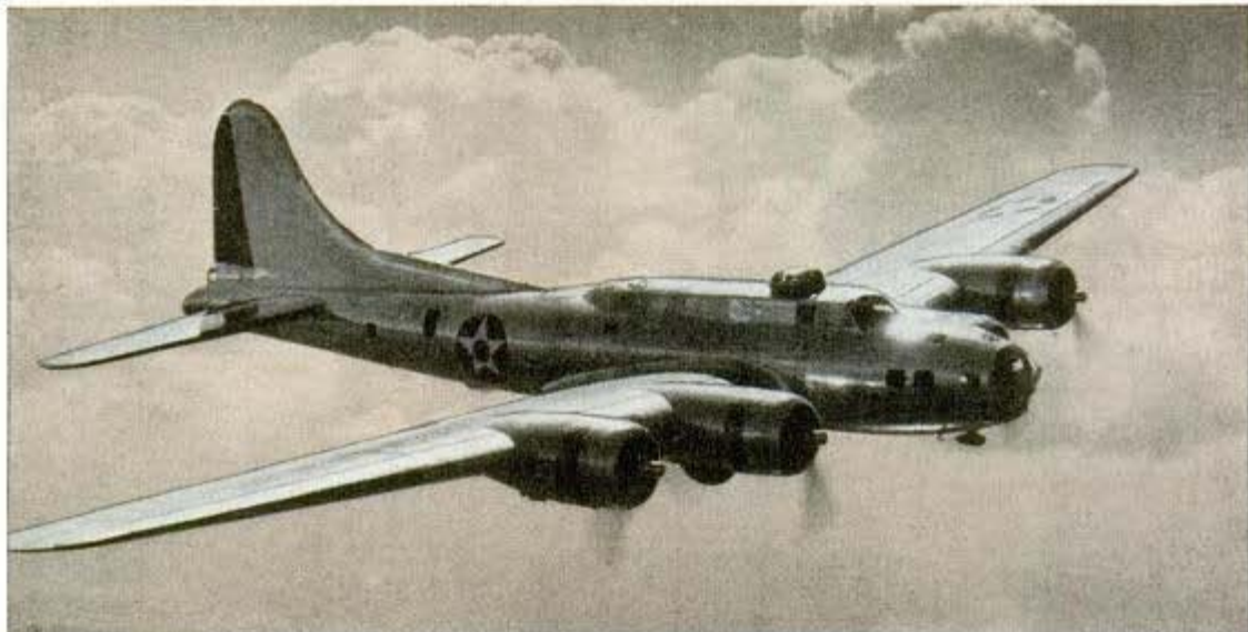
↑ Latest version of the Boeing Flying Fortress showing upper, lower and forward and rear gun emplacements; it is intended for high flying
