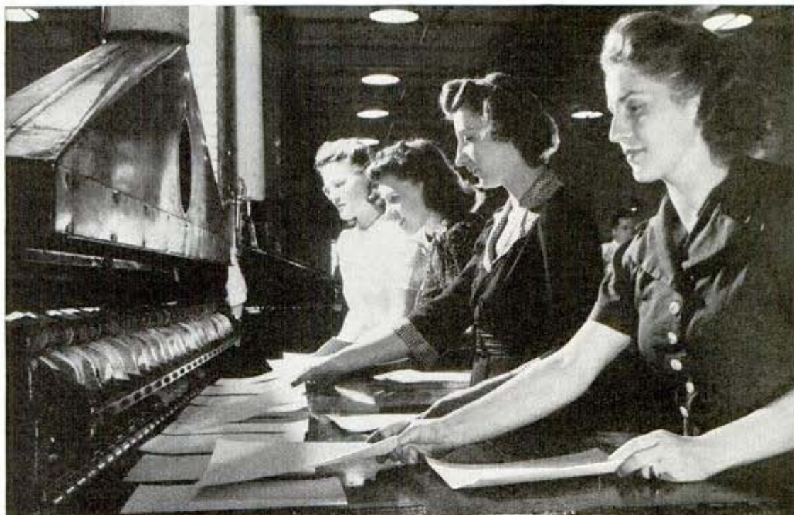
Fed by hand, this printer develops daily thousands of easy-to-read "positive" copies of defense plans
