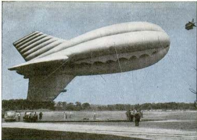
Four-fin balloon (above) inflated and ready for ascent after removal from hangar. Below, odd-looking barrage balloon of type being built for the Army by General Tire & Rubber Company
