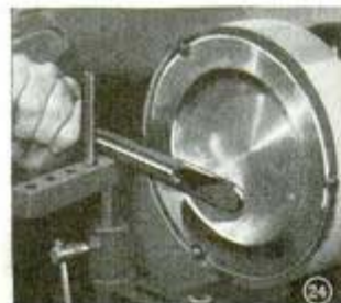
SPINNING SHALLOW TRAY SHAPE ON INTERNAL CHUCK
