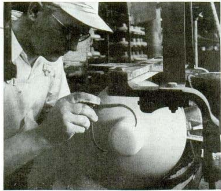
A porcelain high-tension line insulator is turned to shape on a lathe
