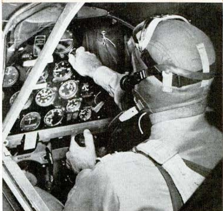
Pilot turning selector switch controlling guns to be fired
