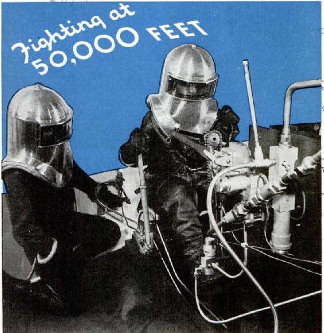
Garbed in fantastic aluminum helmets and heavy fleece-lined horse-leather suits, cold-room workers test hydraulic control system to find how it would work in the high altitudes
