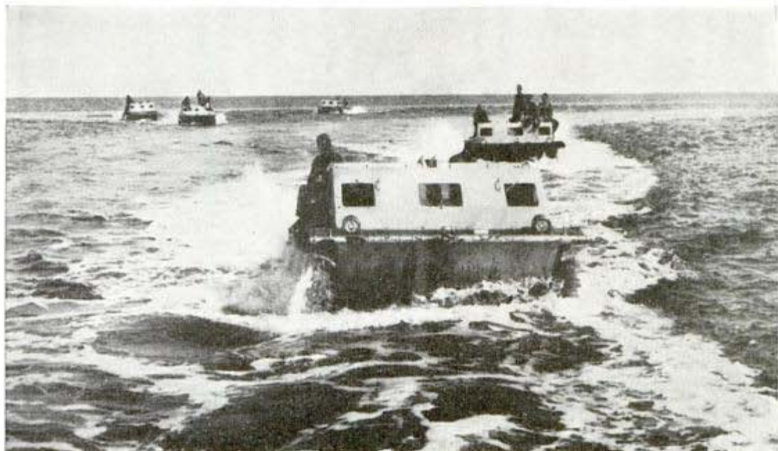
Land-and-water tanks plow through sea at nine miles an hour; they can run at 25-mile clip on land
