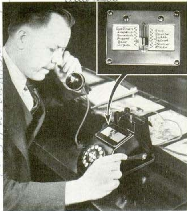
Pointer (inset) and lever make telephone call without dialing
