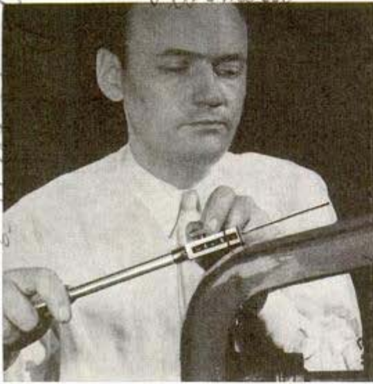
Testing a machine with the meter's vibrating reed
