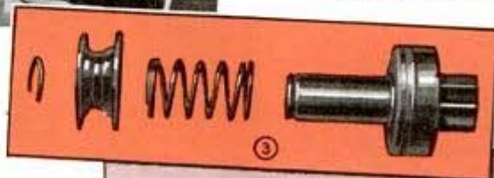
Failure of gear engagement in any starter that has a lever extending down into the starter housing as at the left, indicates a broken engaging spring as shown below. In this type, the pinion is shifted against the teeth of the flywheel under spring tension which results from the movement of the engaging lever against the spring collar. As the lever continues forward the starter switch is closed
