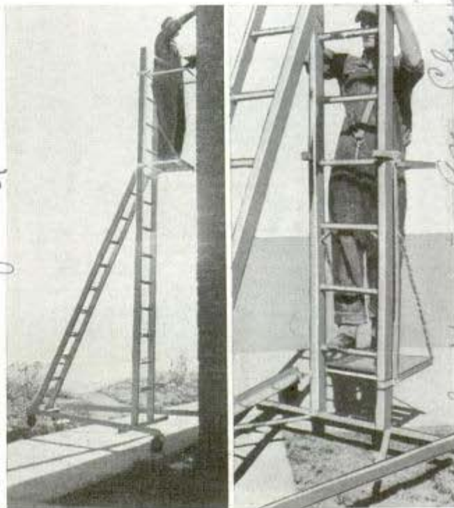
Ladder and platform can be folded quickly to a compact bundle
