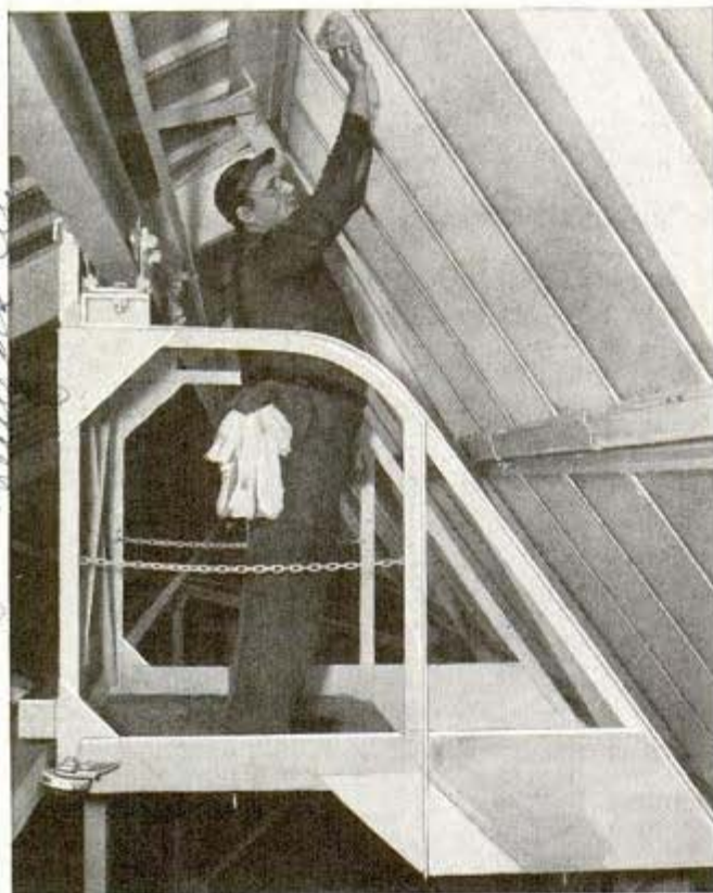
All windows in factory roof can be reached from an aerial car
