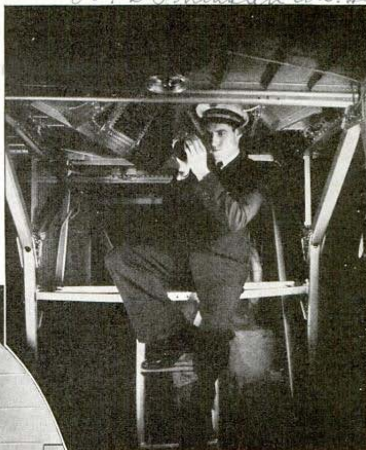
↑ Navigator of a Clipper is shown taking star sight through transparent "astro dome"
