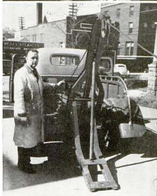
Upper view shows scoop lifting a car by front axle
