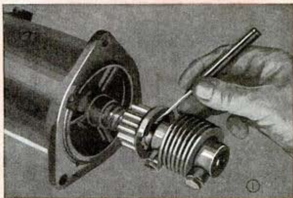
When inspecting a starter-gear mechanism, always be sure the little spring-actuated pin, shown above, is not stuck behind the shoulder on the shaft as this would prevent engagement of the gear with the gear on flywheel
