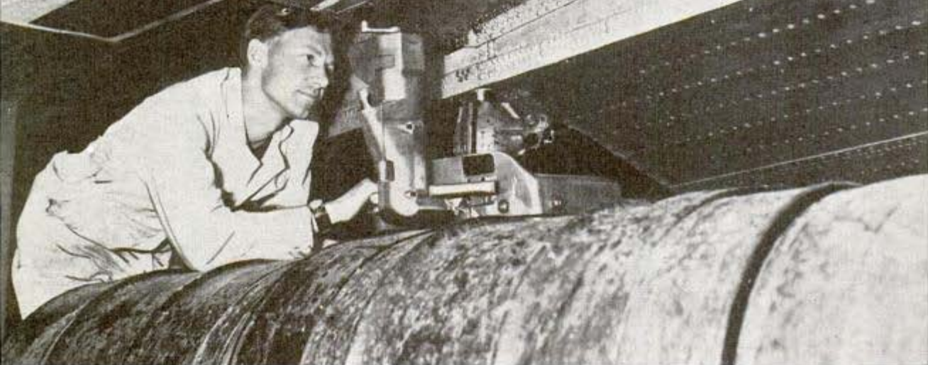
One of four scales on which great Pan American flying boat is placed for weighing at specified intervals
