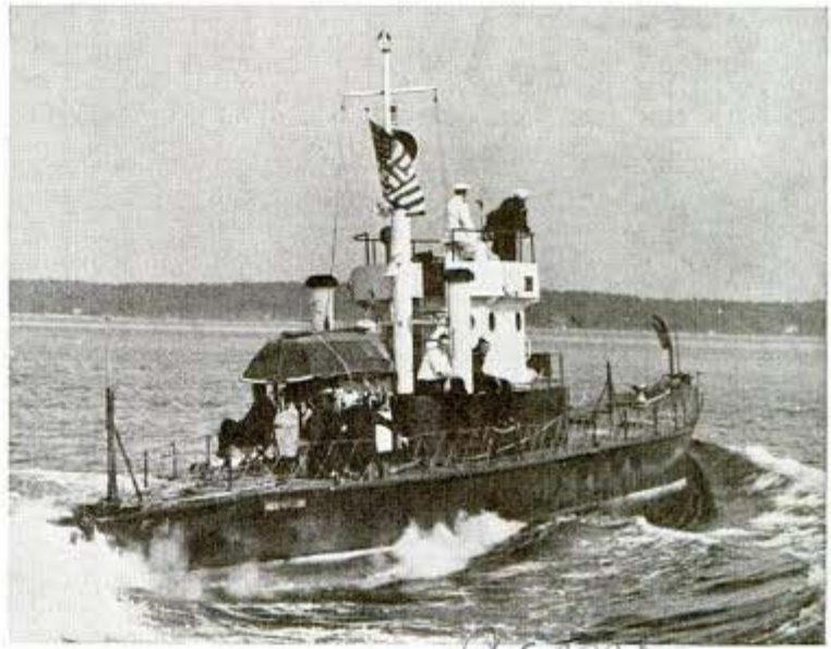
Built for testing purposes, this working model of the "sea otter" is one-third of full-size
