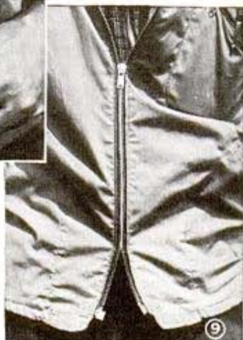
The fastener shown on the sport jacket above has been improperly closed. The combination backstop has not been fitted together before closing the fastener with the result that it has been opened at the rear end as shown in the photo at the right
