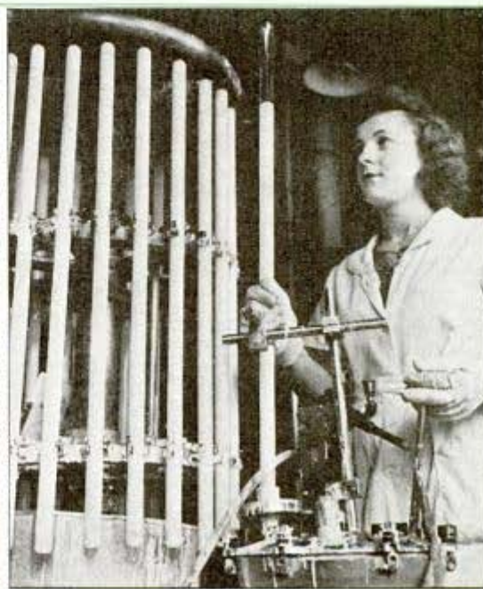
Magnetic pulley wheel, used to ↑ remove iron particles from clay, supports girl by iron in shoes ↓
