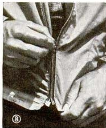
The fastener shown on the sport jacket above has been improperly closed. The combination backstop has not been fitted together before closing the fastener with the result that it has been opened at the rear end as shown in the photo at the right
