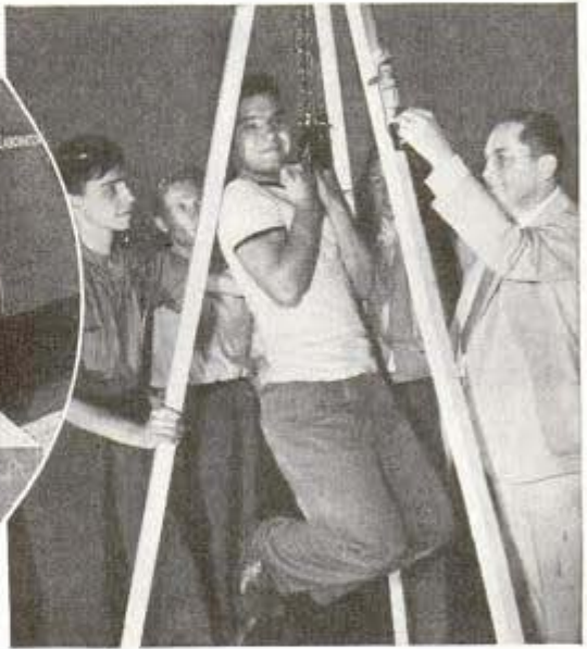
Below, a student hangs from iron disk held by a magnet powered by a flashlight battery. It could support 400 pounds
