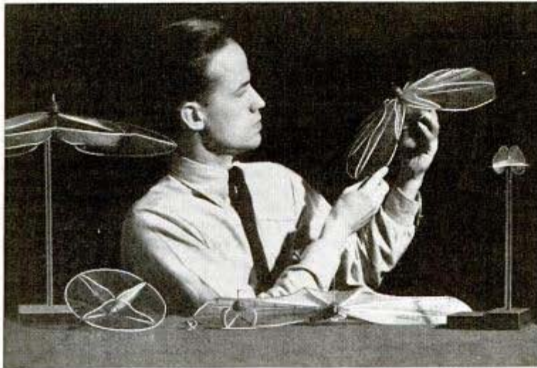
These translucent plastic models show how far street lamps spread light
