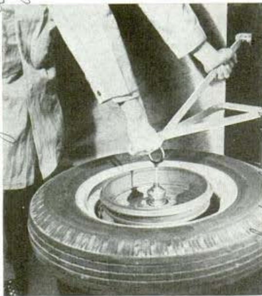
Checking auto-wheel balance with suspension tester
