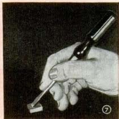
Be sure new brushes are made for a starter; not a generator. Starter brushes show a coppery color when scraped
