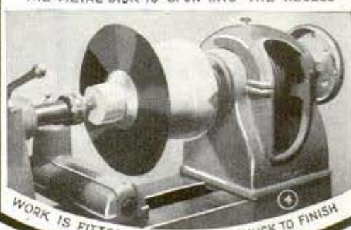
THE METAL DISK IS SPUN INTO THE RECESS
