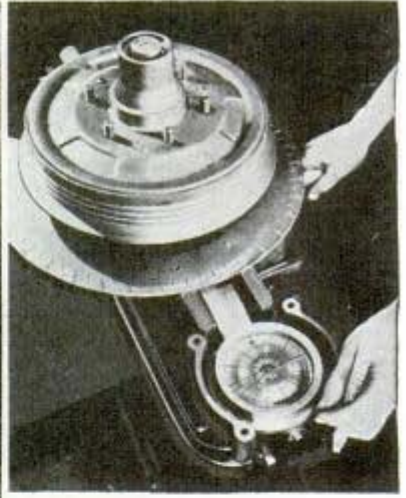
↑ Balancing a brake drum. This helps to eliminate vibration in your automobile ← Operator watches dial to determine amount of excess material to be removed from crankshaft
