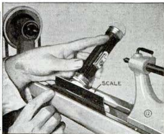
Lead screws on lathes are usually exposed to possible damage and should therefore be examined carefully for ruined threads. Below, checking for wear on lathe ways with a flashlight and a machinist's scale shows up the slightest depressions
