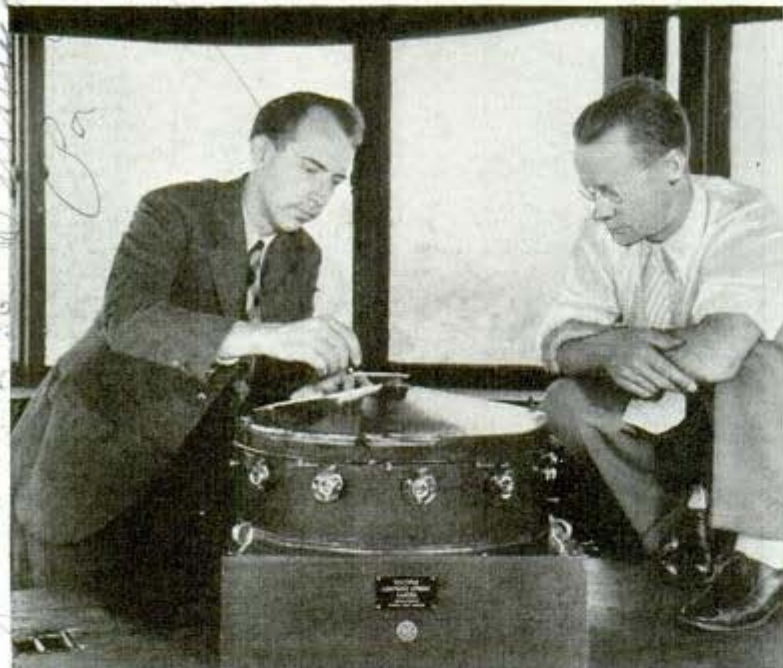
Preparing 12-lens high-speed lightning camera for action in laboratory at Pittsfield works of the General Electric Company
