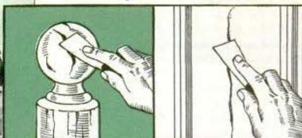
① FILLS CRACKS IN EXPOSED WOOD
