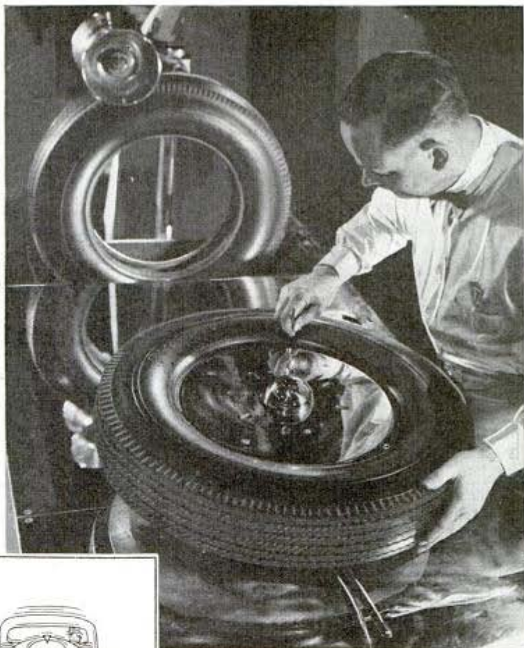
↑ Marking light point on tire casing on balancing machine in Firestone factory inspection
