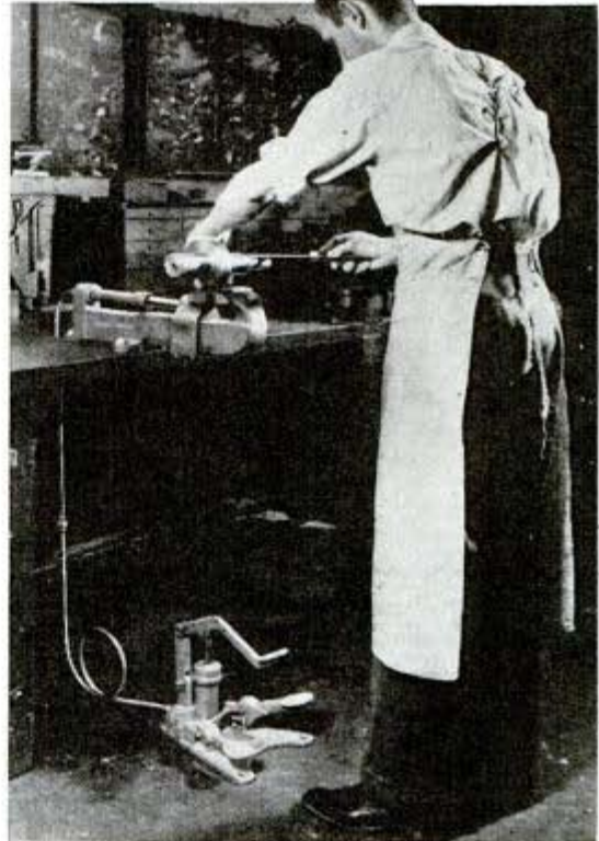
Pedals control movement of vise by hydraulic power
