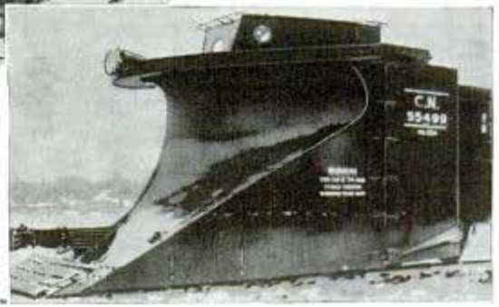
Heavy duty snowplow borrows compressed air from locomotive for extending and retracting massive steel wings. A cupola on top houses controls and protects operator from elements ↓
