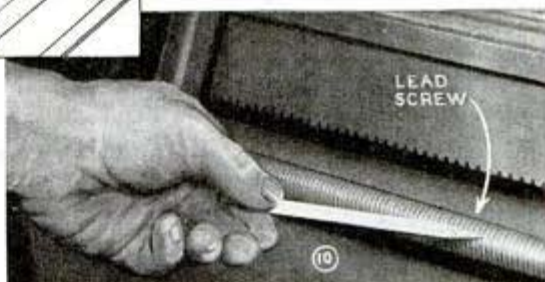
Lead screws on lathes are usually exposed to possible damage and should therefore be examined carefully for ruined threads. Below, checking for wear on lathe ways with a flashlight and a machinist's scale shows up the slightest depressions
