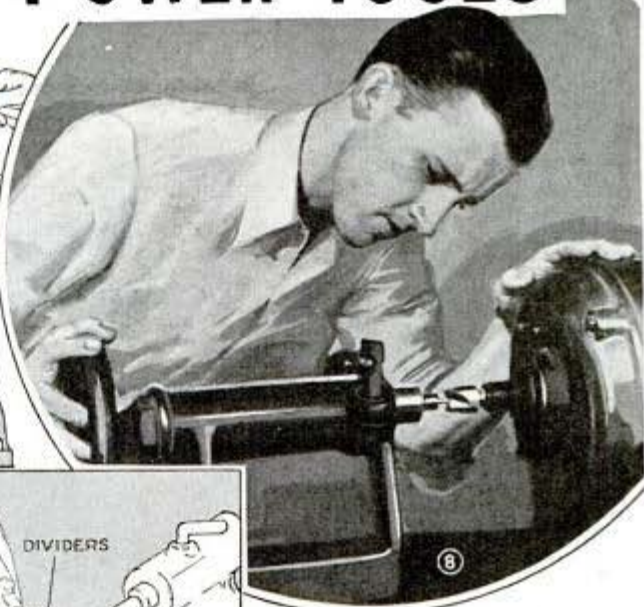
Although by no means an accurate test, two well-ground centers brought as closely together as possible will indicate bad alignment
