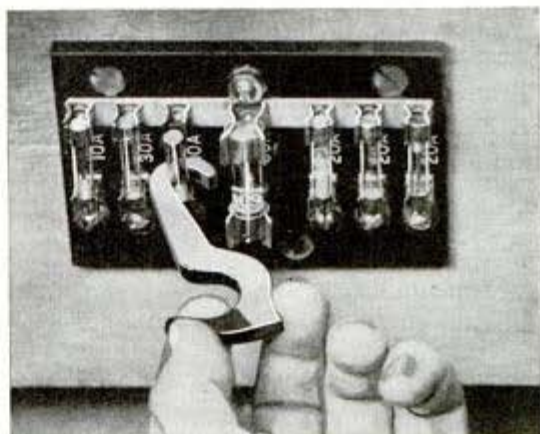
Safe fuse-puller of fiber does not transmit shock
