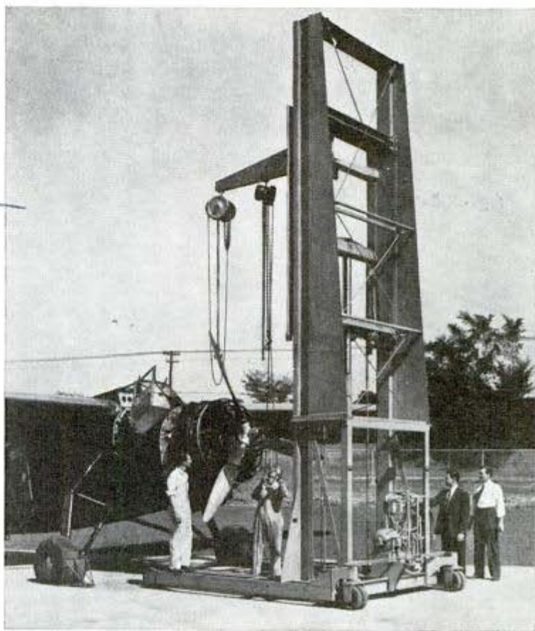
Hydraulic lift can raise 5,000 pounds on its platform or with the boom
