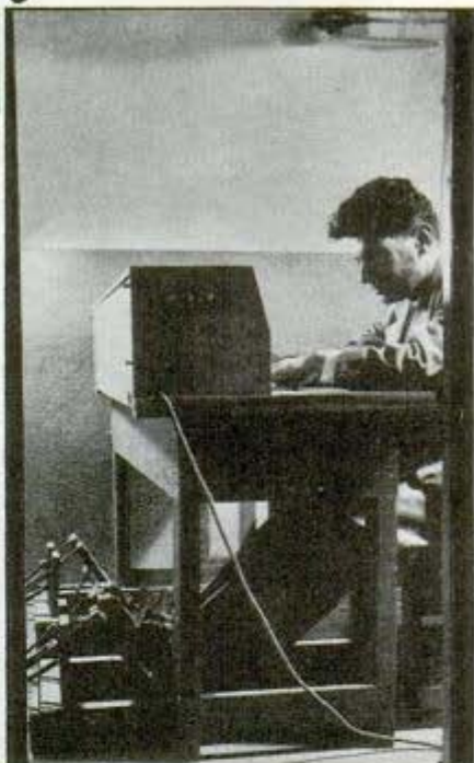
Foot controls linked to work show restlessness of subject in the test chamber
