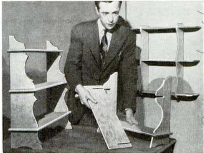
Slots cut in shelves and side panels simplify their assembly
