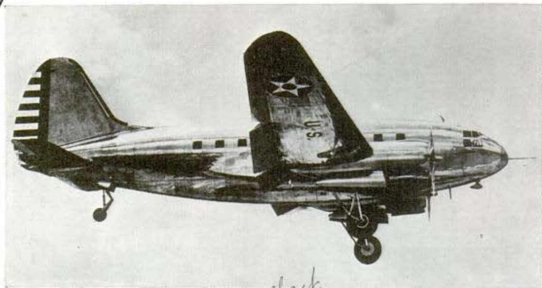
Twenty-ton troop transport plane, converted from passenger ship, has facilities to carry 36 soldiers
