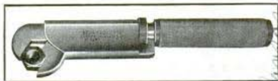
Lower jaw presses two faces against hexagon nut
