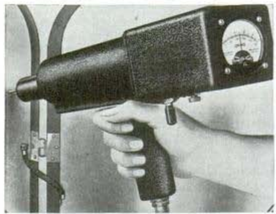
Pistol-grip tester locates faulty electric bonds
