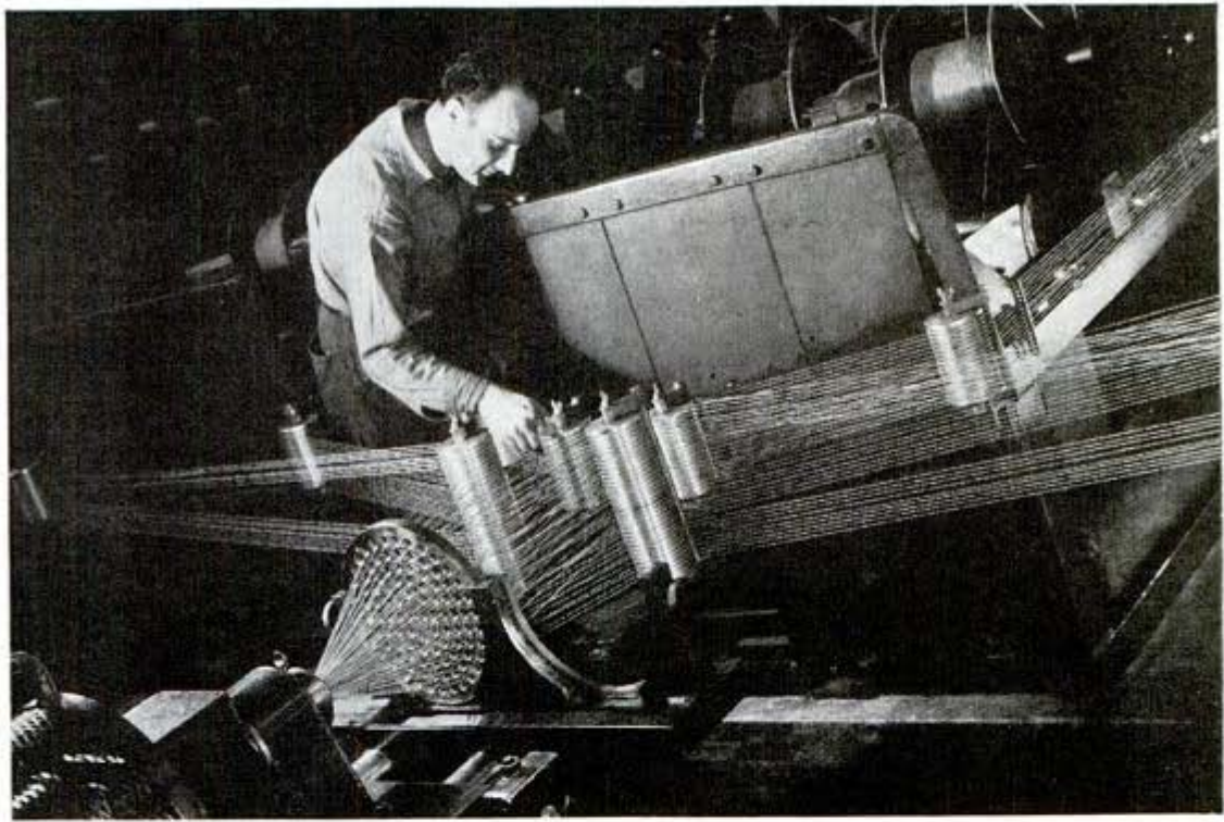
Wires from 101 spools form cone as they are concentrated into cable after passing perforated disk
