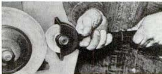
Frequent use of this dresser keeps grinder true
