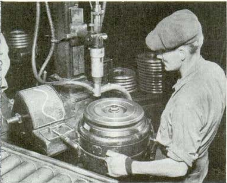
Bulges in line on indicator of static balancer show where fly-wheel being tested is heavy
