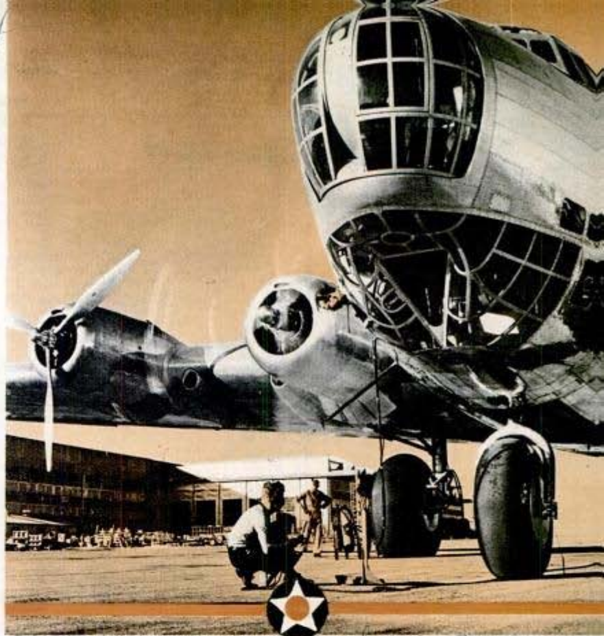
Closeup of the nose of U. S. Army's gigantic Douglas B-19 shows two of the four 2,000-horsepower engines. Below, rushing assembly of advanced training plane. The production pace is being accelerated
