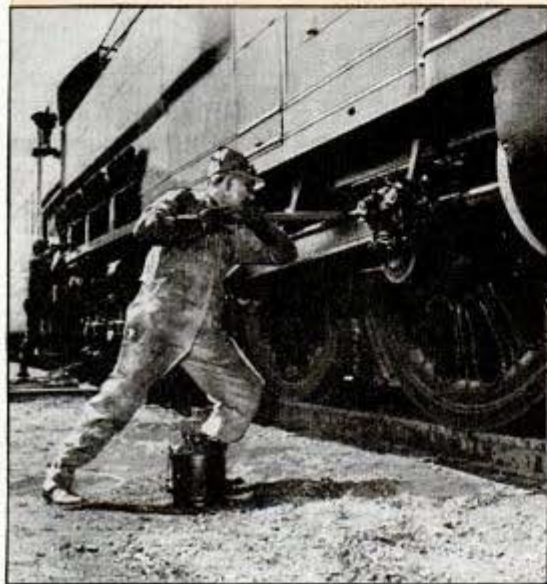
Above, the fireman of No. 6100 checks his gauges as the engineer pulls throttle to start train. Below, lubricating a cross head pin on the engine. There are 350 points for the grease gun
