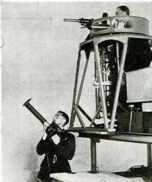
Aerial marksman fires light beam at plane projected on screen
