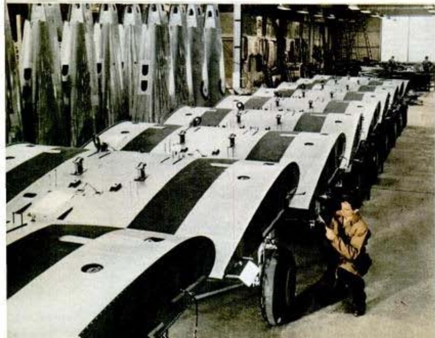
Left, center sections and monocoque rear fuselage sections lined up in North American Aviation plant
