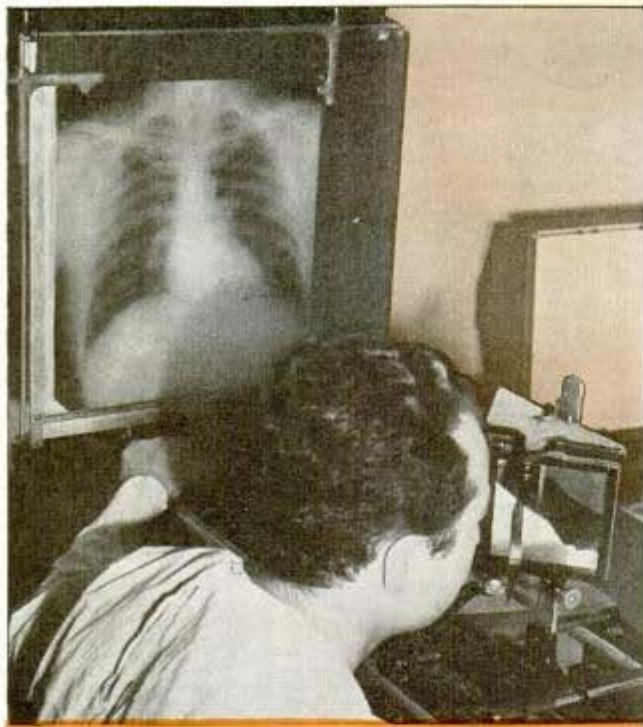
Sighting the stereoptical X-ray viewer, which offers third-dimension effect. One of the two X-ray plates is at upper left
