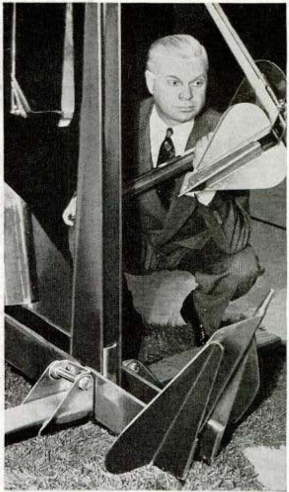
New stainless steel ship anchors weighing 200 pounds replace conventional anchors that weighed tons
