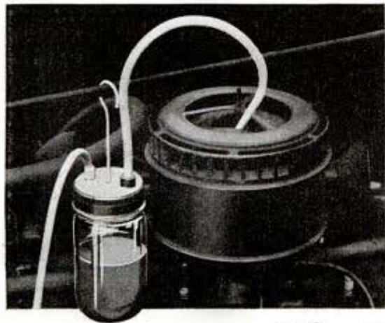
Tube from leak detector carries oil to carburetor through air cleaner, making exhaust visible
