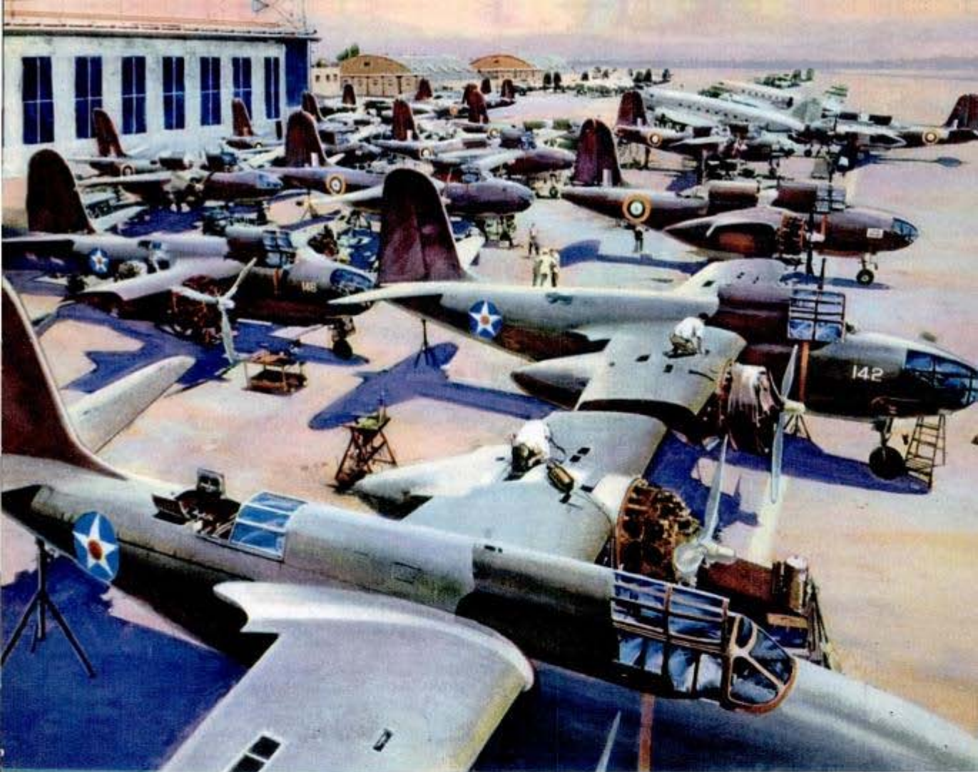
20 2854 Douglas dive bombers and attack bombers on the last lap of their manufacturing and assembly journey
