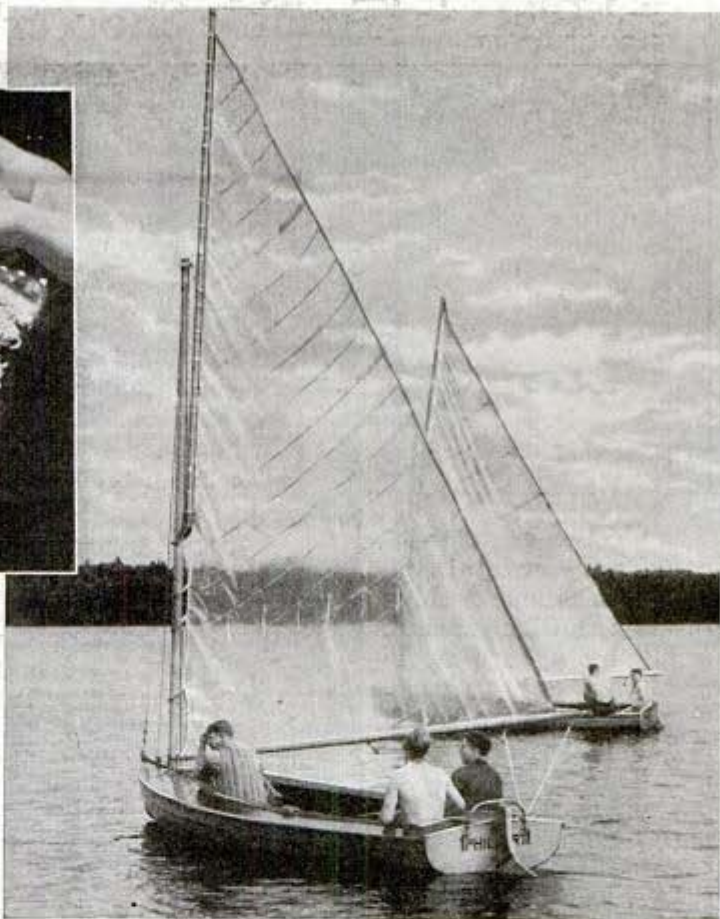
The sailboat in the foreground has a transparent sail fashioned of plasticized Pliofilm. It is light in weight, yet strong and windtight
