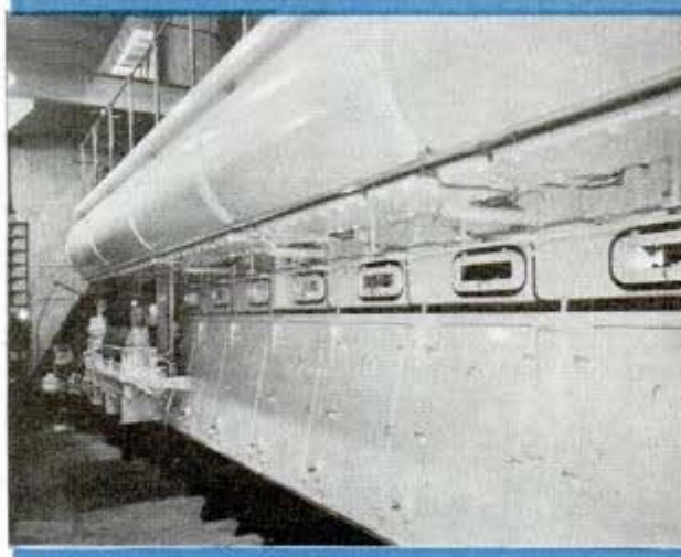
The Kalakala's ten-cylinder Diesel engine is streamlined, too. Ports are for observation of the pistons in operation
