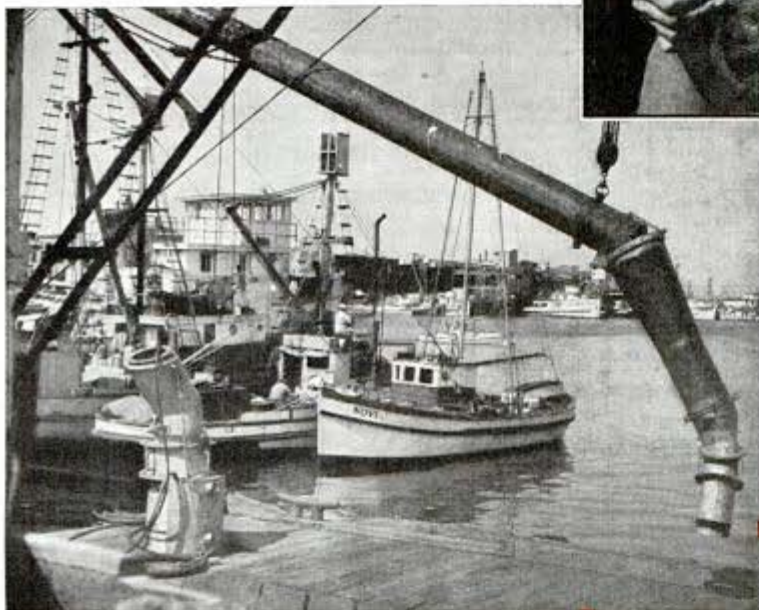
← This is Fish Harbor, Los Angeles, now claimed to be the greatest fishing port in the world. The tube in the foreground is used to load cracked ice in the holds of the fishing vessels
