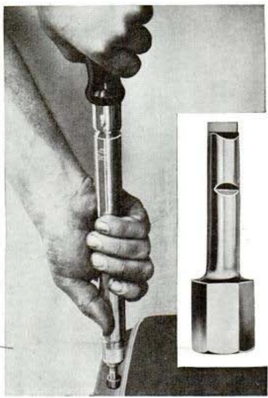
Bit, shown at right, is driven by spiral screwdriver
