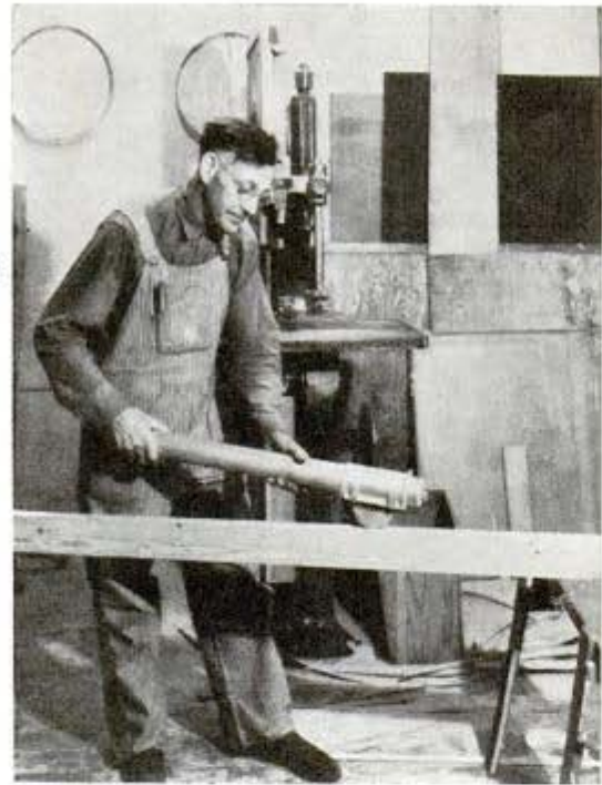
The glue gun lays down its sticky ribbon on a board
