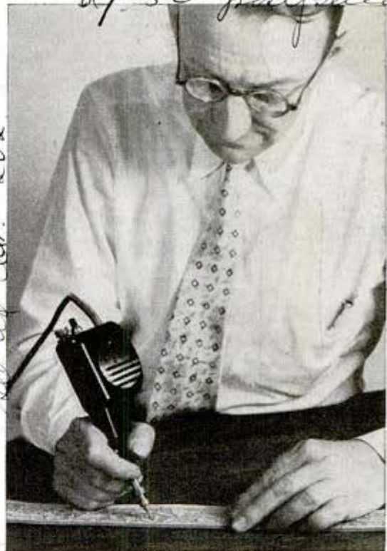
Electric tool vibrates shaft in up-and-down motion to operate hammers, cutters, files and other heads
