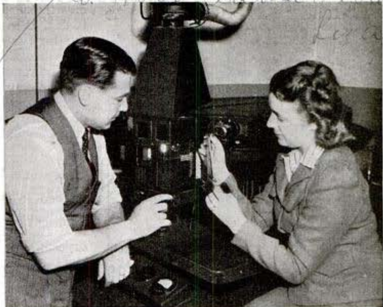
↑ Identity and purity of metal sample is determined with spectrograph
