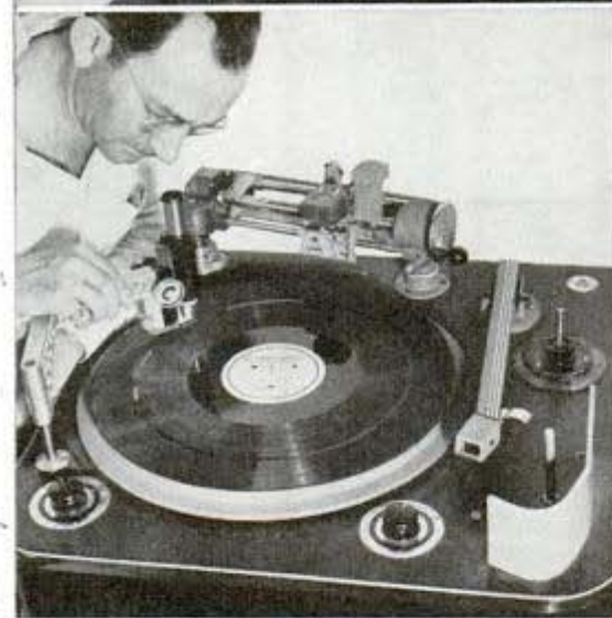
Upper left, scanner transforms movie image into impulses for recording on vision-and-sound disk, shown below. Right, coin machine playing sound movie disk
