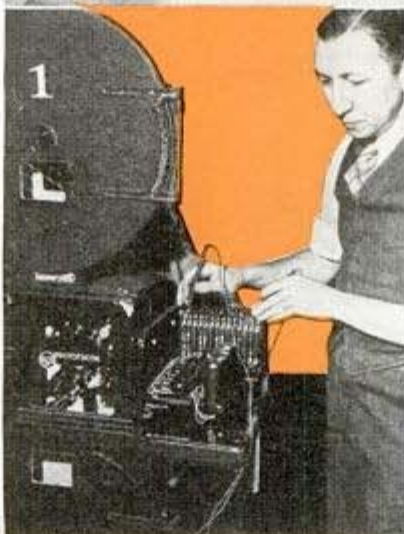
← Engineer testing contact points on newly perfected sound projector that handles special film on which are three sound tracks and one control track which regulates frequency and amplification and controls the speakers from which the sound will come in theater
