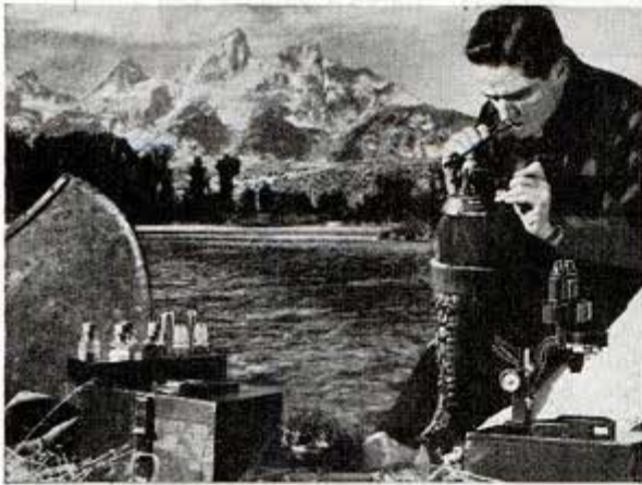
Modern prospector with microscope, blow pipe and chemical reagents making mineral test in the field
