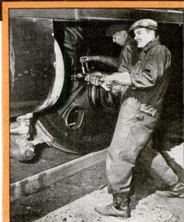
Greasing the rods at the engine's private pit
