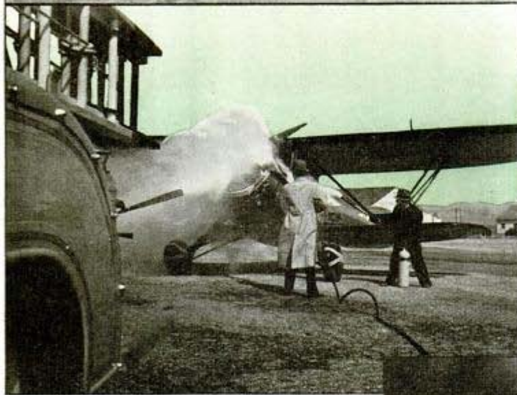
↑ A crash truck on a Long Island flying field pours carbon-dioxide "snow" on a blazing airplane motor Photo, Walter Kidde & Co.
