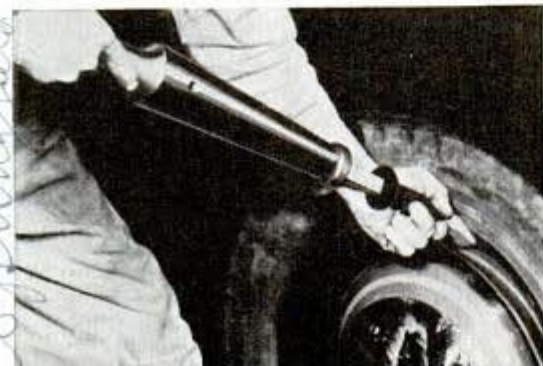
Sliding handle drives wedge between tire and rim
