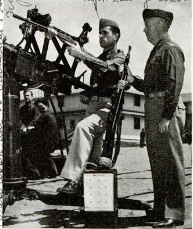
Gunner testing BB rifle attached to .50-caliber machine gun
