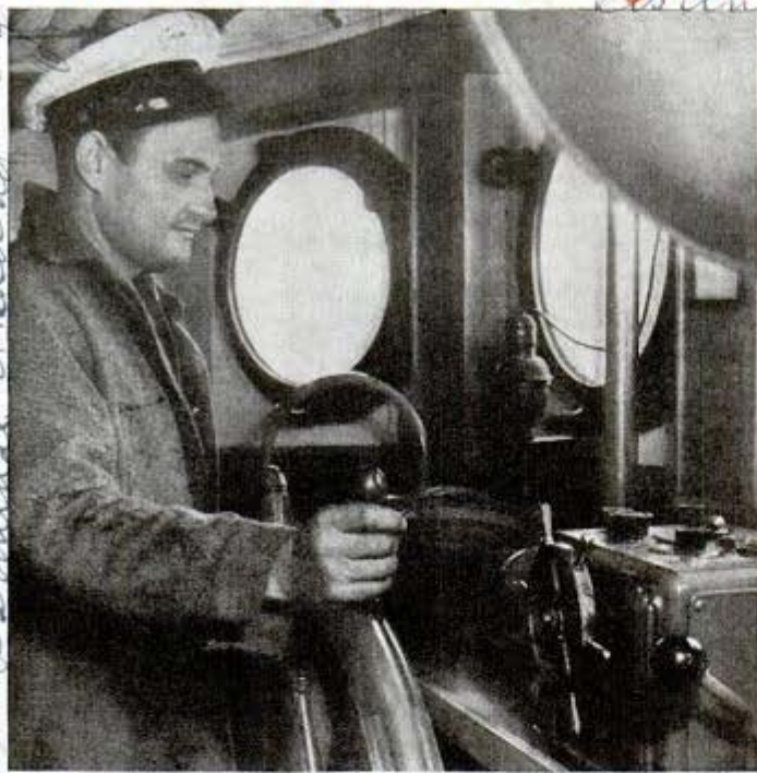
In the wheelhouse of a purse seiner, with "metal mike" automatic wheel in foreground and loop of radio direction finder in the rear
