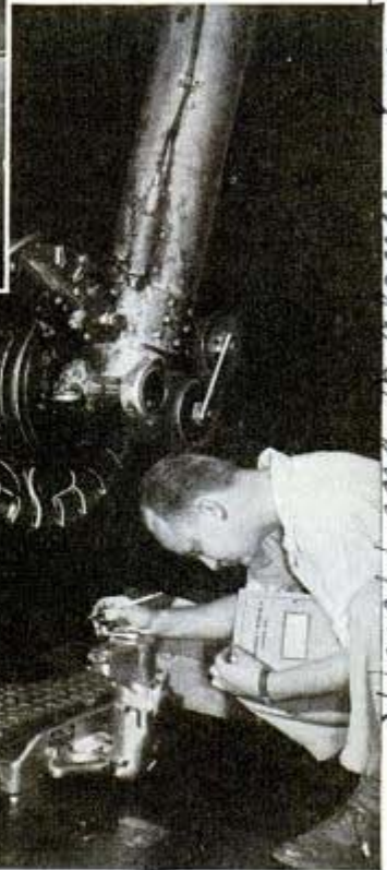
Checking weight shown by two sets of 15,000 pound scales under one of the huge wheels. Total weight was 31,200 pounds
