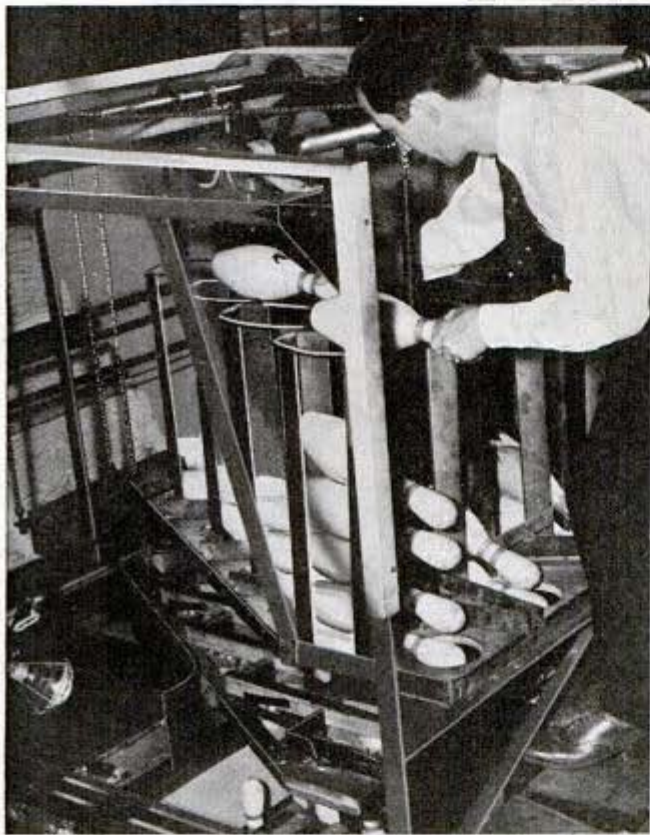
Top, operator presses buttons corresponding to pins knocked down; below, loading pins into the magazine from conveyor belt
