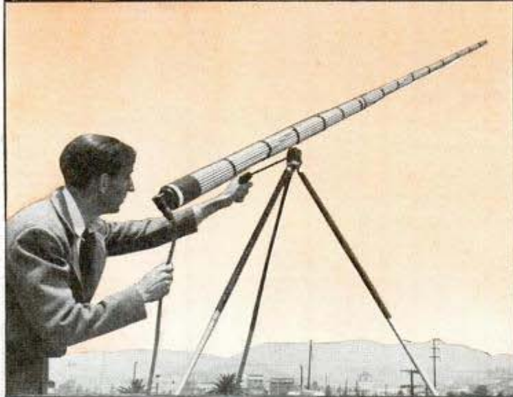
↑ Gun-type microphone screens out all sound except that from direction in which it is pointed
