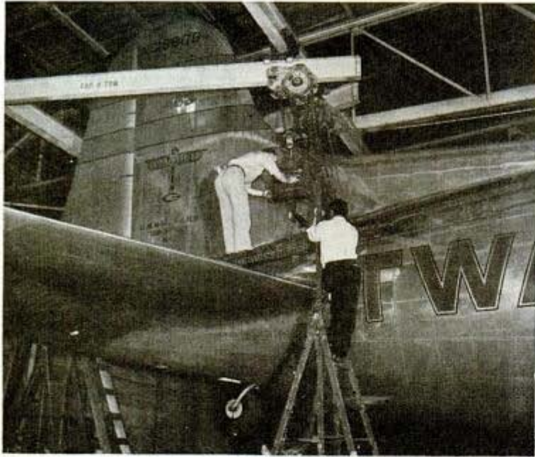
← Tail of Stratoliner suspended from two sets of scales for weighing. Top of fin, in this position, is 30 ft. above floor
