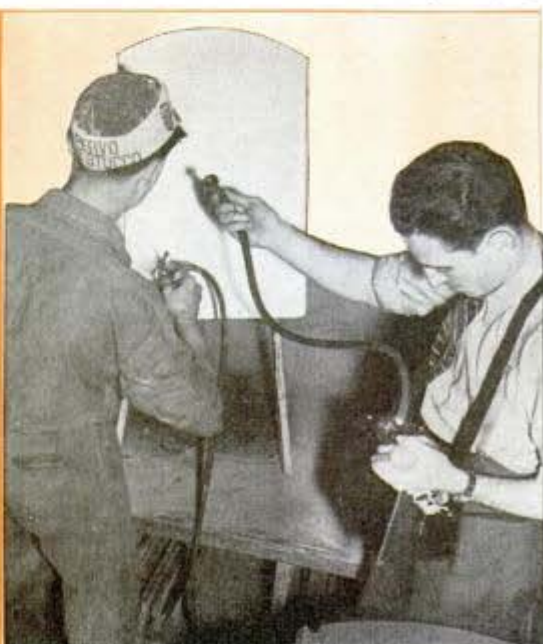
Gas indicator tests toxic fumes from a paint spray
