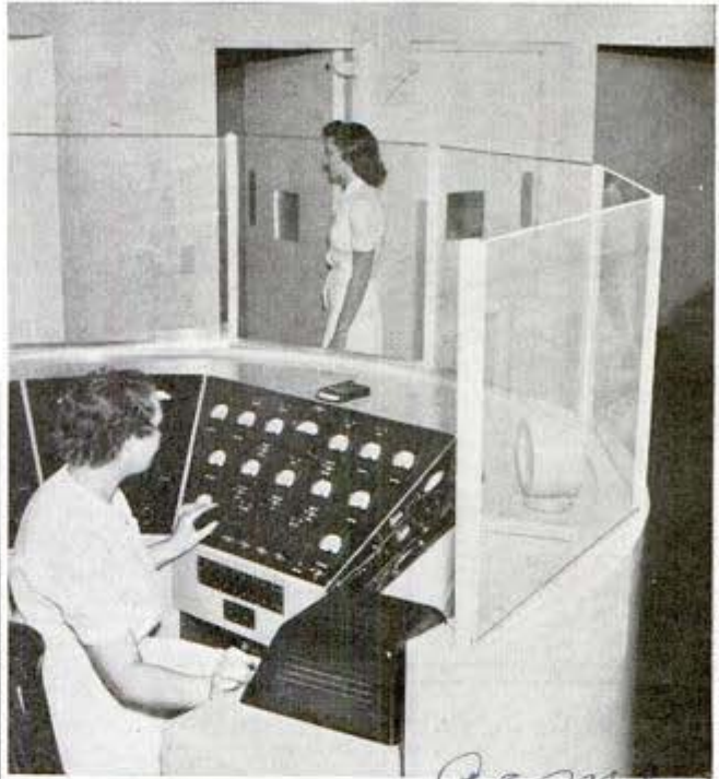
Scene Control desk for the giant and four other X-ray "cancer tubes"
