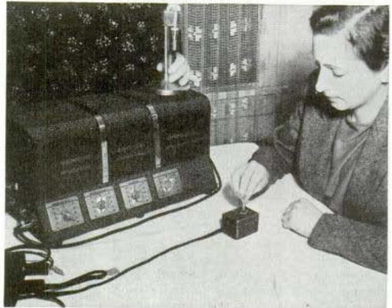
Below, same unit conveys sound from microphone to fingertips
