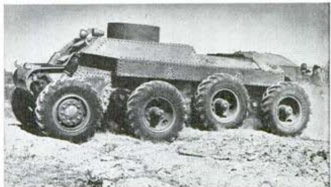
Acme All wheels of "trackless" tank follow rise and fall of ground
