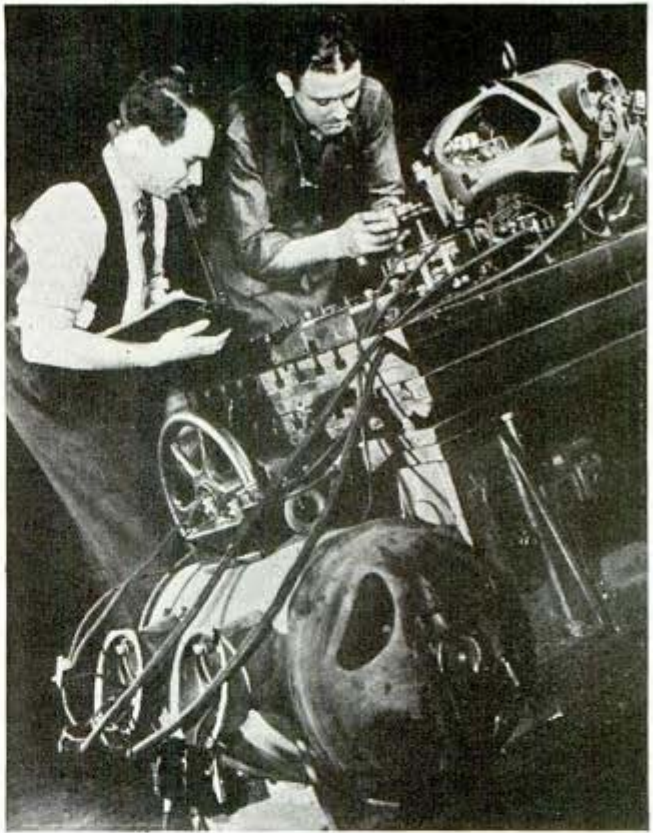
Direct-current motor on bench receives power from generator on floor which in turn is driven by alternating-current motor
