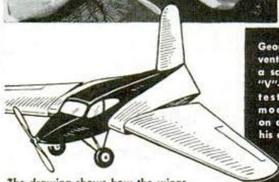
The drawing shows how the wings, rocked in unison or opposition, act as ailerons and elevators
