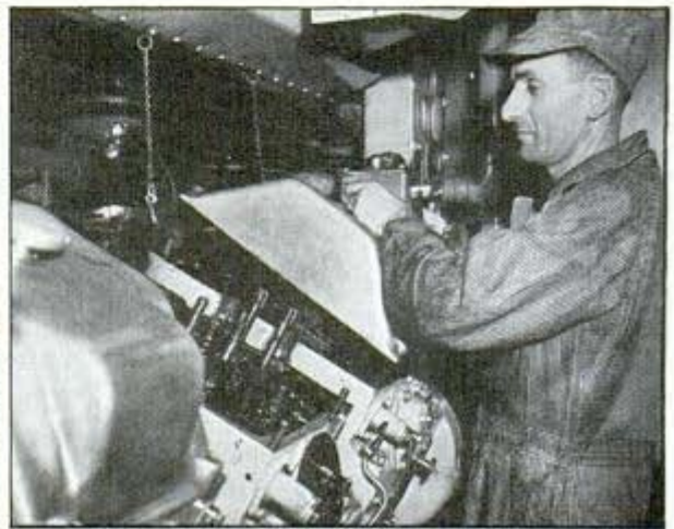
Maintainer of streamline Diesel engine lifts cylinder-head cover to inspect the valves and injector rockers Santa Fe Railway
