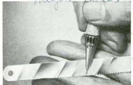
Fine teeth at left end of hacksaw blade start cut in metal; then coarse teeth finish job
