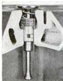
Valve and Bushing in engine ready for grinding.
