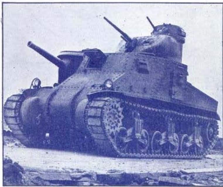
The iron cavalry travels fast and well-armed. Two-way radio keeps in touch with the command and guns are ready for a brush with the enemy Hundreds of these big gun carriers will be rolling from the Chrysler factory before the year ends. This is the "M-3 medium 28-ton tank"
