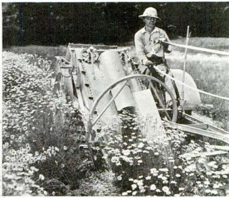
This "daisy" harvester is gathering pyrethrum heads, from which insect sprays are made. Previously pyrethrum flowers always were hand-picked
