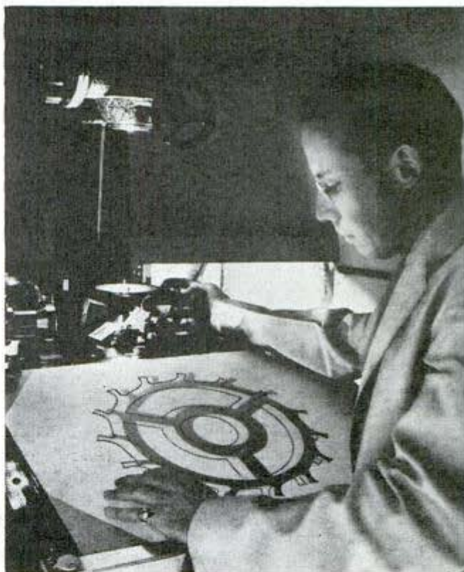
Escapement wheel for watch being inspected by comparing its shadow, greatly magnified, with an enlarged scale drawing.
