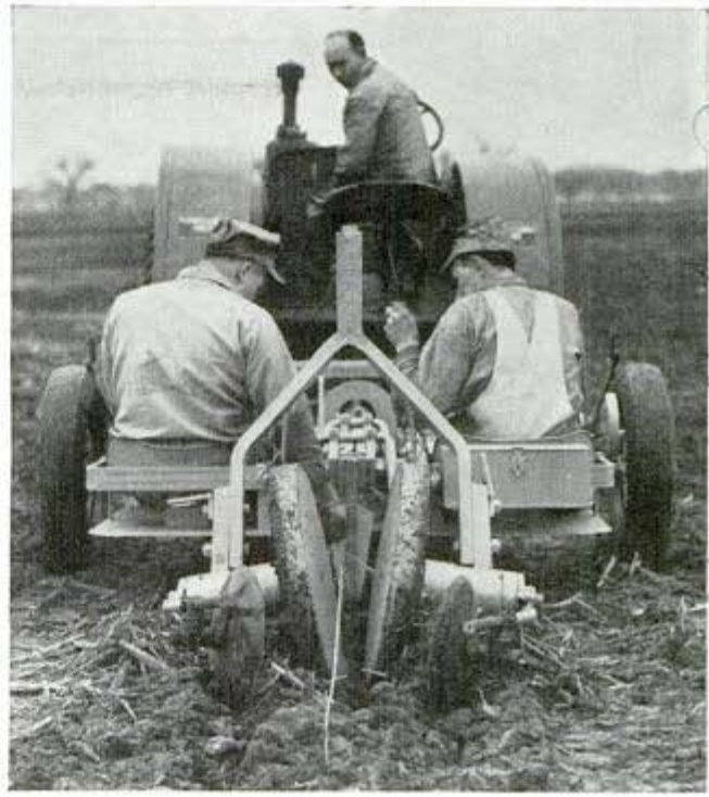
Two men seated at rear of planter alternately set trees in crevice opened by plow, after which packer wheels press soil
