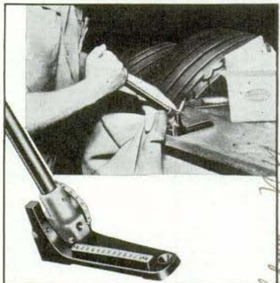
Fastened firmly to a bench, this valve-bending tool may be set for any angle required by auto wheel
