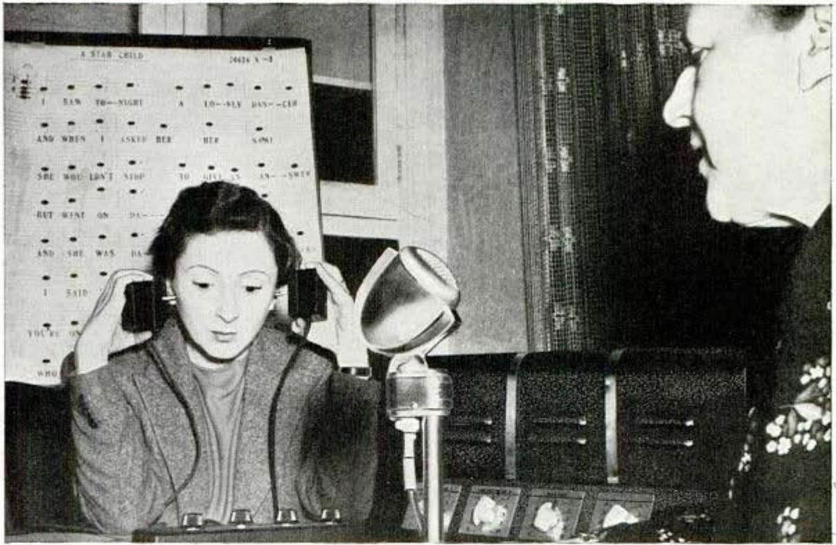
Above, two Phipps units applied to bones in front of ears help person almost totally deaf. Amplifier controls pitch and volume of sound from "mike" to unit
