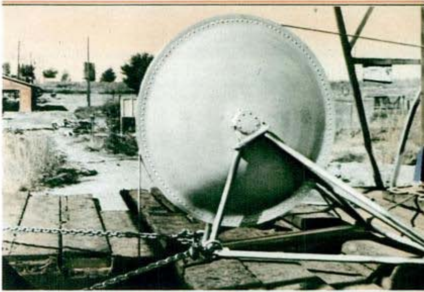
Above, wheel by which depth of gamma ray detector in well is measured. Below, part of modern refinery installation
