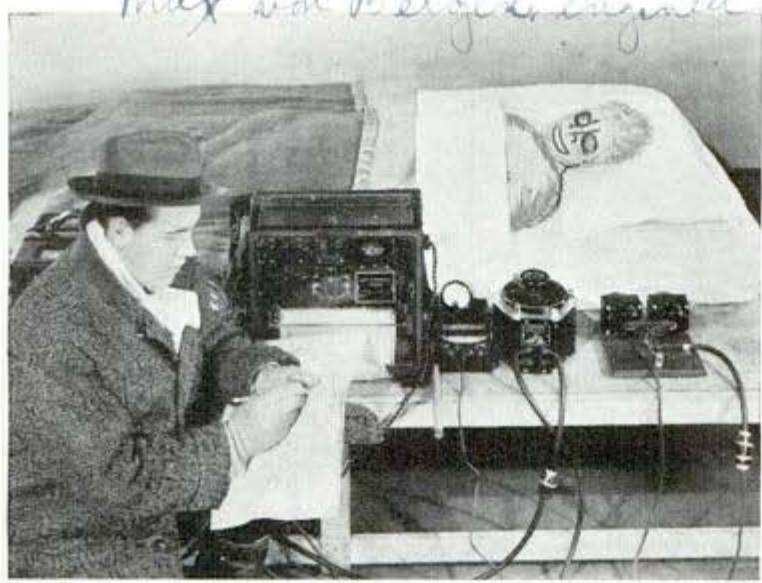
Engineer reading charts at bedside of Maggie the dummy in tests to determine how well the automatic blanket serves to keep the sleeper warm
