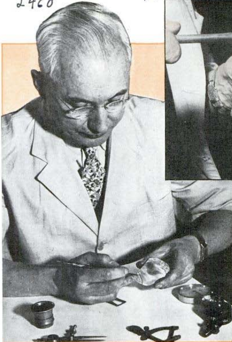
The Vargas with steel blade in place for tapping. If cutter is lucky, diamond splits along black lines which indicate grooves cut with another diamond
