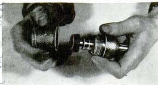
Assembling sandblast nozzle with break-off head
