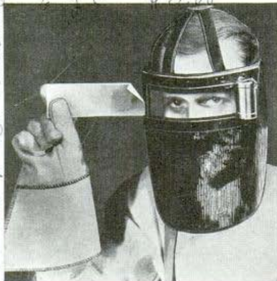
Vision is cleared quickly in helmet by tearing off soiled film, replacing it with fresh piece from roll
