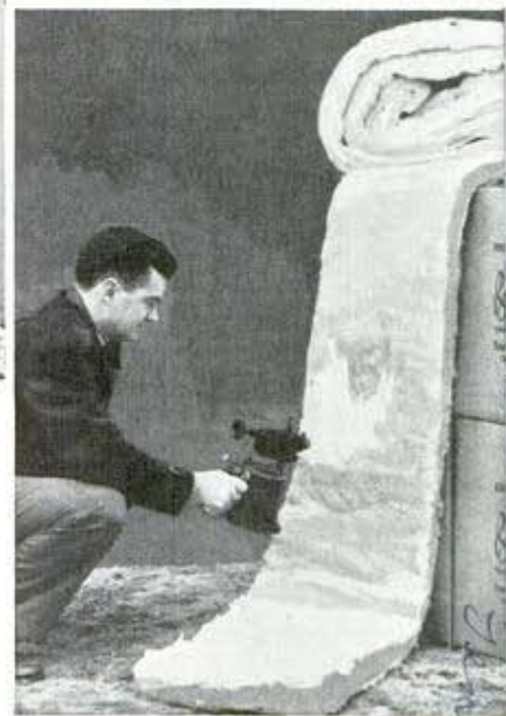
Torch-testing fire-resisting cotton insulation Photo courtesy Barnhardt Mfg. Co.
