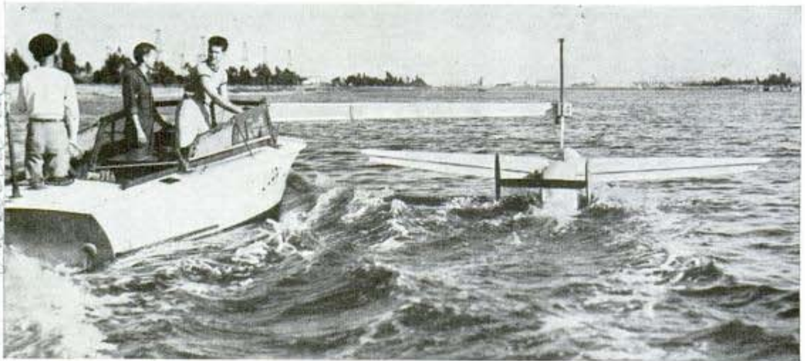
Attached at the side of speedboat by a long arm, this model seaplane is towed on water to correct faults of the big ship in taking off. Crew members take motion pictures of its action at various speeds
