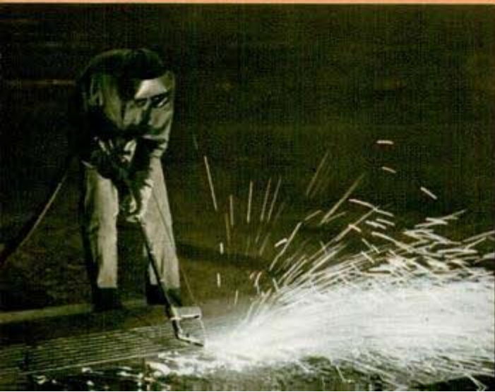
Below, workman in mask and protective clothing is shown performing another steel-mill operation known technically as "scarfing"
