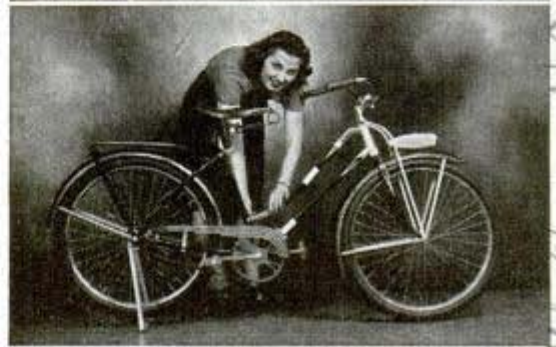
The man's bicycle, top, is converted for woman's use, below, by changing position of the detachable bar
