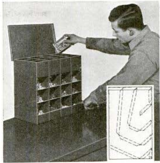
Bottom bin replenished by filling chute at back of case. Diagram shows arrangement of chutes and bins
