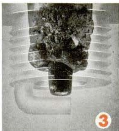
BLISTERED Oxide Coating Too late for cleaning
