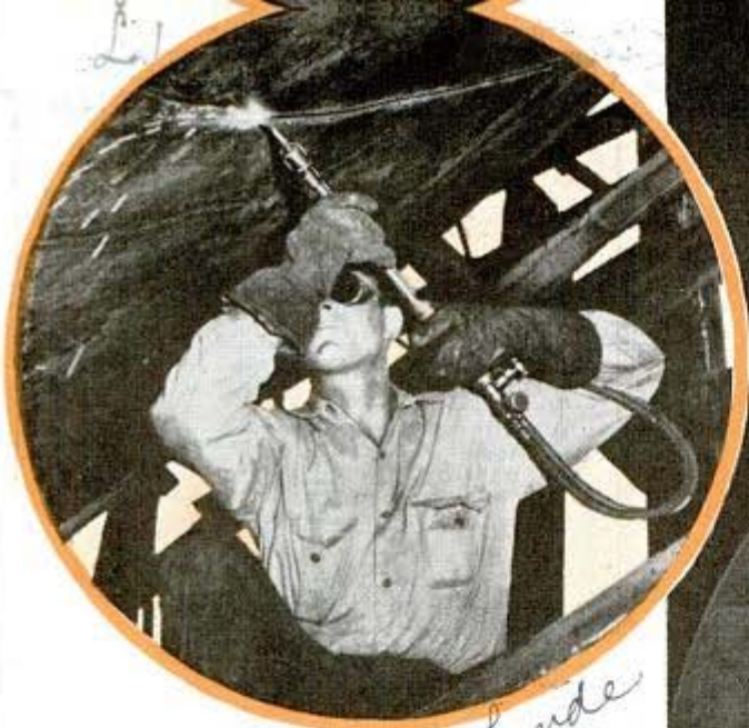
Circle, oxy-acetylene process called gouging removes narrow strip of metal from steel plate. Right, portable flame-cutting apparatus in use
