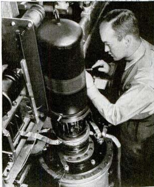
Left, power change switch at General Electric short-wave transmitters, South Schenectady, N. Y. Right, the 100-kilowatt transmitting tube of WGEO, western hemisphere's most powerful short-wave station, is cooled by a constant stream of water pumped through it. The delicate filaments are replaceable
