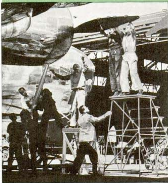
It takes four men to turn one propeller over by hand, so auxiliary engines start the main engines
