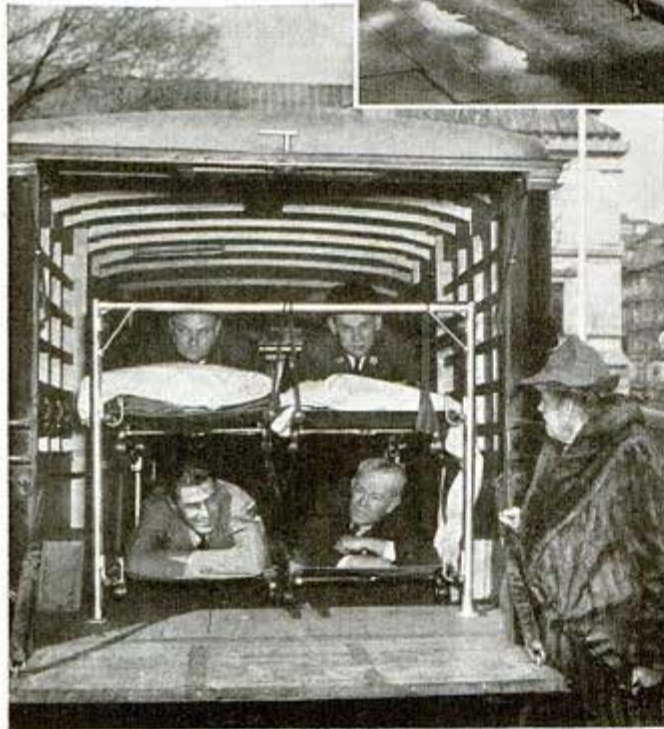
Lightweight metal frame designed to carry four stretchers, above, can be placed in a delivery truck, as shown at left, converting it into an ambulance when emergency may demand
