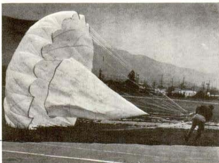
Inventor bracing himself as he ground-tests small-size parachute. Note cone in center which forces air into 'chute to decrease speed of descent
