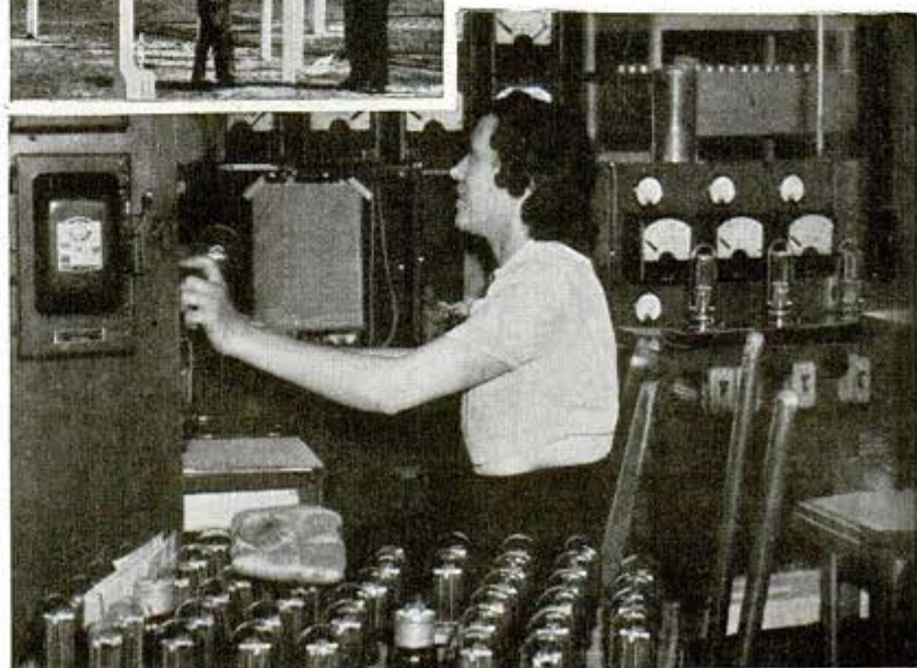
Below, testing characteristics of vacuum tubes in laboratory
