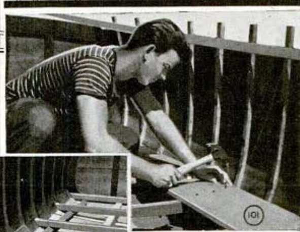
Except for the two center boards aft of the engine well, the flooring can be nailed to the timbers
