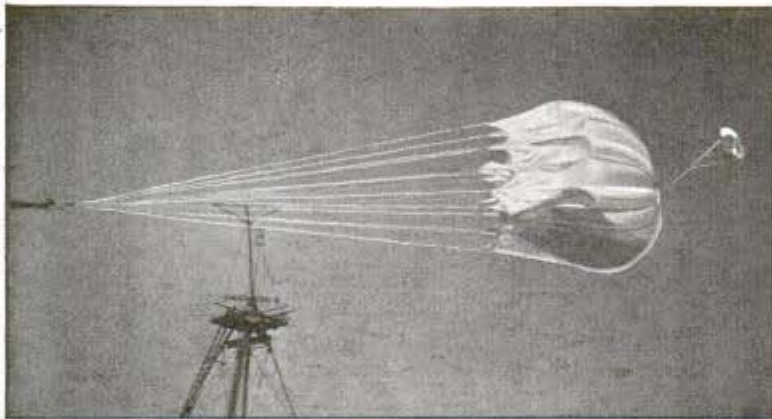
Above, a 'chute opening as it whirls around the Pioneer Parachute Company test tower
