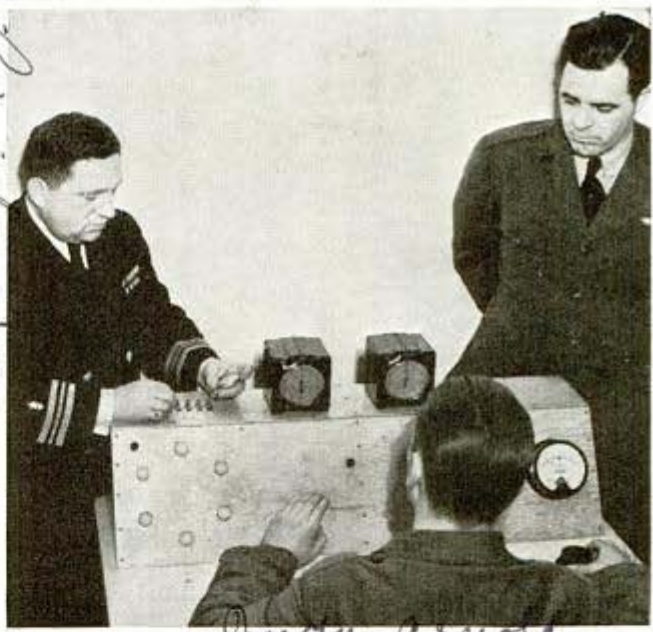
Meters register student's dexterity and speed as he turns out red and green lights and keeps needle in center of the dial
