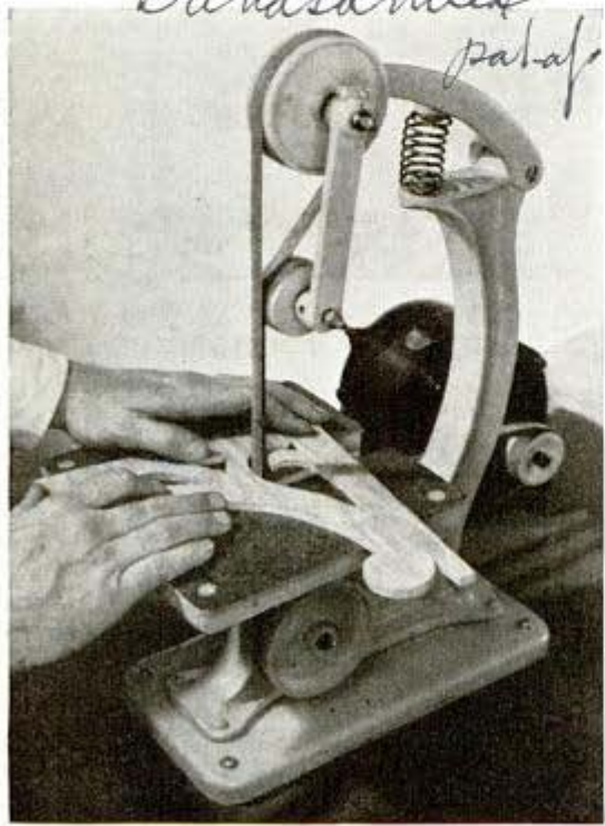
Note how sand belt is pressed together by idler wheel so it will operate on inside edge of scroll
