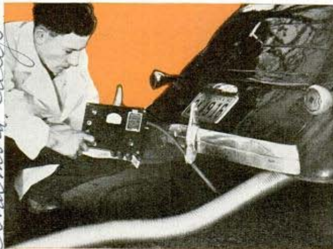
Exhaust-gas analyzer which aids in tuning carburetor to proper air-fuel mixture
