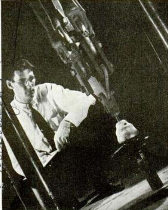
Two views show powerful pulling machine tugging at insulator coated with high-strength glass
