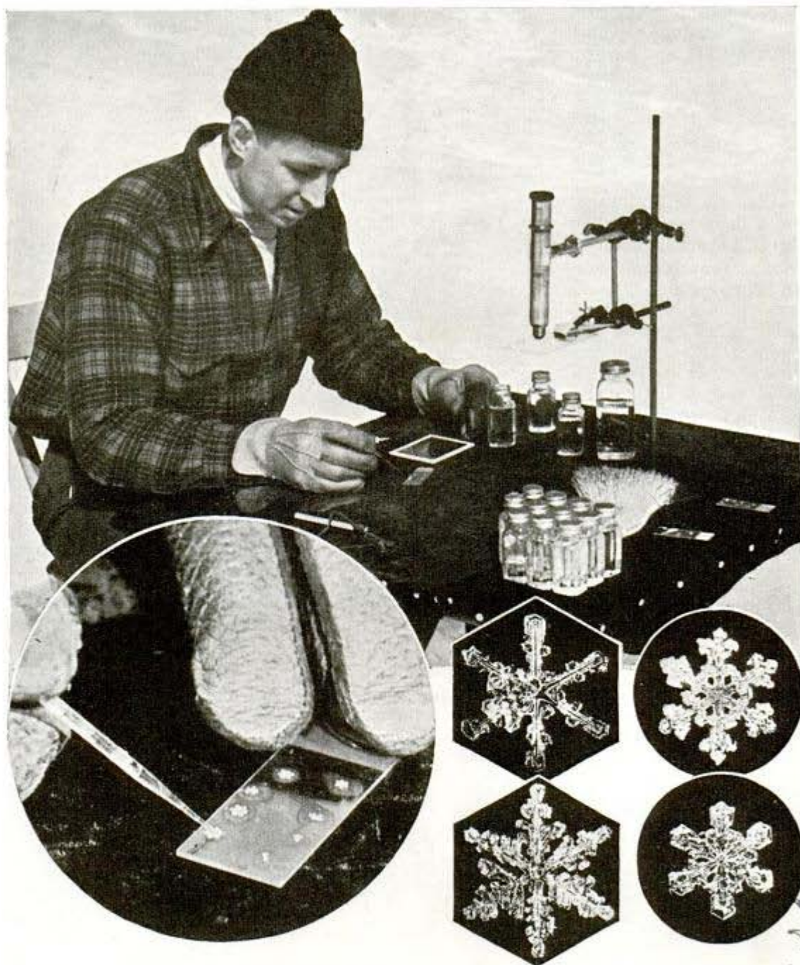
Top, Vincent J. Schaefer with his snowflake casting equipment; microscope is used only to pick out the flakes he likes. Bottom, left, making casts on a glass slide; right, enlarged photos of casts
