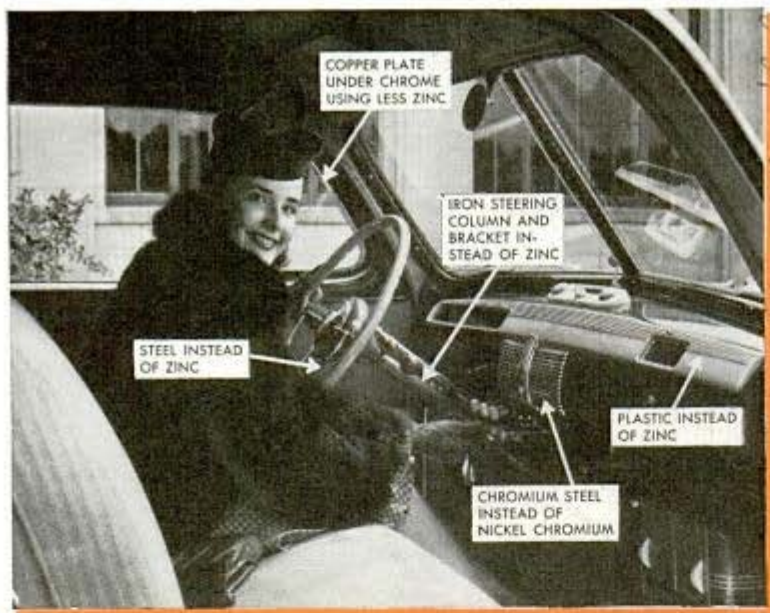
Substitutions which Ford engineers find possible to make in interior of automobile to release materials vital to national defense
