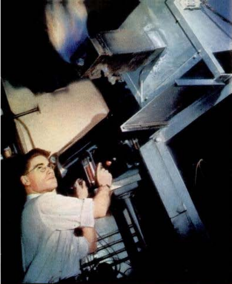
2151 Small Endogas generator in Westinghouse laboratory. Note flame shooting from its "mouth." Endogas is used in heat-treating parts made of steel
