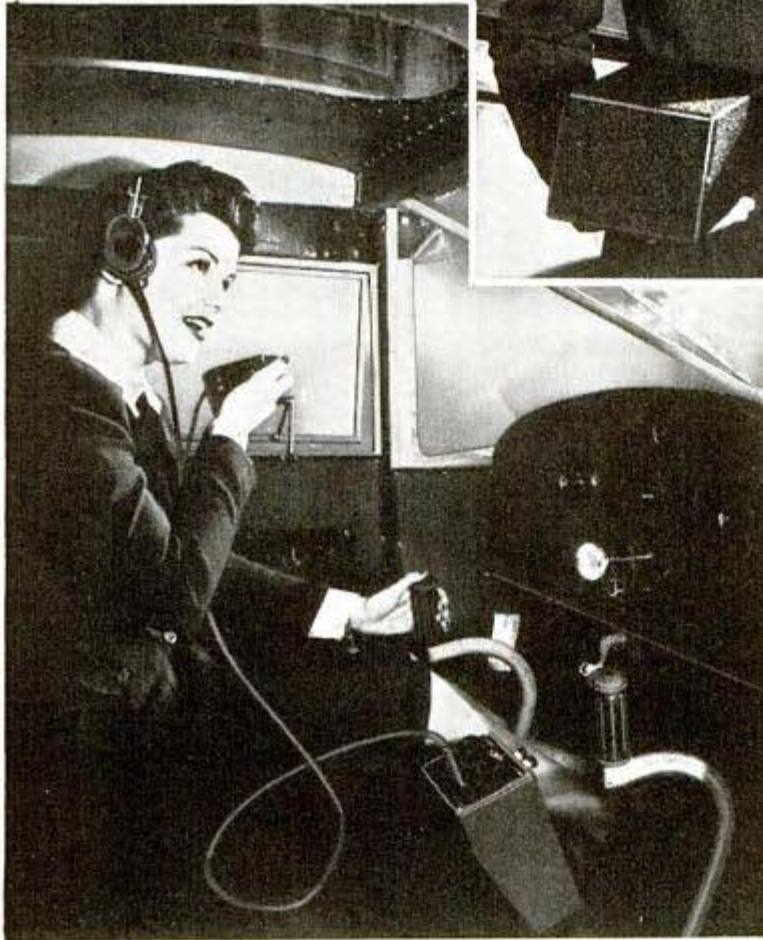
Two small handfuls—one case containing a two-way radio unit and another the batteries, etc.—weigh only 10\frac{1}{2} pounds, making compact radio communication system for lightplane
