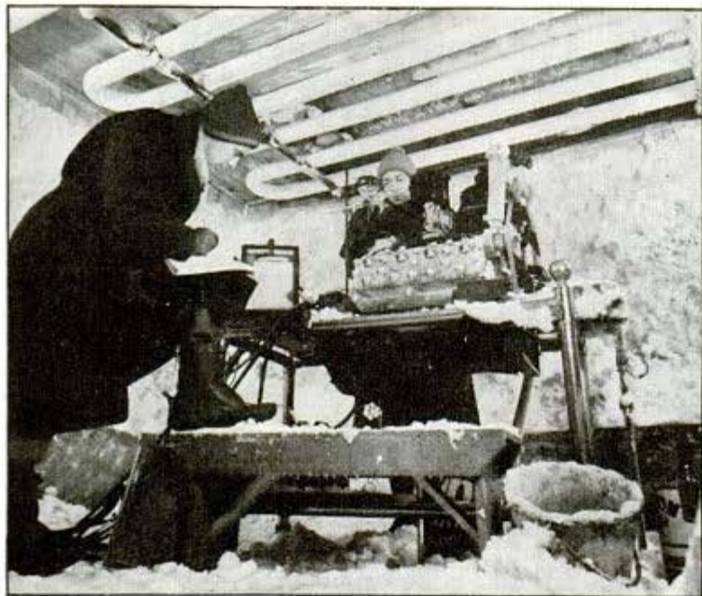
Cold laboratory for studying performance of oils and gasolines under winter conditions. Note heavy clothing workers must wear
