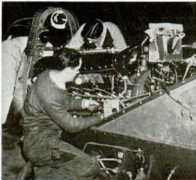
Above, servicing the big 12-cylinder, 1,150 horsepower Allison engine
