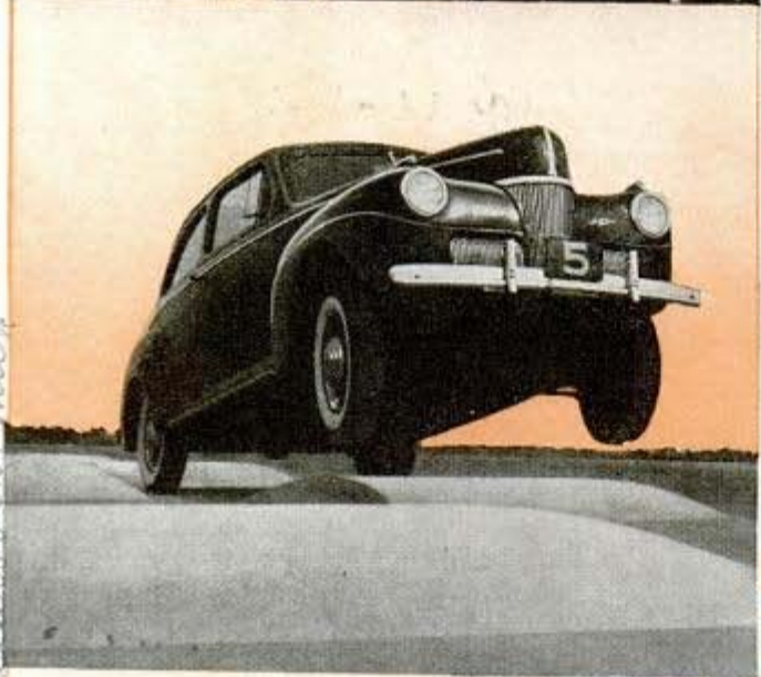
Above, car "waltzing" over "wobble road" at Ford test track. The section consists of double line of staggered concrete mounds over which cars weave, twist and leap at 30 miles per hour. Right, examining "fifth wheel" that records speed. The wheel is attached to a car undergoing tests at the General Motors proving ground
