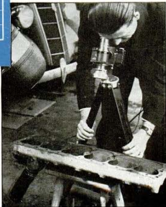
Photographing carbon deposits in combustion chamber as part of research on pre-ignition
