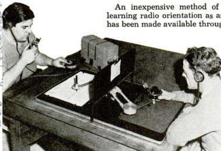
Orientator reproduces signals used in "blind" flying for teaching pilots
