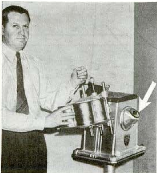
Conditioner for mixing paint in the can may be set to run for any length of time up to fifteen minutes
