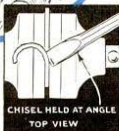
Heavy sheet metal is sheared by clamping it in a vise so line to be cut is flush with the jaws, and using a flat chisel held at an angle to the work
