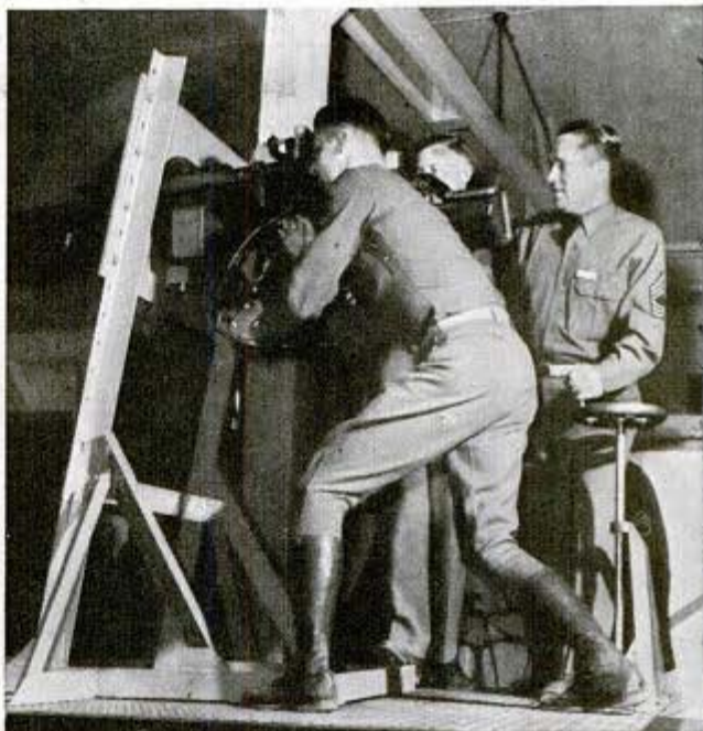
To make gunnery practice with a 37-millimeter tank gun realistic, (above) it is mounted on a rocking foundation
