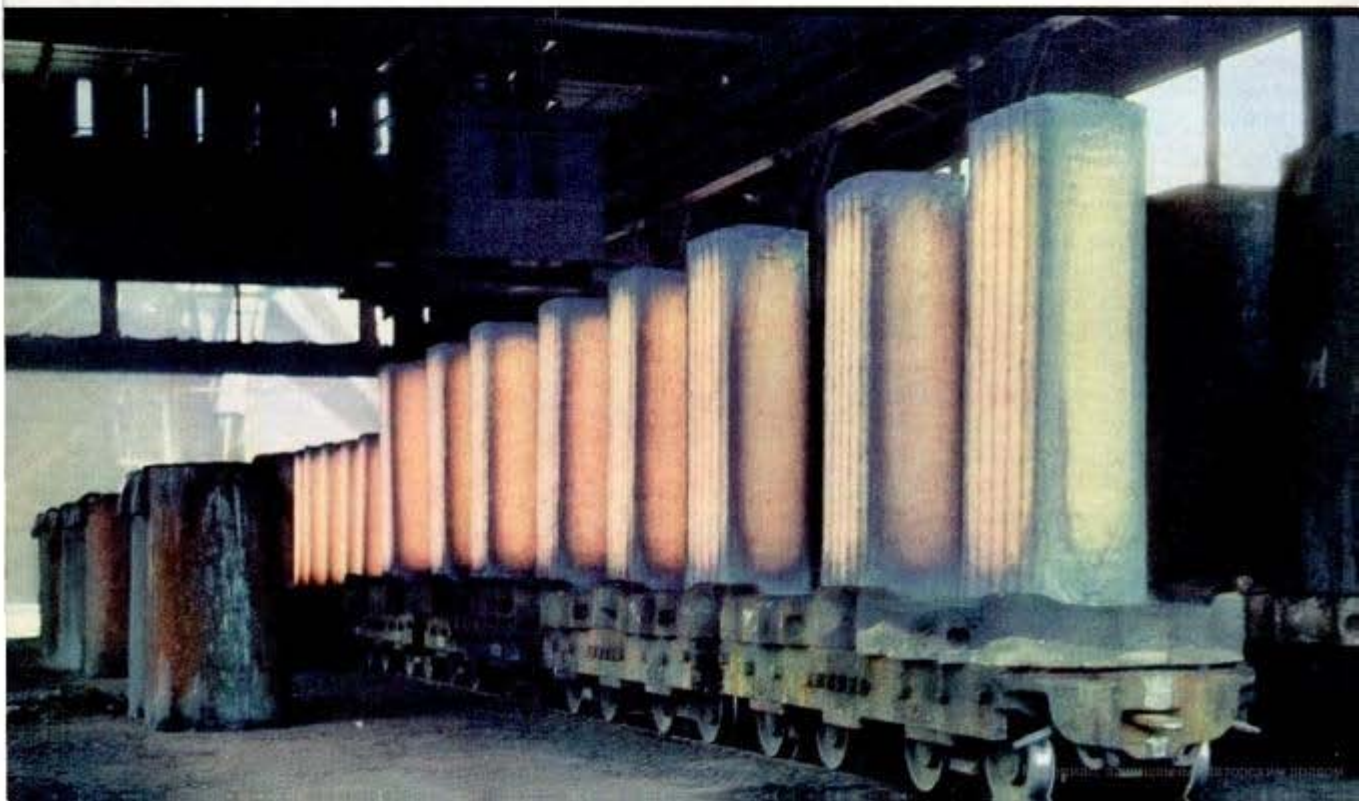
Below, still glowing after being stripped of their molds, these hot ingots are on way to the soaking pits. This is a natural-color photograph
