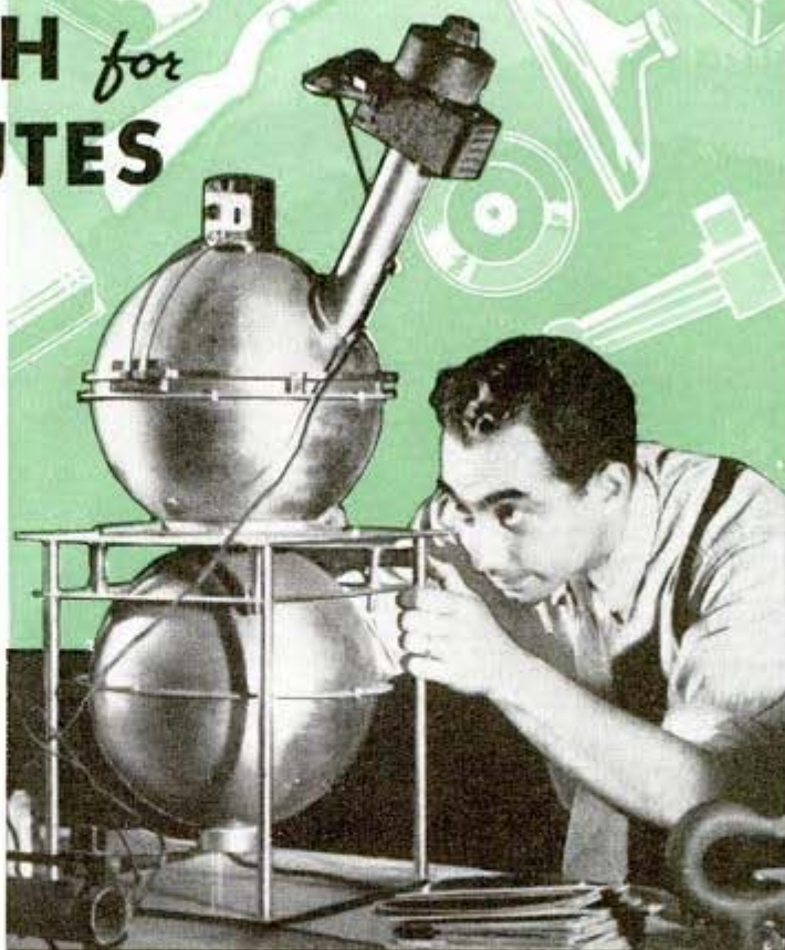
Above, reflectometer in General Electric laboratory tests plastics which are in demand as substitutes for defense materials
