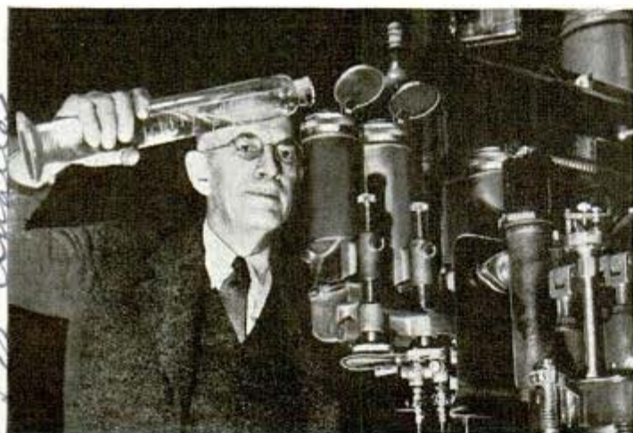
Pouring sample of blended fuel in knock engine to test its detonation qualities before using in racing car
