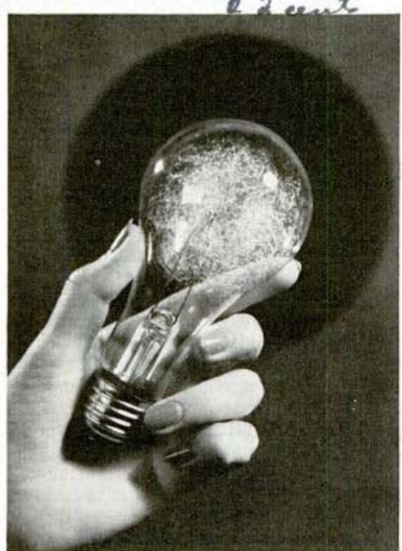
Foil is finely shredded in this new photoflash lamp in order to produce a light of greater intensity
