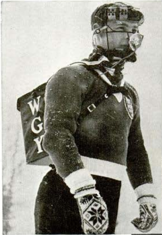
Skier poised for takeoff, above, is wired for sound with short-wave radio transmitter strapped to his back and microphone on wire mask
