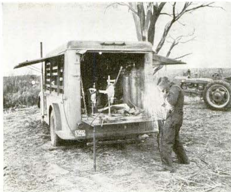
Welder working at bench made by lowering tailgate behind mobile shop
