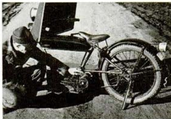
Battery-operated motorcycle runs 30 miles per hour
