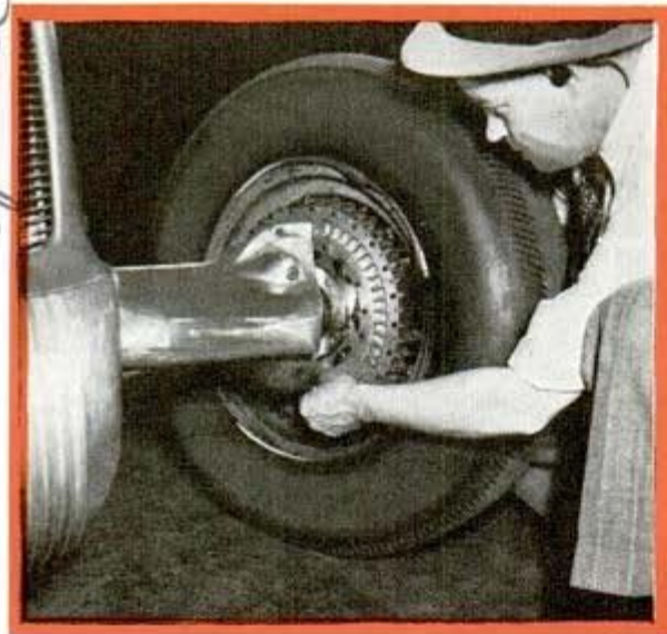
View of special brake that has only two moving parts, reducing chance of failure
