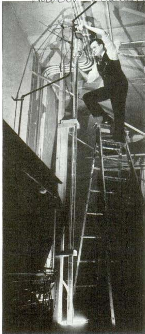
Inside the tall glass tube is another containing a gaseous element whose atoms are to be sorted
