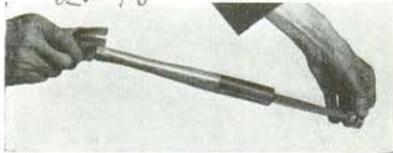
File pulled out from hammer handle is ready for use. Cap at end is turned when you want to push it back
