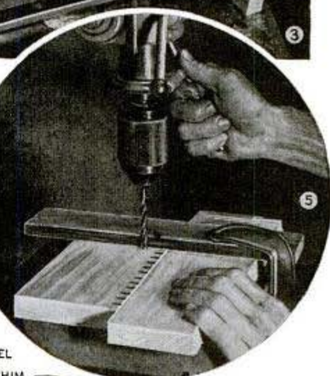
Special care should be taken in spacing the holes in the guide as shown in Fig. 5
