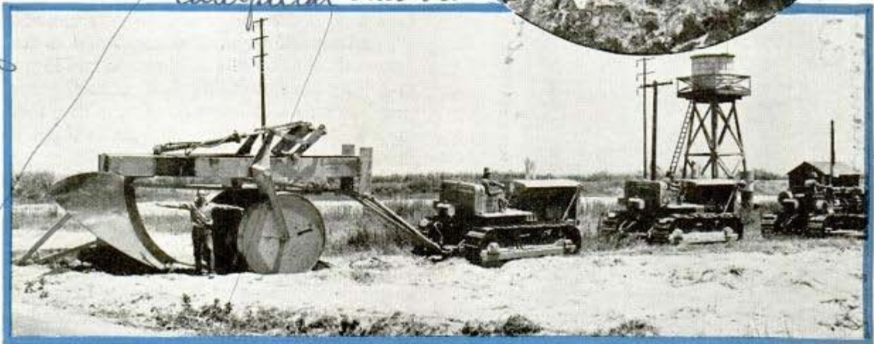
Below, huge six-foot plow built to bring up rich peat soil buried in flood sands
