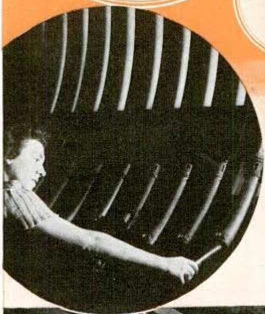
Rhythm of machines, clash of steel and humming of motors play a symphony of industry as America's factories turn to defense. Above, like an organ console are De-ion arc extinguishers, which perform job formerly done by fuses
