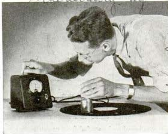
Measuring the thickness of a sheet of steel, with the magnetic cylindrical gauge head held on the sheet
