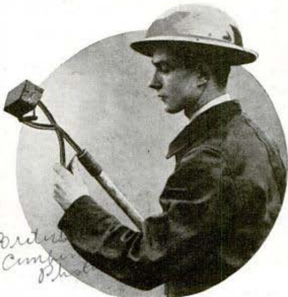
Fireman shows how the claw grips incendiary bombs
