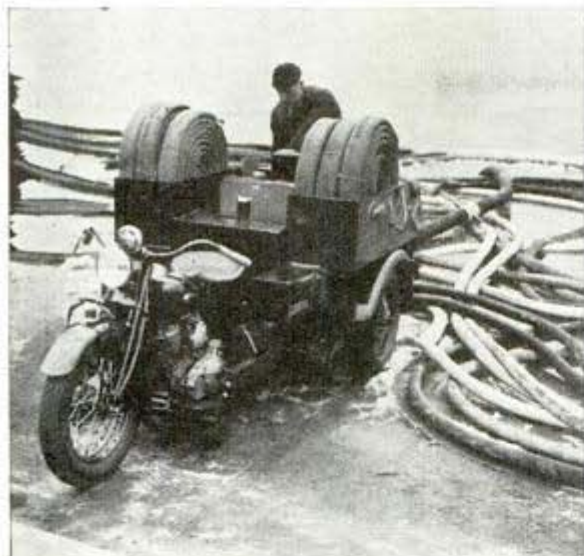
Motorcycle pumper at left, equipped with a V-8 engine, feeds 500 gallons of water per minute into hose lines. At right, Boston fire fighters man a line of nozzles in a test of small trailer and motorcycle pumps
