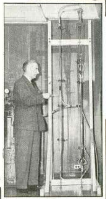
Laboratory on wheels is used to analyze drilling mud for signs of oil
