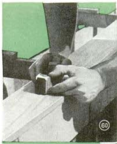
Planks to be installed on extreme curves first must be cut slightly concave on the inside before they are steamed
