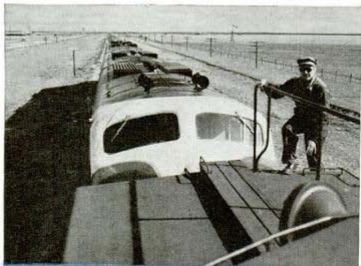
Through louvres on roof of locomotive, above, heat from electric brake is dissipated
