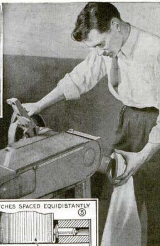
A wooden ring fitted with three catches as in Figs. 2 and 3, and tacked in the mouth of the dust bag of a sander makes the bag easy to remove or replace
