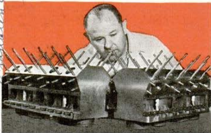
Fred Offenhauser finishing the two blocks of new V-8 supercharged engine to be used in this year's race. Below, view of Indianapolis Speedway with racing cars passing stands at high speed
