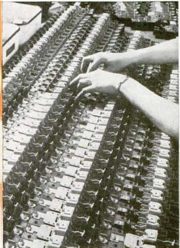
Rhythm of machines, clash of steel and humming of motors play a symphony of industry as America's factories turn to defense. Above, like an organ console are De-ion arc extinguishers, which perform job formerly done by fuses
