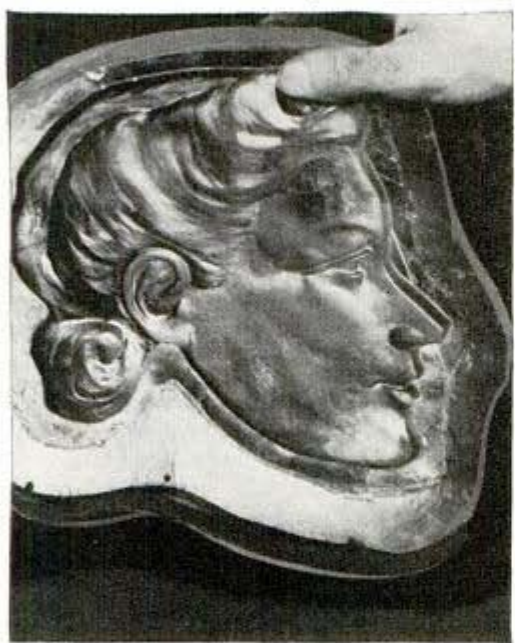
Above, lead mold of head, first carved out of wood, is good for thousands of plastic copies
