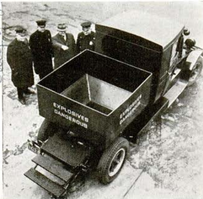
If bomb being transported in this truck explodes accidentally, its force will travel upward with little chance of doing harm
