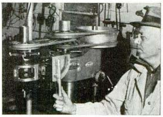
Lever is moved back and forth to change speed
