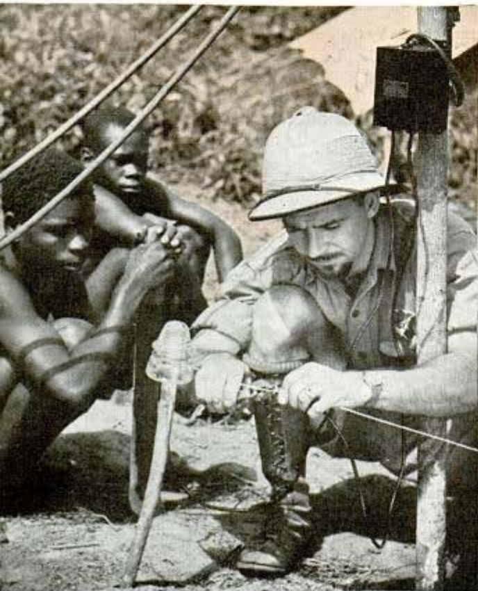
The transformer steps up the charge in this single wire encircling the camp to 4,500 volts as a discouragement to wild animals prowling around at night
