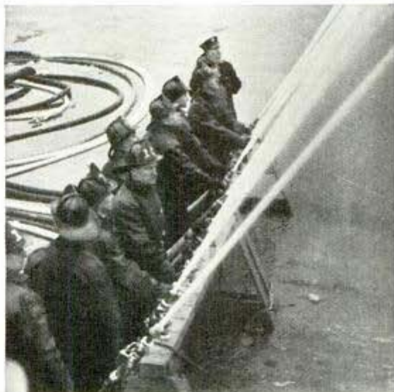
Motorcycle pumper at left, equipped with a V-8 engine, feeds 500 gallons of water per minute into hose lines. At right, Boston fire fighters man a line of nozzles in a test of small trailer and motorcycle pumps
