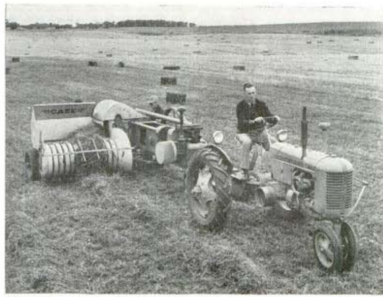
Baler picks up hay left in field and packs it into bundles made up like slices of bread so it may be pulled apart easily when the wire is cut
