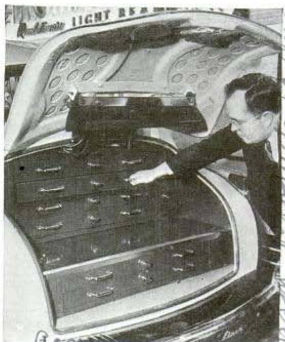
Large chest built into trunk compartment of salesman's auto contains drawers to hold samples
