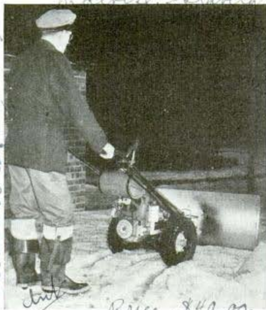
Price - $40.00. Operator simply guides this snowplow, since a one-cylinder engine supplies the power to push it
