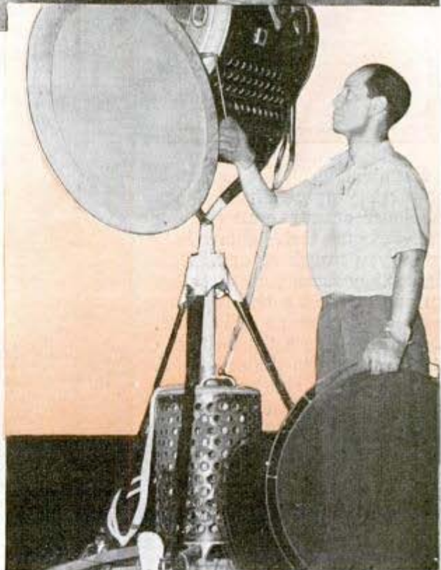
Above, a "juicer" trains his lamp down on floor set of "Tin Pan Alley." At right, a "scrim" in front of light reduces its intensity
