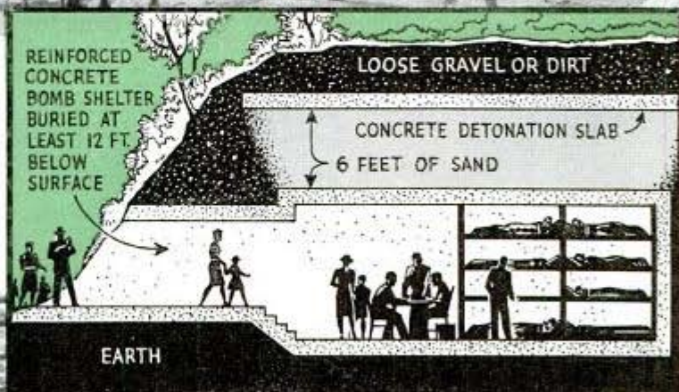
Above, Coast Artillery headquarters during practice firing. Right, sketch of typical underground shelter. Bottom, part of fire alarm, emergency phone and code network that operates on batteries
