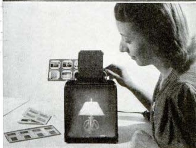
At the top the projector throws the image on a wall screen; below, the opposite end of the instrument is used as a viewer
