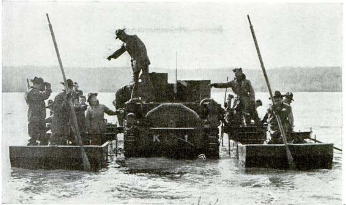
Army engineers ferrying medium tank across river. The ponderous machine is lashed to a couple of flat-bottom boats which serve as pontoons, and men in the boats use oars to help guide and propel it
