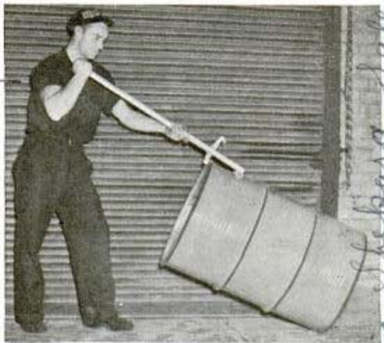
Pronged collar takes a firm hold on edge of barrel and the long handle makes the lift easy
