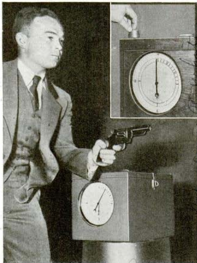
As the finger is withdrawn from contact button (see inset), timer begins operating and continues until bullet clips target
