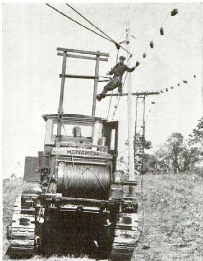
Outdoor laboratory crew hanging bricks on telephone wires in test to ascertain amount of ice the lines can endure in storm
