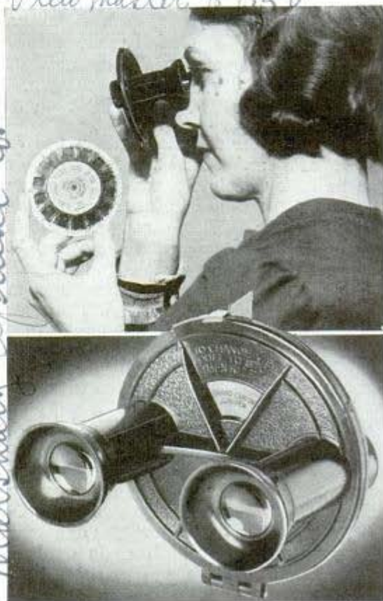
Disk of seven pictures, top, loads into stereoscope. Bottom, lever at top edge turns disk to change scene
