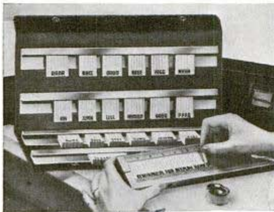
At left, laying out a sign in the adjustable holder with type faces taken from blocks of letters
