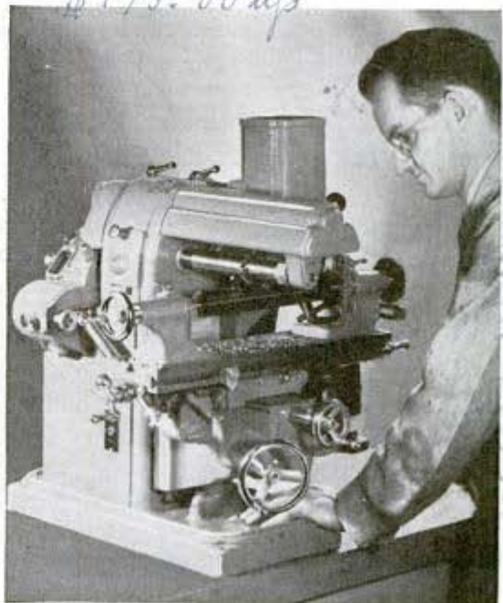
Baby-size miller relieves big machine of small jobs
