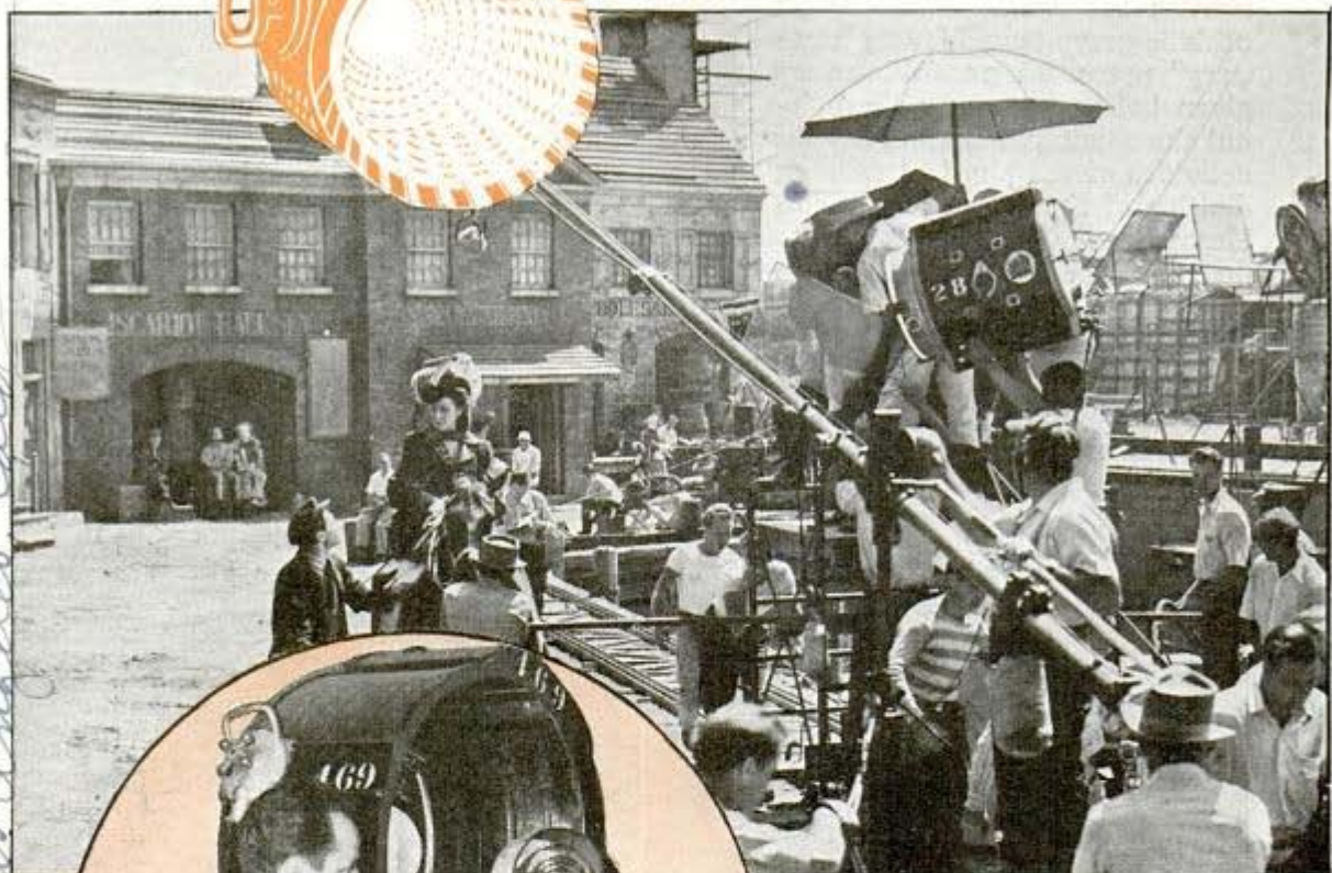
Arc lights (above) reduce shadows on faces in scene from "Chad Hanna." Left, placing "spill ring" to break up beam of large incandescent lamp. Below, arranging stage lights for portrait
