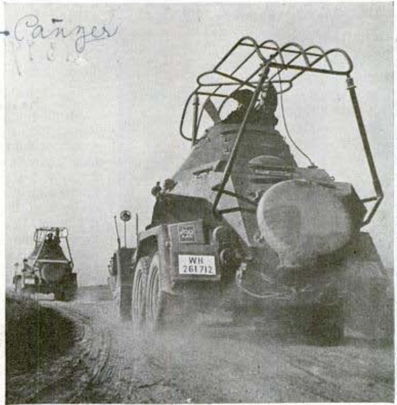
Aerials mounted on these German scout cars, built of extra heavy metal rods to withstand the rigors of war, are essential in keeping contact with other units of tank division that follow
