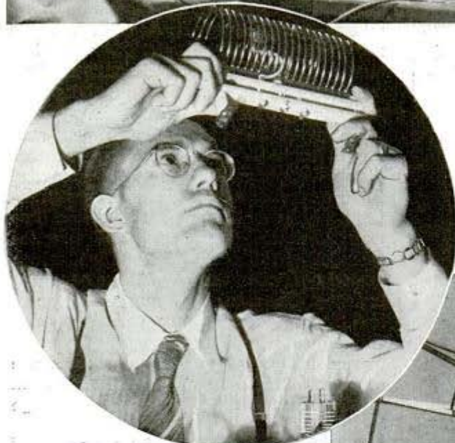
Top, amateur operator at station controls. Center, plug-in frequency coils used to change station's transmission wave length. Bottom, rotatable beam antenna
