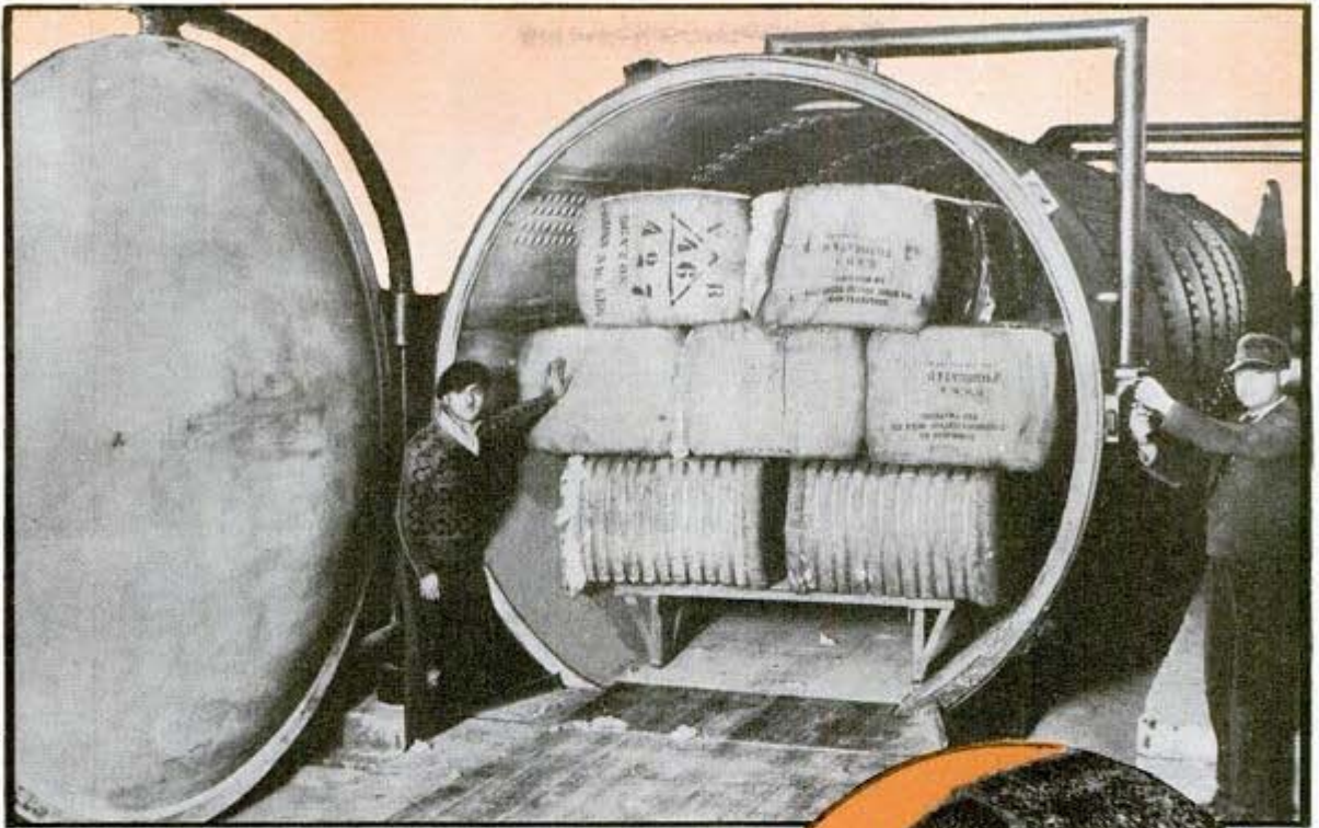
Above, fumigating cotton at San Francisco. Right, magnified view of white fringed beetle, an alien newcomer which destroyed up to thirty per cent of the potato crop in certain parts of Mississippi recently. Bottom, operating controls of fumigating chamber
