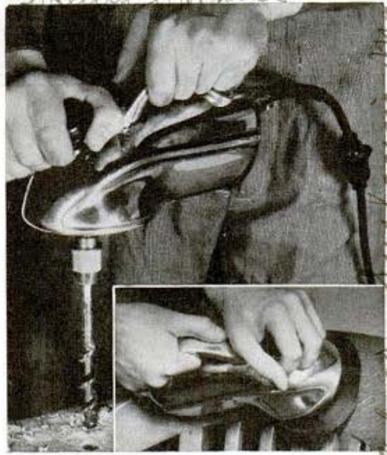
Upper picture shows the tool used as a drill; below, its flexible disk sands a curved surface
