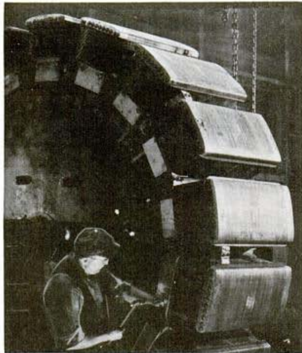
Assembling rotor on medium-size vertical waterwheel generator in the Westinghouse East Pittsburgh works
