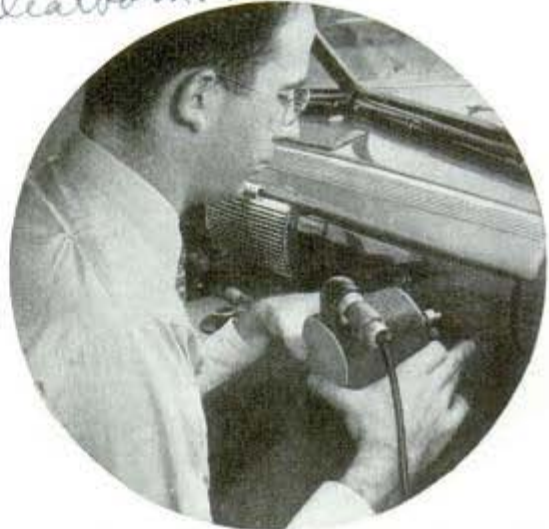
By pressing this instrument against panel of auto, expert traces noise-making vibration to its source
