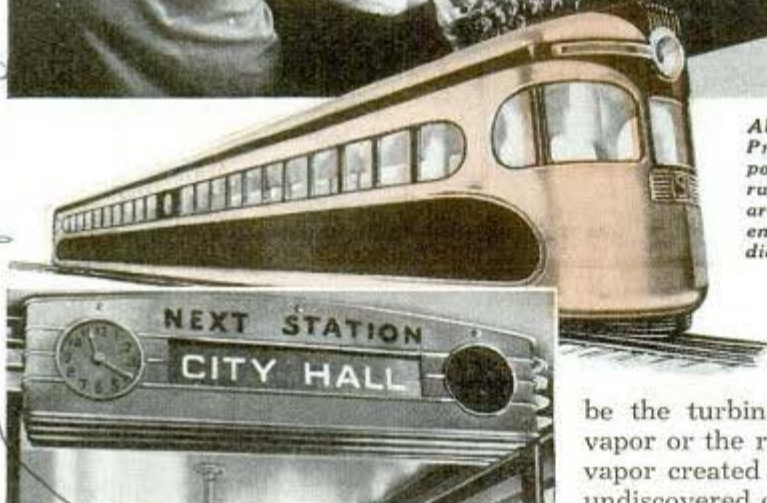
Station stops in Philadelphia's subway coaches are announced by automatic electrical device
