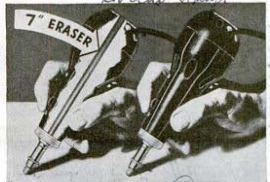
Cutaway view of machine, at right, illustrates hollow shaft through center that houses seven-inch eraser. As rubber wears down, the core may be extended until it is all used up
