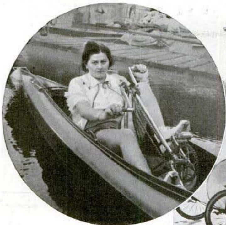
Both Germany and England are exerting themselves to conserve precious gasoline, and wherever human muscles can do a job they are doing it. Witness, above, the pleasure boat that made its debut recently at Berlin. It has a propeller with chain and sprocket drive calling on arm and leg power; not so romantic as paddling a canoe, but it gets places. At upper right a Londoner pedals to work in a "Velocar," of French origin. In the two-seater model both driver and passenger provide the motive power of the toylike car
