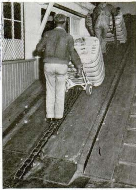
Taking it easy up a twenty-degree incline, men let Link-Belt conveyor chain haul load and themselves
