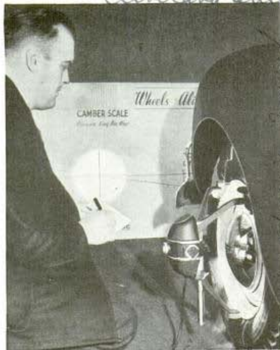
Testing wheel alignments of the entire car is a task of a few minutes with this three-lens beam system
