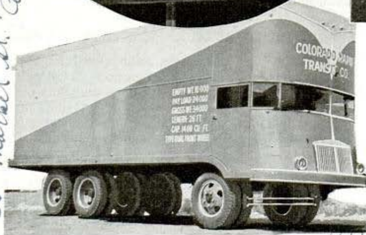
At left is the twelve-wheel truck, with a cargo capacity of twelve tons. Notice its roomy cab (top); beneath it is the engine, and above it a large space for freight. Closeup of the dual front wheels, above, shows the overhead cylinder which houses a coil spring providing a smooth ride
