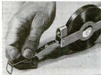
Bulb in "nose" of tapeline reel lights up figures, making them easy to read in dark
