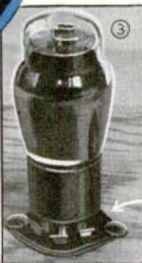
(2) Paper dial marker cemented to panel. (3) Wafer-type sockets mounted up-side-down with thumb tacks on plywood for temporary hookups
