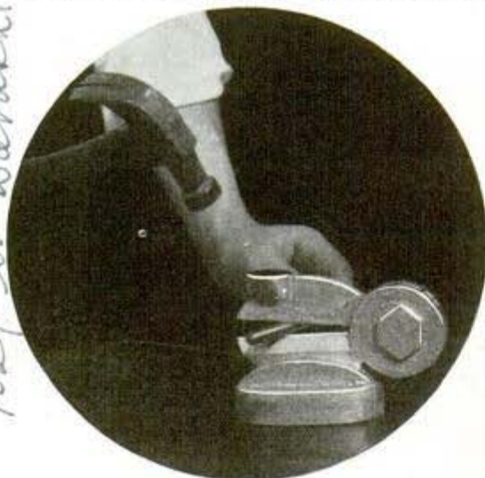
Cutting a bolt with the hammer-operated shears, which will bite through a half inch or more of metal
