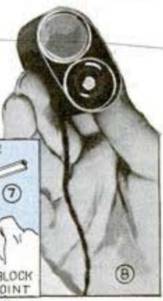
(8) Flashlight cells, now commonly used in pocket-type receivers and testing equipment, may be taped together in compact A or B-battery units. Cells should be arranged for polarity as shown to permit use of short soldered leads for series connections. (9) Inexpensive lead-in insulator assembly made from porcelain tube, stand-off insulators and a "Pyrex" custard cup on external side. To drill custard cup for the threaded brass rod, place cup on a block of soft wood and pour in a little turpentine. Use 1/4-in. drill, or preferably a piece of 3-cornered file
