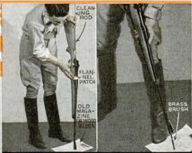
A SWAB THE BORE WITH NITRO SOLVENT ON PATCH B RUN A BRASS BRUSH THROUGH BORE THREE TIMES
