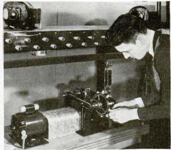
Center, left, rotary shock tester which revolves electric lamps around their own axis and around periphery of large drum. Thirty-six times a minute the forty-five pound drum drops a short distance to simulate service on vibrating machinery. Right, rough-riding merry-go-round for tiny lamps produces vibrations similar to shocks if lamps were used on automobile instrument panel. Bottom, boxlike drum treats lamps roughly, some of them being subjected to equivalent of bouncing down 400 steps varying six to fifteen inches each in height. This "torture" reveals strength of globes, bases, filament, lead and support wires and all other parts
