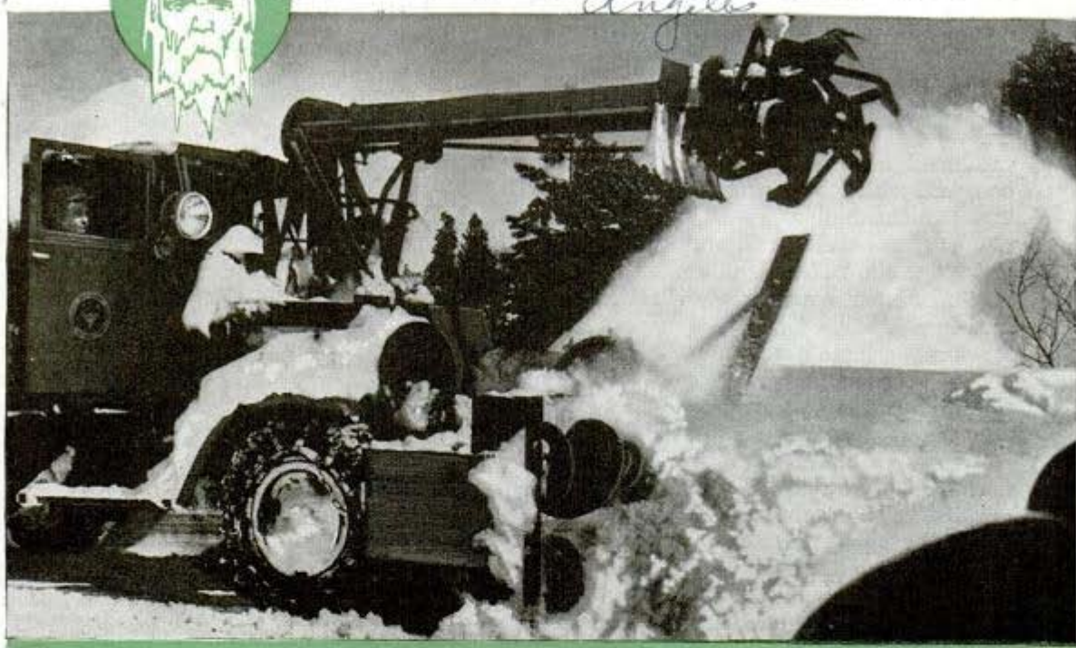
Boring into a snowdrift on one of California's mountain highways, this huge combination rotary plow has a special revolving claw attachment for reducing snowbanks
