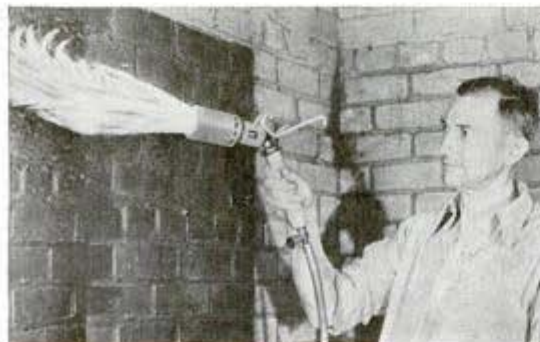
With this torch a two-foot flame is available for crisping paint on brick wall or other uses in shop
