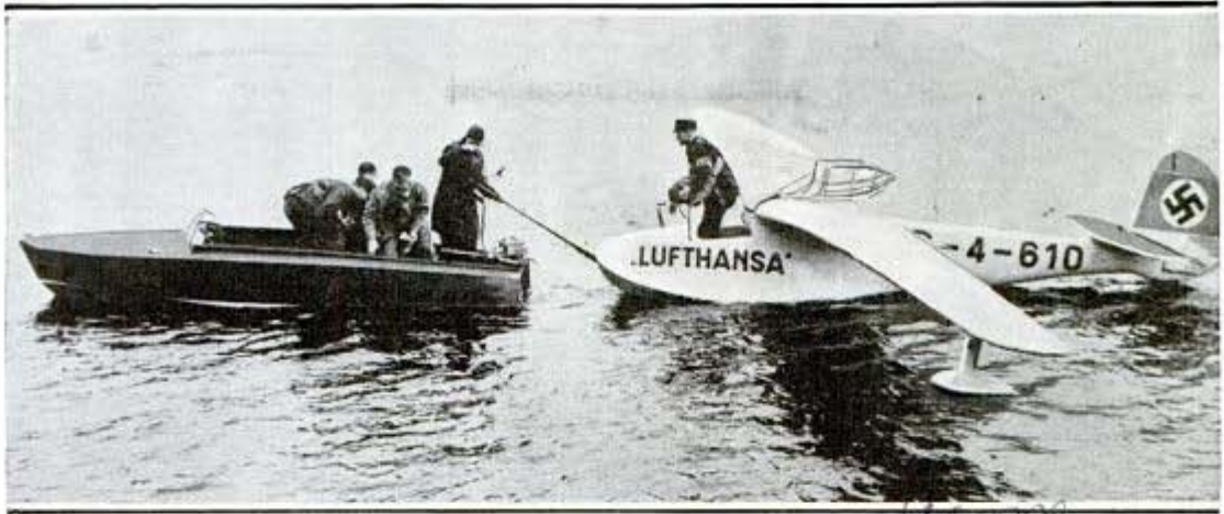
Towed at a speed of fifty to fifty-six miles an hour, this amphibian glider, built at Berlin, can take off either from land or water. The craft has a wingspread of fifty-nine feet and weighs 375 pounds
