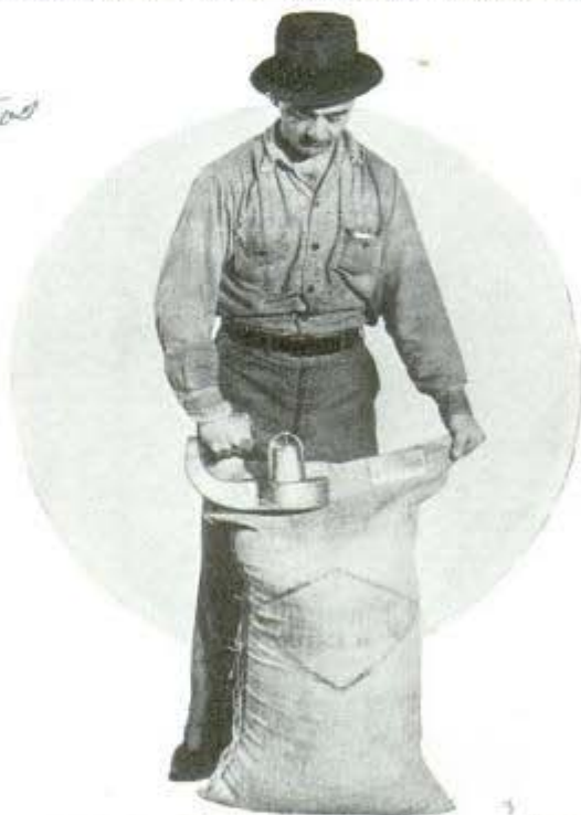
Notice the label that has been applied automatically as sewing machine was drawn across top of bag
