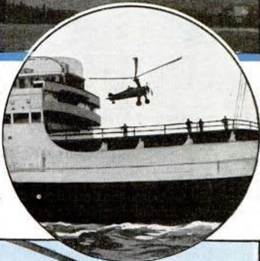
Top, helicopter hovering while bag is removed from basket by man standing on the ground. Circle, giro may operate easily from ship since it may ascend or descend almost vertically. Bottom, Kellett autogiro being used by the U. S. Army
