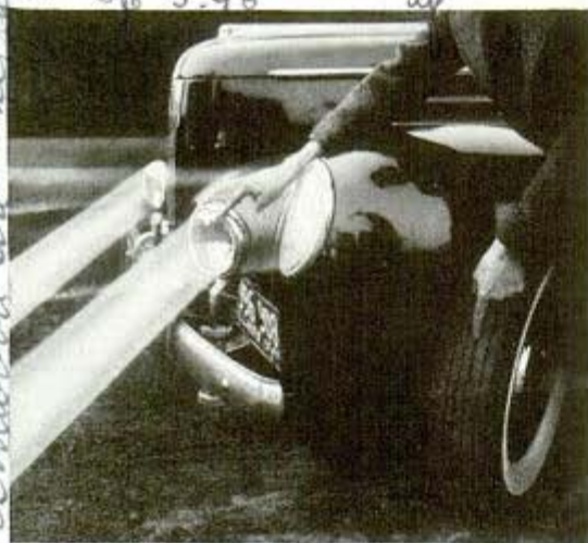
These automobile road-lights, mounted on special brackets, turn in same direction wheels are turned
