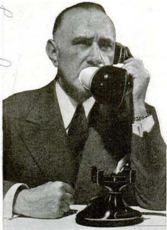
You can't hear the words spoken into this "silent" mouthpiece unless you are at the other end of line
