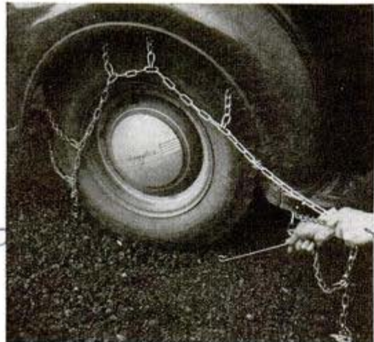
Rod held in the right hand is poked under car, behind the tire, to connect with other end of chain
