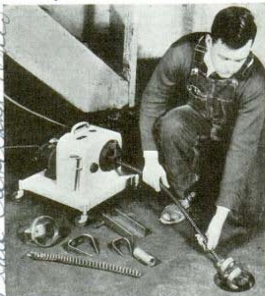
Electric drain-cleaning tool spins cutters capable of slashing opening through pipe clogged by roots
