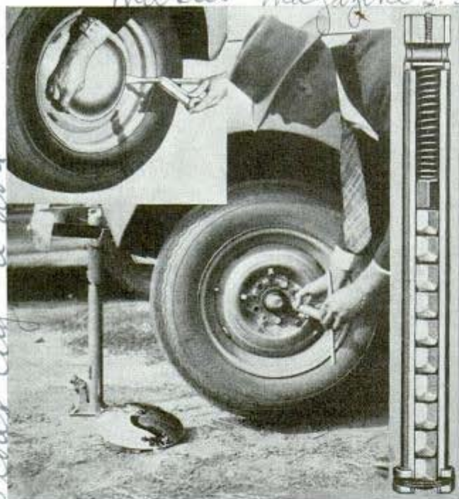
Auto wheel wrench retains lugs in magazine (see inset, right) as they are removed. Upper left, handle loosens hub cap
