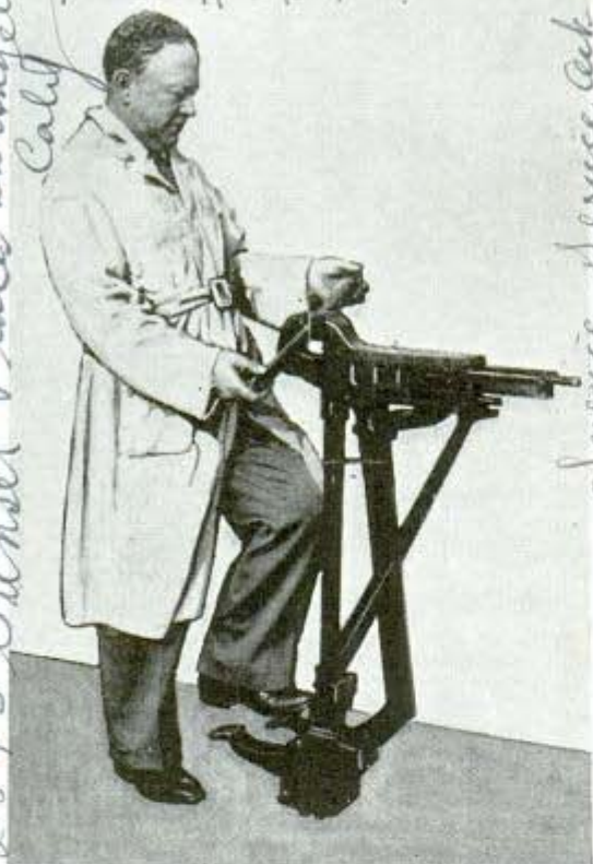
With one foot applying pressure on the pedal, the operator has both hands free to hold work in vise
