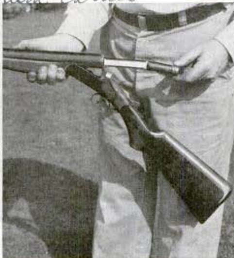
Charge of powder insecticide, left, spreads over wide area when fired from shotgun. Right, reloading with cartridge and paper "projectile"
