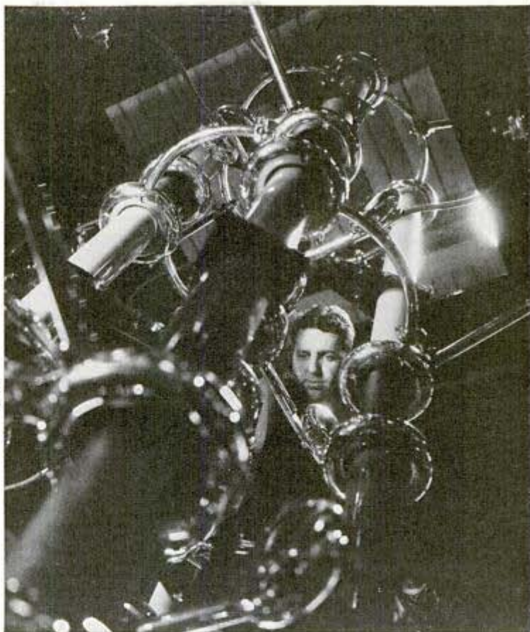
This "skyscraper" of capacitors reproduces the action of a thunder cloud in storing up electric charges and releasing them as lightning
