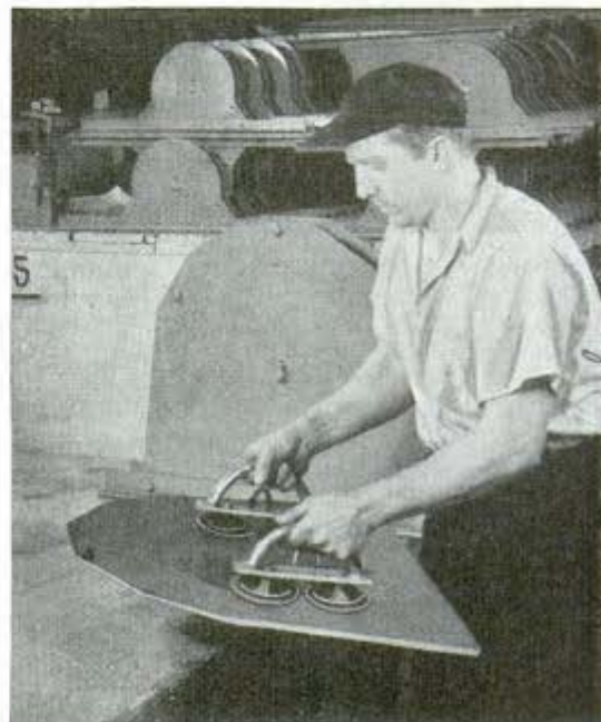
Two suction-cup lifters provide carrying handles for heavy flat sheets of metal or plate glass
