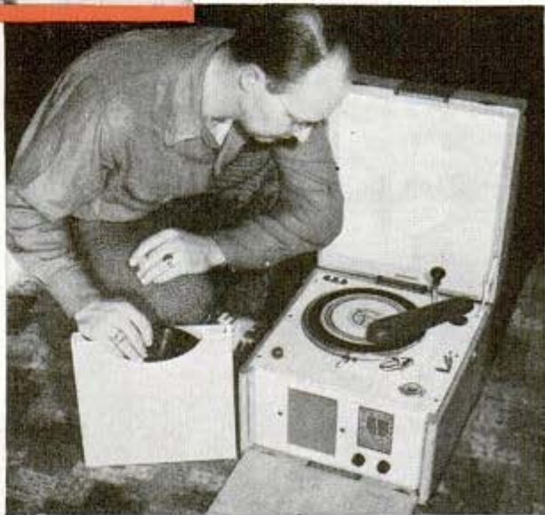
One of the lightweight portable instruments which incorporates a radio and a phonograph. Some portables are to be plugged into an electric outlet, others house batteries for operating the radio, and the phonograph is hand-wound
