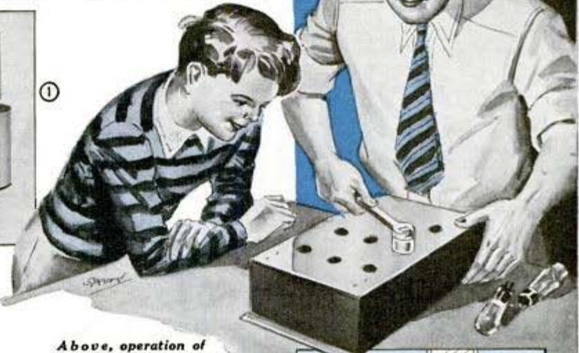
Above, operation of tool is simple matter of drilling a small hole for the cap screw and then using an ordinary wrench
