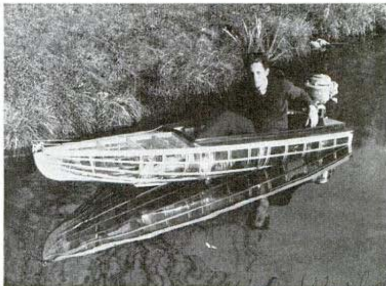
This boat is made of transparent plastic material so strong that ribless plastic boats, which would be practically invisible, are predicted
