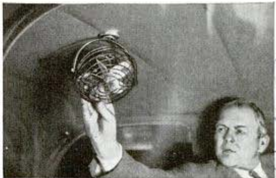
Fan in auto ceiling can be tilted in any direction
