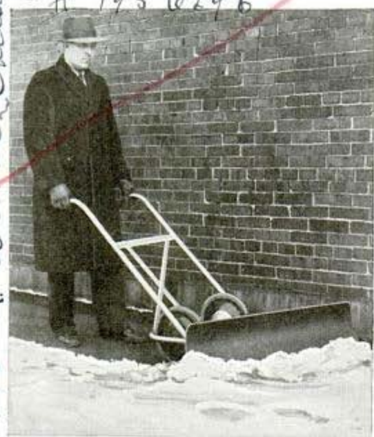
Plow built like hand truck saves labor in pushing snow off sidewalk; wheels help in moving it about
