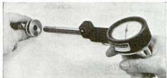
Inside diameters are measured quickly by releasing trigger after inserting gauge into the hole or tube
