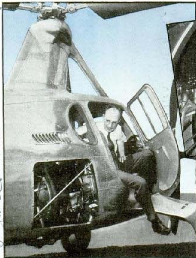
Left, Harold F. Pitcairn points out motor location in new-type autogiro that rises vertically (see photo at bottom) before starting forward motion. Above, instrument board of Kellett autogiro
