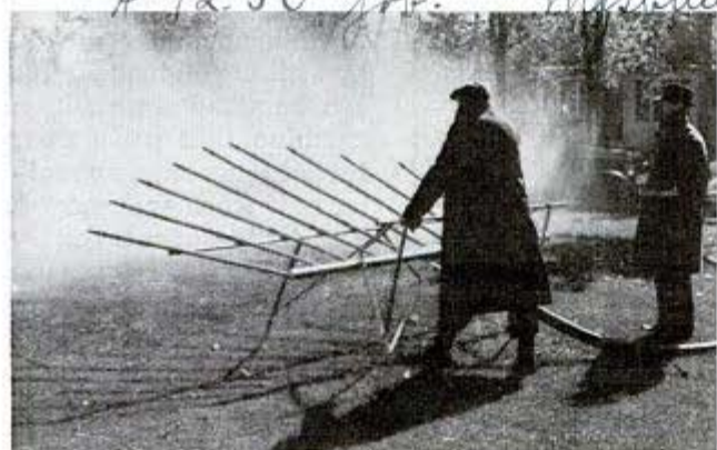
Spreading water in a mist over a wide area, this sprayer quickly builds up layer of ice thick enough for skating rink
