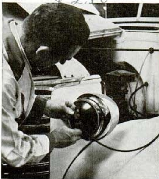
Suction cup, for removing headlight lenses and for other tasks, gets vacuum from intake manifold
