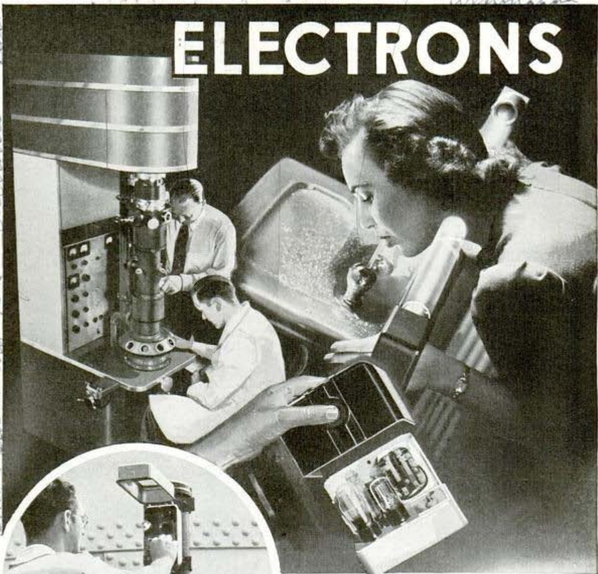
Electron microscope (upper left) magnifies up to 30,000 diameters; right, fountain flows as drinker breaks light beam. Center, a photoelectric relay. "Electric eye" in circle turns on red lights on tower near LaGuardia airport during darkness or fog
