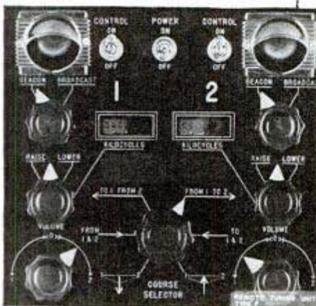
Above, bank of selector and control knobs used by pilot in airplane. Right, sketch compares new with old type radio control; dual system points plane upwind to keep it in straight line, while former system does not allow for drift
