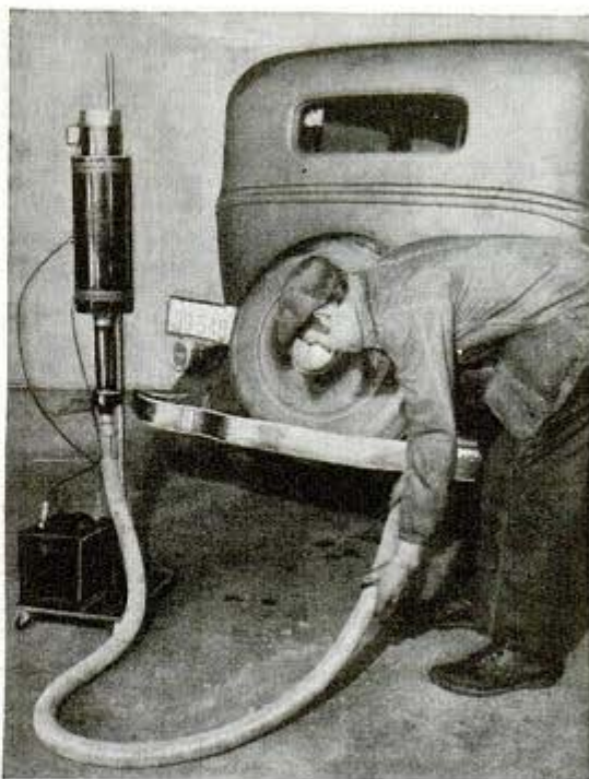
Auto exhaust gases lose their death-dealing fumes when they are passed through this catalytic chamber
