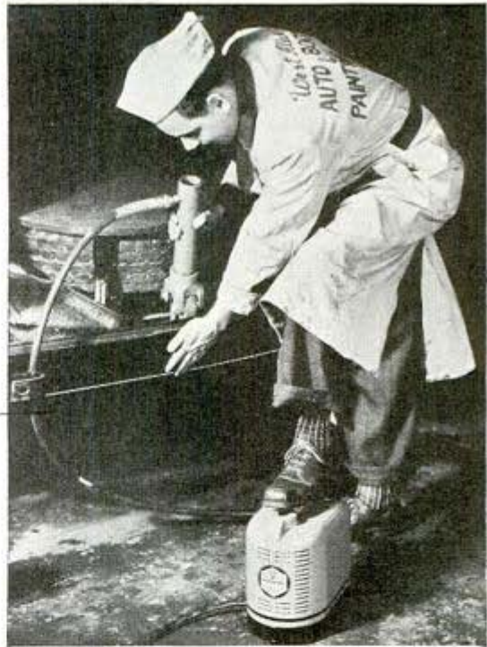
Electric pump in foreground provides hydraulic power for tool being used on crushed back panel
