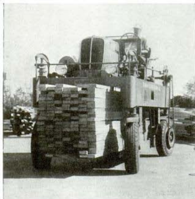
Head-on view of self-loading truck equipped to scoop up pile of lumber, haul it away, and set it down under its own power
