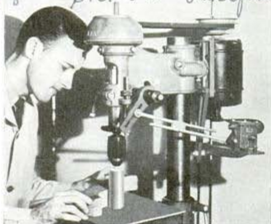
Gear reducer mounted below motor at extreme right motor shaft. An adjustable connecting rod
