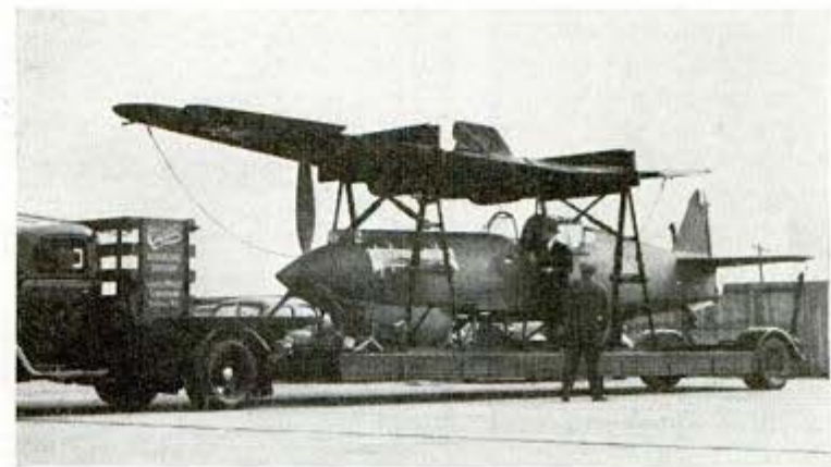
Still grounded, new planes for U. S. army "hitch-hike" on trailers to airport for assembly. Here a Curtiss P-40 pursuit ship is being towed
