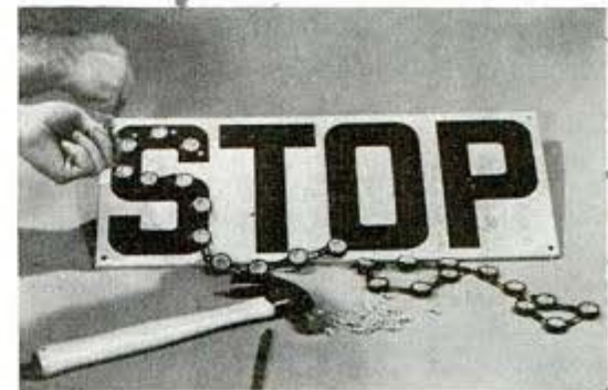
Making a "stop" sign visible at night by tacking the chain of reflector buttons over the letters
