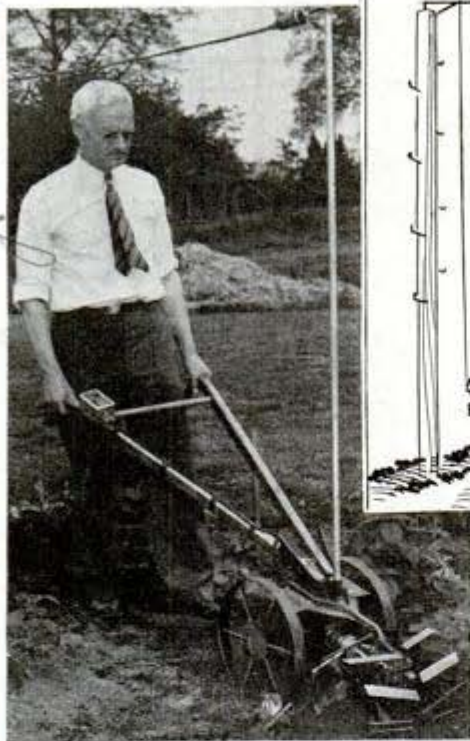
At left is the electric hoe with its mast connected to a power outlet in the field. The drawing above shows how the weight and pulley arrangement keeps the wire out of the operator's way and permits cultivation over 100-foot square areas
