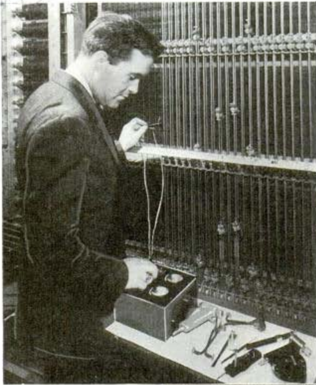
Top, portable printing equipment used for study of contact in a telephone central office. Metals make their mark by a certain color on special paper when an electric current is passed through them. Prints made by this method are studied by micro instruments
