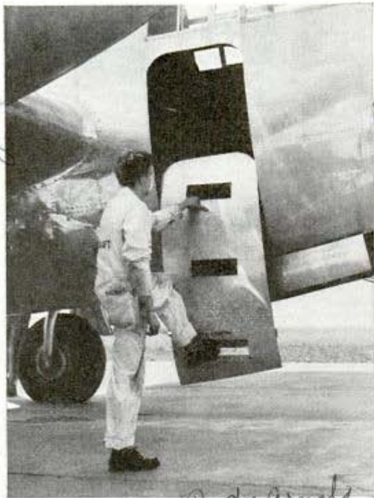
Cabin door of big fighting plane converted into convenient stairway by sliding it down built-in tracks
