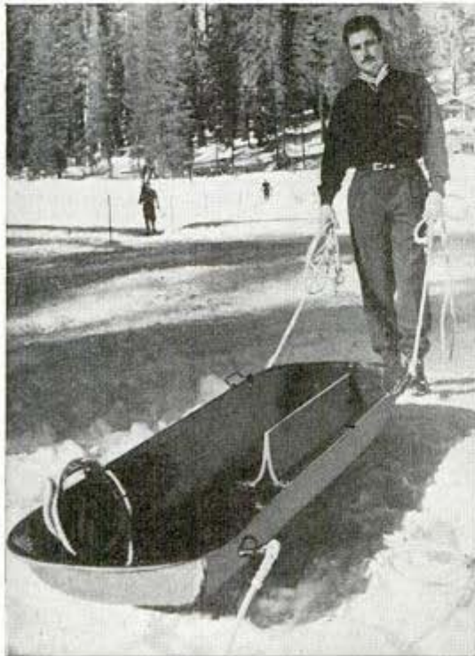
Metal sledge replaces toboggan for rescuing skiers injured on snow slides of Yosemite national park
