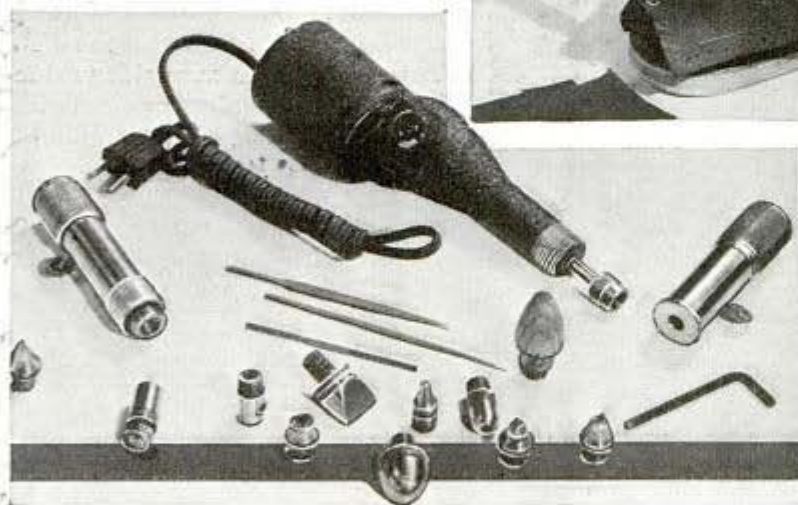
Three uses for electric plunger tool; top, left, hammering copper plate; right, tooling piece of leather and, below, filing opening in pen tray. Bottom, left, the tool with various heads and special holders
