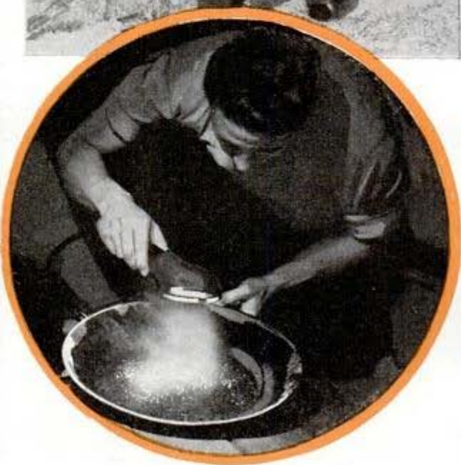
Top, left, examining abandoned mine tunnel with quartz lamp. Right, light portable outfit contains battery and high-voltage transformer for operating quartz lamp. Below, testing pan of concentrates with black-light lamp. A blue glow reveals presence of tungsten ore
