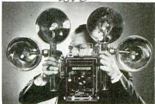
Two flash synchronizers connected together supply powerful floodlight for action or color pictures
