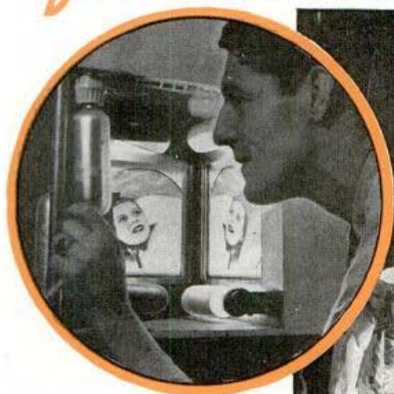
Above, an optical mechanical dissolve—titling device for television—reproduces dissolves and wipes for camera. Right, battleships maneuver in a "minnie" seaport. Bottom, building a miniature set
