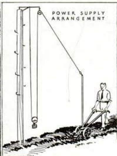
At left is the electric hoe with its mast connected to a power outlet in the field. The drawing above shows how the weight and pulley arrangement keeps the wire out of the operator's way and permits cultivation over 100-foot square areas
