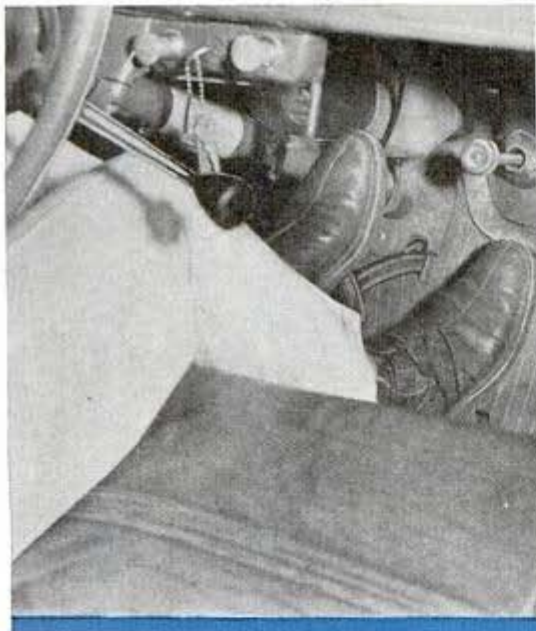
Left, gaining control on flat curve by braking with left foot and accelerating with right. What may happen if brake alone is used in going into curve is shown in photo at right. Diagram illustrates proper method of rounding curve. Below, right and wrong grip for straightaway driving
