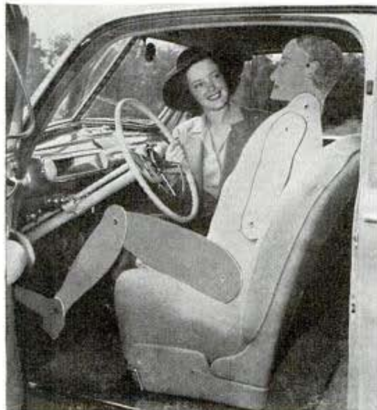
Cardboard man, hinged at ankle, knee, hip and shoulder, helps test new car models for seating comfort
