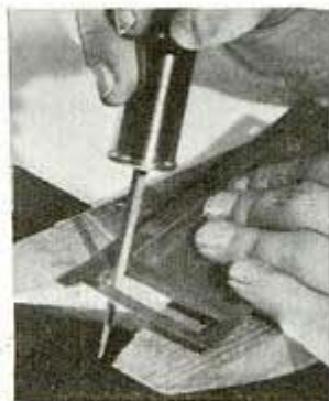
Three uses for electric plunger tool; top, left, hammering copper plate; right, tooling piece of leather and, below, filing opening in pen tray. Bottom, left, the tool with various heads and special holders
