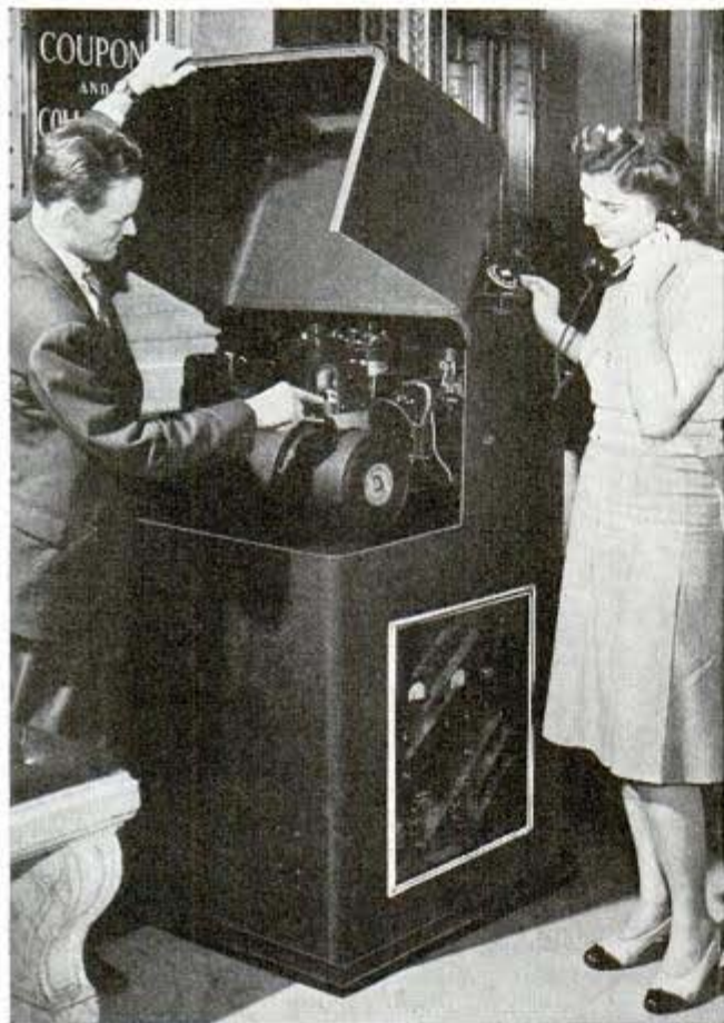
© Milwaukee Journal Self-contained instrument automatically gives correct time to customers who call the business house by telephone
