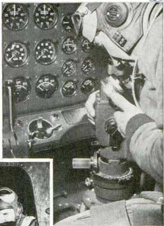
Above, photographer directing pilot through telephone in order to position plane above area to be mapped. Bottom, latest photographic plane in flight. Its cabin is electrically heated so the crew may operate in comfort at 25,000 feet. Pilot, navigator and cameraman use throat microphones which pick up laryngeal vibrations and do not interfere with supply of oxygen from cylinders on walls
