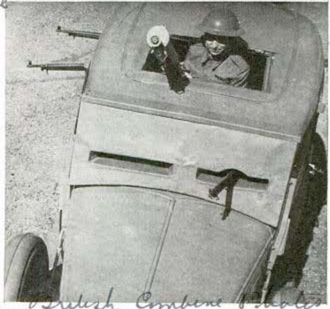
Ready for action, above, armored car has firing ports at sides and slots in front; here it is backed by three members of home guard unit. Right, roof of car opens for machine gunner ready to blast any attempted attack upon the factory
