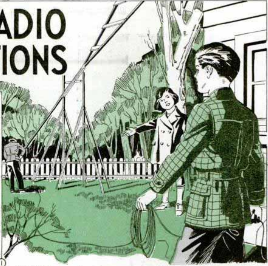
(1) "Well-sweep" antenna mast makes adjustments easy. Sweep support made with two 18-ft. 4 by 4-in. pieces placed 4 ft. apart and set 2 ft. in cement. Braces, with ends in concrete, support uprights. Mast proper is an 18-ft. 2 by 4-in. piece and two 3/4 by 6-in. pieces 18 ft. long lapped as shown; bottom ends are spread 3 1/2 ft. apart. Mast is counter-balanced on 3/4-in. pipe trunnion and spacing blocks
