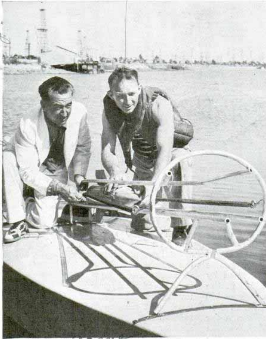
Preparing to fire a dummy torpedo with the "sling shot" coil spring arrangement built on deck of an outboard racing boat for a demonstration.
