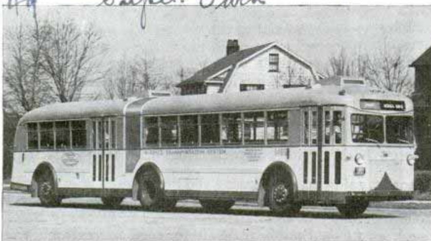
"Knee joint" permits bus to arch in middle to keep all wheels on street
