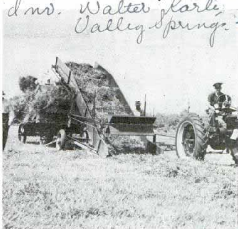
This tractor-operated machine built by a South Dakota farmer picks up either grain shocks or hay and loads the rack wagon
