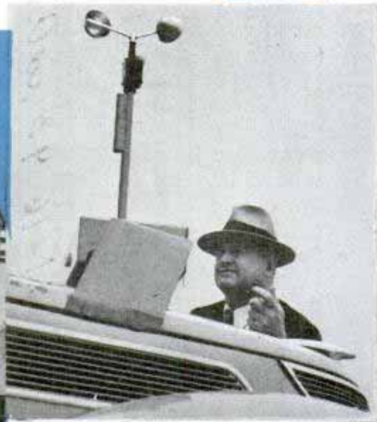
Left, directing traffic on Golden Gate bridge from electrical control booth. Above, portable wind recorder mounted on automobile hood is moved to various locations on bridge to check wind velocities. Below, an engineer inspects cable 740 feet above the water
