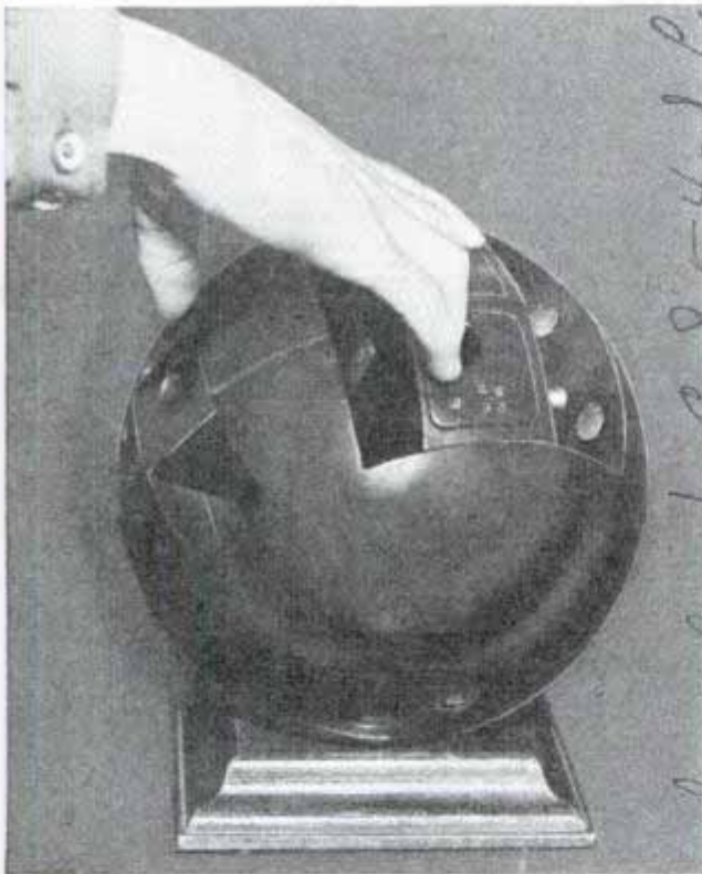
Natural span of the bowler's grip is measured with the adjustable plugs of this gauge
