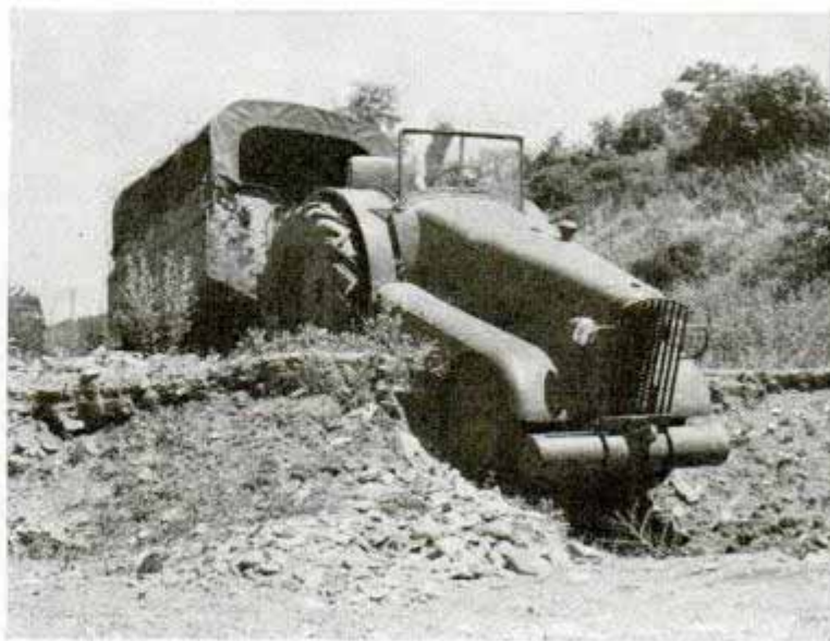
Rugged army tractor can travel over roughest terrain or keep up with caravan at fifty miles an hour with howitzer in tow
