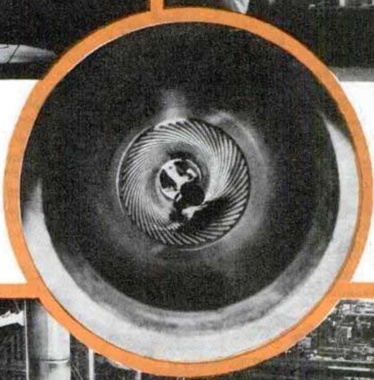
Above, final assembly of a big Douglas transport wing. Circle, workman at Rock Island arsenal inspects rifling of a 155-millimeter howitzer barrel. This gun is of the world war period and will be reconditioned if the rifling is satisfactory
