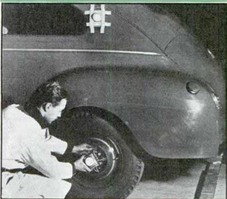
Top, photographing moving gears with stroboscopic illumination. Center, attaching telltale lights so each will trace moving line of light across photographic plate (bottom) in test of Plymouth riding qualities. Note irregular line of wheel light indicating spring action
