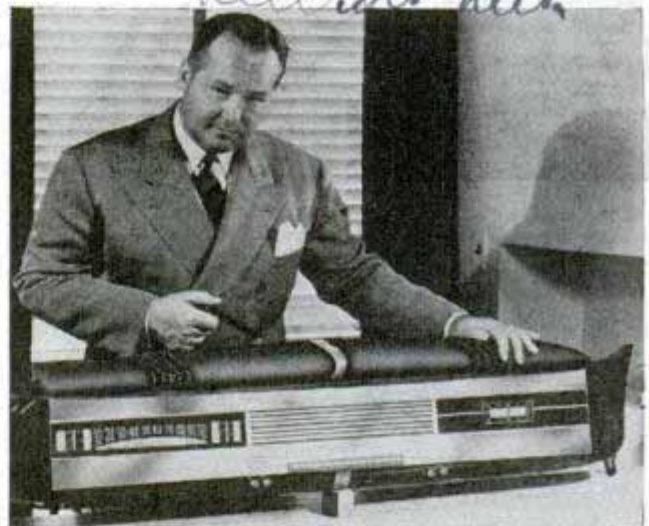
Bulging upper edge of instrument panel is "crash pad" that absorbs shock if riders bump against it
