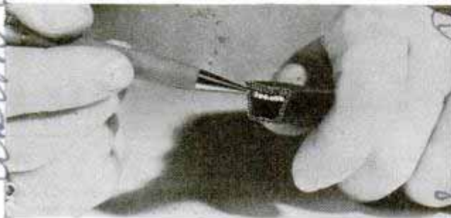
Resistance to static built into V-belt prevents large electrical discharges and stops short circuit
