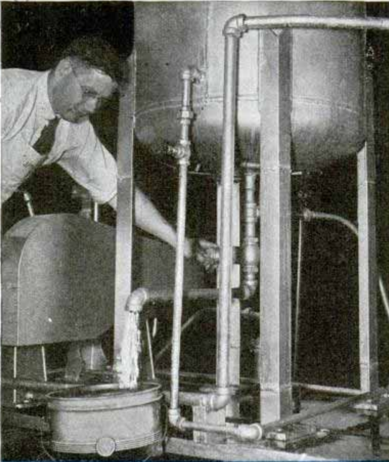
Top, buna emerges as a liquid; it is a synthetic rubber product of petroleum cracking. Below, lining a tank with Kerozeal for handling acids; right, sheets of Ameripol (left) and natural rubber (right)
