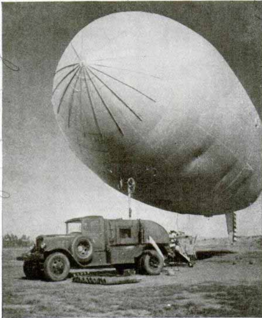
A winch mounted behind the cab handles more than 4,000 feet of steel cable anchoring the observation balloon to its mobile base
