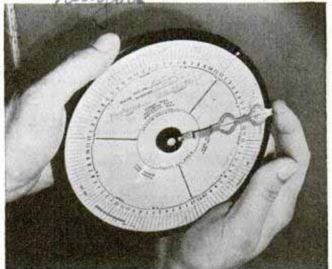
If you ever rent an airplane it's likely to carry one of these meters to show how many hours you fly
