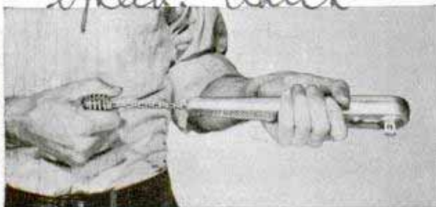
A few jerks of chain spins nut on or off the bolt
