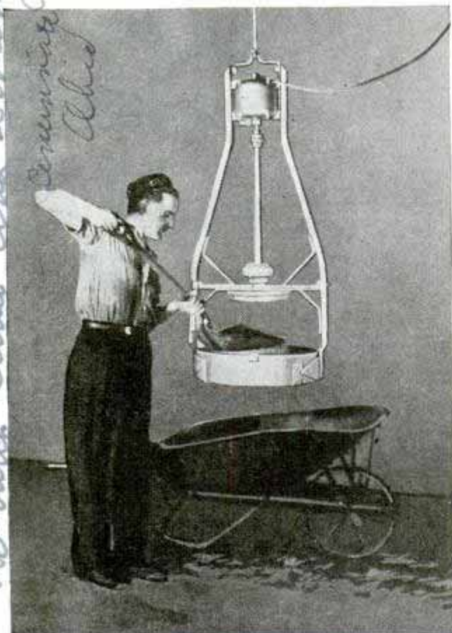
Electric screen, shaken by a rotating head connected with motor, quickly sifts material shoveled into it
