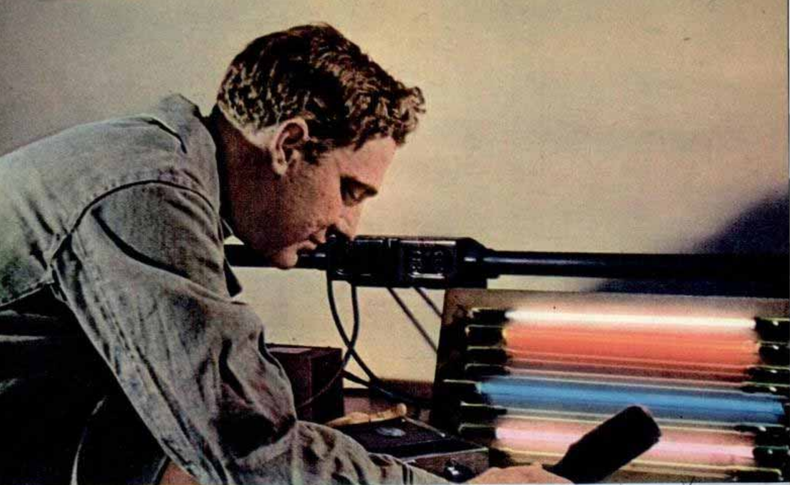
K 68 d 424 Westinghouse color photo showing gaseous discharge tubes on rack. Top to bottom, helium, neon, mercury and nitrogen. Left, color mixture by addition of wave lengths of light and by subtraction. Bottom, fluorescent lamps of all colors being tested at Nela Park, headquarters of General Electric lamp department.
