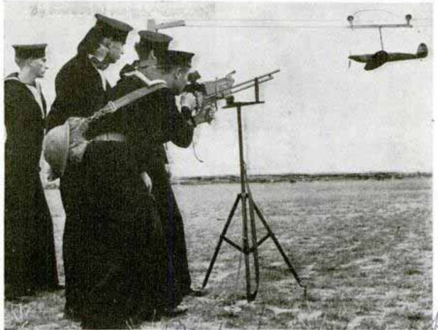
British camera gun and trolley target may be set up either indoors or outdoors for training aerial gun crews in defense against air raiders
