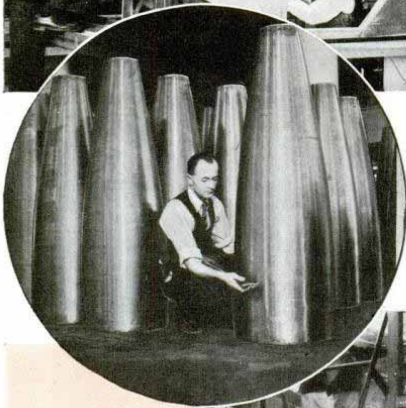
Above, heavy steel framework or jig inside of which a Vega airplane fuselage is being assembled. Left, machinist-inspector measuring new torpedo rear sections in the Navy's plant at Alexandria, Va. Some parts of modern torpedoes must be accurate within 1/10,000 inch. A torpedo costs several thousand dollars, considerably more than the cost of the biggest and deadliest bomb which does not require such delicate mechanism
