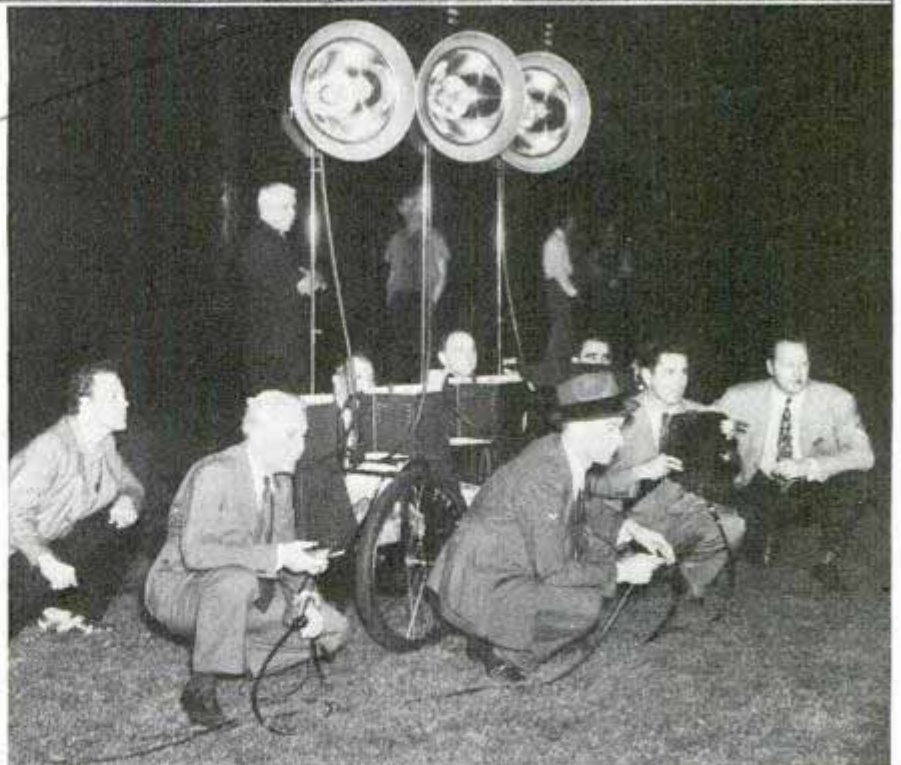
Ref: Chicago Tribune The brilliant flash of the battery of high-speed lights captured the fast action of a night football game (top) in an exposure of only about 1/34,000 of a second. The cameraman and his light crew are shown below. The three lamps in special reflectors produce light equal to 120,000 fifty-watt bulbs. On their rubber-tired dolly the lights could be rolled up and down the sidelines to follow the action of the game
