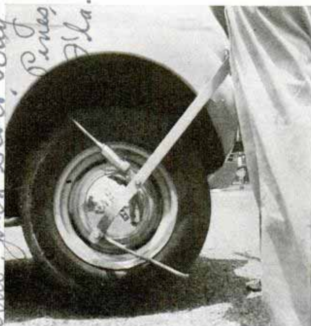
Pressure is applied to hand lever with brakes set, and gauge is read as wheel begins to slip
