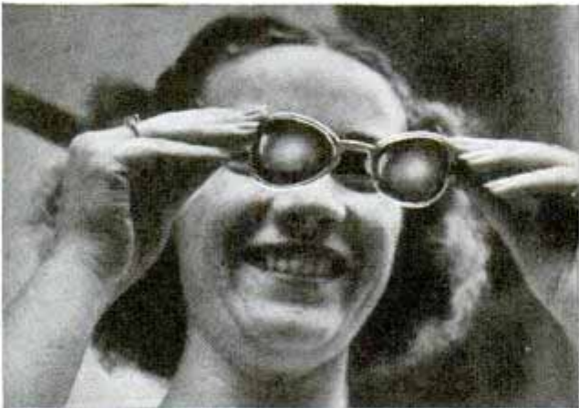
Night driving glasses with clear center and dark edges reduce headlight glare when head is tilted
