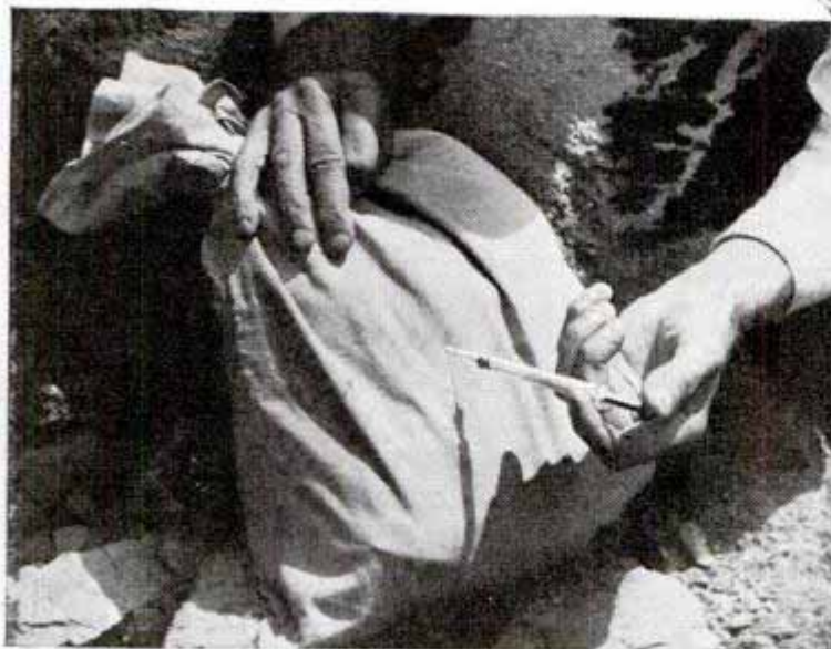
Top, photographing spot where samples have been taken, a safeguard against salting. Center, false rivet in shovel handle allows gold dust to drop into gravel. Bottom, needling gold solution into sample bag
