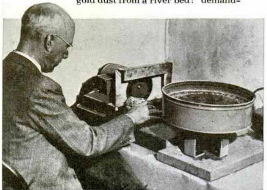
Slicing thin section of rock on diamond-studded wheel. Top, examining ore under petrographic microscope to study the appearance of individual grains and, right, gold dust being rolled in cigarette
