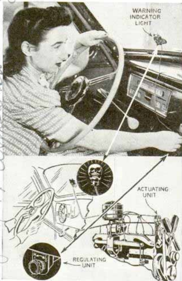
Top, turning control knob to set auto speed-light; sketch below shows installation of light and switch
