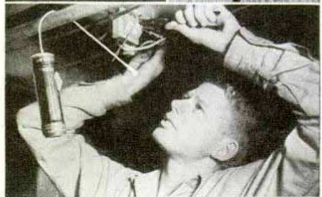
Screwed into the flashlight socket, the extension lamp lights up work at inaccessible spots
