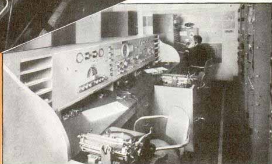
On the navigation bridge of the S.S. "America," above, is the radio compass with which the liner's position can be determined. At left is the engine room and main switchboard. The ship's two sets of triple expansion turbines develop 34,000 shaft horsepower at 128 revolutions per minute, giving her a twenty-three knot speed
