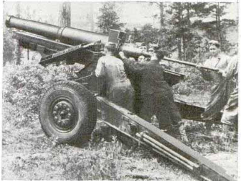
For high-angle firing, the front of the gun carriage is raised on a jack, forming a tripod with the split trail
