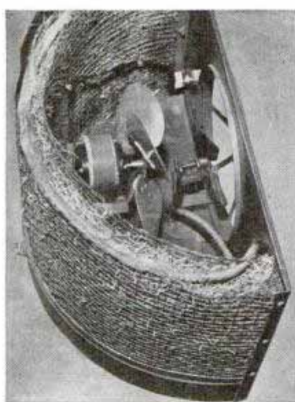
The view at left shows the wall of excelsior which is kept moist to cool the air passing through it, evaporating three gallons a day
