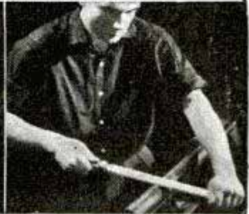
● LONG ANGLE LATHE FILES —For clean shearing, self clearing, and smooth finishing under light pressure.
