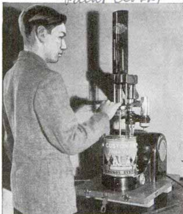
With this mixer storekeeper can blend any desired color in can of base paint while customer looks on
