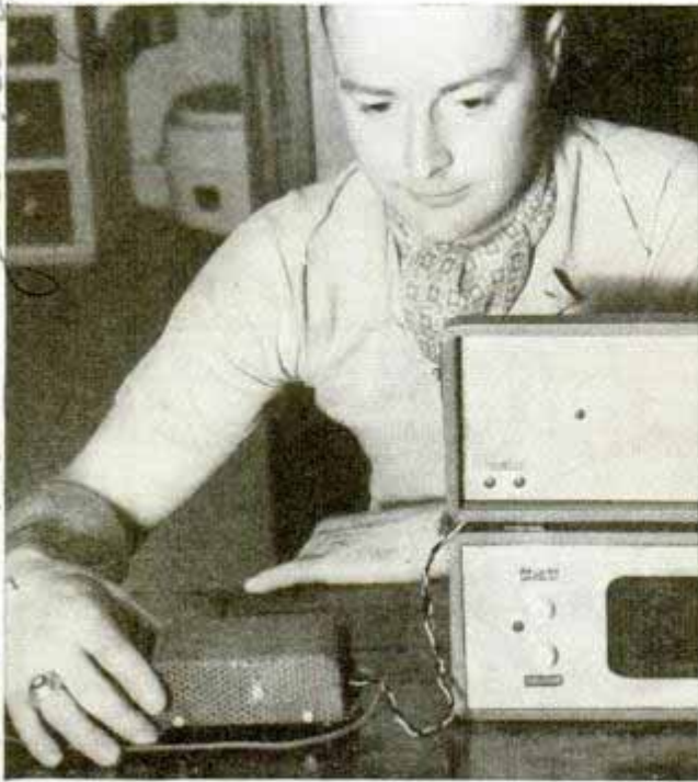
Rectifying unit, using house current, here seen plugged into portable radio to charge dry batteries
