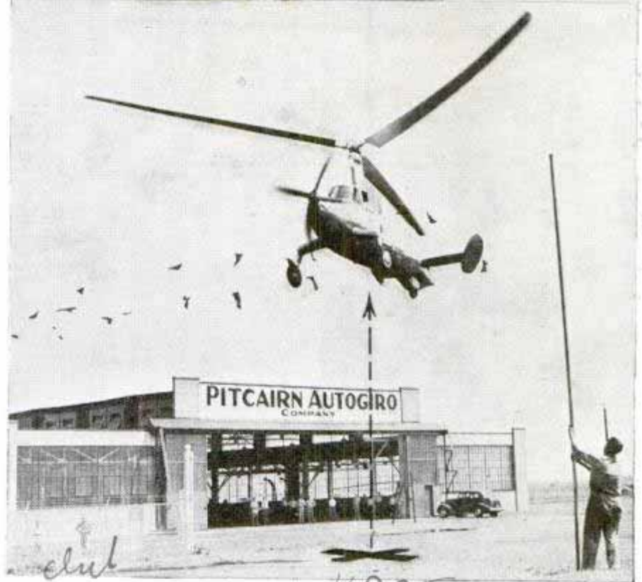
Top, rotor hub of autogiro, heart of the rotor blade mechanism, undergoes inspection by Agnew Larsen, its inventor, at left, and Harold F. Pitcairn, president of the autogiro company. Bottom, the new PA-36 autogiro, in first public demonstration, rose vertically from ground and then was flown horizontally over artificial obstacle, to show the craft's independence of ground hazards
