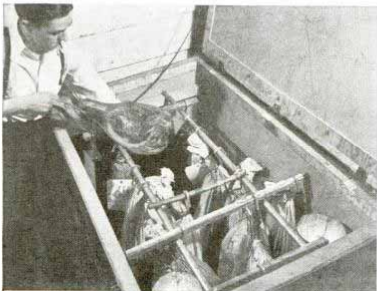
Fifteen hams at one time can be cured in this electric cabinet, which can be plugged in wherever there is a 110-volt outlet
