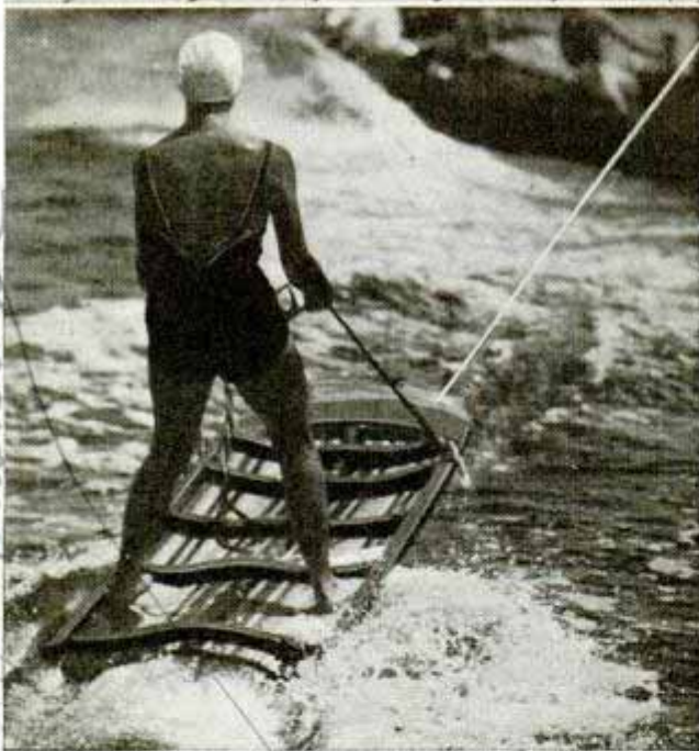
Shaped by steam-bending lengths of mahogany and spruce, this aquaplane rides more smoothly
