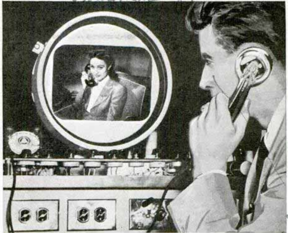
When the receiver is picked up in the world's fair demonstration of the "television telephone," the image of the caller appears on the screen
