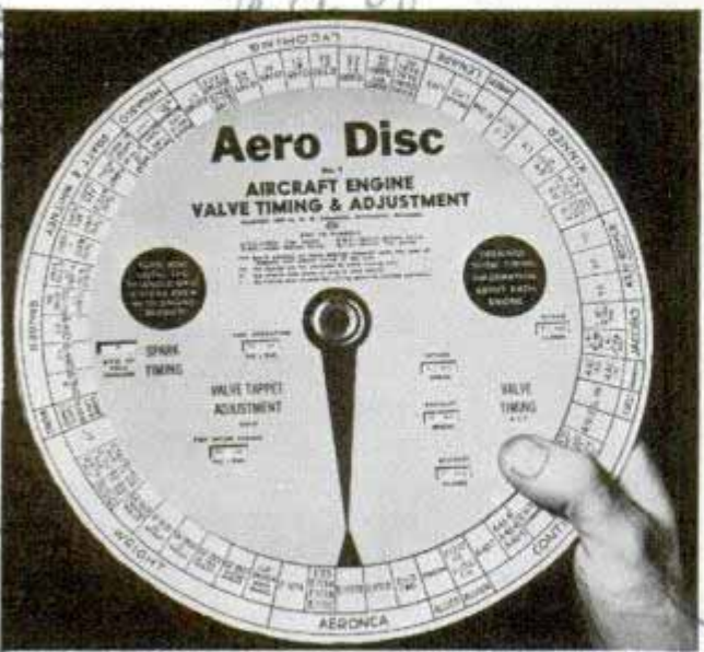
Openings on dial show mechanical data on engines
