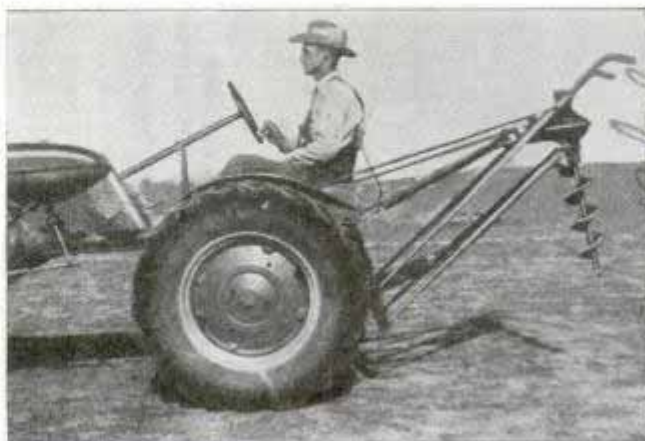
Drill mounted at rear of tractor, taking power from the engine, is able to dig a post hole in ten seconds
