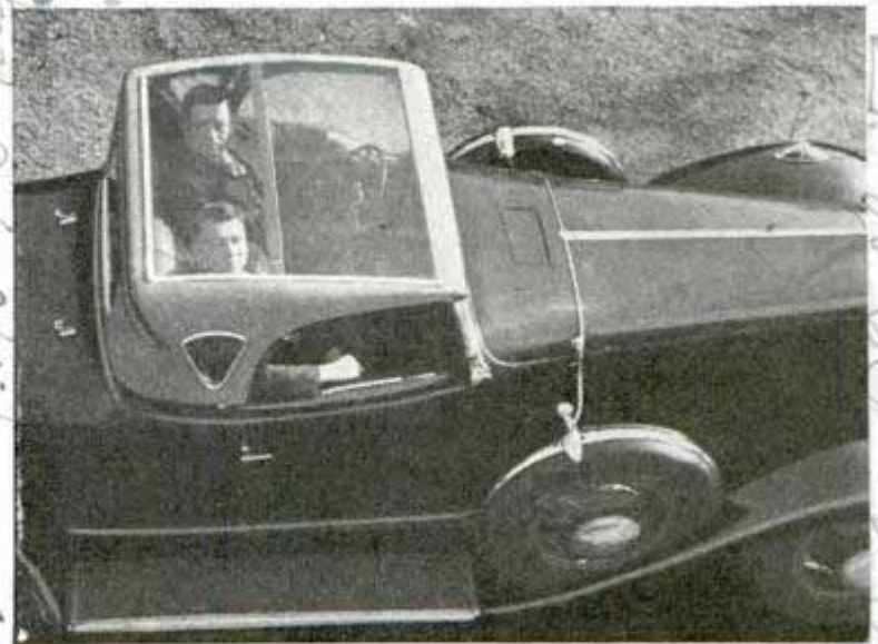
Driver and passenger have wide view of scenery overhead from auto equipped with transparent roof for mountain sightseeing
