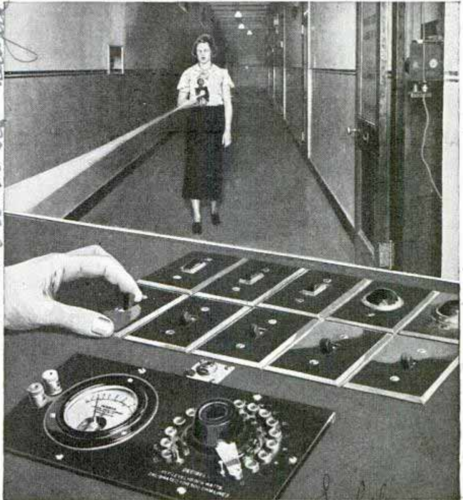
Portable buzzer sounds as long as it is held in light beam projected from wall. Switches arrange beams to lead blind person to various locations
