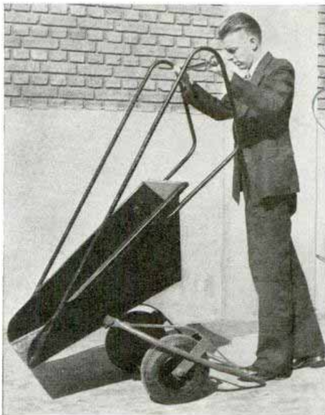
Stepping on bar at rear of wheelbarrow tilts the pan forward and dumps its load
