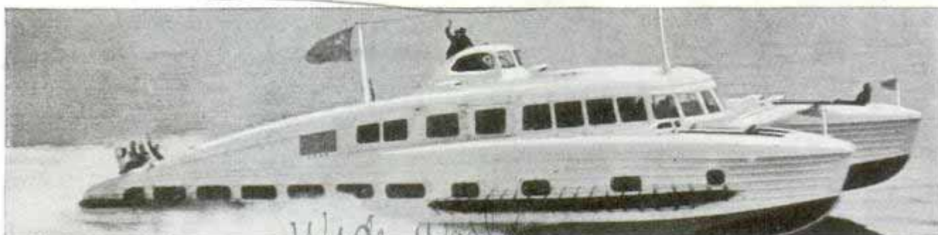
In ferry service on the Black Sea is this speedy Russian twin-hull glider boat, carrying 140 passengers
