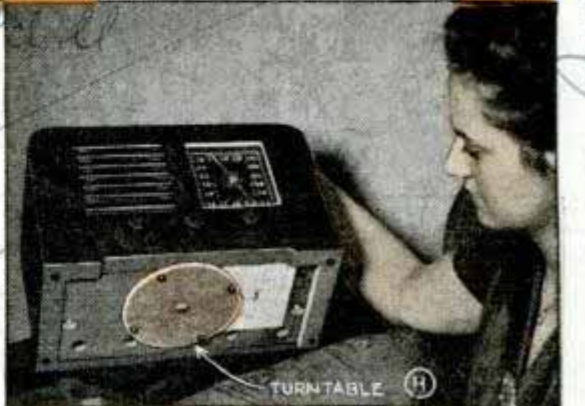
(E) Antenna-switching relay suitable for any type of experimental high-frequency switching. (F) Small electrolytic condensers easily assembled in required values and strapped together to form any filter block combination. (G) Interchangeable 2 and 3-pole receptacles and plugs for serviceman's kit. (H) Rotating base acts as turntable for small standard set; permits user to turn receiver for maximum signal strength from built-in loop antenna
