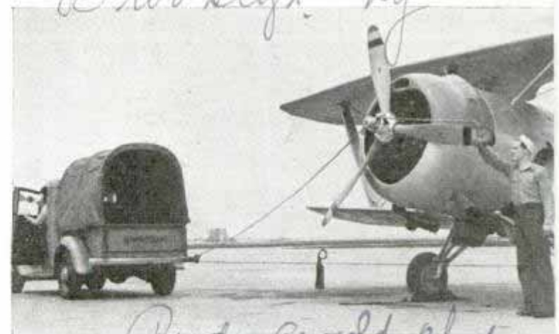
Truck helps start stubborn plane engine by turning propeller with cable attached to mitten that slips on and off blade easily
