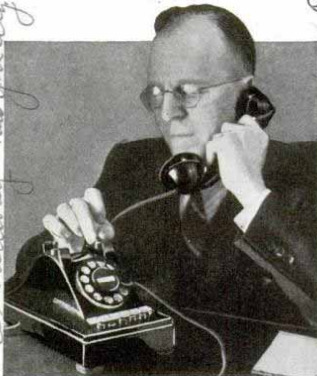
Telephone used as switchboard, inter-office or extension phone, is made private by raising tiny post
