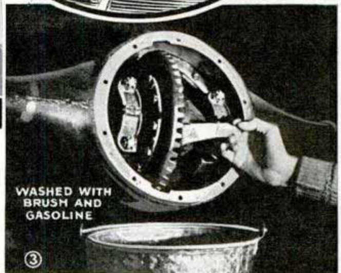
Differential cleaned thoroughly
