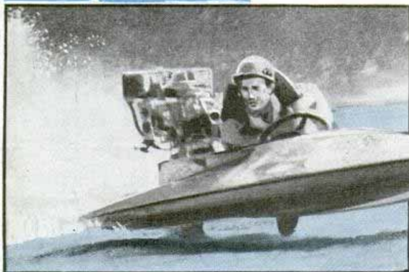
Top, lowering $700 motor into 225-class hydroplane hull. Circle, Jack Cooper, a 225-class record holder, in outboard. Bottom, bouncing along at fifty-eight miles an hour with only seven inches of hull touching the water.
