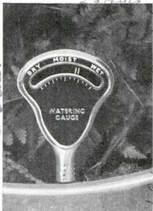
Thrust into the soil, the gauge shows whether the plants need more water
