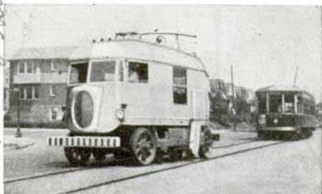
Track grinder moves out of street car's way under own power; grinders get power from trolley wire
