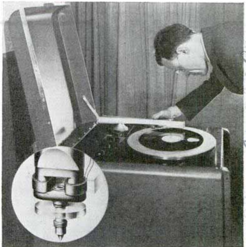
Notice the viscous disk on the stylus mount. This eliminates any high-frequency resonance due to material of the record
