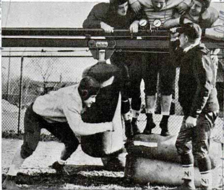
As the player charges, the dummy's movement on its overhead track is resisted by a pneumatic cylinder, and the coach reads his power on dials.
