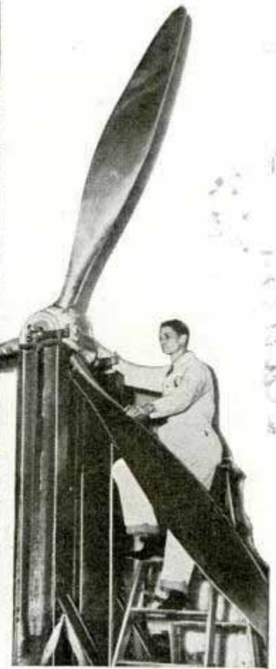
Part of the regular routine of servicing a Clipper plane is to check the tank compartments (upper left) of the hydrostabilizers, the two lower stub wings. Each of these "sea wings" holds 1,500 gallons of gasoline. Above, a three-blade propeller is checked for static balance. Each of the four propellers weighs 460 pounds
