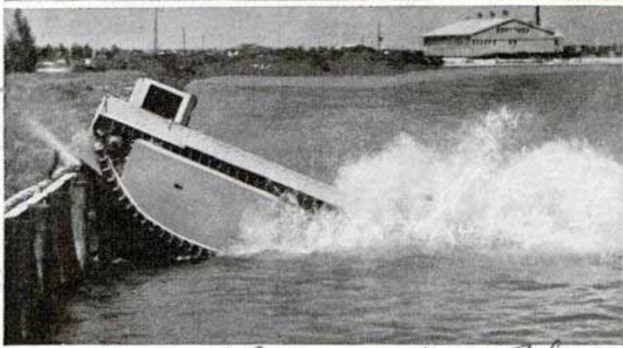
Amphibian tractor, above, carrying crew of sea scouts over body of water, supplied inspiration for design of monster land and water going war tank to be built for the United States, which will transport forty men and 7,000 pounds of equipment. Left, tractor, nicknamed "alligator," plunging into water; it was built for navigating water, swamps and land in Florida Everglades
