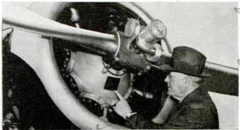
First American-made Diesel to receive a government license for aircraft use is the Guiberson engine shown above
