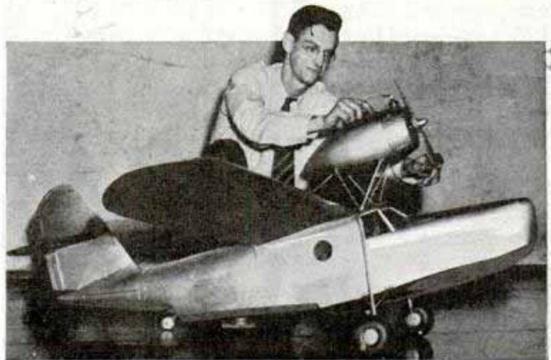
Ready for "contact," this scale model of a Fleetwing amphibian plane is powered by a one-fifth horsepower engine
