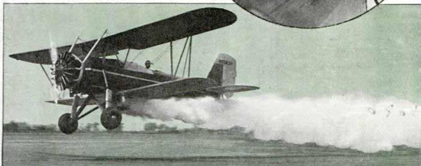
Top, filling airplane's hopper with barrels of insecticide. Center, pilot sits high for clear view of ground and hazards ahead. Bottom, flying just above ground, the pilot dusts lime over freshly planted alfalfa
