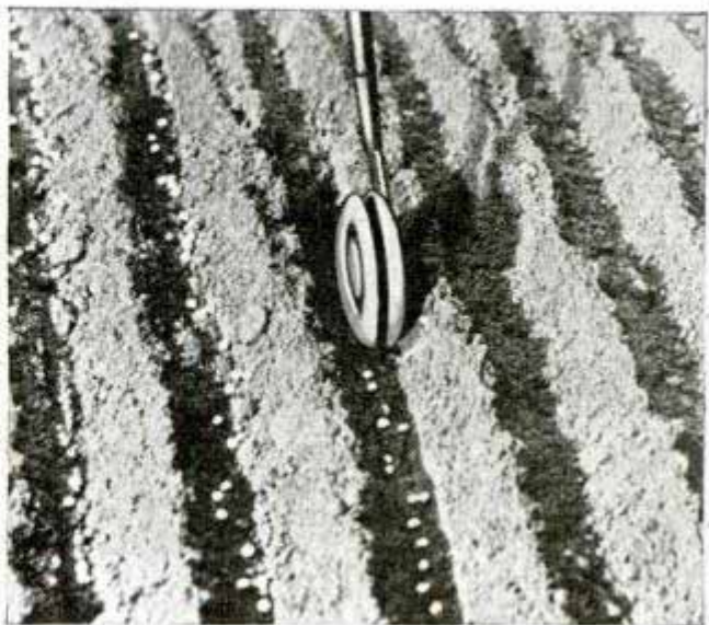
Holes in rim, adjustable for proper spacing, drop seeds at regular intervals as wheel is pushed along
