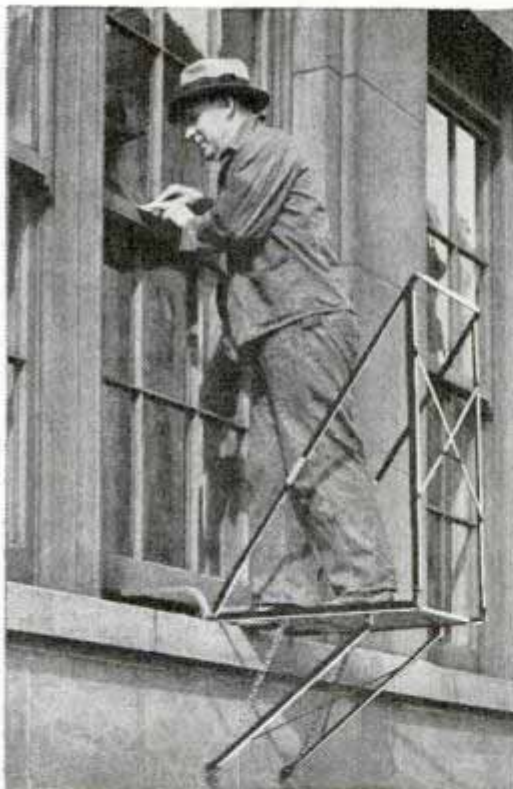
Workman has sure footing on sturdy platform that he can fold up to carry away
