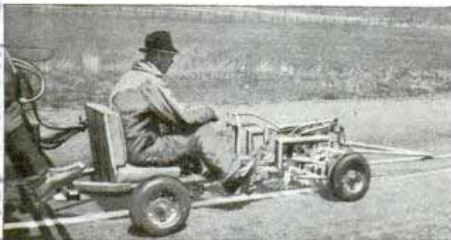
Highway striper mounted on narrow-gauge chassis is pushed by cab-over-engine truck carrying paint tanks
