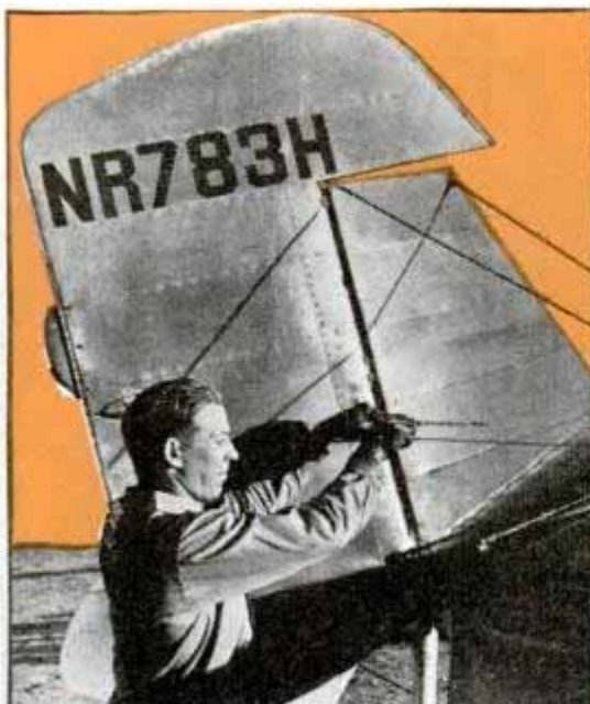
Exhaust stacks lead over the wing to keep sparks away from the trailing cloud of dust beneath plane (top). Tail (lower left) is sheathed in metal to minimize damage and assure control in case of dust explosion at rear. Pilot regulates flow of seed or dust with hopper gate lever in right hand
