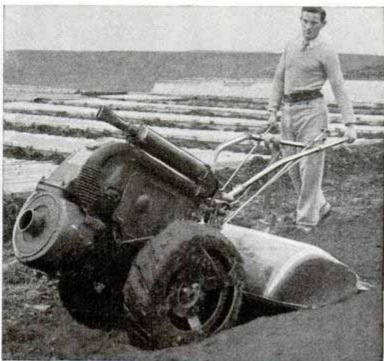
Rotary tiller breaks up the soil with pointed tines that are sharpened while they work. Degree of fineness is adjustable.
