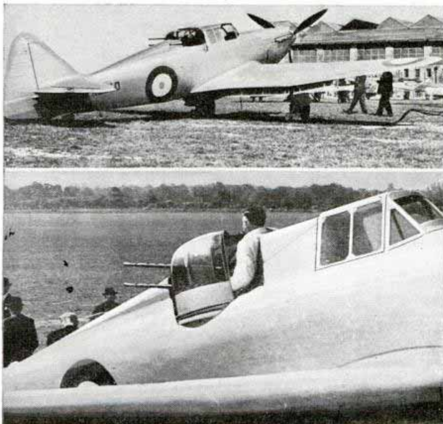
British fighter with guns in turret is more effective against bombers
