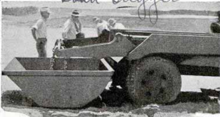
Dump truck placing detachable body on ground to be loaded; when filled the body is again lifted to truck by hydraulic power
