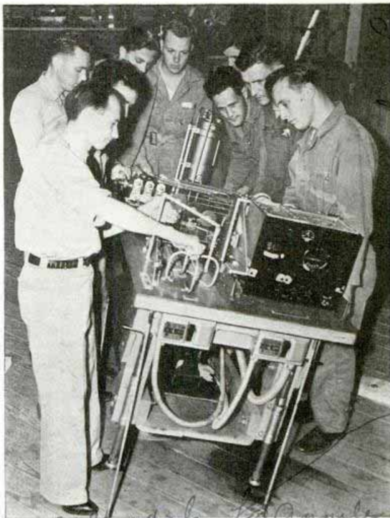
Aviation instructor using automatic pilot mounted on table to show air corps students how instrument levels tilted airplane
