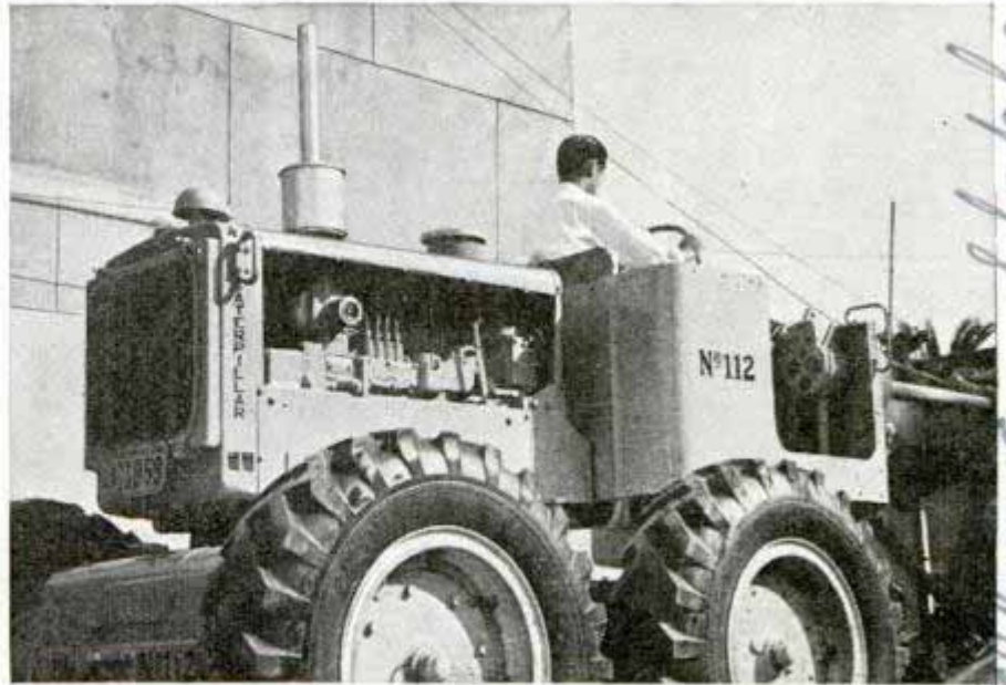
Diesel road scraper with engine at rear can be operated by one man who is able to watch performance of the scraper blade from driver's seat
