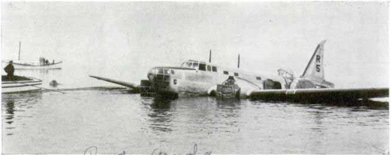
With engines, instruments and portion of the tail removed, this giant bomber was floated with the aid of oil drums tied to engine mounts and towed a distance of six miles to Floyd Bennett field
