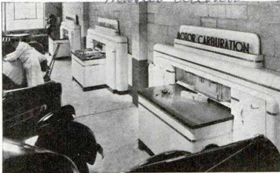
Specialized tools, supplies and working space for each section of "departmentalized" garage are centered in these "streamline" workbenches
