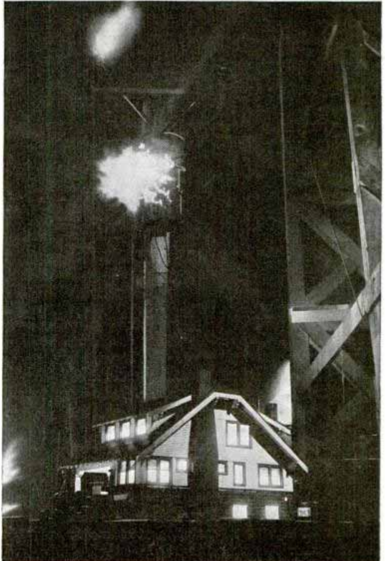
Engineers say natural lightning (top) hits earth ten to fifty million times a year. Right, half-million-volt static charge stands girl's hair on end. Below, lights stay on in toy house as 3,000,000-volt stroke detours from transformer to ground
