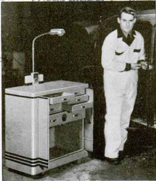
Drawers in top part of portable chest hold socket wrench set. Note electric outlets at base of lamp
