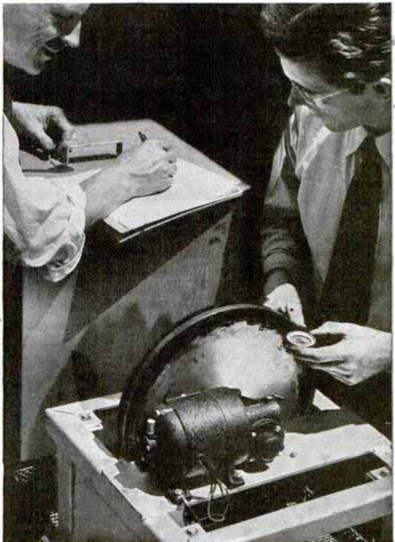
Westinghouse Fulchronograph, left, measured current in bolt striking a skyscraper. Right, (top) space between spheres is adjusted to regulate voltages up to 750,000 in circuit-breaker test; (bottom) checking magnetism in recording wheel of fulchronograph
