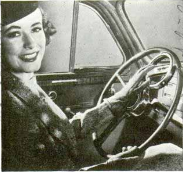
Small wheel at top of steering wheel offers an easy grip when turning sharp corners or parking the car
