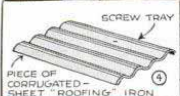
(3) Uni-directional microphone reduces background noise; the four-side call-letter plate is optional. (4) Piece of corrugated sheet metal makes handy screw tray for workbench. (5) Simple method for holding small machine or wood screws to shorten by filing
