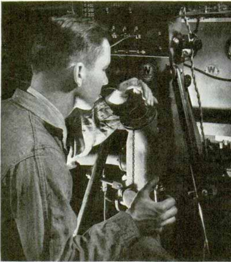
Peering into a cathode-ray oscillograph, engineer above watches path of sixty-kilovolt artificial lightning stroke through lightning arrester. Lightning flashes up to 3,000,000 volts surge between spheres at right
