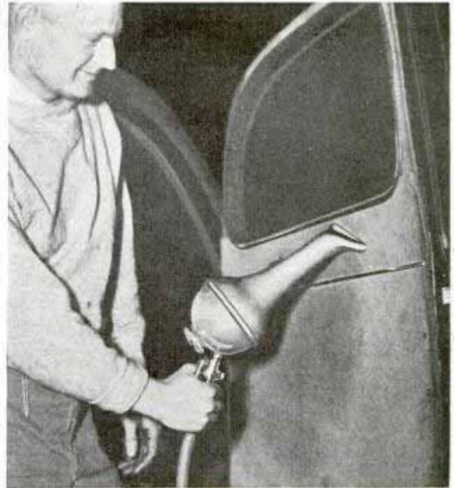
Handy vacuum cleaner for service stations operates on compressed air and produces a strong suction
