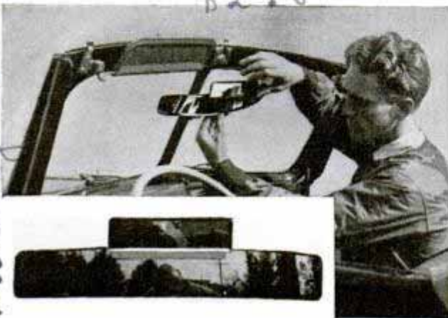
The small mirror is flat; the broad convex mirror gives full view of sides and rear
