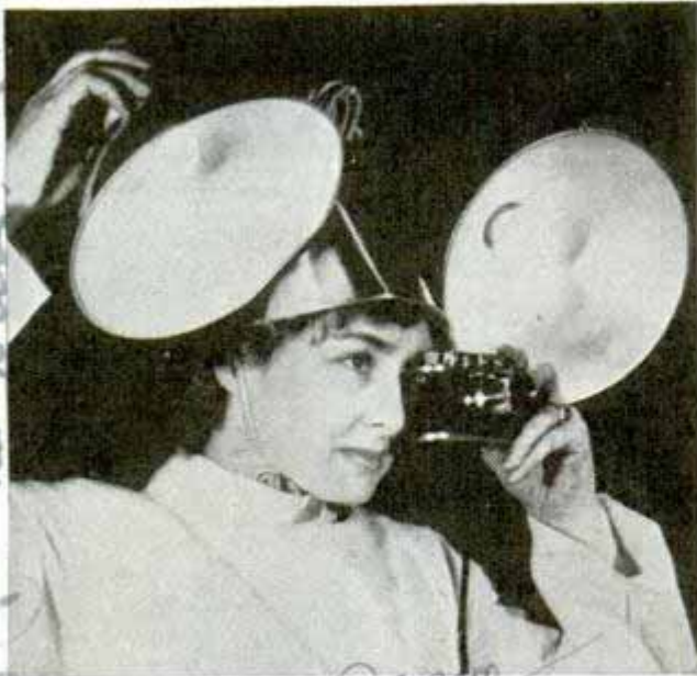
Two reflectors clamped to another which is worn helmet fashion free hands for manipulating the camera
