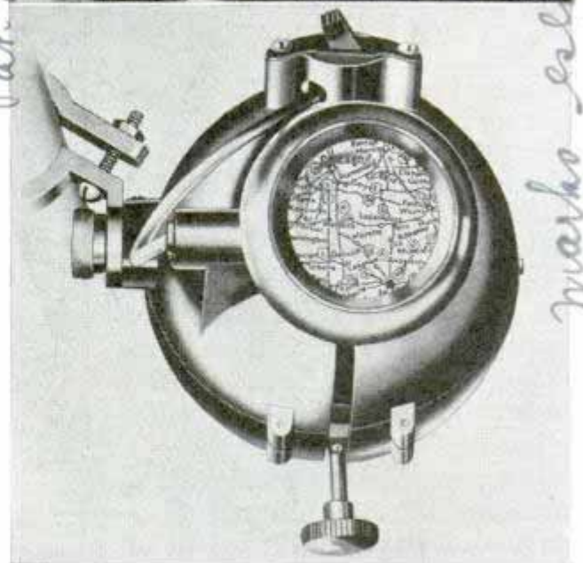
Road map mounted on steering column has light inside and a magnifying glass to enlarge markings
