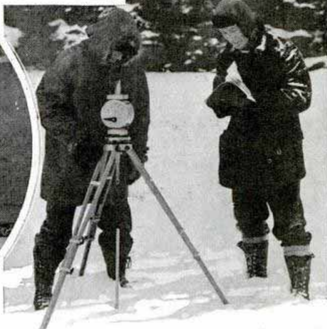
Lugging one of the portable huts on toboggans over ice, left, top, in search for ore deposits; and, bottom, engineer in hut reading meters. Right, magnet attraction of ore being measured from surface
