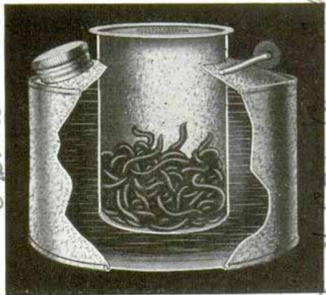
Worm can immersed in cold-water jacket keeps life in the wrigglers by condensing moisture within can
