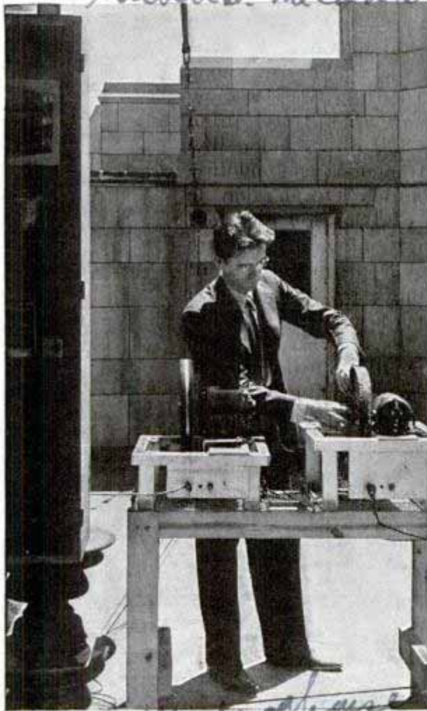
Westinghouse Fulchronograph, left, measured current in bolt striking a skyscraper. Right, (top) space between spheres is adjusted to regulate voltages up to 750,000 in circuit-breaker test; (bottom) checking magnetism in recording wheel of fulchronograph
