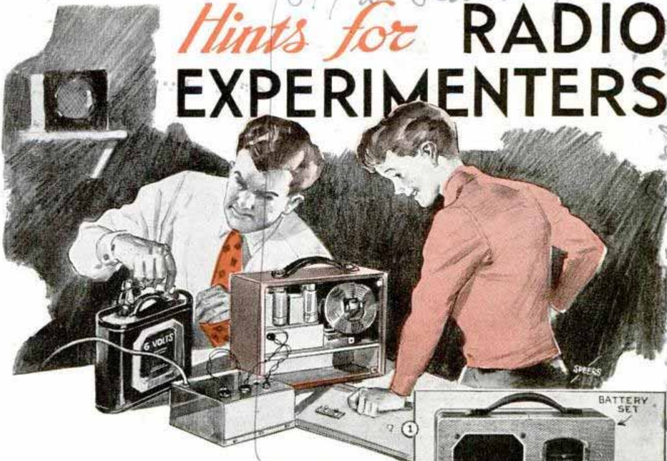
(1) You can use this compact power unit to operate any portable battery receiver from a 6-volt "hot shot" battery, or the storage battery in your car, by clipping one terminal on ammeter and grounding the other. In auto, a pole-type antenna would be employed. Power unit supplies all voltages at low drain
