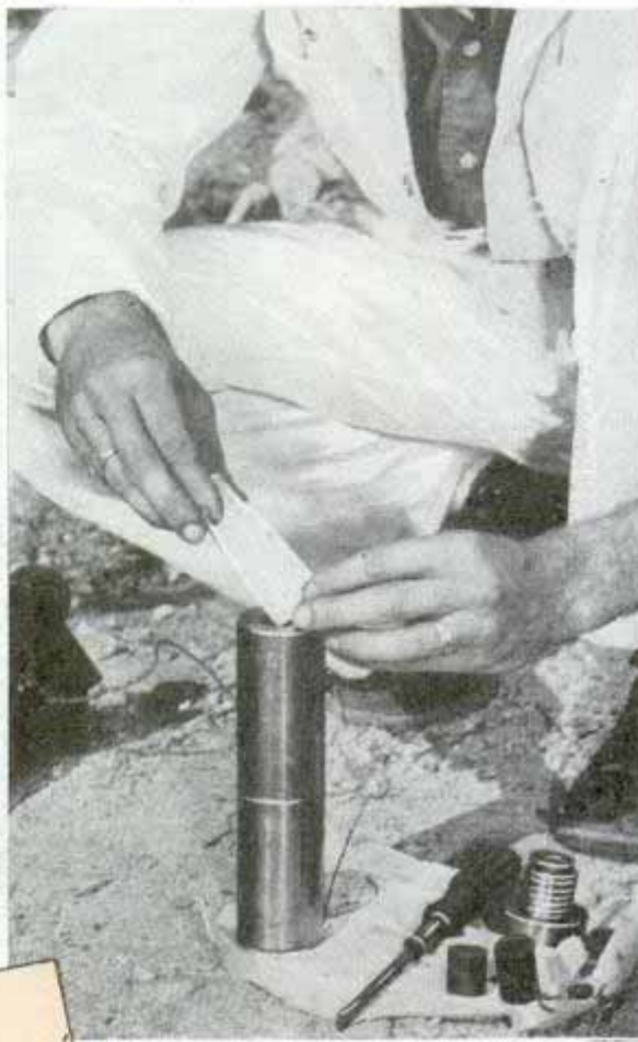
Small test rocket is loaded into firing stand, upper left, to trace its characteristic path. Above, putting powder charge in rocket. Diagram shows man's altitude records and his hopes for the rocket
