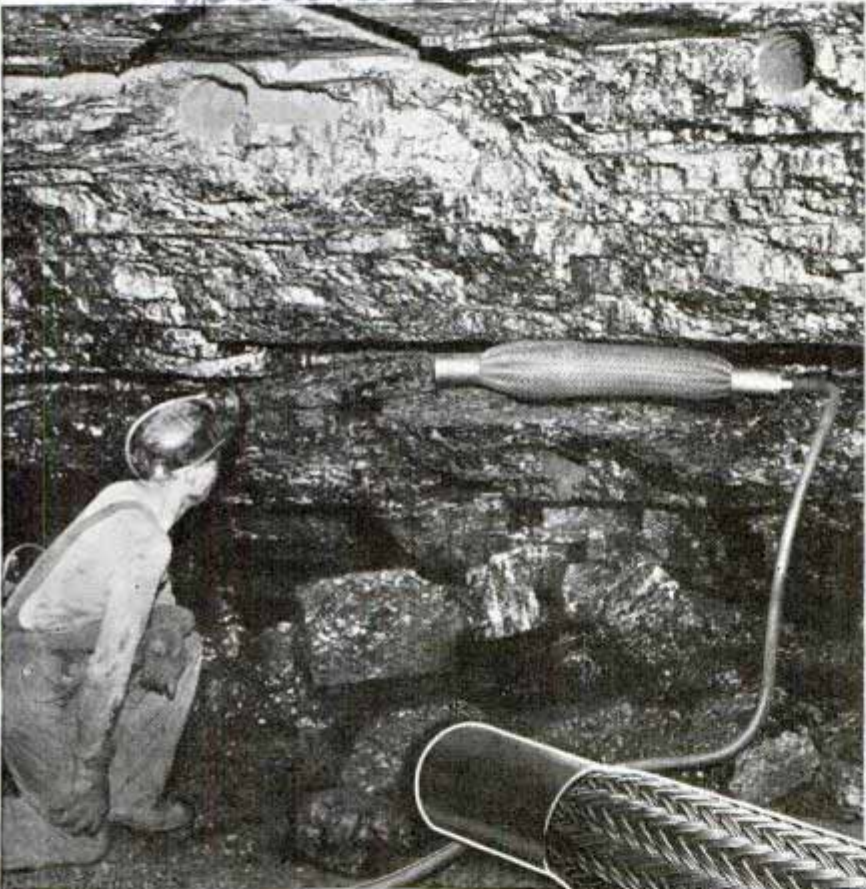
At right, miners insert the tube into hole drilled in wall of mine; left, hydraulic pressure expands tube and will shortly break coal loose along natural lines of cleavage. Cable braid around tube prevents over-expansion
