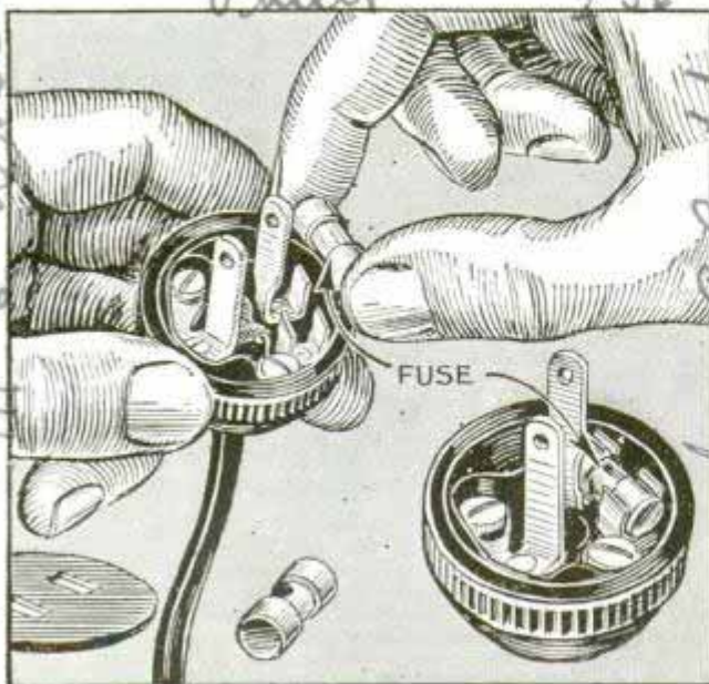
Tiny fuse inserted in wall plug at contact point prevents short circuit from overloading main fuse
