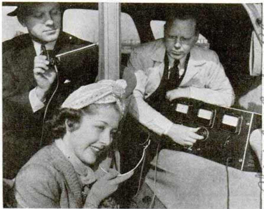
Listening to the vibration of an automobile with earphones in which the slightest jiggle or jar is amplified into a loud roar
