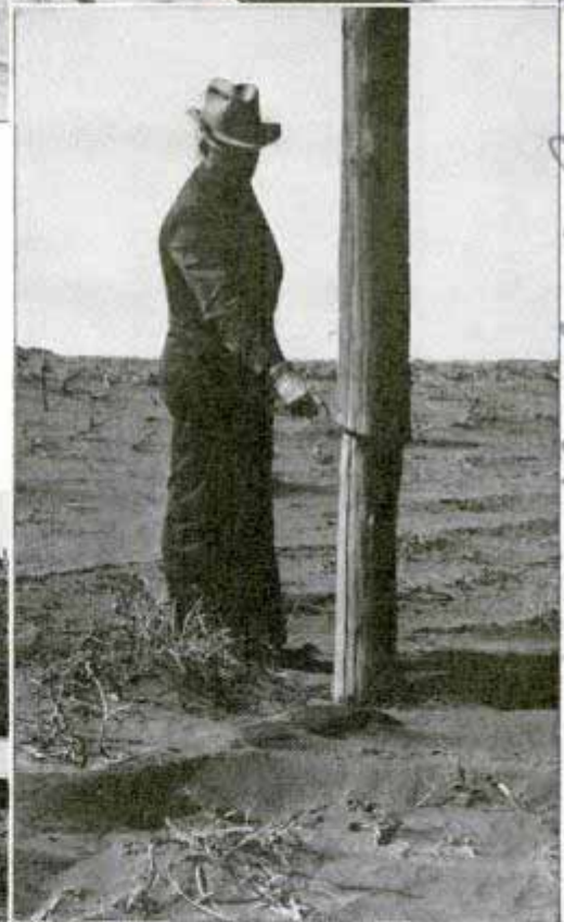
Top, strip rotation of cotton and small grain is one means of combatting erosion. Center, pointing to original ground level on telephone pole, indicating a loss of two and one-half feet of earth. Bottom, device used for measuring loss of soil caused by water erosion
