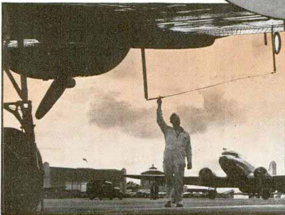
In circle, assembling the tiny radio transmitter to send weather data automatically from the raob balloon; batteries are at right. Below, a TWA mechanic inspects the radio lead-in strut on a sky liner
