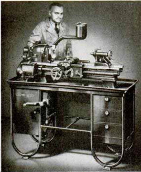
10" swing x 3½' bed 1" Collet Underneath Belt Motor Driven Bench Lathe, with All Steel Bench. Shipping weight 890 lbs. ....$700.00
