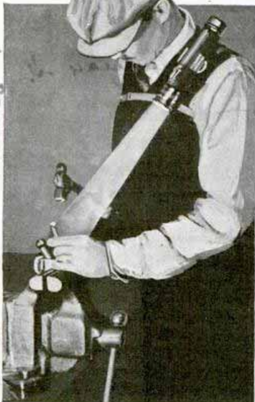
Flashlight in shoulder strap is adjusted quickly to throw beam in any direction
