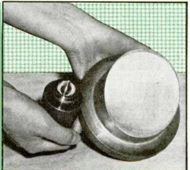
The 1,400,000-volt X-ray tube is enclosed in column at right of picture above, and connected to high-voltage direct current generator by long aluminum tubes. At left, the "end of the trail" for an electron beam at bottom of big tube. Below, cathode filament (left) and target of tube
