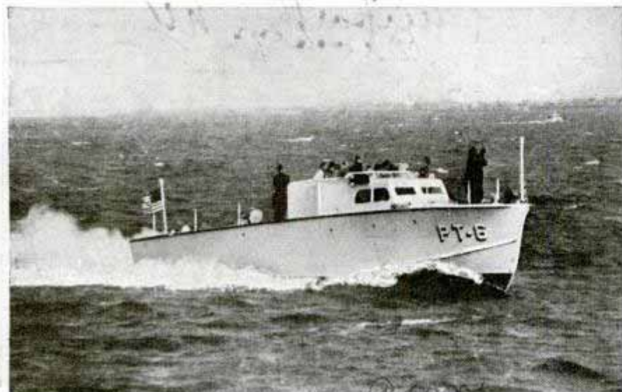
Sixty miles an hour is the probable top speed of this eighty-one foot torpedo boat tested for United States navy as new coast defender
