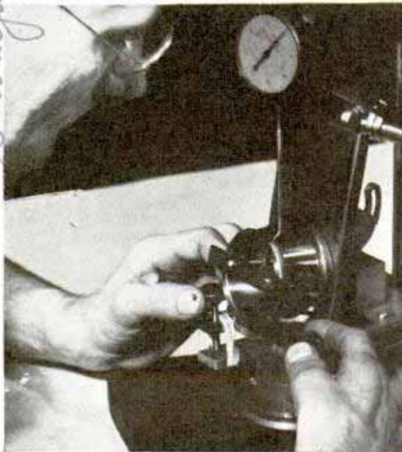
Top, photo-diagram showing how graph of surface roughness is obtained, from where specimen is placed on machine by operator to the sensitized paper where graph appears. Lines and arrows indicate the operation. Bottom, left, leveling specimen on same machine. Right, illustrating how precision manufacture of ball bearings makes it possible to interchange parts without loss of efficiency
