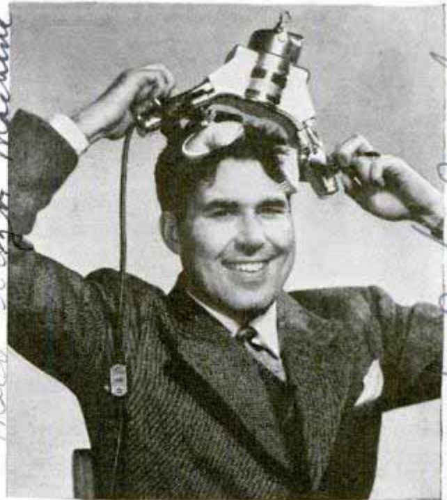
Crowned to fit head, multiple disks with 480 fingers massage scalp to remove dandruff and loose hair
