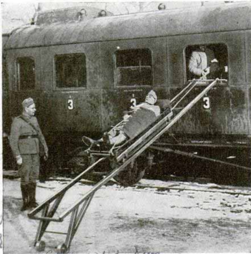
Columb. News Hospital car in the Netherlands is equipped with inclined track on which stretchers bearing wounded soldiers can be hauled aboard comfortably
