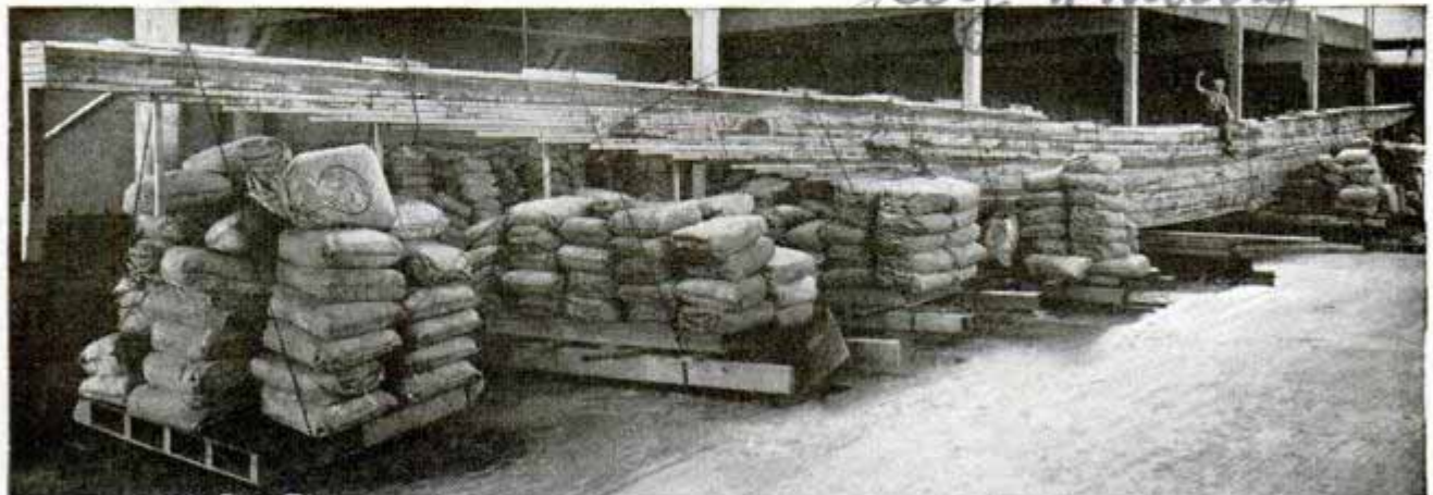
Resembling a large wagon spring, this huge laminated beam 110 feet long was built of lumber, no piece being more than twenty feet long, sealed together with casein glue. Here it is under a terrific test load
