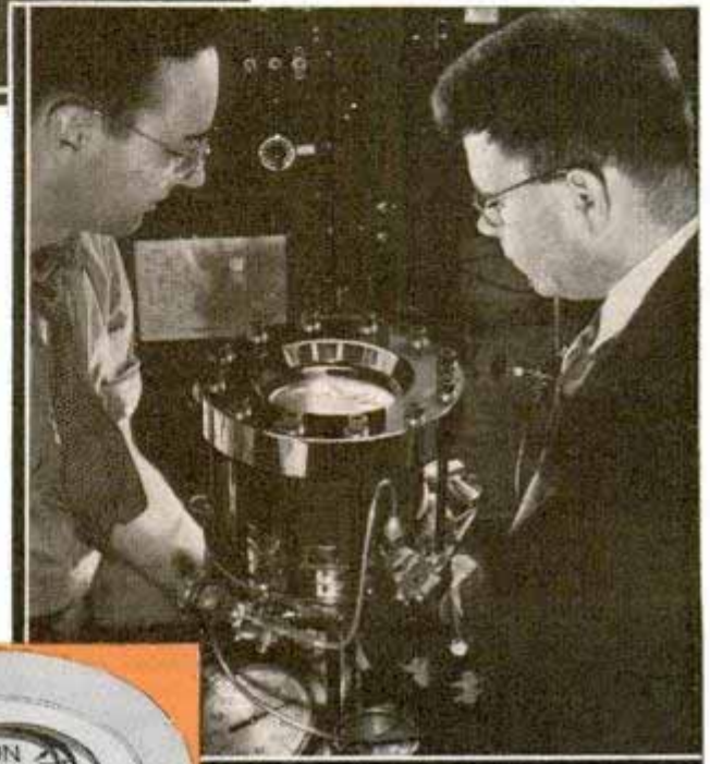
Left, screwdriver held in space by magnetic lines of force radiating from mass spectrometer. Below, chamber used in studying or photographing sub-atomic collisions. Below, left, sketch shows paths followed by particles of three different masses in mass spectrometer (spectrograph). Heaviest particles travel slowest, so follow inside "track." Bottom, section of giant vacuum tube
