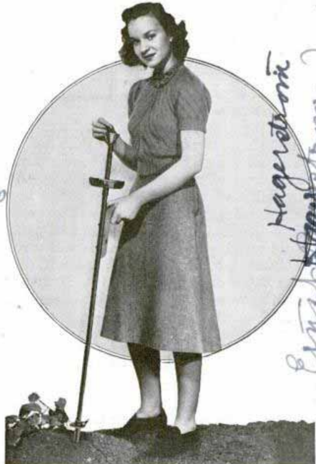
Seeds are placed in container at top, then shot into ground with trigger. No stooping is necessary
