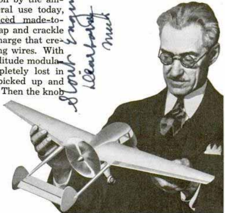
Examining model of low-priced 1940 Sky Car that is pushed by propeller at rear and has seat for two passengers side by side
