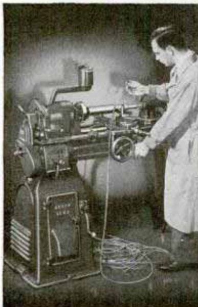
Below—11" x 4' Quick Change Gear Underneath Belt Motor Driven Lathe. Shipping weight 965 lbs. . . . . $625.00
