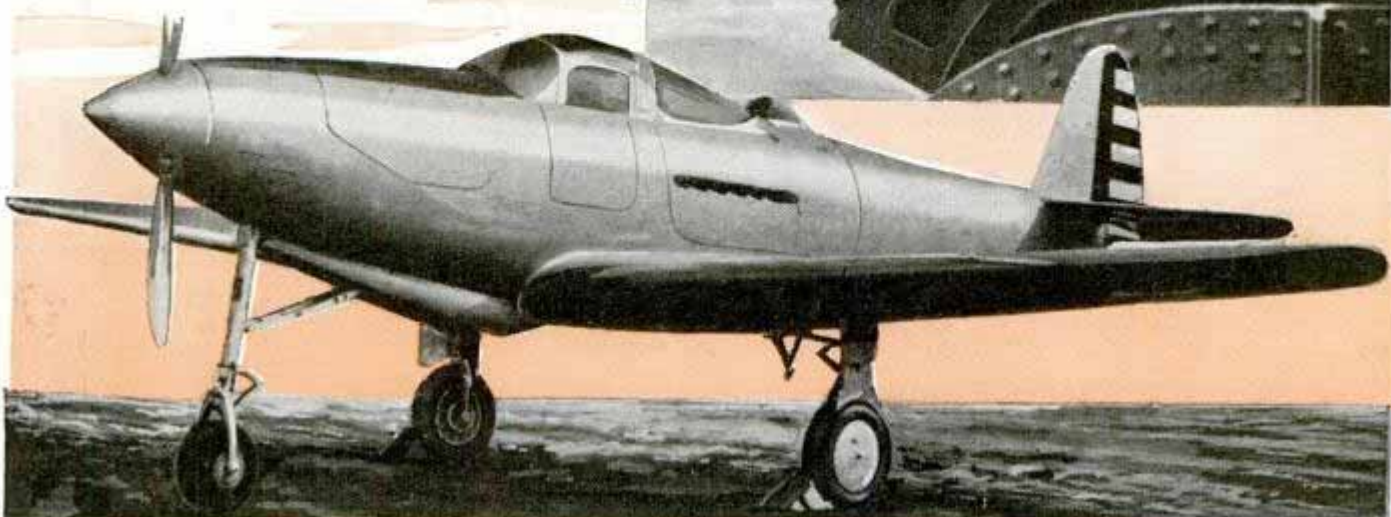
Rolling off its miniature railway track at stern of a mine layer in North Sea, a mine (right) plunges down to join the deadly belt between Germany and England. Below is the "Airacobra," U. S. army 400-mile-an-hour pursuit plane which fires 37-millimeter shell from cannon in nose
