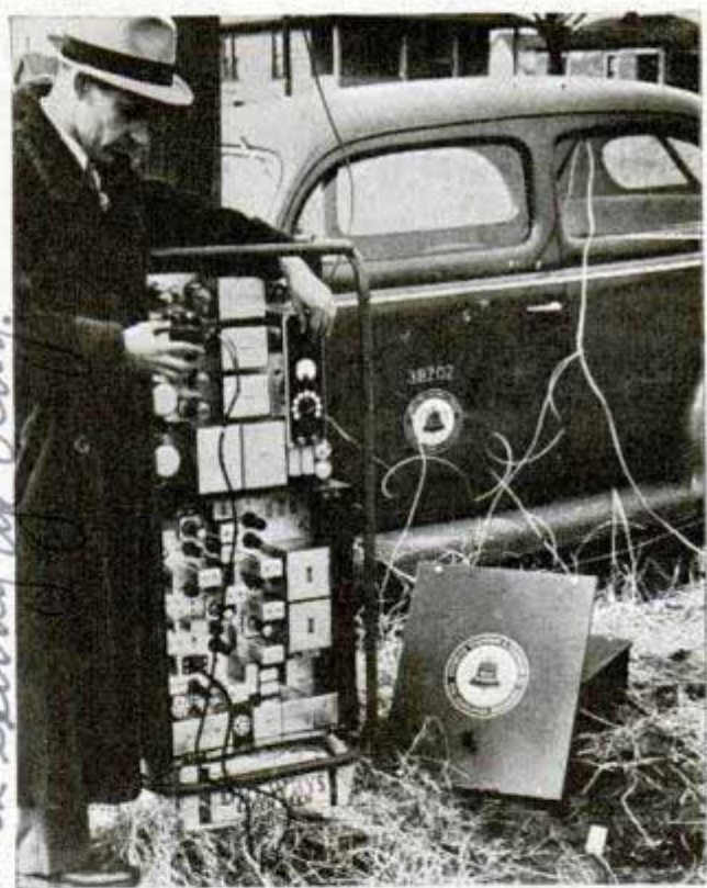
Radiotelephone establishes temporary connection between stations that lose contact over regular line
