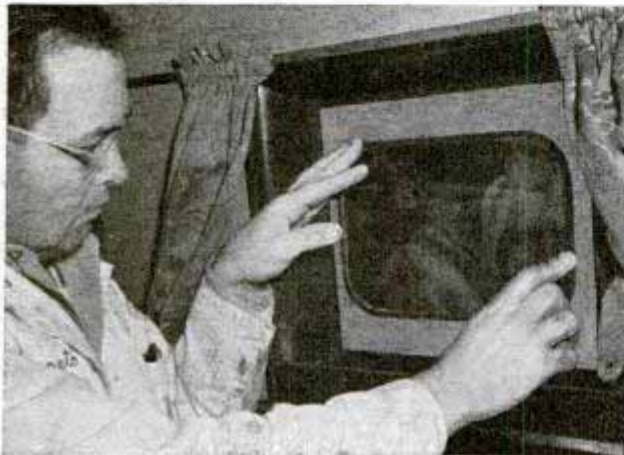
Installing non-frosting panel on window of TWA sleeper. This permits good visibility at all times
