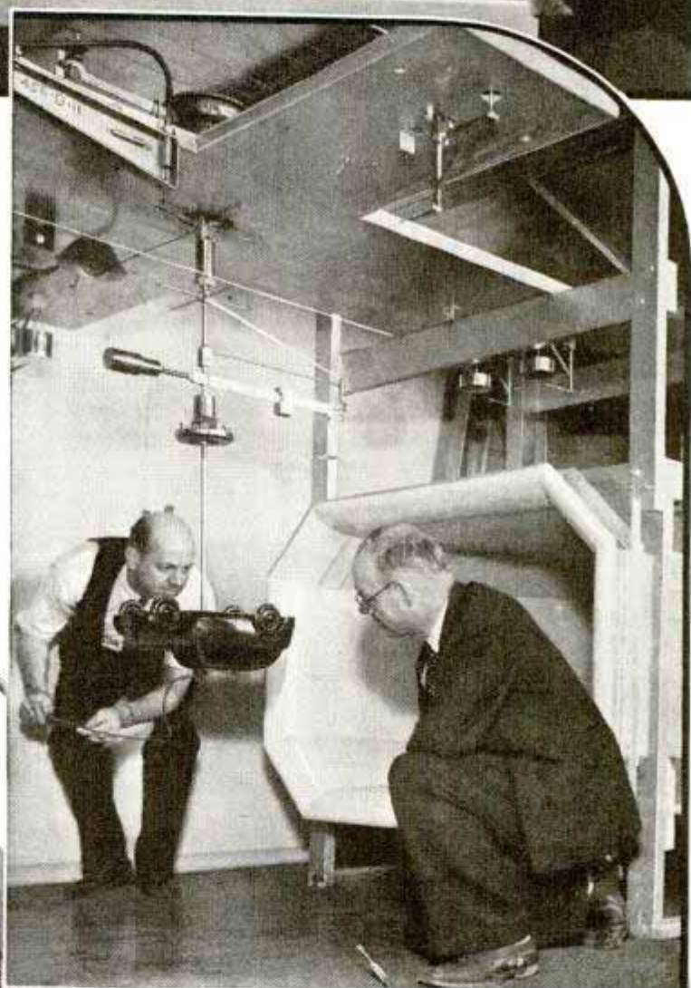
Above, working with exact-scale model of auto in wind tunnel at the laboratories. Left, X-ray tube, such as is used in probing secrets of mysterious bonds that hold metals together. These are only a few of the machines and instruments employed in the new laboratories to study every factor affecting comfort, utility, safety and service of automobiles and trucks. No engineer is satisfied with today's car, rather, he is constantly looking to tomorrow's model
