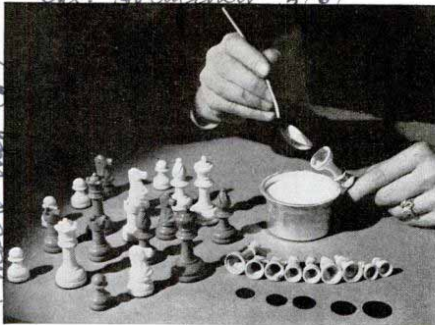
After filling plastic shells of chessmen with ballast, felt bases are applied
