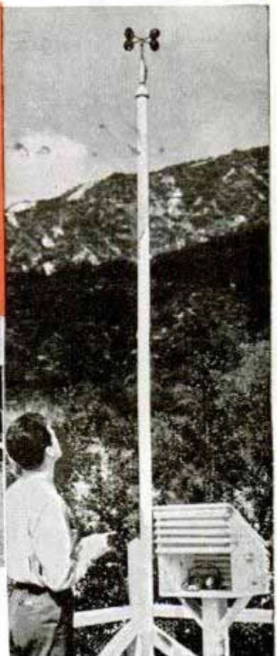
Forest service radio truck with collapsible mast, top, used as field base in fighting fires. Below, (left) weighing fuel moisture sticks for humidity; (center) ranger reports progress of fire fighters to headquarters; (right) measuring wind velocity with anemometer in plotting fire danger factors
