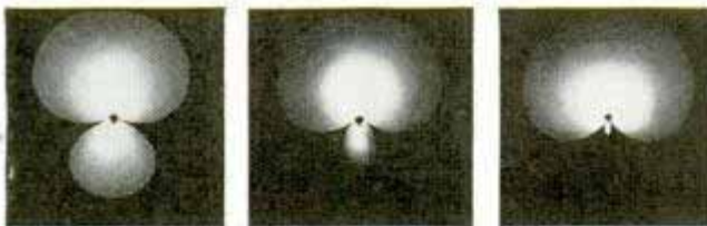
Diagrams indicate by light-to-dark variations how microphone (top) decreases in field of sensitivity
