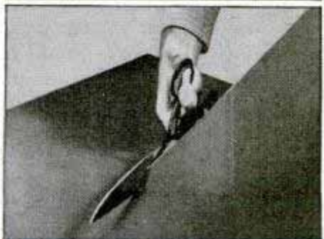
THIN STOCK CAN BE CUT WITH SCISSORS
