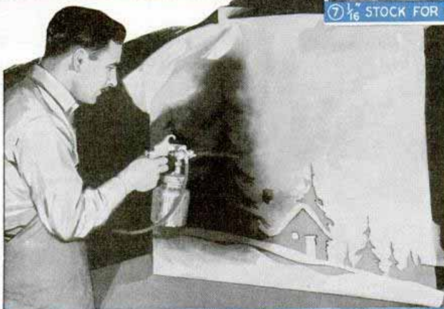
8 THE DESIGN CAN BE SPRAYED, BRUSH PAINTED OR SANDBLASTED
