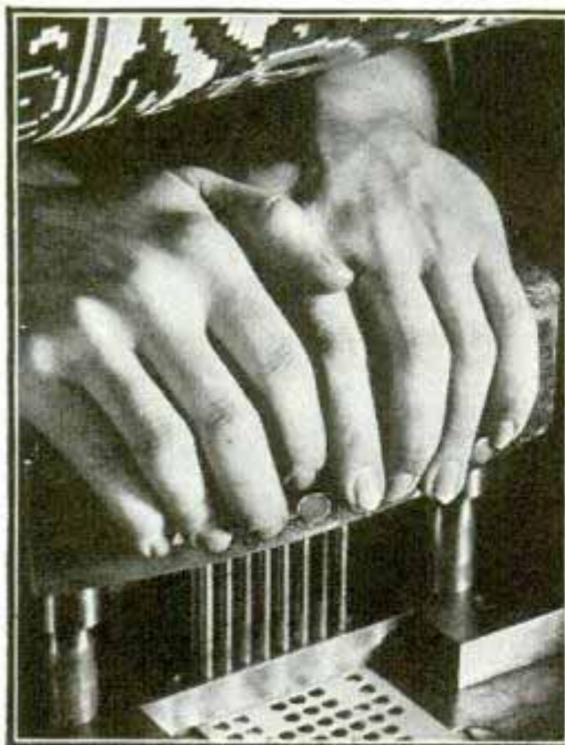
In ancient times a lifetime frequently was spent weaving one rug. Today American manufacturers produce a million pounds of rugs each working day. Above, a card puncher "piano playing" a pattern, translating a paper design into the cards on the loom by pressing keys on the cutter
