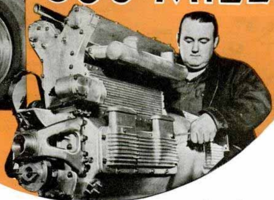
Mechanics check camber and toe-in of a racer's front wheels, top. Below, at left, a new radiator is given a fitting on last year's winning Maserati car; right, new Offenhauser engine for Joe Marks has enlarged crankcase providing more air and better circulation
