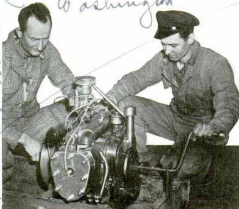
Inspecting speedboat engine, with two opposed cylinders, that was built from used automobile parts at a cost less than $100
