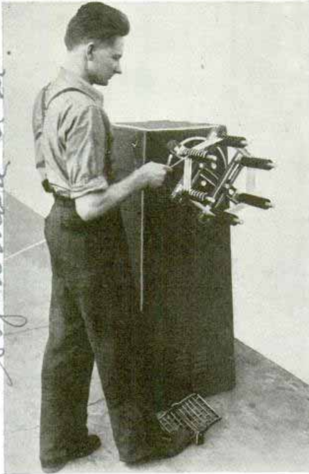
With foot on treadle operator can govern rotation of reel to assure uniform tension of finished coil
