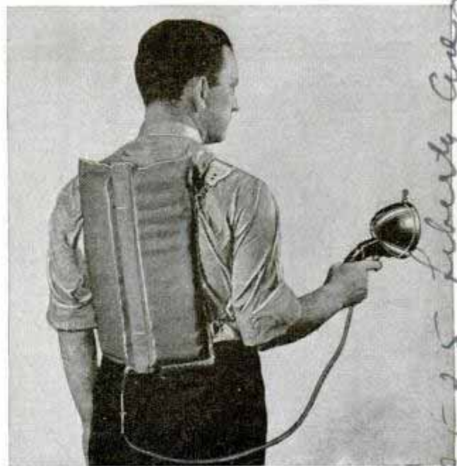
Batteries carried in the back pack have enough power to throw a strong beam over a quarter of a mile
