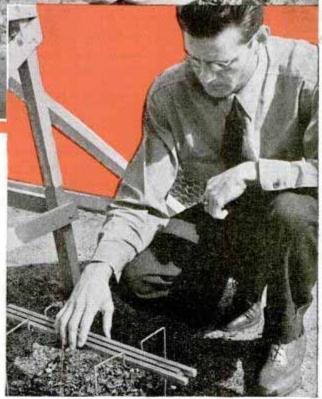
Light bulbs on relief map represent lookout towers and area they light on map is actual range of vision from tower. Below, a ranger places oven-dried sticks on rack to test humidity of air and vegetation
