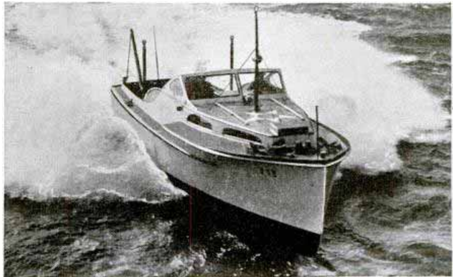
Acme Army rescue boat carries portable derrick and an emergency hospital
