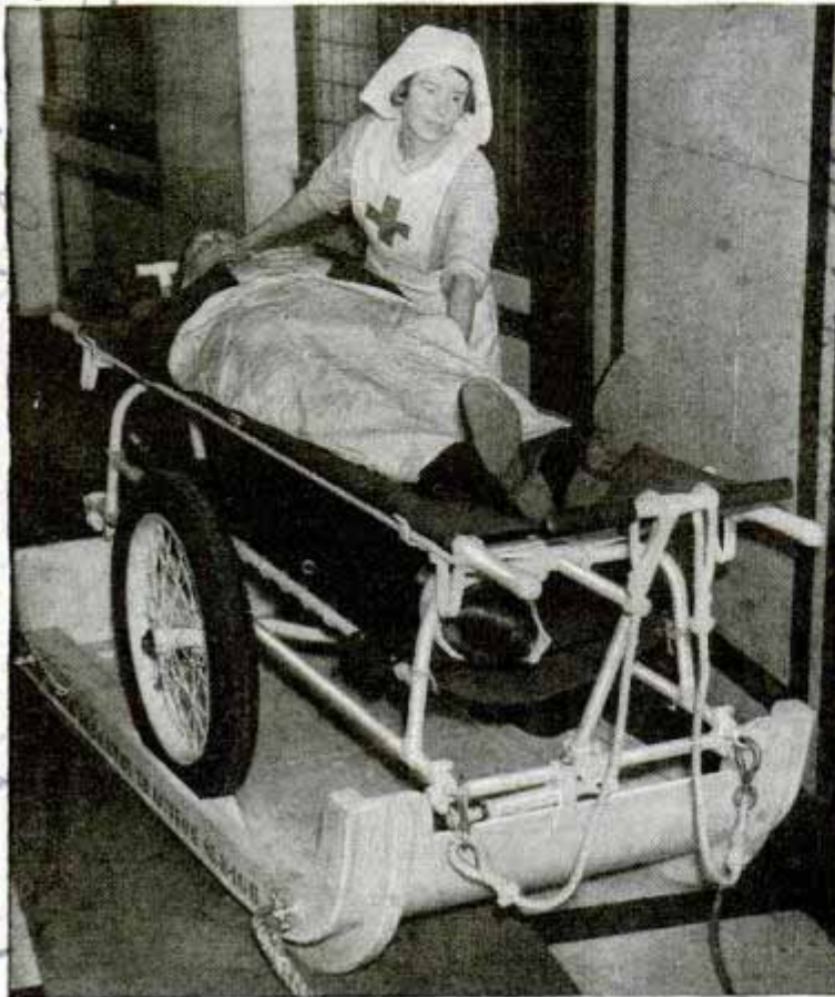
Major Harold Frutberg Frutberg's Infantry Coaction Carriage Double-deck ambulance mounted on sledge glides easily over heavy snow where wheeled vehicle would make slow progress
