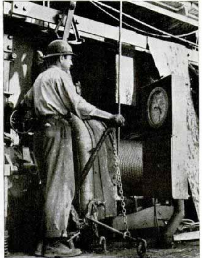
Drill boss at controls by which he governs speed of rotation of drill and weight on drilling bit
