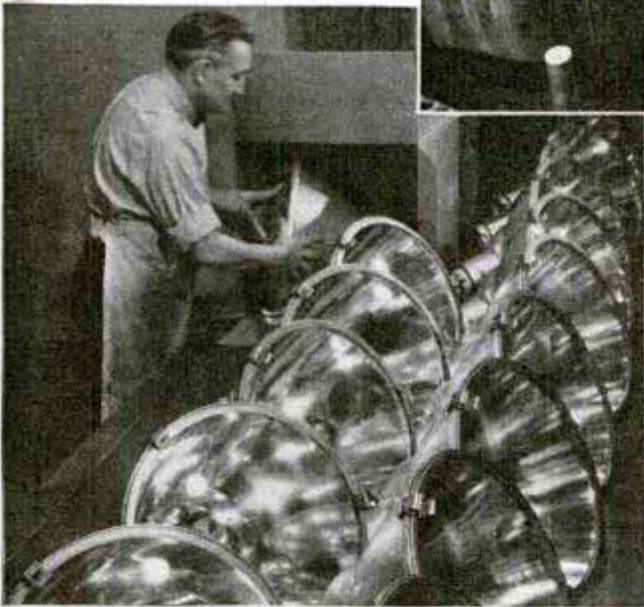
Machinist is mirrored in highly polished surface of aluminum reflector disk, above, being spun in lathe. Left, floodlamps ready to be installed at ball parks
