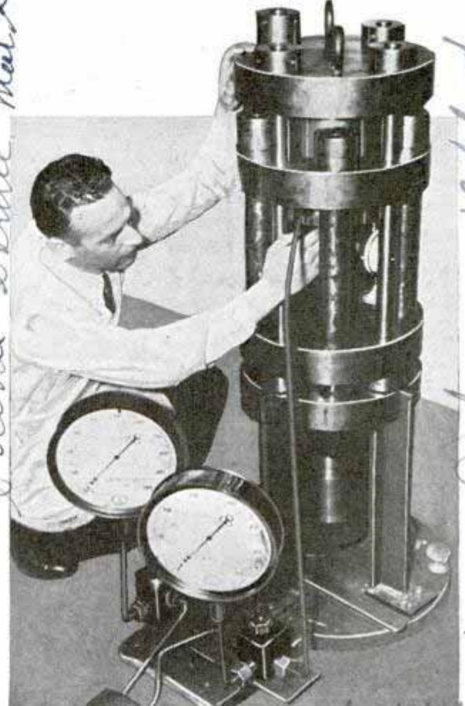
"Cascade bomb" able to produce 6,000,000 pounds pressure gives clue to conditions deep in the earth
