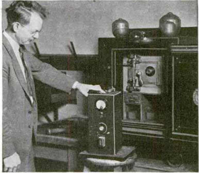
Meter keeps watch over stored radium, issuing a warning of danger if vault becomes "overloaded" or insulation is inadequate
