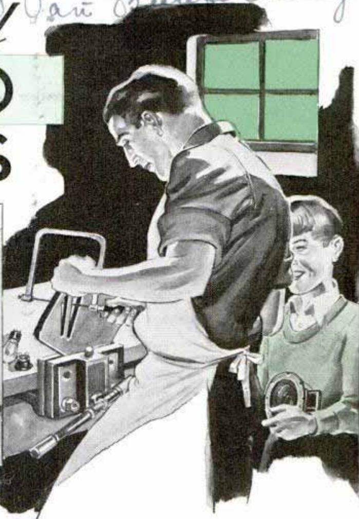
Above, cutting grille opening for front of "speaker-microphone" baffle case; grille is backed with cloth and case is mounted on an old-lamp or "mike" stand. Holes are drilled in rear cover by cut and try method; start with 3 or 4 and increase until natural voice-frequency response is obtained
