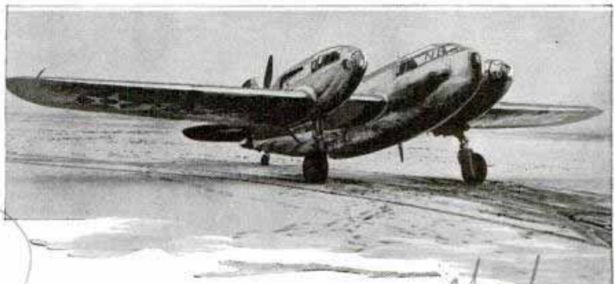
This is called a multiplace army plane because use of pusher-type propellers and engines provide two extra "cabins" for crew and armament
