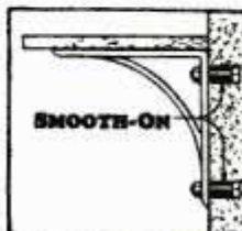
Anchoring in masonry
