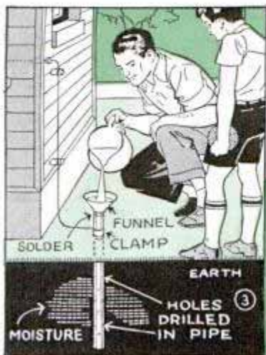
Photo, Fig. 2, shows tiny 5 and 6-prong tube sockets and retainer ring designed for the new "Bantam Jr." tubes now available for portable hearing-aid circuits, pocket-type receivers and compact testing equipment. Fig. 3, tin funnel soldered in end of ground pipe so that water may be added easily as required to provide sufficient moisture to insure a good radio ground in dry, sandy localities where efficient ground connection is difficult to obtain
