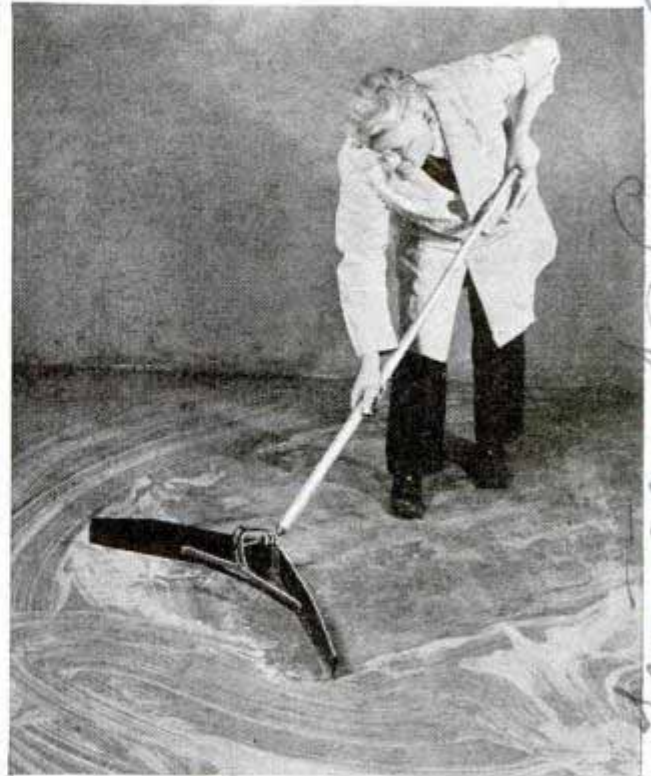
By twisting handle, V-shaped floor squeegee is made to steer itself when working in close quarters
