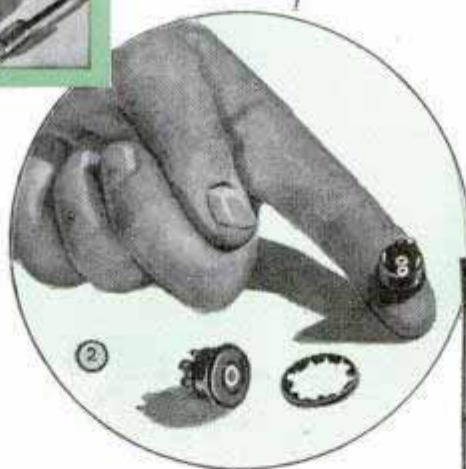
Fig. 4, prongs taken from an old tube base make neat cord tips to fit clips or tip jacks; tin wire, insert and apply heat to prong. Fig. 5, kinks and twists in coil wire quickly removed by pulling wire through prongs of a tube base. Fig. 6, pocket-type dry battery checker and voltmeter tests all dry batteries under load
