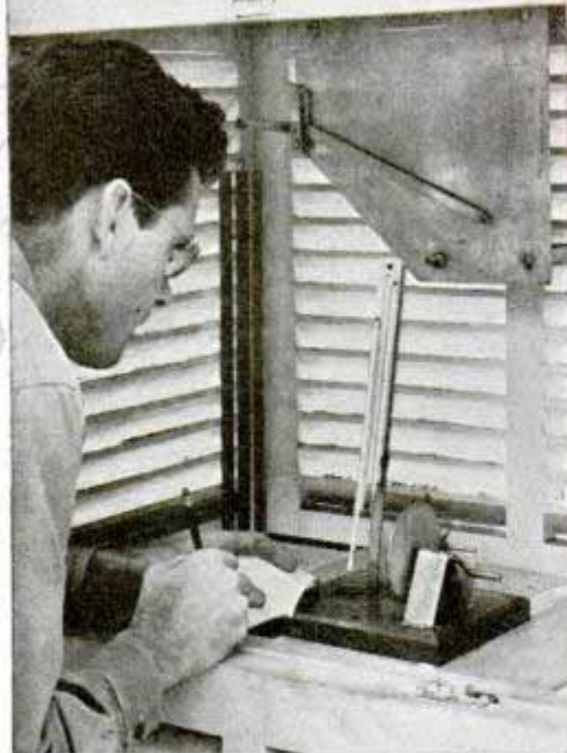
Forest service radio truck with collapsible mast, top, used as field base in fighting fires. Below, (left) weighing fuel moisture sticks for humidity; (center) ranger reports progress of fire fighters to headquarters; (right) measuring wind velocity with anemometer in plotting fire danger factors
