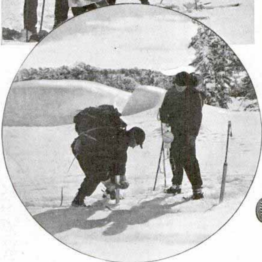
Above, the jointed aluminum tube is thrust deep into the snow to take a sample. In sub-zero cold and blinding blizzard 150 hardy woodsmen of "Snow Patrol" range over hills and 14,000-foot peaks
