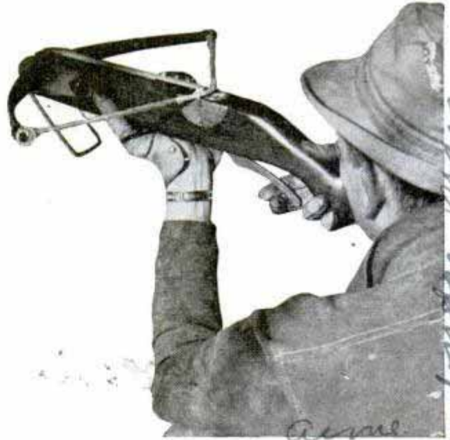
Shoemakers' twine, a billiard ball and an automobile spring went into this homemade crossbow
