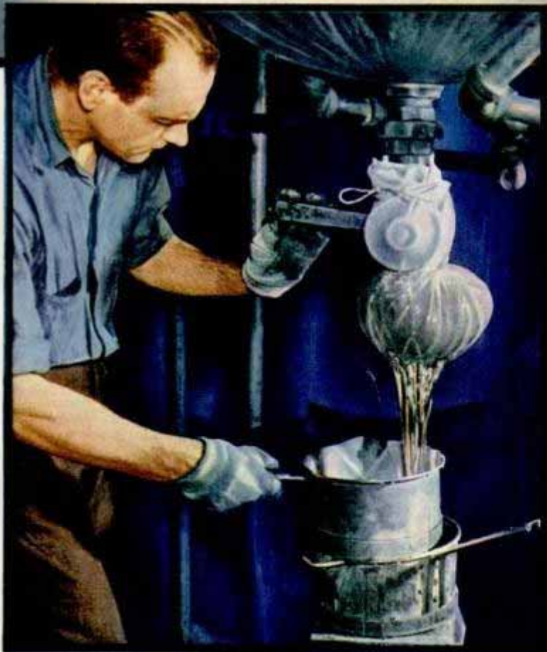
Brooches of Lumarith by Celluloid Corp. (top). Drawing resin from still (below) in Marblette plant. Mottled effects are produced by dipping glass rod into resin of contrasting color, plunging it into kettle resin and swirling it about, leaving trail of oddly shaped veins.
