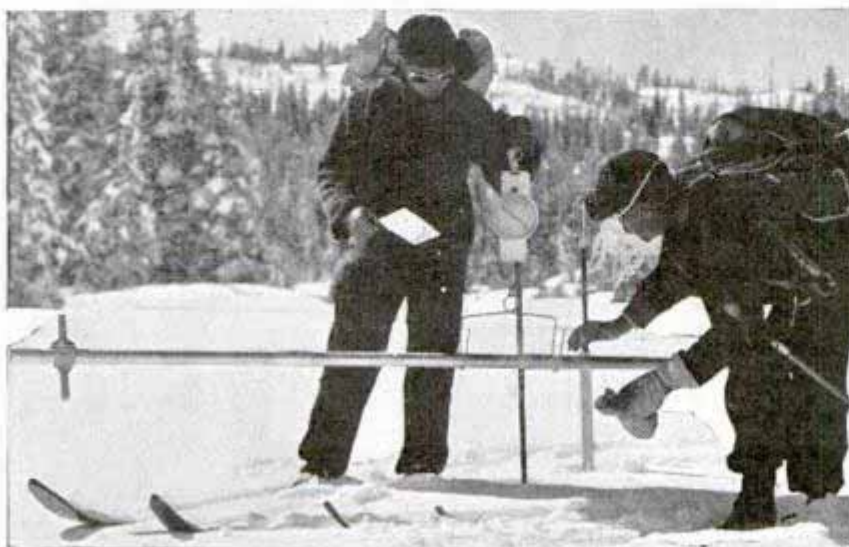
Above, the jointed aluminum tube is thrust deep into the snow to take a sample. In sub-zero cold and blinding blizzard 150 hardy woodsmen of "Snow Patrol" range over hills and 14,000-foot peaks
