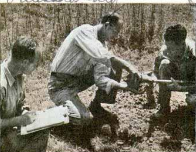
Geochemists, above, transfer a sample of subsoil from auger to jar for analysis. At left, hard facing the teeth on self-cleaning rock bit cones. The cutaway model of an oil field, below, demonstrates how wells reach oil from deposits separated by a fault
