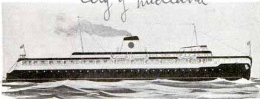
Passengers enjoy all modern conveniences and comforts on this car ferry designed to transport thirty-four freight cars as well as 100 automobiles
