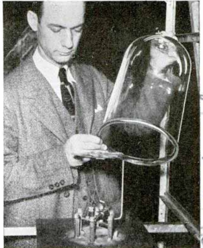
White Water Metal fluorides evaporated in jar coat lens surface
