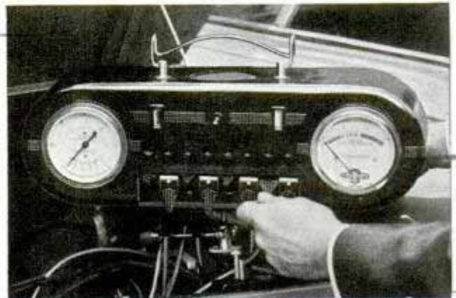
Analyzer reports condition of engine and electrical system, and also frees sticking valves with solvent
