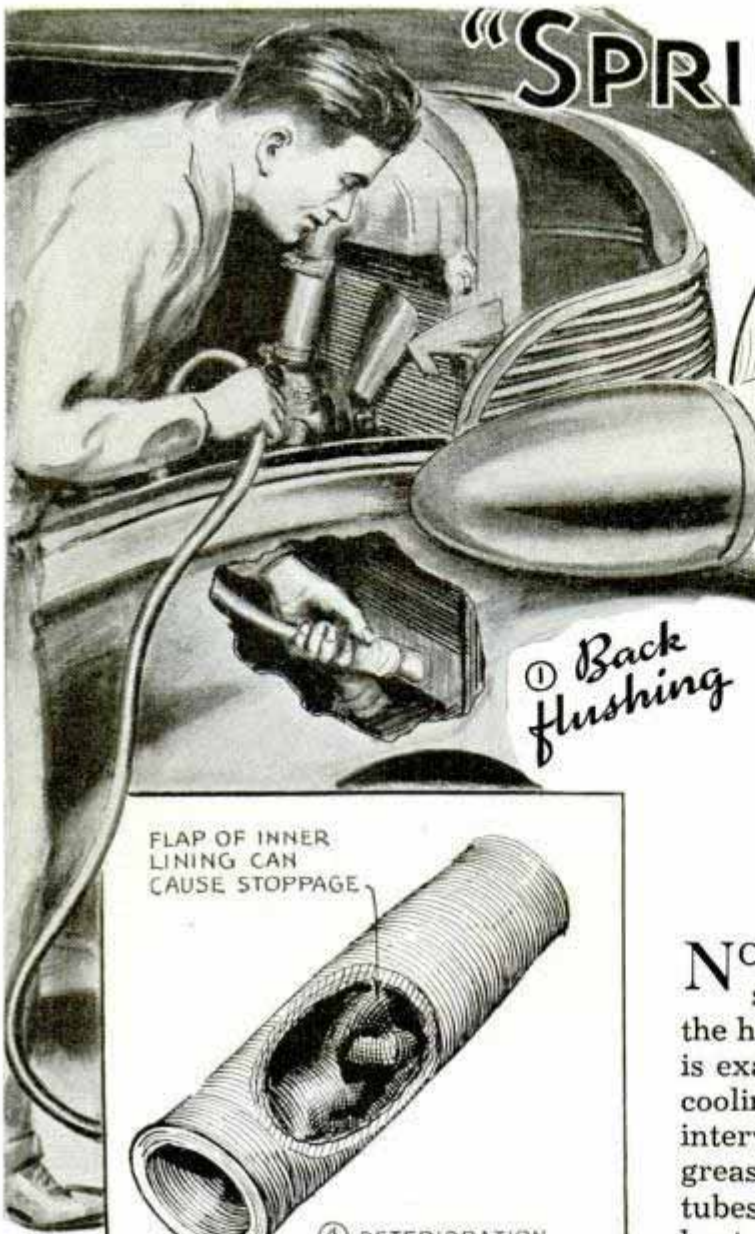
④ DETERIORATION OF WATER HOSE
