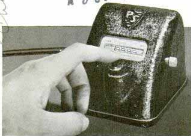
Direct-reading electric stop watch shows time in tenths of a second. Push button starts and stops it
