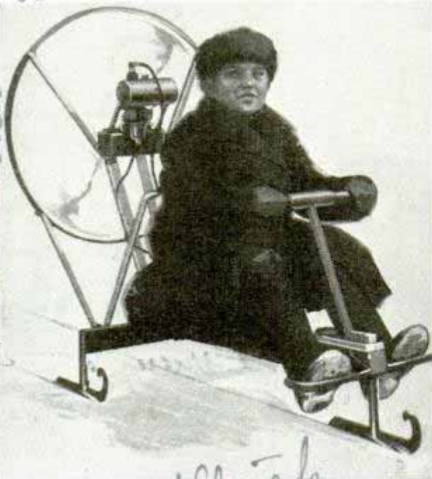
all in one Light engine and air propeller push "aerosled," made with skate runners by school children in Russia
