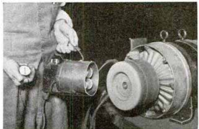
Counting revolutions of shaft under neon stroboscope gives slip speed for computing revolutions of motor
