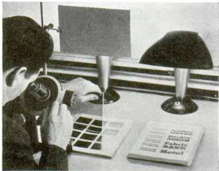
Holding Polaroid screen between glaring lamp and book, at left, restores visibility. Lamp fitted with screen is shown at right
