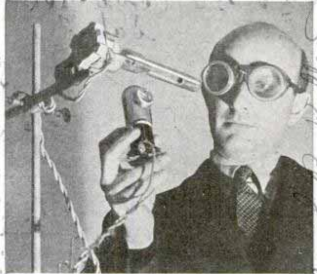
Holding tube that measures output of germicidal lamp
