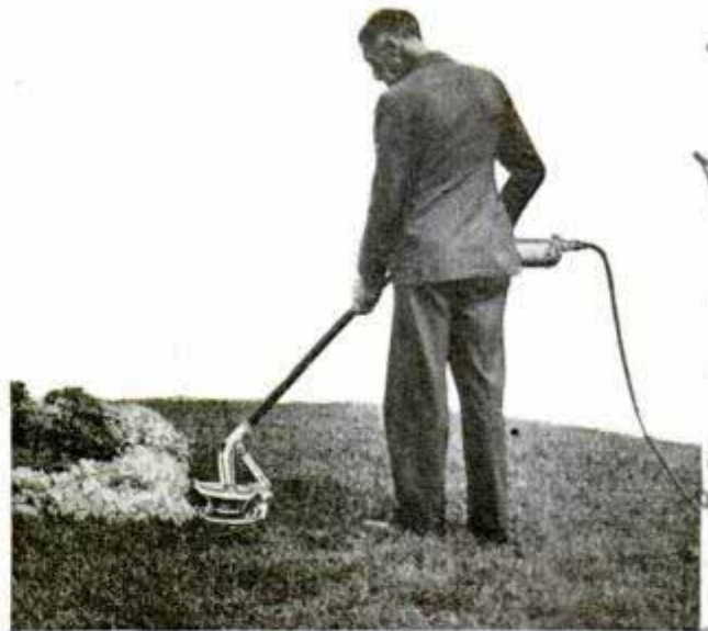
Air suction helps this electric lawnmower draw grass into its cutters when trimming lawn near obstacles
