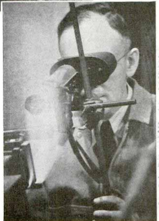
Qualities of a metal are determined largely by what is mixed with it in foundry stage of production, top. Below, measuring with a pyrometer the temperature in an electric furnace used for production of sintered alnico
