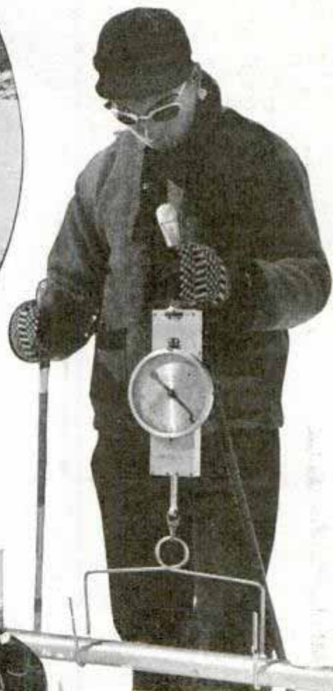
At left and above, the tube filled with snow is weighed on a specially calibrated scale with a simple bent-rod hanger. The reading is immediately recorded, and from hundreds of records taken over the mountains an accurate estimate is made of the flow that will be available for irrigation next summer. The apparatus is easy to carry and simple to operate
