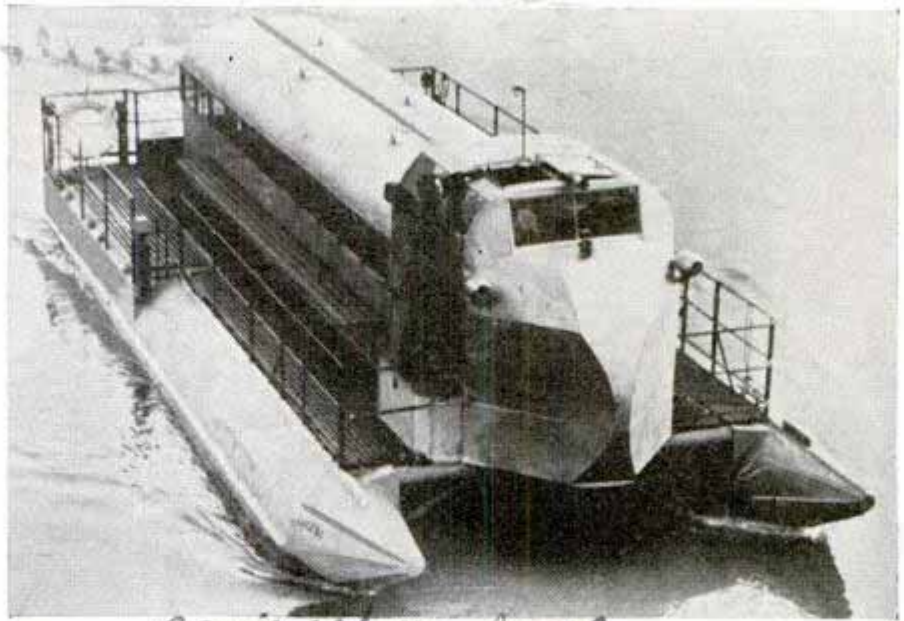
Watertight cells built into the two pontoons will retain enough air to keep the cruiser afloat even if half of their compartments become flooded
