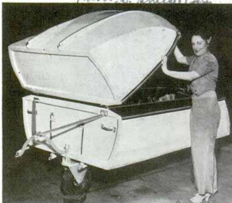
By folding bow over stern this boat is converted quickly into trailer for convenience in towing it to and from the water
