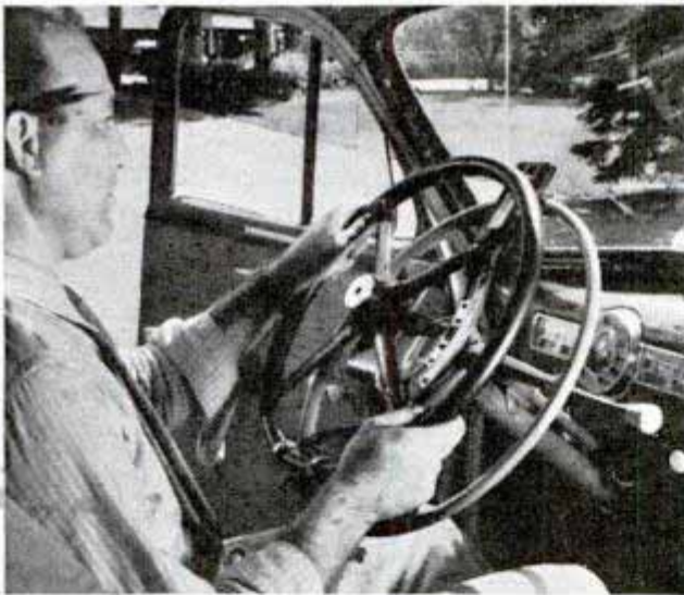
Gauges installed on steering wheel and other driving levers record amount of energy expended by motorist
