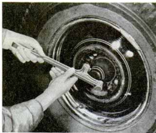
Tool applies leverage for easy removal of grease cap, and hub cap is lifted by inserting other end under rim
