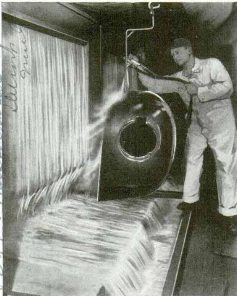
Man-made Niagara carries away fumes and particles of sprayed enamel. Note fog being blown from fender toward water curtain
