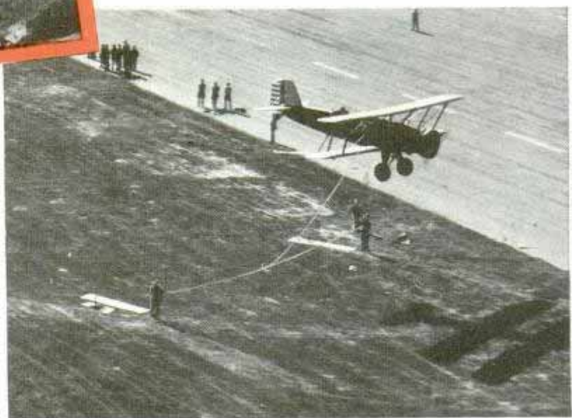
Top, throwing out message tied to streamer that burns colored light at night. Center, laying out message panels so observer aloft may read them. Bottom, plane picking up message with grapple hook from rope supported by uprights held by men on ground
