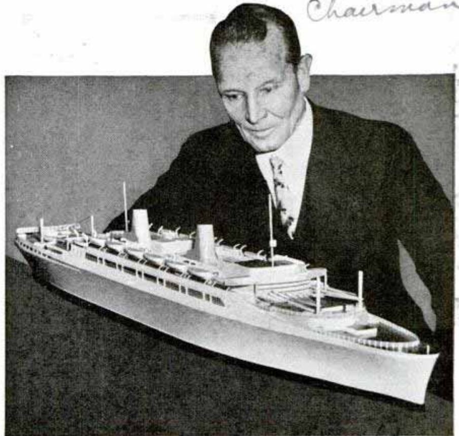
Model of luxurious ocean liner that is designed for ordinary travel or carrying cargo, but can be converted into an airplane carrier if needed
