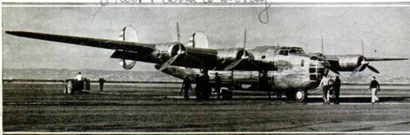
Bomber for United States army has a carrying capacity of four tons of bombs, and a total of 4,800 horsepower makes it capable of speeding more than 300 miles an hour and permits cruising range of 3,000 miles
