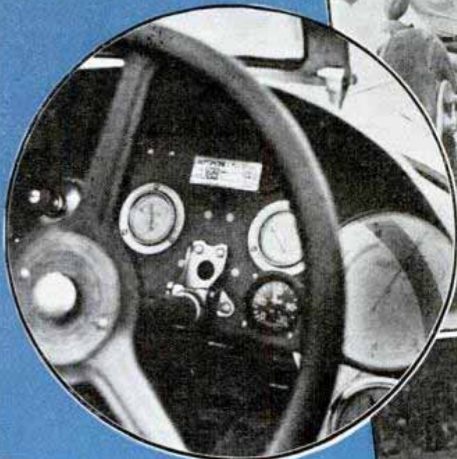
Circle, instrument panel of racing car. Large dial at right gives engine revolutions in thousands per minute. Top, working over Maseratti car in Indianapolis pits
