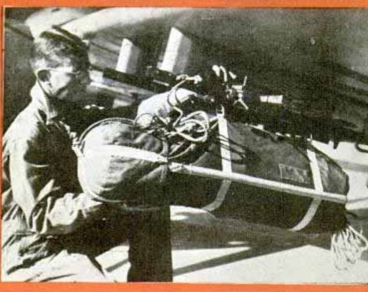
Top, left, observer, oxygen tube in mouth, looking through bottom of fuselage. Right, looking downward from above observer. Center, firing at sleeve target. Bottom, strapping parachute food container to bomb release mechanism
