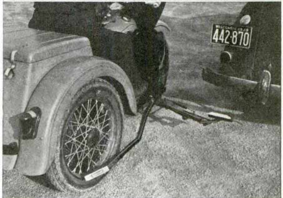
Right, top, long extension arm swings out to mark tire of car parked at forty-five degree angle, while the twenty-one inch arm, bottom, will reach auto parked parallel to curbing
