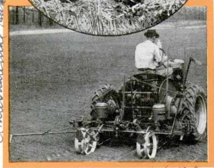
Farmall B Low-slung truck, top, handles bales as they are bound, saving an extra pick-up. Center, one of the new light, three-wheeled tractors operating one-row corn binder. Two-row checkrow corn planter at bottom can cover twenty to thirty acres a day
