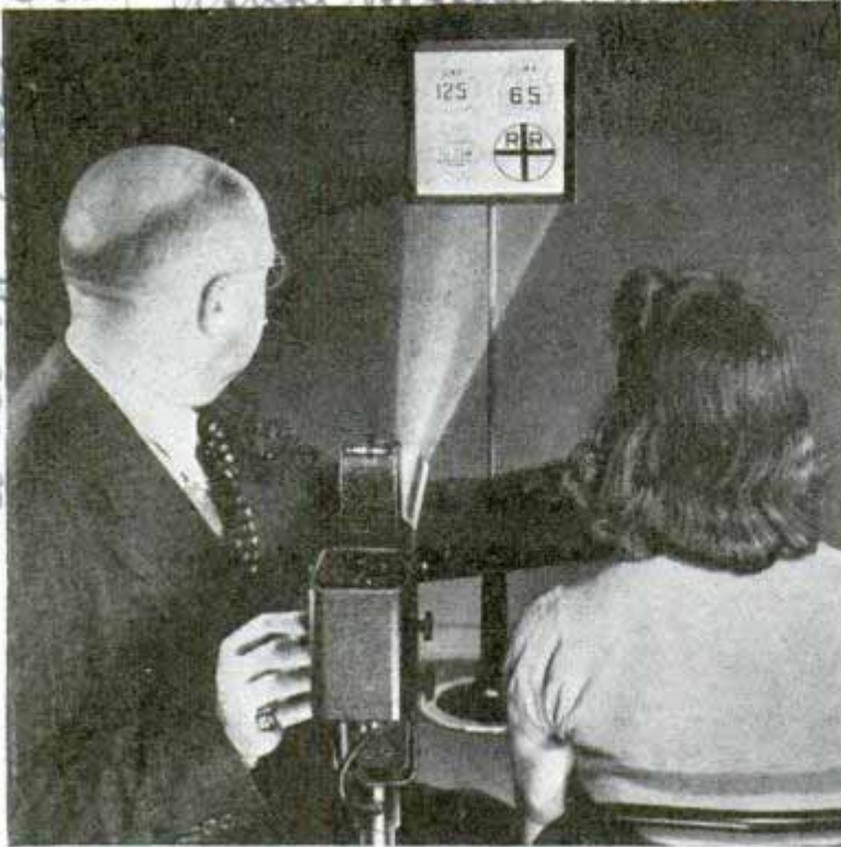
Road signs are projected on screen to test vision of drivers instead of using the customary chart that can be memorized
