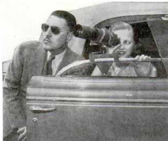
Motorist uses telescope from auto in comfort, with instrument mounted on support that fits window
