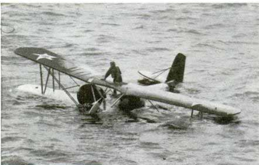
As soon as this land plane hit the water, rubberized water wings automatically filled with carbon dioxide which could keep it afloat nearly a day
