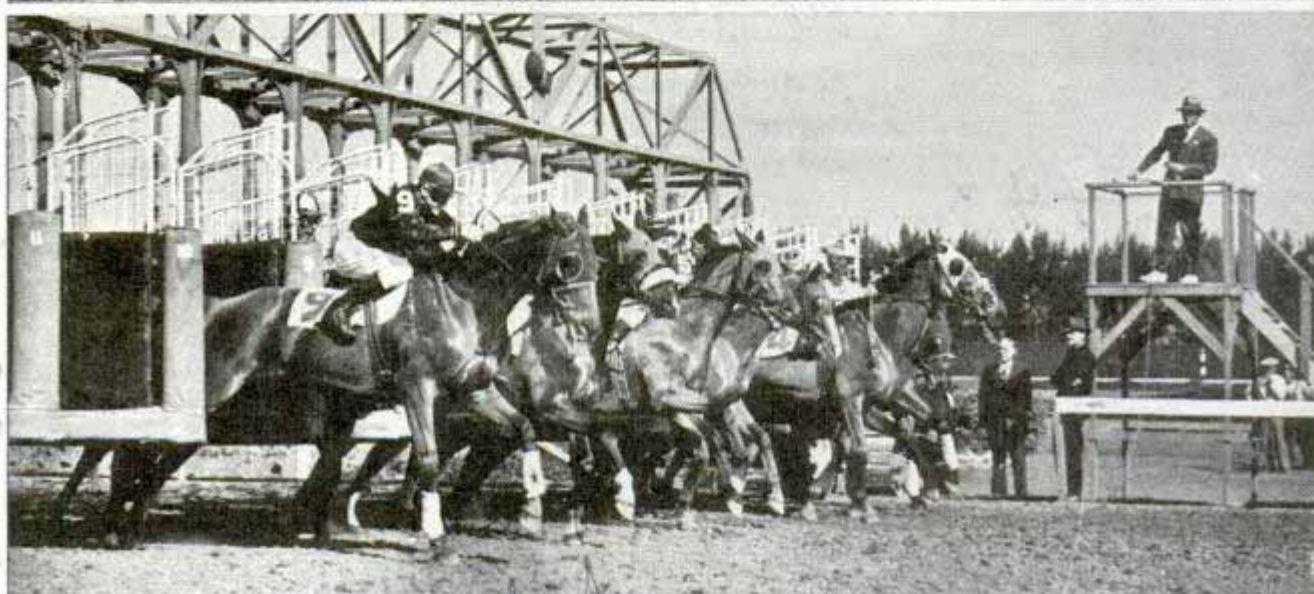
Top, race horses locked in magnetic gate cannot jostle their neighbor if they become restless. Below, they're off to a fair start as soon as starter presses switch that opens all gates at one time
