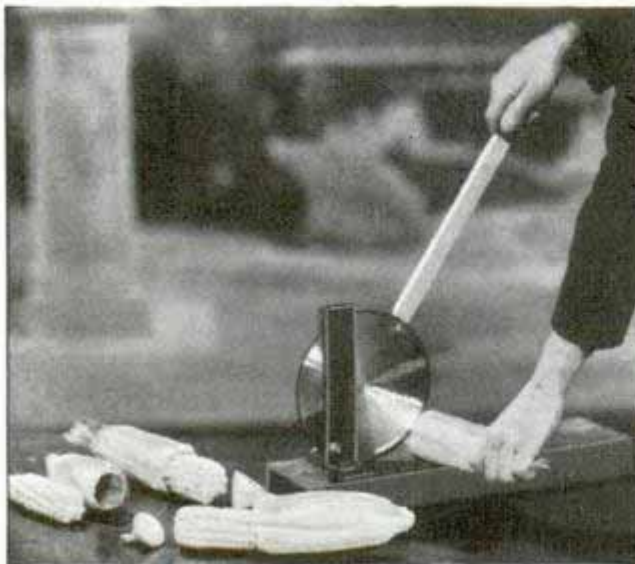
Knife severs hull at base for quick and easy shucking
