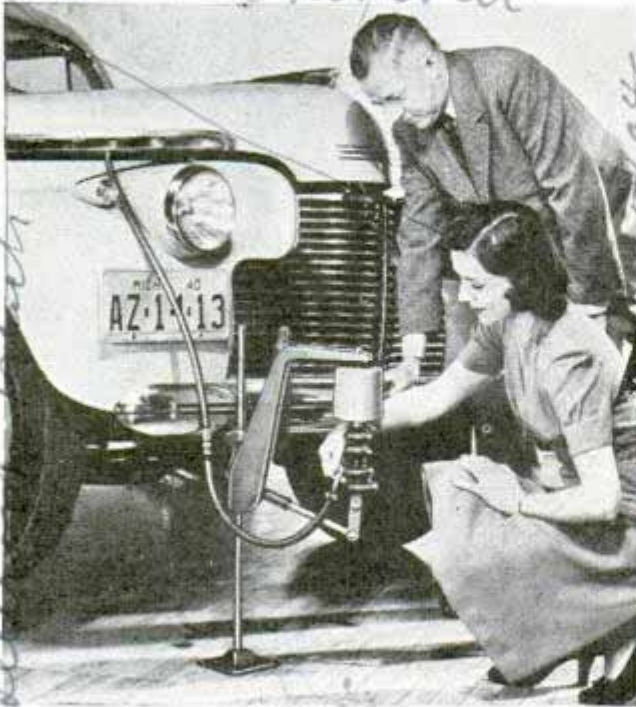
21482 Cylinder used for shifting gears, connected by tube to engine, is shown jacking up car by vacuum power
