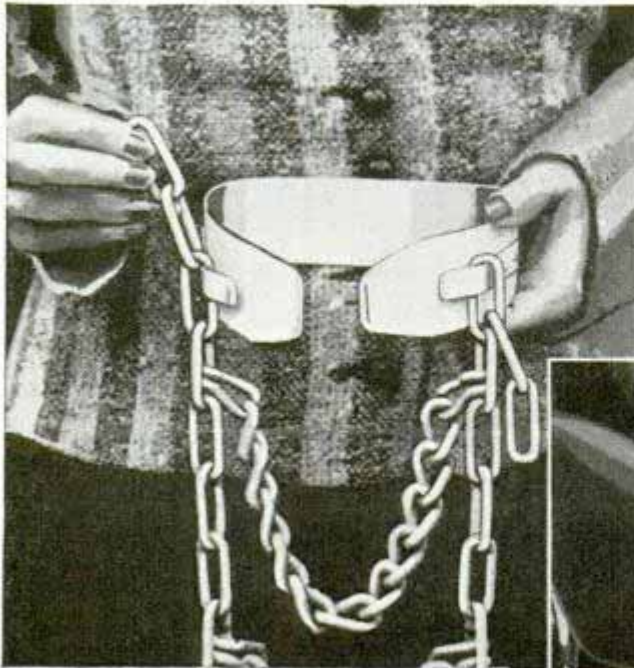
Above, holding spring clamp with tire chain hooked on clips. When chain is straightened out as at right, wheel will pick it up when car moves forward, wrapping it around tire so it may be locked easily
