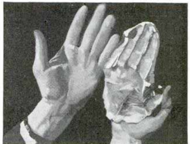
el ll Above, the spray gun and some of its accomplishments: filling dented automobile fender, coating plaque and covering lathe-turned wood with metal. Below, reproducing hand prints in metal
