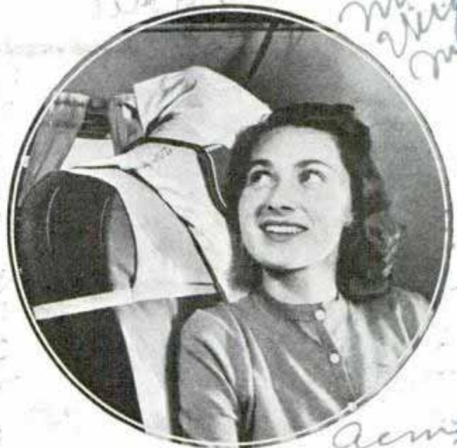
Radio speaker in form of pad, resting on back of seat, permits individual passenger to hear program
