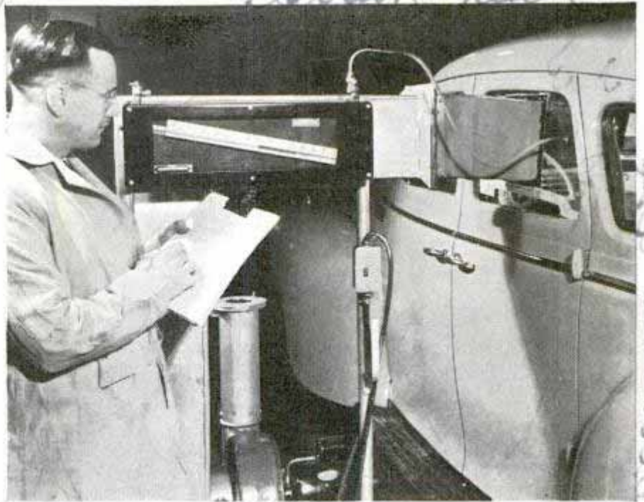
Checking auto body seal against drafts. When air is drawn out vacuum gauge tells at a glance whether too little or too much air leaks into car
