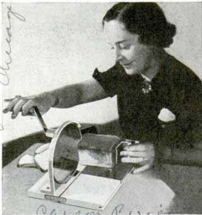
Bread being sliced to uniform thickness on hand-operated slicer that will cut meat, fruits or cheese
