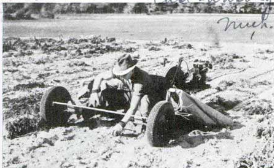
Potato picker sits near ground on powered crawler where he can reach potatoes turned up by digger and load them into bags at right and left sides
