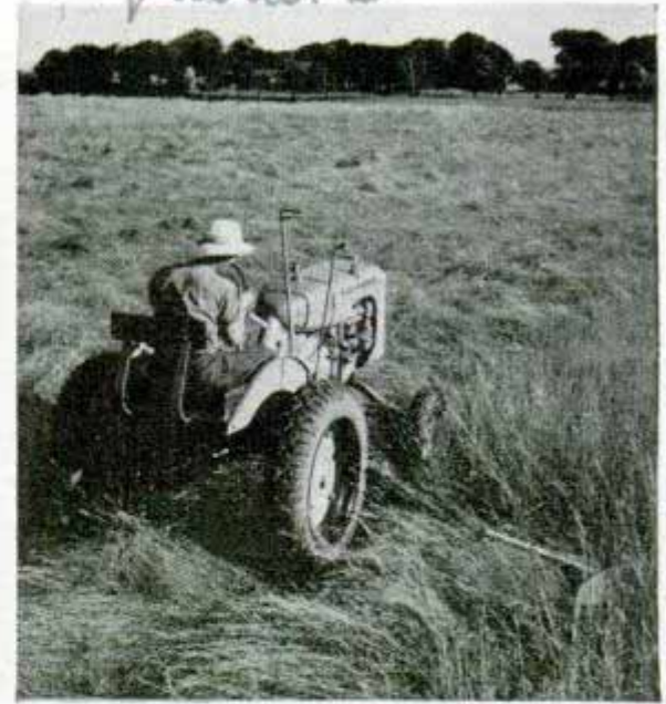
Left, field pick-up baler cleans field and stacks crop speedily. Right, five-foot mower which attaches to tractor in a few minutes. Bottom, forty-inch harvester operated from power takeoff of small tractor
