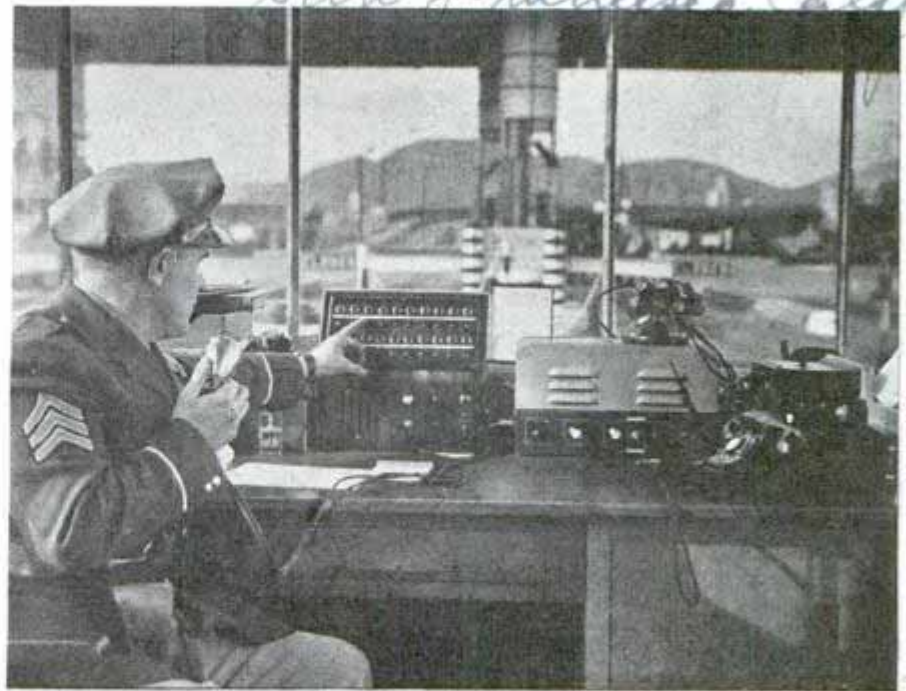
"Traffic dispatcher" in bridge control tower talks through "mike" to any toll station or directs cars by issuing orders through loud speaker
