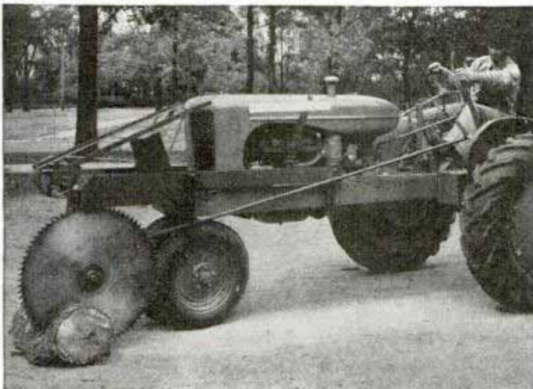
Tractor-powered saw cuts tree logs where they fall
