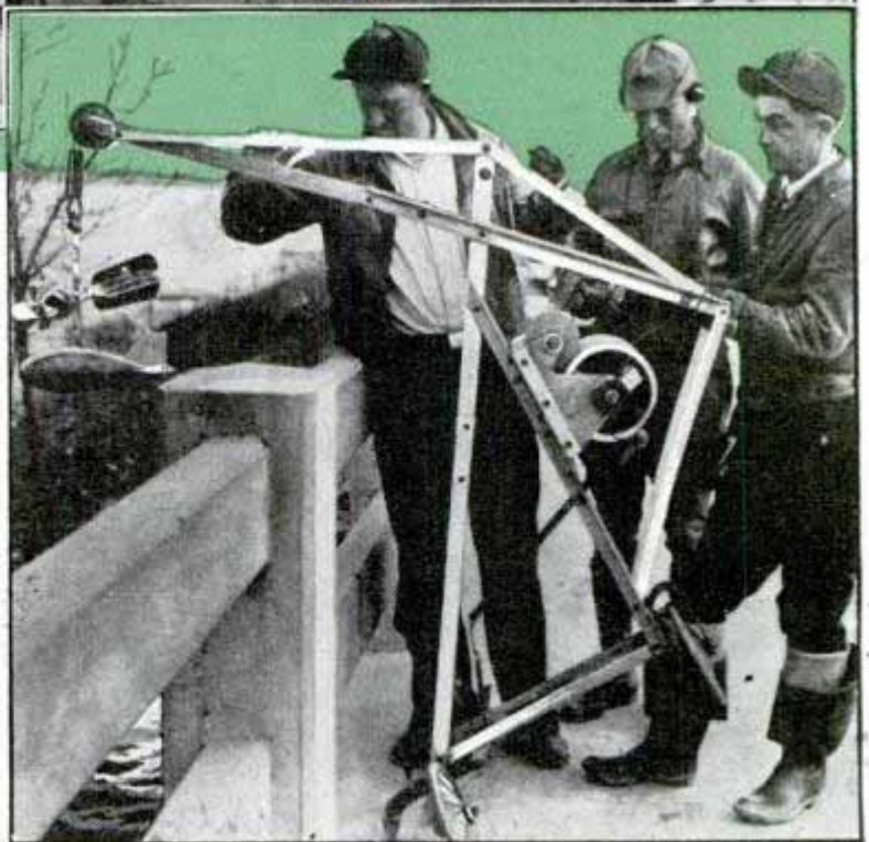
Flood besieges Huntington, W. Va., top; circle, portable communication set; below, measuring river depth and velocity
