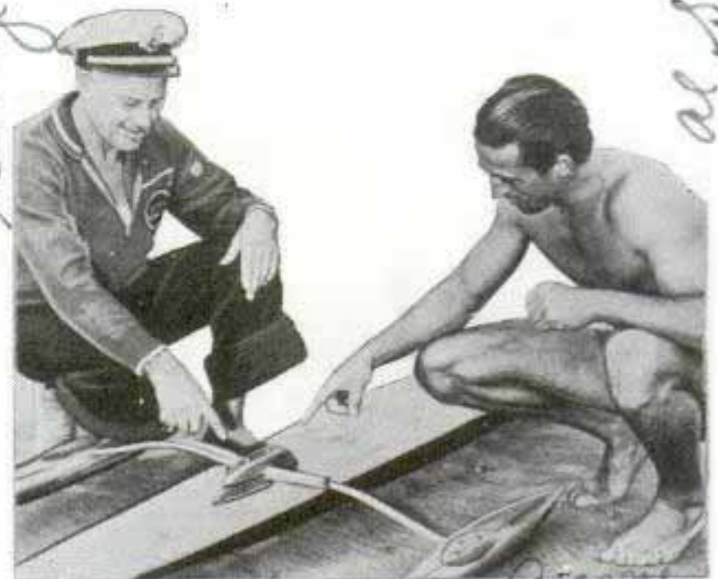
George Watkins Outriggers mounted on paddle board give stability to the narrow float and keep it from turning over
