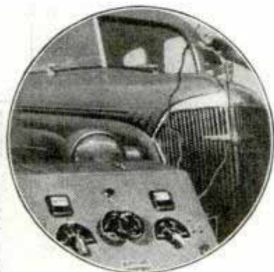
This new portable electro-plating outfit plates on the spot, where article is located. No dismantling.
