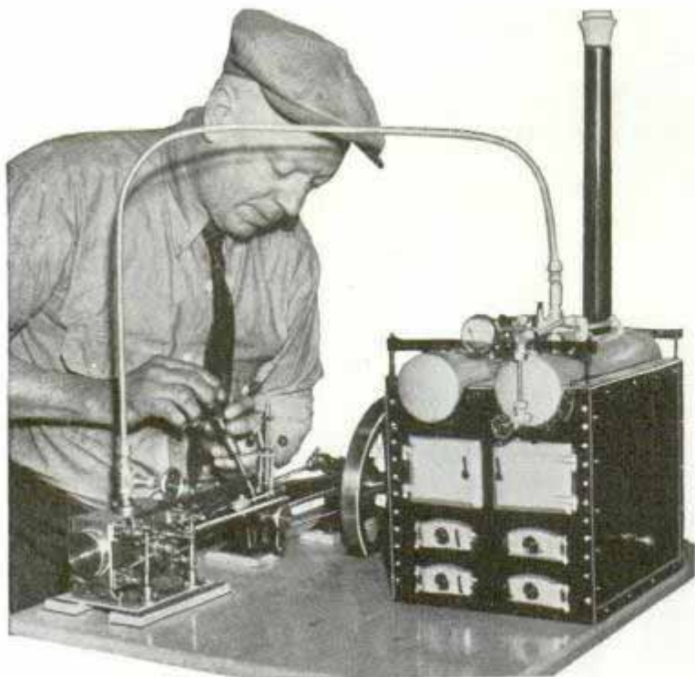
This scale model of boiler and steam engine was constructed in four months of spare time from odds and ends in machine shop
