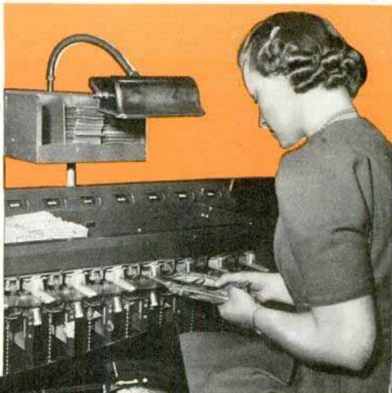
Paper money is sorted into various compartments of automatic currency counter, above, according to type of bill and issuing bank; dial above each bin shows the total. The meter is so delicately adjusted it will refuse two bills fed in at once. At left is the alarm and guard signal panel in police headquarters of Chicago bank. Below, guard turret overlooking banking floor
