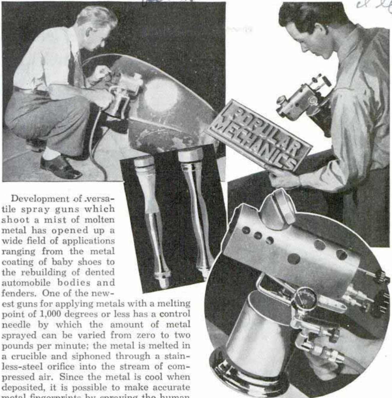
el ll Above, the spray gun and some of its accomplishments: filling dented automobile fender, coating plaque and covering lathe-turned wood with metal. Below, reproducing hand prints in metal
