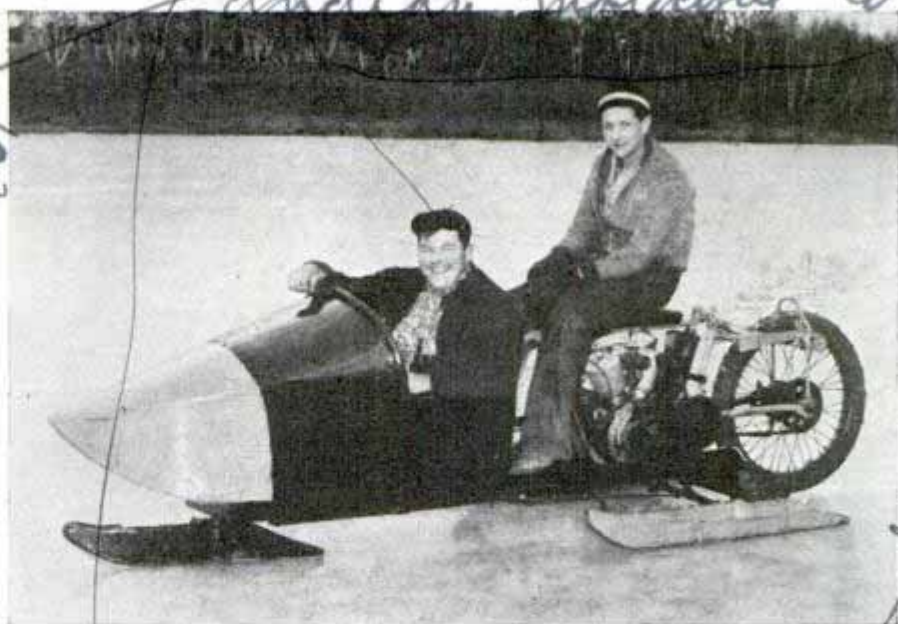
Motorcycle engine and spiked rear wheel give the builders of this iceboat a fast, thrilling ride. Streamline cockpit in front cuts wind
