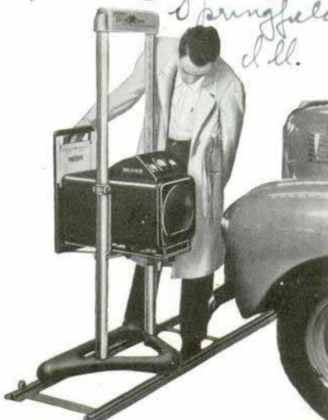
Condition of auto headlights is read on three dials of instrument that scans beam pattern with photocells
