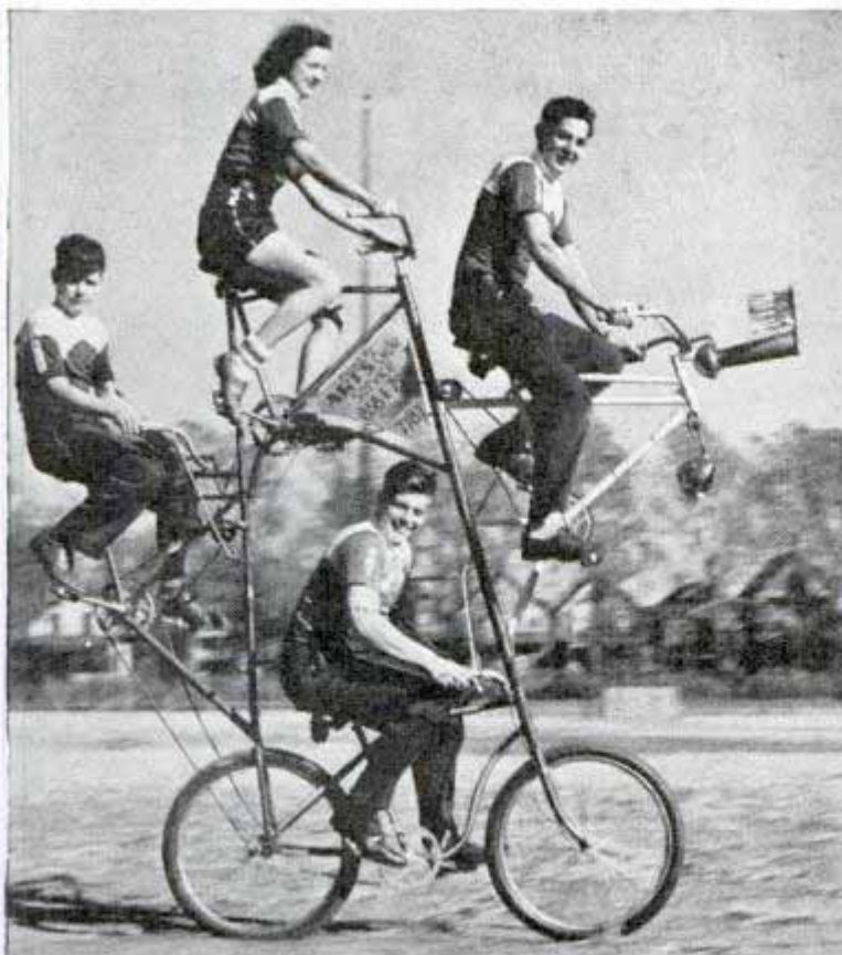
Four-passenger bicycle, ten feet high, is pedaled by all through series of chains and sprockets, and top rider does the steering
