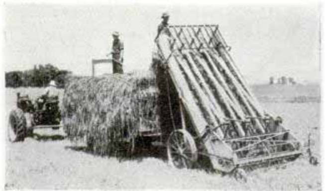
Loading grass silage immediately after cutting; sturdy loader is needed when crop is green
