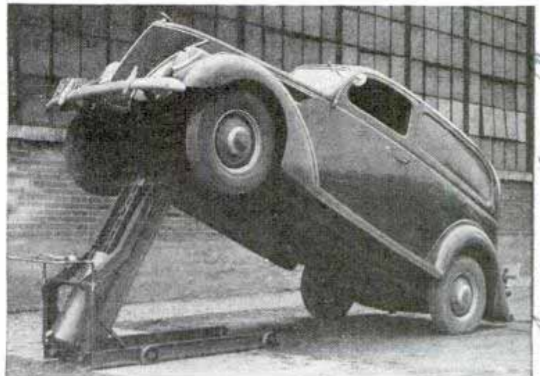
Powerful air-jack raises front end of car for inspection or repair
