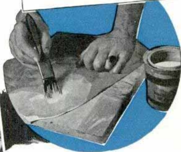
Closely woven cloth may be waterproofed with one coat, while several coats may be applied to make rubberized sheeting
