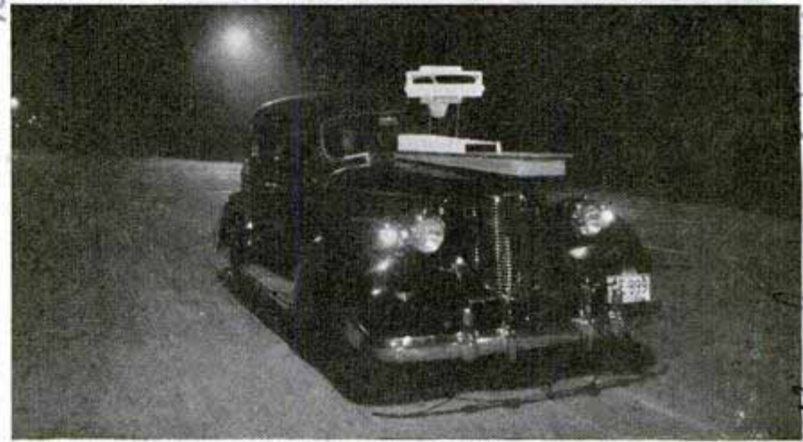
Top, note figure on miniature "street" directly above headlight lens; "eye" over windshield measures glare. Bottom, making street-light test
