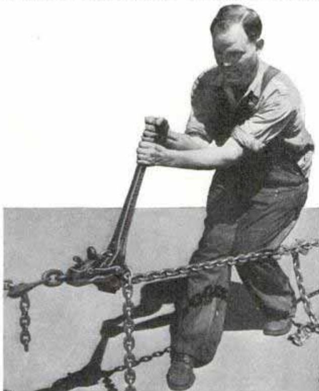
More than three tons can be lifted by one man with aid of lever and chain "jack" that has many uses
