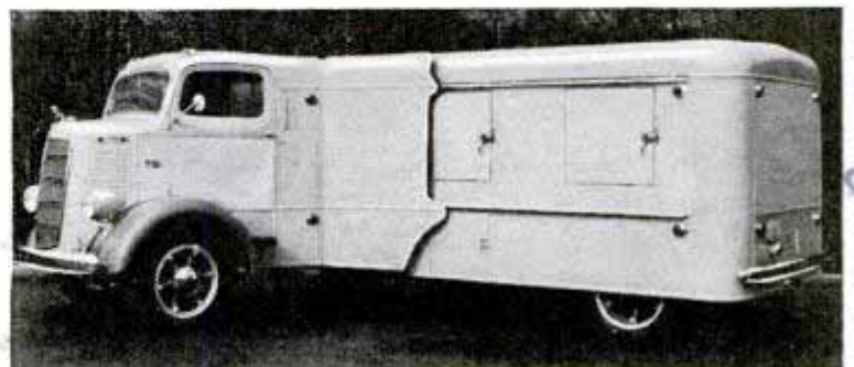
Open space between tractor and trailer is concealed by "wings" at the sides, which slide along body when vehicle makes a turn
