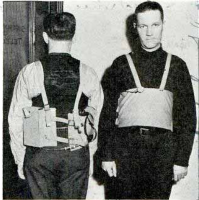
Rear and front views of two-way radio. Transmitter and receiver hang on right side, batteries on left
