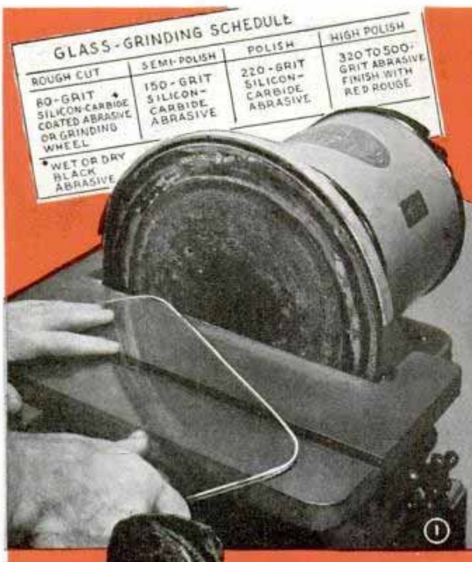
Polishing is done with silicon-carbide abrasive. For the last stage use red rouge (above), which is then washed off with muriatic acid (below)
