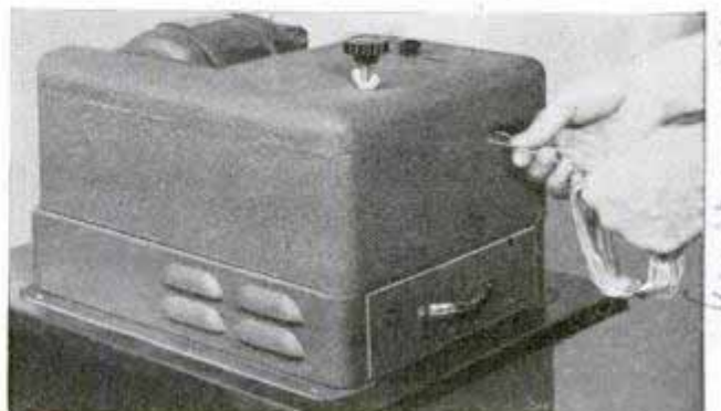
Drawer catches insulation waste stripped from wire
