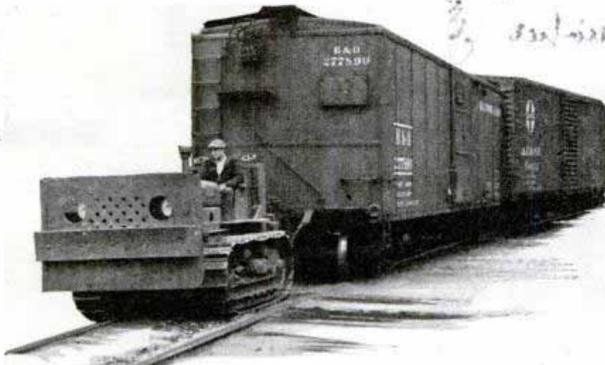
Needing no rails, tractor hauls freight cars in yard operations and can move to next track to pick up another string without using switches
