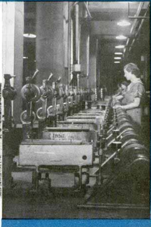
Top, boring diamond dies for drawing tungsten wire; right, 4,000,000-pound hydraulic press; below, fine tungsten wire stronger than steel is drawn from reels at left through gas furnaces and diamond dies
