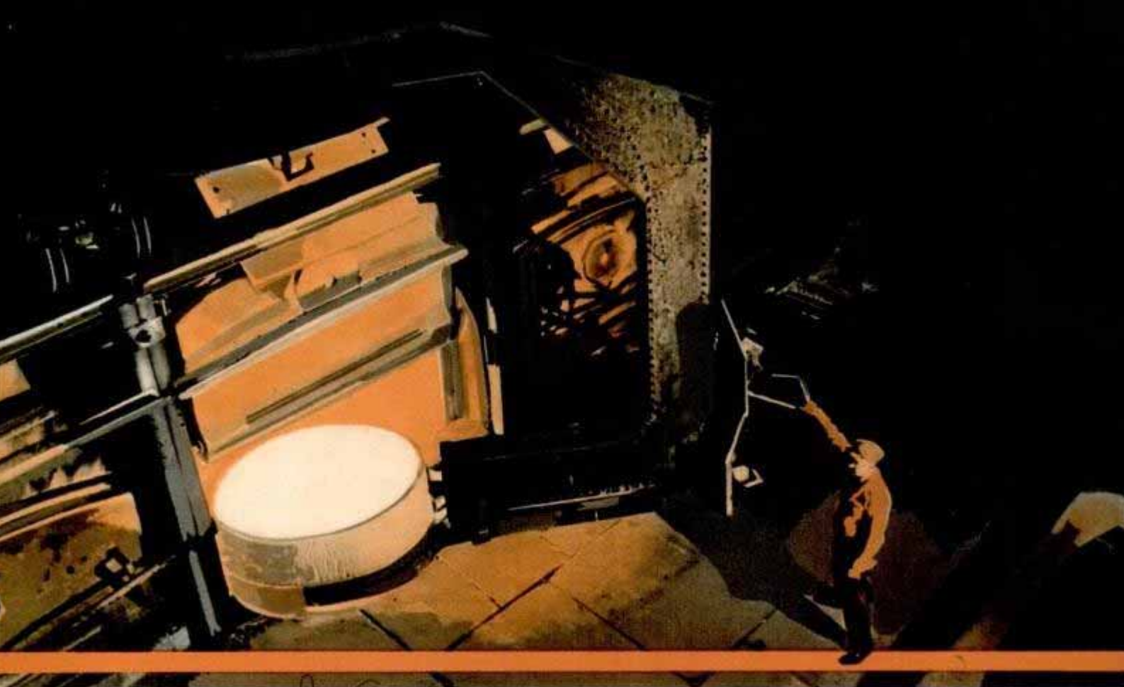
Claw of steel, operated by overhead crane, reaches into oven for pot of white-hot glass after terrific heat has fused ingredients into a molasses-like liquid.
