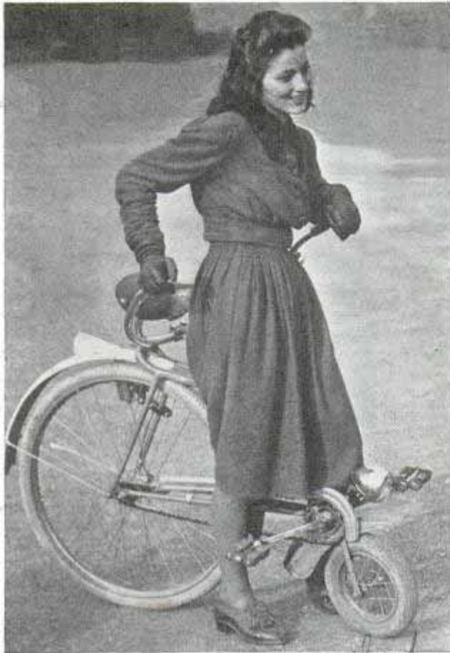
Bicycle with small wheel in front and handlebars mounted beneath saddle is easy to mount and control
