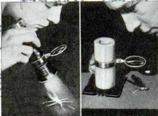
Magnifier that clips on flashlight can be mounted on stand, as at right, to leave both hands free
