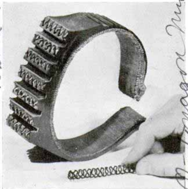
Corrugated spiral wire in foreground is imbedded in tread of tire to grip ice when car tends to skid
