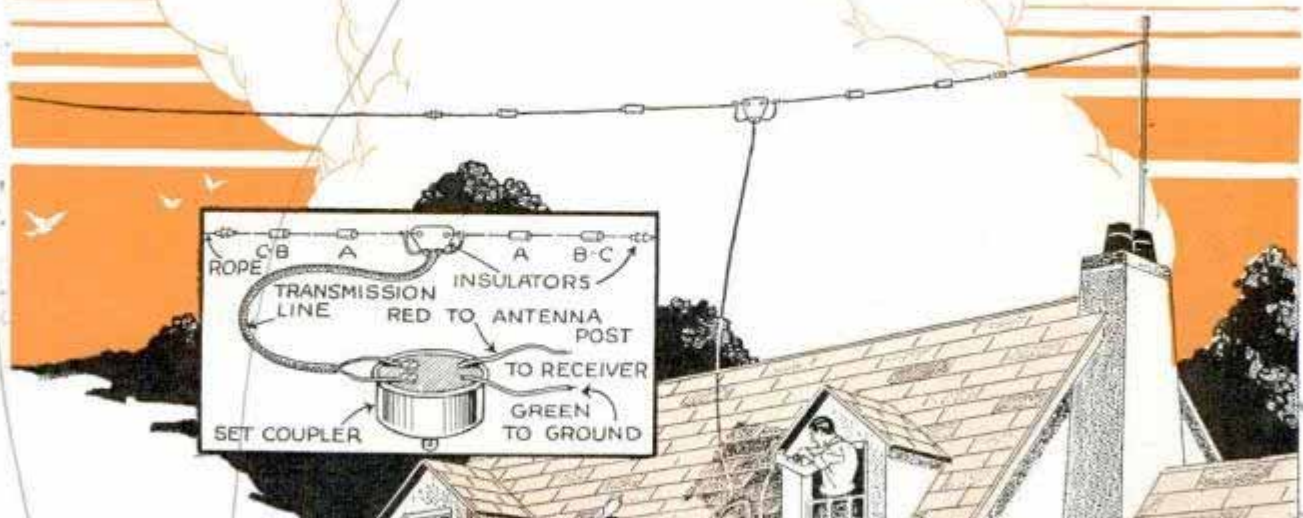
Photo Fig. 1, and sketch above, show a peak-band doublet kit antenna system specially designed for maximum efficiency in the 10, 20 and 40 meter bands. Traps A and combination trap and loading coils B-C are weatherproofed
