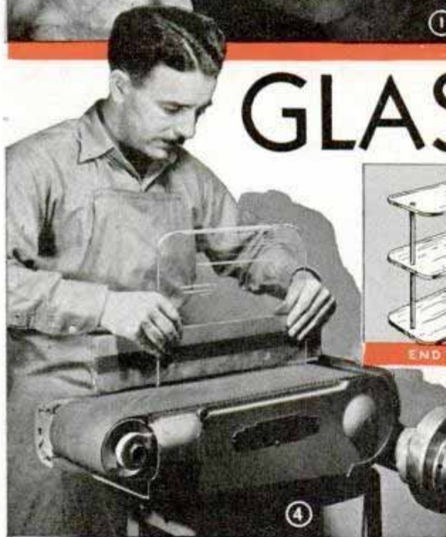
Glass edges can be ground smooth on common shop equipment. Below, running in a border with a small silicon-carbide wheel mounted in the drill-press chuck
