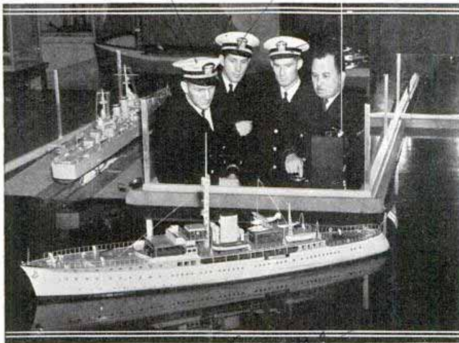
Left, radio-controlled boat responds to orders transmitted by short-wave impulses. Below, operating new telephone dial that is used for selecting the proper impulses to send in executing any given maneuver
