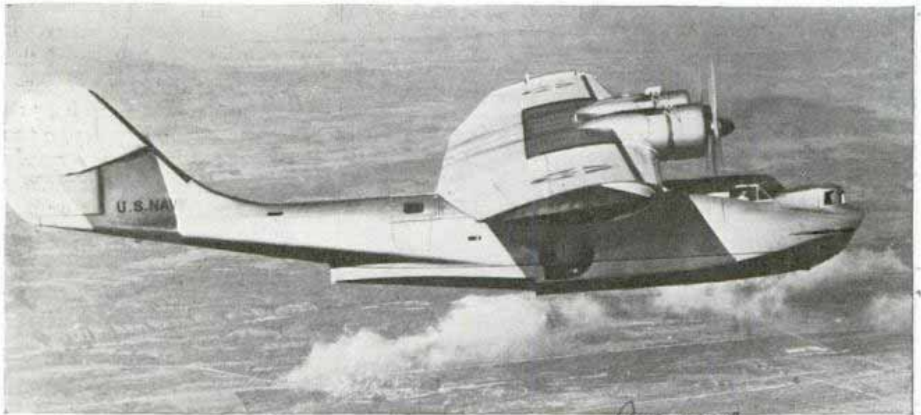
acme Efficient on land and water alike, the navy's new flying boat is equipped with tricycle landing gear which can be lowered in water for beaching on sloping shore without aid of outside crew
