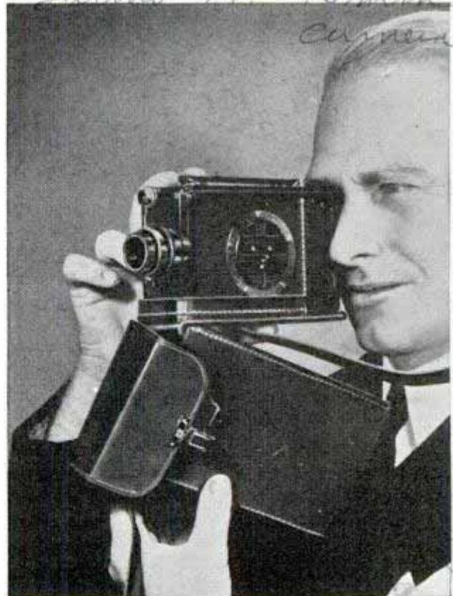
Screwed to tongue attached to its carrying case, camera is steadied in position for taking movies
