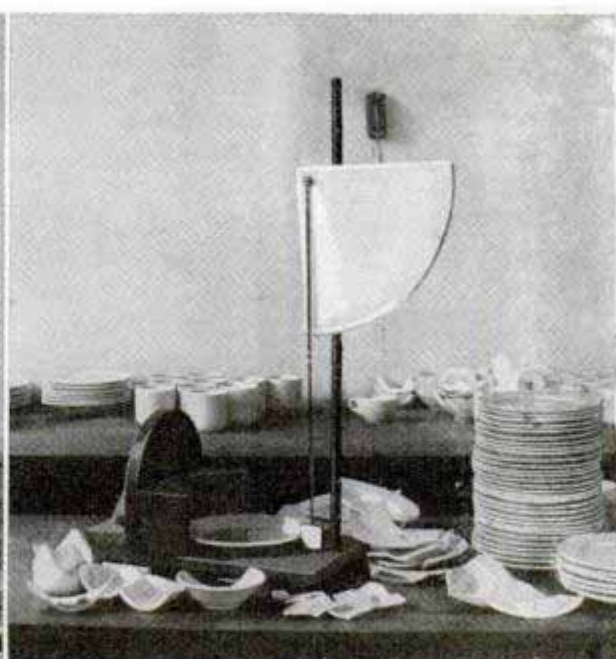
Breaking strength of belts is determined on machine at top, which has 50,000-pound capacity and also records tensile stress and stretch of belt. Below, left, airplane engine on test rack; right, breaking crockery with impact apparatus in the search for more durable tableware
