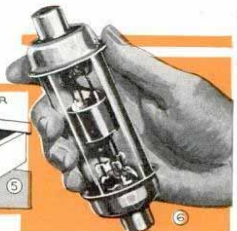
Fig. 5, short towel rack, or dowel, fitted with wood brackets and fastened across the front of a drawer in your radio workbench, serves as a handle and also provides an excellent rack for spool wire; Fig. 6, compact heavy-duty vacuum-sealed tank condenser for single-ended or push-pull amplifier in cw or phone rigs
