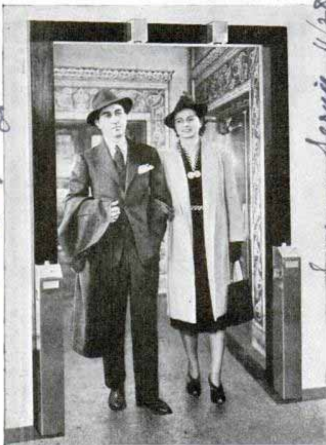
Photo-electric "eyes" in panels at sides of door and overhead scan visitors and count attendance
