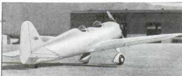
Plastic body and wing covering for airplane permits high-speed mass production to meet need in wartime
