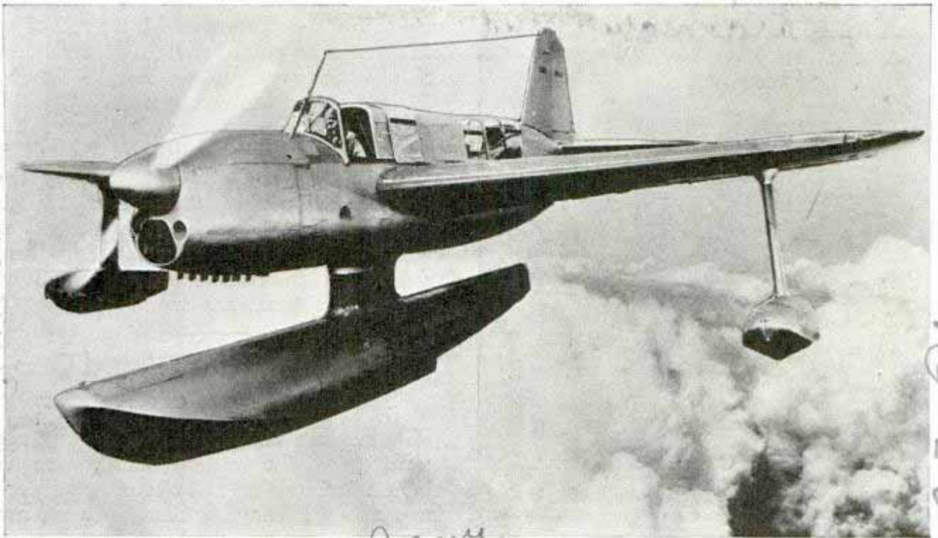
some Built primarily for surveillance work by navy fliers, this seaplane also can be adapted for flight over land by installing wheeled gear instead of the triple pontoons. It is a high-speed observation ship
