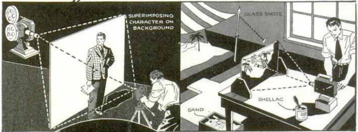
Above, filming an actor against a projected background, and shooting scene with the help of a painted-glass screen. Left, editing film with a small viewer that enlarges each frame separately. Below, amateurs obtain best results by mounting cameras on tripods
