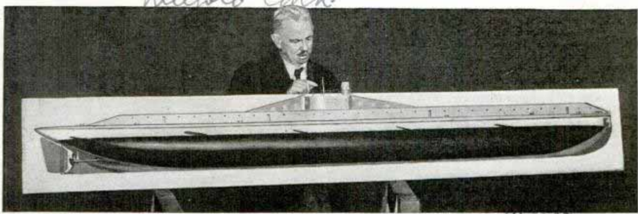
Drawing shows freight-carrying submarine which is capable of diving below surface of sea when it faces danger of attack by enemy raiders and could be built to take on a cargo of 7,500 tons
