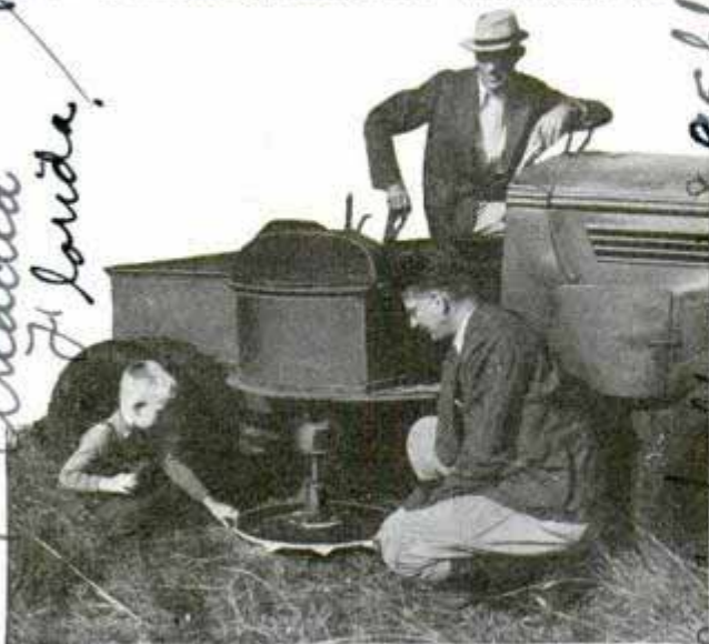
One of the rotating disks may be seen beneath truck
