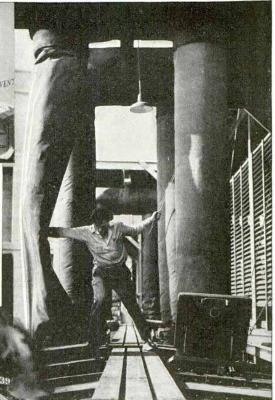
Top, left, mechanical loader at work. Right, air-conditioning tubes blow cold air into one end of car and exhaust warm air from other end. Bottom, heavy locomotive hauling fast food express
