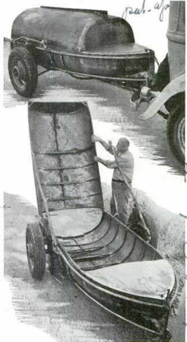
Forming its own trailer when towed on land, above, metal boat is unfolded when it reaches water
