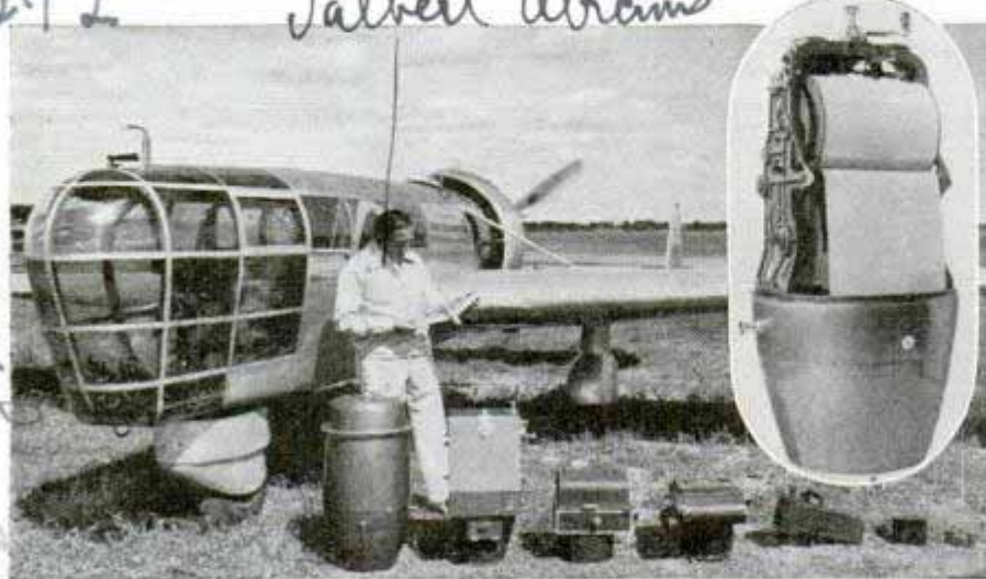
Mapping plane and aerial cameras; that in inset carries 500-foot film
