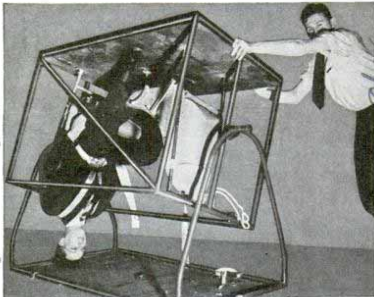
Spring-equipped safety belt for pilots being tested in chair that vigorously rocks subject and turns upside down
