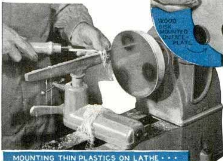
MOUNTING THIN PLASTICS ON LATHE . . .
