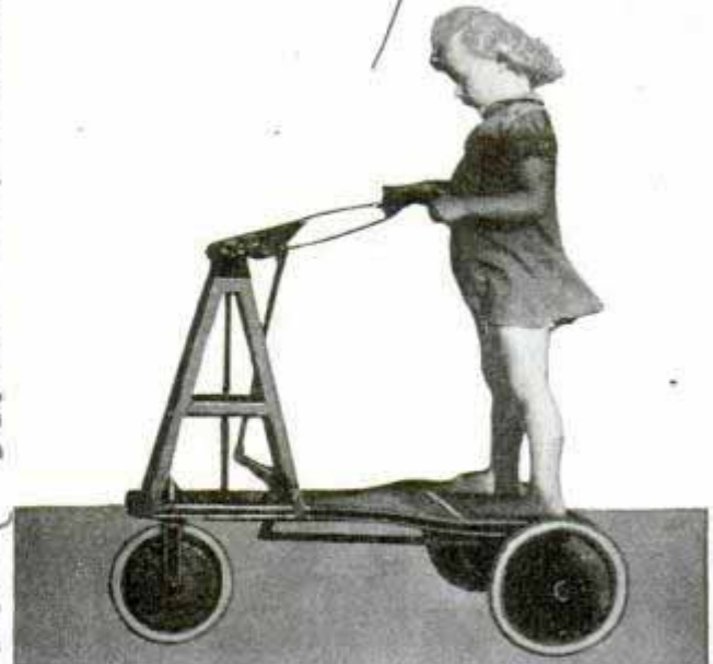
Child pumps driving-handle up and down to propel three-wheel scooter that saves pushing with feet
