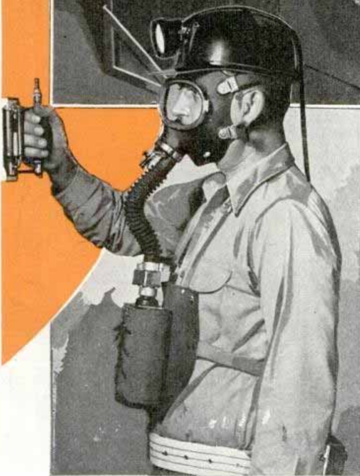
Surface indicator at top measures smoothness of metal or painted surface. Below, miner wearing gas mask and helmet carries a carbon-monoxide detector
