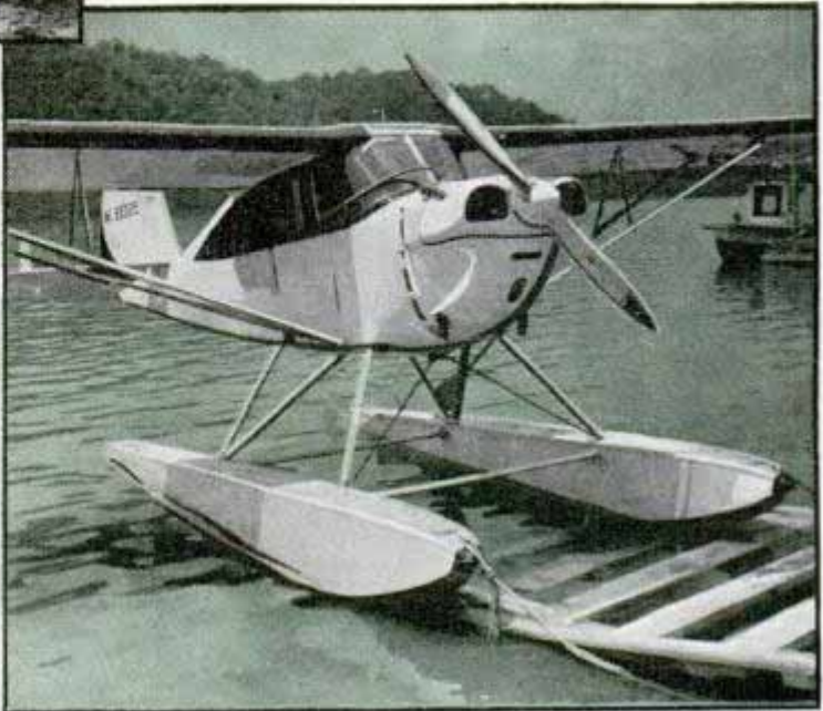
Stinson 105, with arrows indicating essentials of this 75-horsepower ship (top). Federal inspector examining a Cub just before it leaves factory (center). Aeronca seaplane powered with 65-horsepower engine
