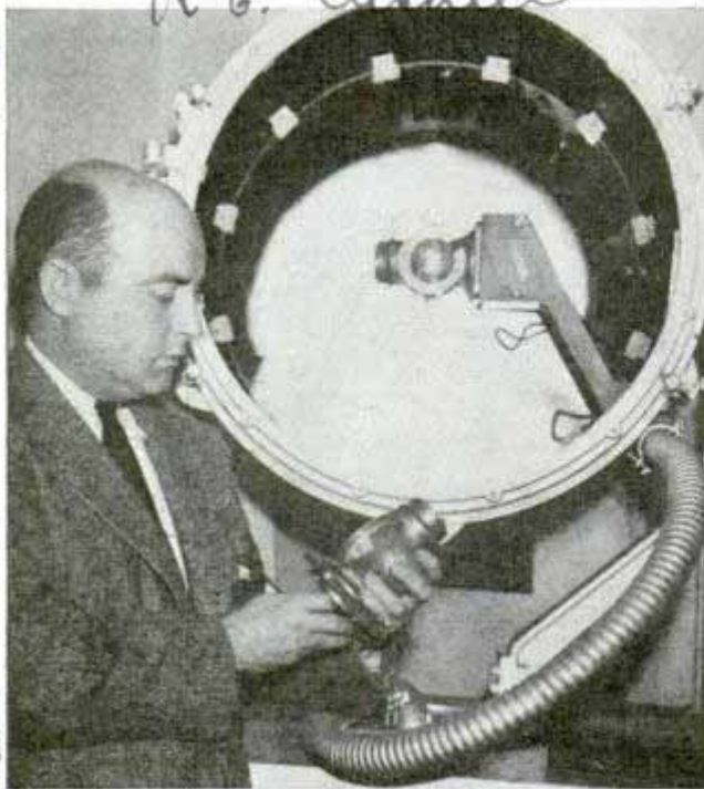
Powerful searchlight is shown above with one of the mercury-lamp units held by lighting specialist
