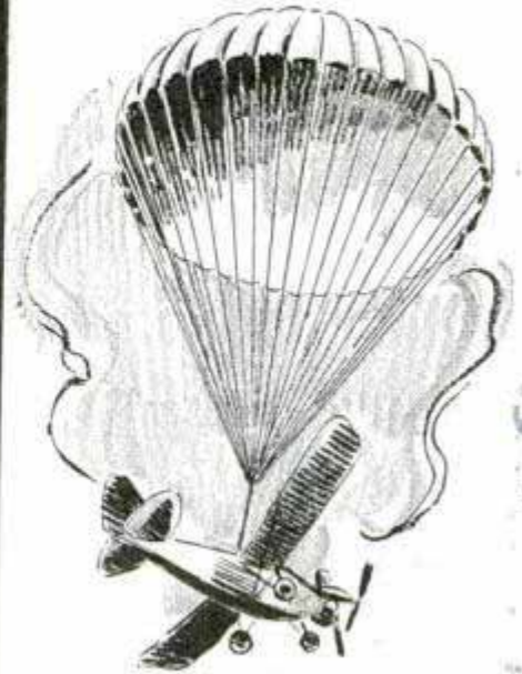
MERE PRESSURE OF A BUTTON ON THE INSTRUMENT HELD BY THE OPERATOR STOPS THE MOTOR, RELEASES THE PARACHUTE AND THE PLANE SETTLES GENTLY TO EARTH
