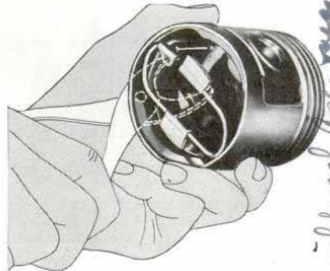
Spring-steel expander is placed in piston while it is in the cylinder and without removing rod or pin
