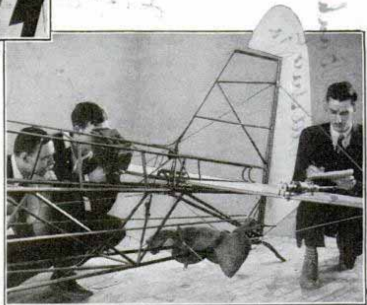
Pilot's compartment of the Stinson 105 (top); instrument panel of a Piper Cub (center), and testing vibration of tail unit in Piper factory
