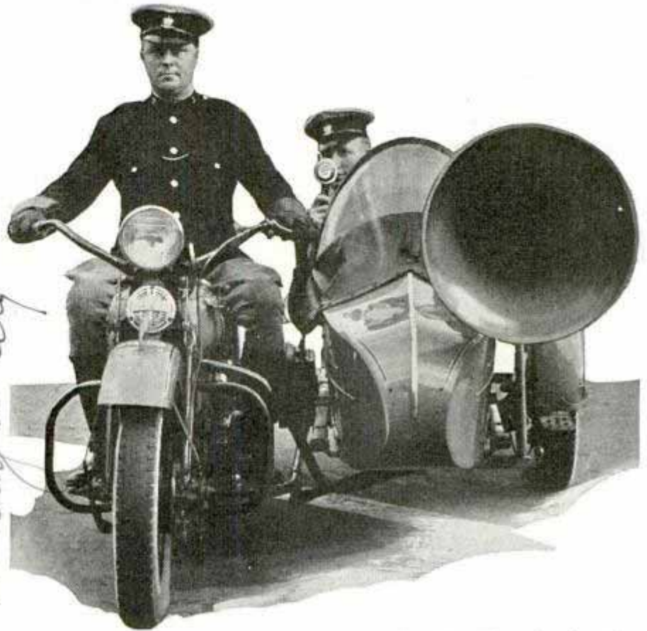
Durban policeman using loud speaker mounted on his sidecar for directing vehicles and pedestrians, while his comrade drives the motorcycle
