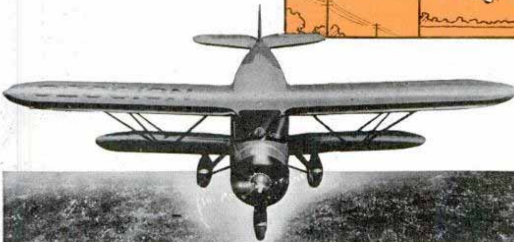
Refueling fifty-five horsepower Cub in midst of its record endurance flight of 535 hours 49 minutes (top); sketch showing difference between landing with standard gear (upper panel) and with tricycle gear (lower panel). Bottom, Waco "N" coming in to land. Note tricycle gear
