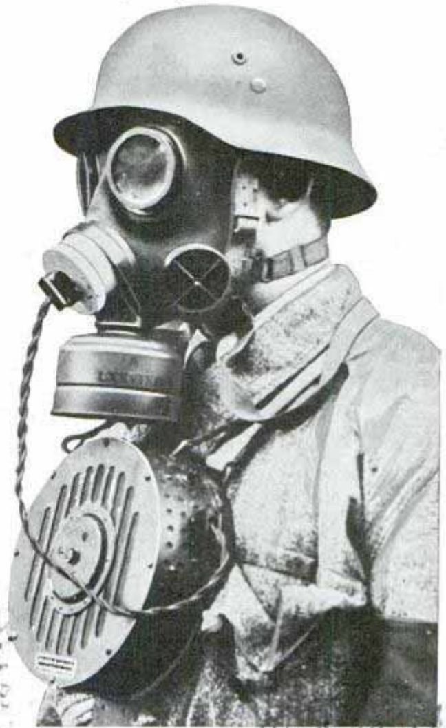
Speaker and microphone combined with gas mask enables soldier to be heard without removing guard
