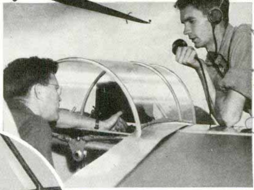
Above, testing radio before the sailplane takes off. Left, circle, operator in auto receives pilot's message giving location of sailplane. Below, ground crew arrives at point where the aircraft has landed and the pilot approaches the car. The radio is also valuable for instruction purposes on local flights, such as warning beginner pilots of obstacles in their path. The two-way radio weighs twelve pounds, including batteries
