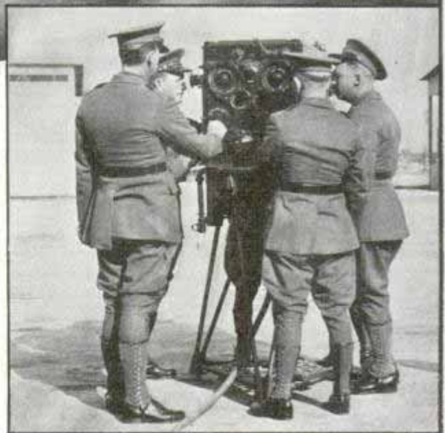
Circle, control board with switches by which lights showing position of enemy raiders can be flashed on map. Center, army bombers in test raid. Bottom, army men group around mechanical device that figures angle at which anti-aircraft gun should be fired
