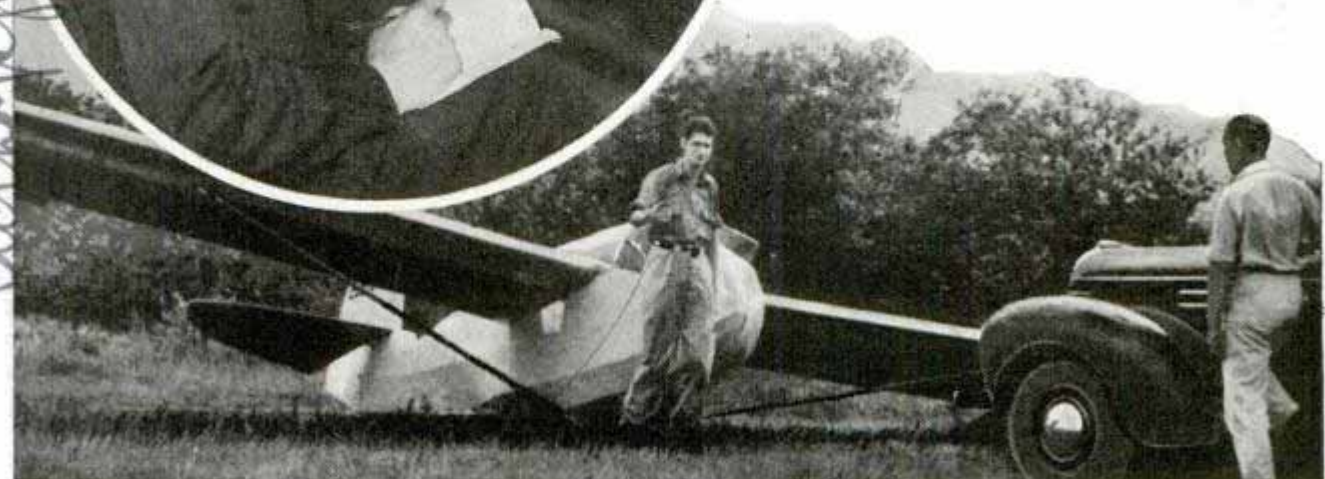
Above, testing radio before the sailplane takes off. Left, circle, operator in auto receives pilot's message giving location of sailplane. Below, ground crew arrives at point where the aircraft has landed and the pilot approaches the car. The radio is also valuable for instruction purposes on local flights, such as warning beginner pilots of obstacles in their path. The two-way radio weighs twelve pounds, including batteries
