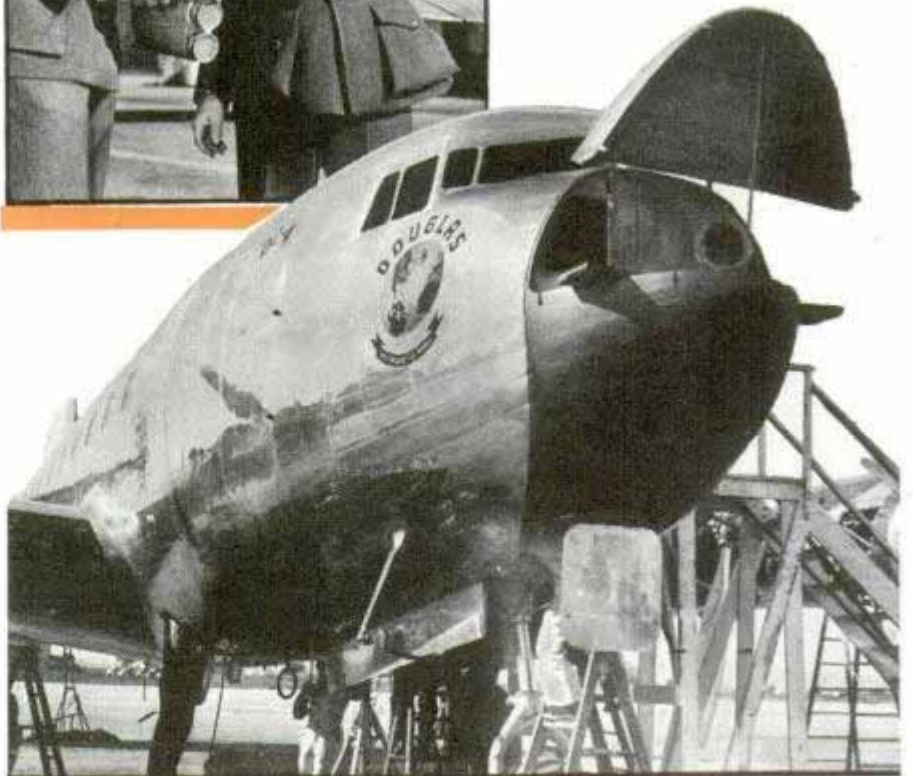
Top, how pilot's compartment is curtained off. Center, examining cartridge that contains reel on which trailing wire is unwound to diminish static. Bottom, nose of DC-4 opened to expose radio compass loop
