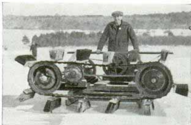
Chemical Culture Company Pushed forward by hand, sled sweeper brushes snow to one side with its twelve brooms on endless chain
