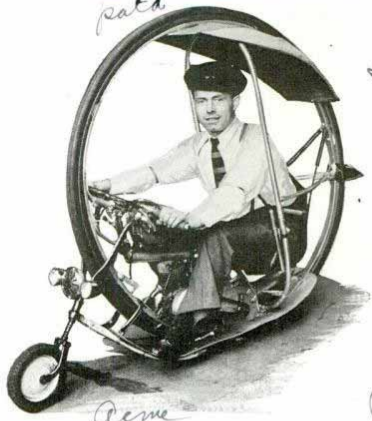
Motor and seat for rider are mounted inside hooplike wheel which is steered by handlebars attached to small front wheel
