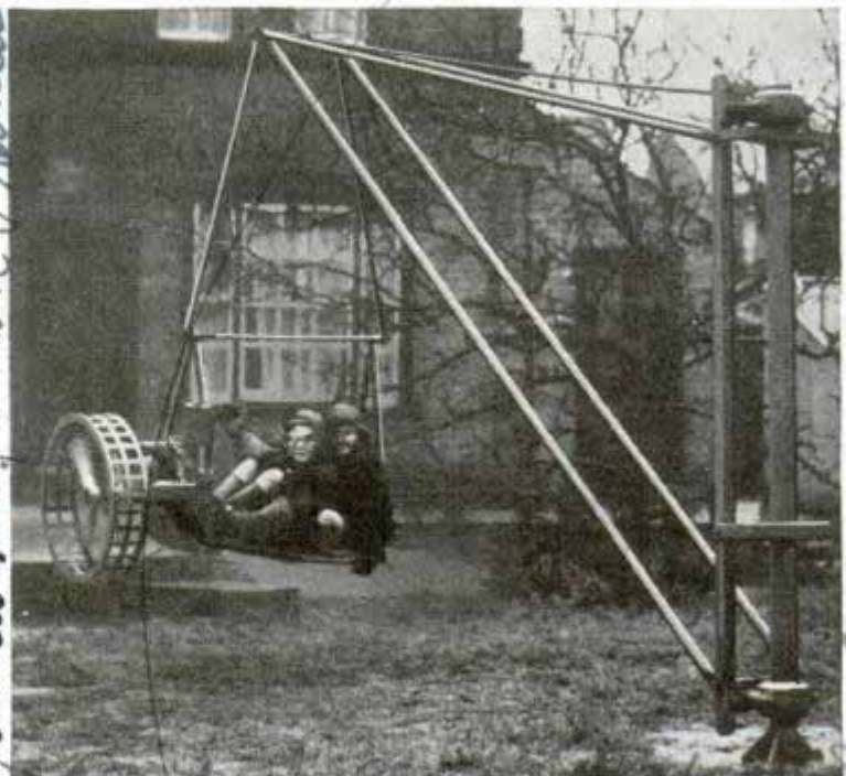
Homemade flying merry-go-round, erected in back yard, is driven like an airplane by a one-horsepower engine
