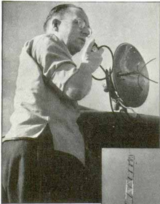
Top, talking on directional beam over parabolic antenna. Right, rotating beam antenna on sheriff's station finds direction of other transmitters. Bottom, mobile transmitter and power supply
