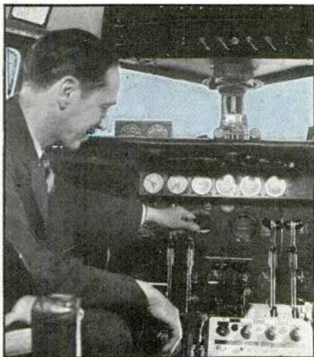
Left, Bennie Howard demonstrating throttles in DC-4. Right, instrument, in demonstrator's hand, has cross pointers which pilot follows in making landing. Below, special antenna, atop fuselage, makes possible uniform reception of radio signals required in making instrument landing
