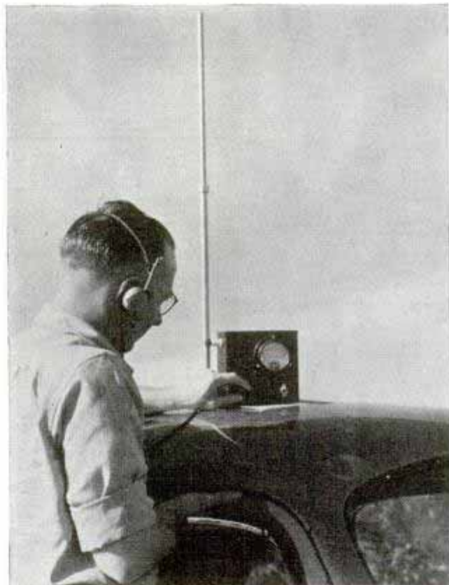
Portable receiver for short-wave beam messages; antenna rod is adjusted for different wave lengths
