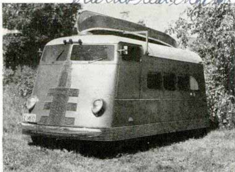
Motorized "trailer" for long non-stop runs has sleeping quarters for four, and permits one to drive while the other rests
