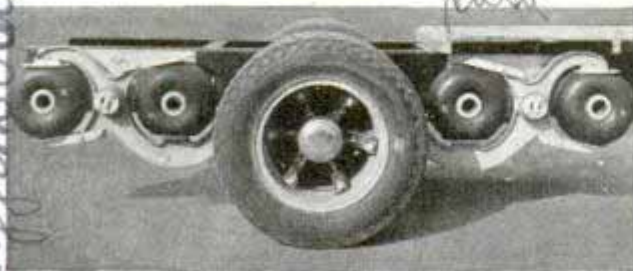
Four airplane tires on each side cushion truck load on air, improving traction and reducing tire wear
