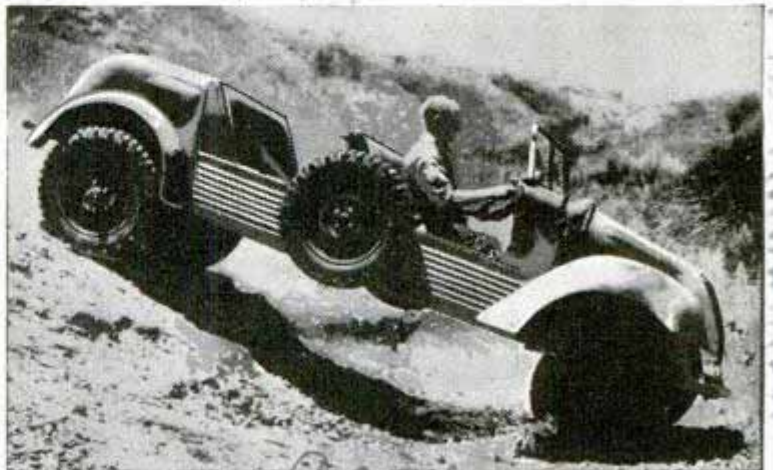
Acme Sturdy auto of German army travels rough terrain, climbs forty-five degree incline, and attains seventy-mile speed
