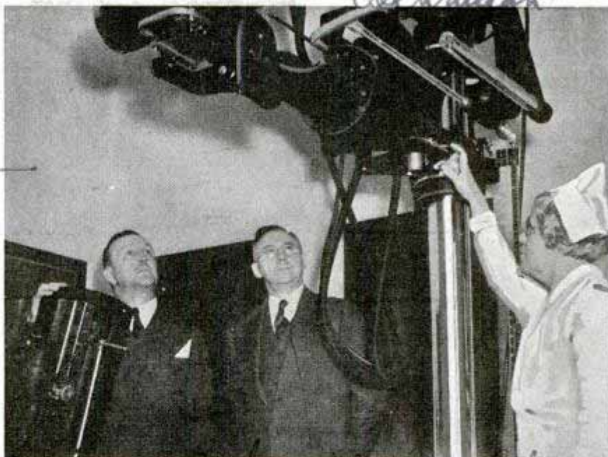
Automatic X-ray camera releases charges of 100,000 volts of electricity when trigger is pressed to make split-second pictures of beating heart
