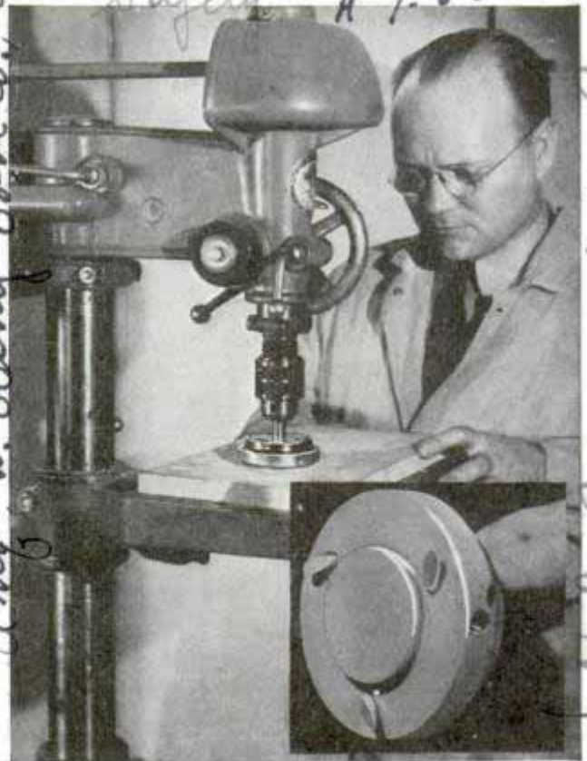
Planing piece of wood in drill press. Inset shows new tool with its three cutters held by set screws
