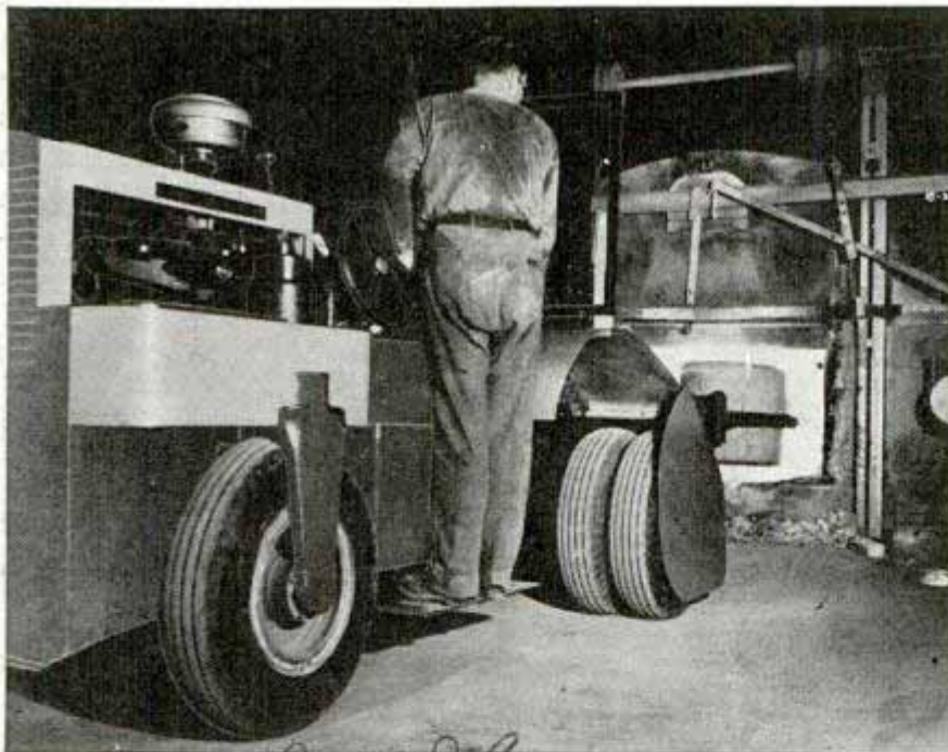
Truck controlled by "electric eye" rolls back from fiery furnace at exact instant two-ton crucible of optical glass must be withdrawn
