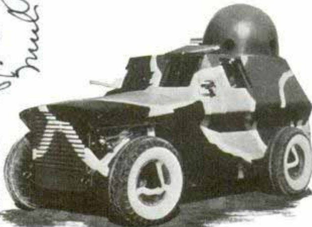
High-speed bulletproof auto with rotating turret on top is designed to combat low-flying airplanes
