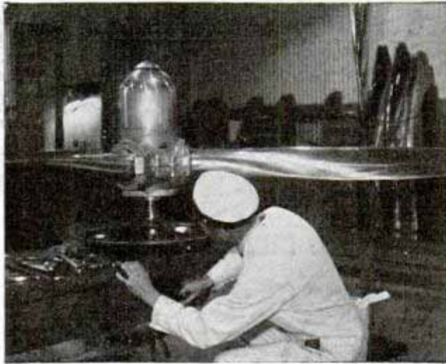
Giant propeller on test stand for checking after its mechanism has been serviced thoroughly
