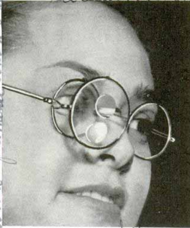
Telescopic mounting for spectacle lenses helps near-blind to see well enough to perform normal work
