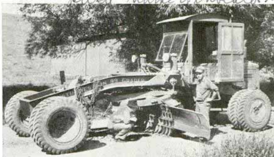
Inspecting special toothed blades attached to road machine. Two types are used, one for loosening gravel, the other for removing ice
