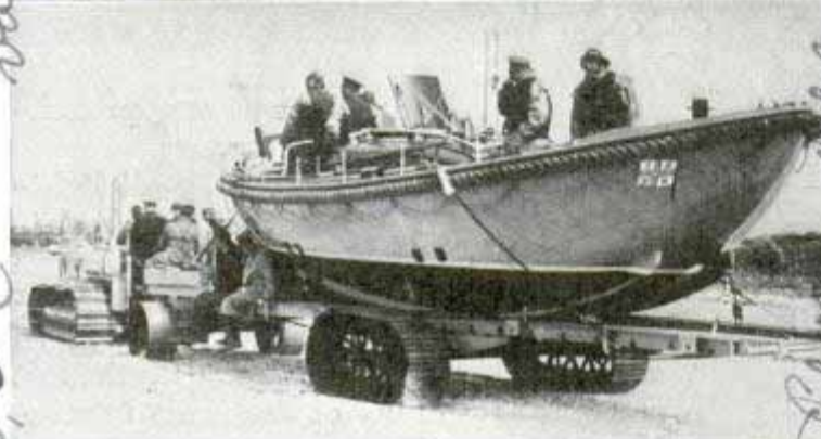
Watertight tractor, top, speeds launching of lifeboat by hauling it into water on track-type trailer as shown in lower picture
