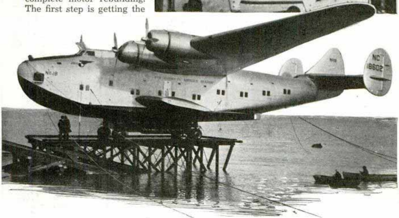
Engineer in position to work on engine in flight (top) and Clipper being brought to land on cradle similar to that of a marine railway (bottom). This is first step in the maintenance routine
