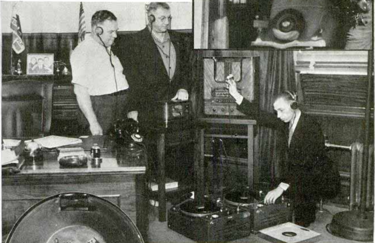
Radio car finds direction of short-wave station by rotating on grease rack, top. Center, recording high-speed signals, to be played back slowly for decoding. Bottom, tiny beam transmitter sends signals twenty to thirty miles
