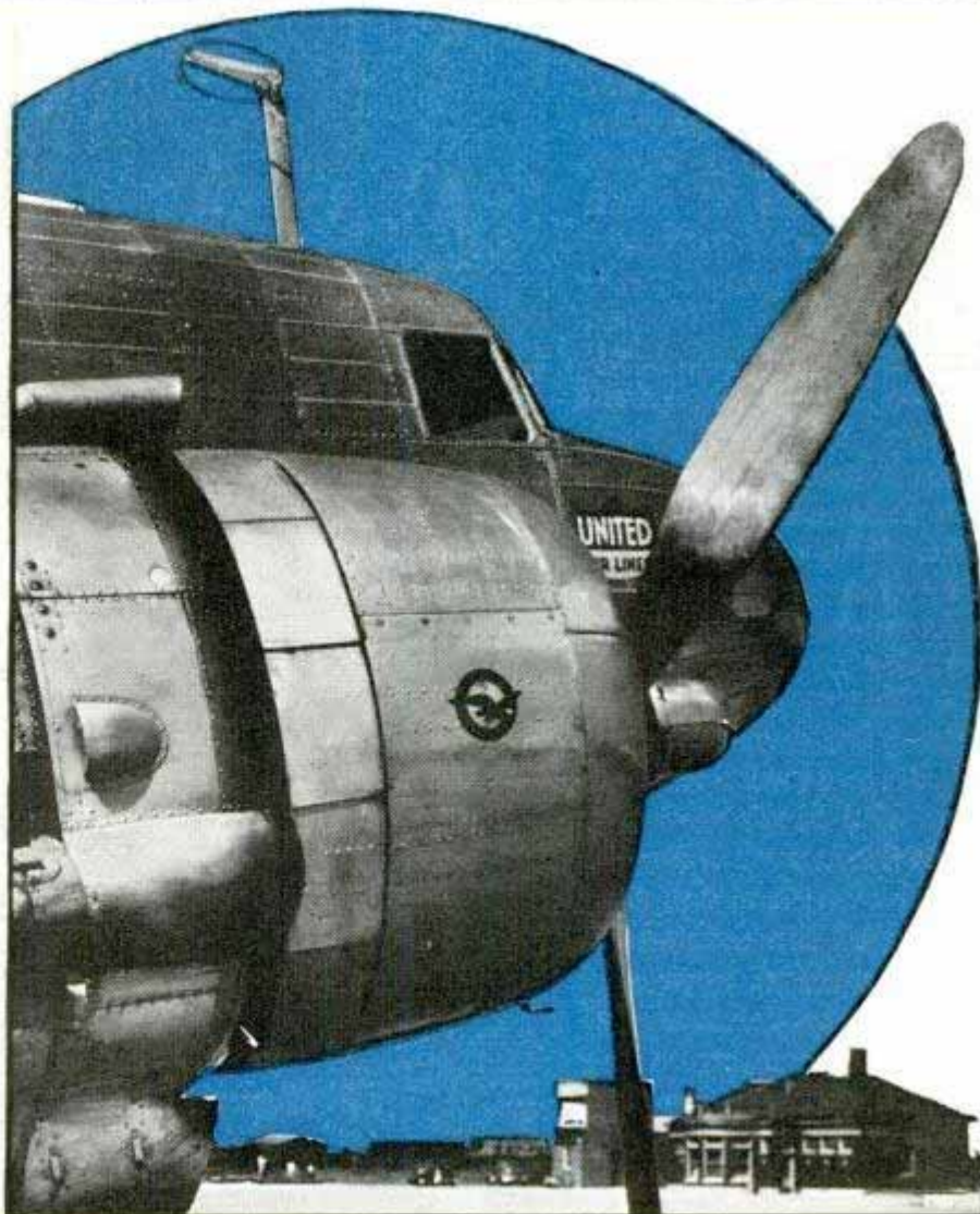
Left, Bennie Howard demonstrating throttles in DC-4. Right, instrument, in demonstrator's hand, has cross pointers which pilot follows in making landing. Below, special antenna, atop fuselage, makes possible uniform reception of radio signals required in making instrument landing
