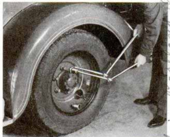
Handy two-in-one wrench which speeds up work on truck and bus tires
