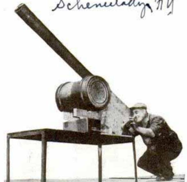
Circuit breaker set up in unusual position. Base contains mechanism and long barrel serves as muffler
