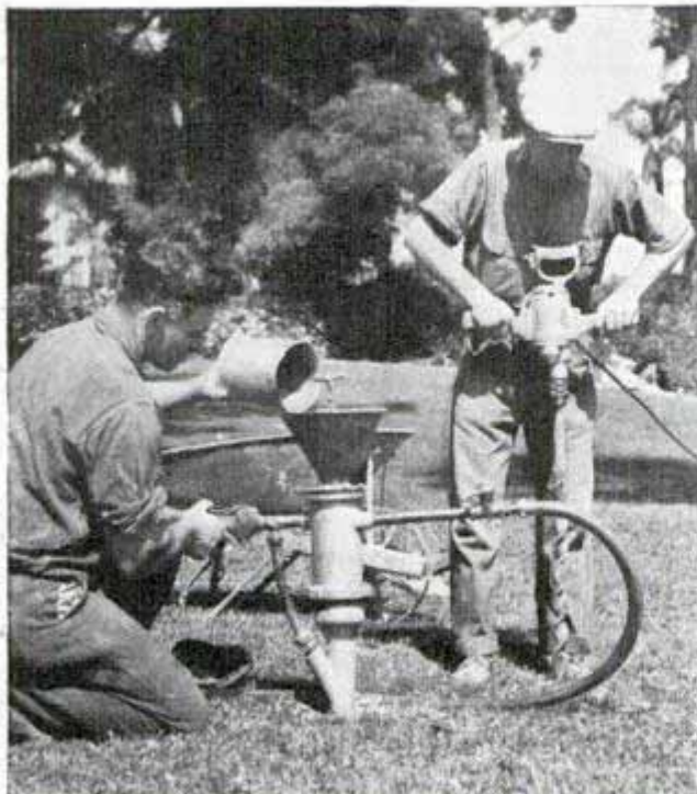
One worker drills hole while the other forces fertilizer deep into the soil
