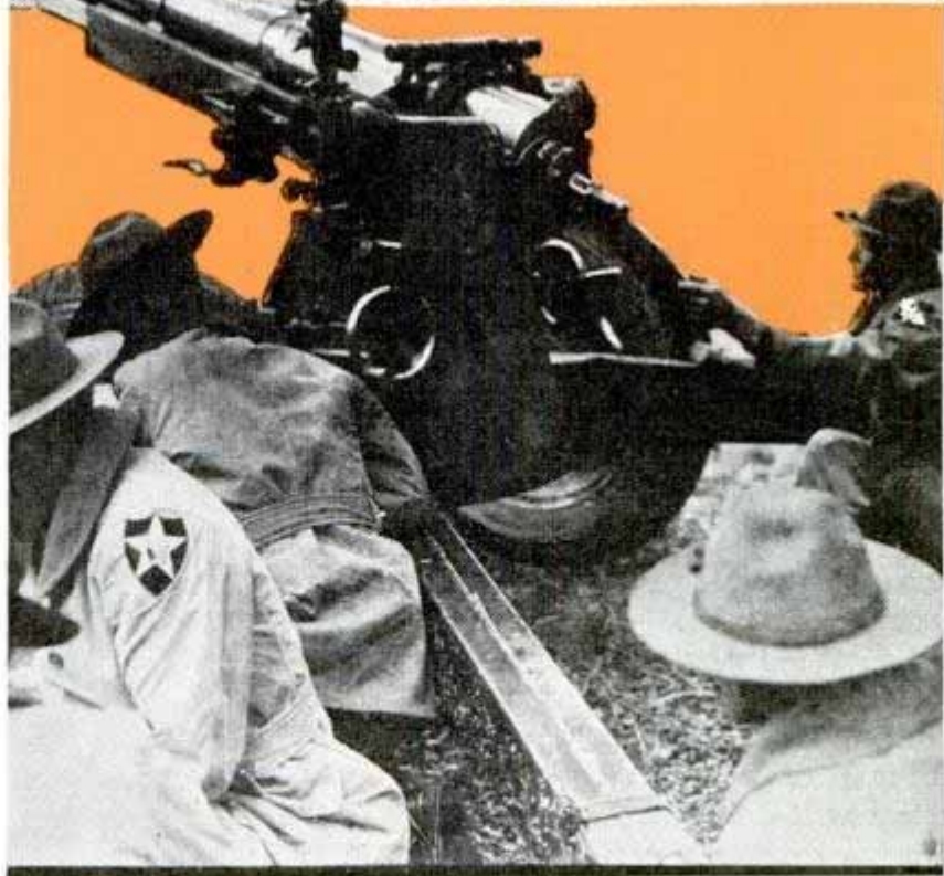
Top, observation planes flying above the U.S.S. cruiser "Portland." Bottom, new 4.5 field piece, with split trail, ready for firing. Note that the gun is mounted on a carriage which facilitates rapid movement as the attacking force advances on the enemy
