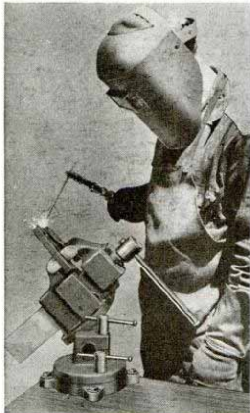
Welding vise with double-swivel arrangement turns at any angle required by work
