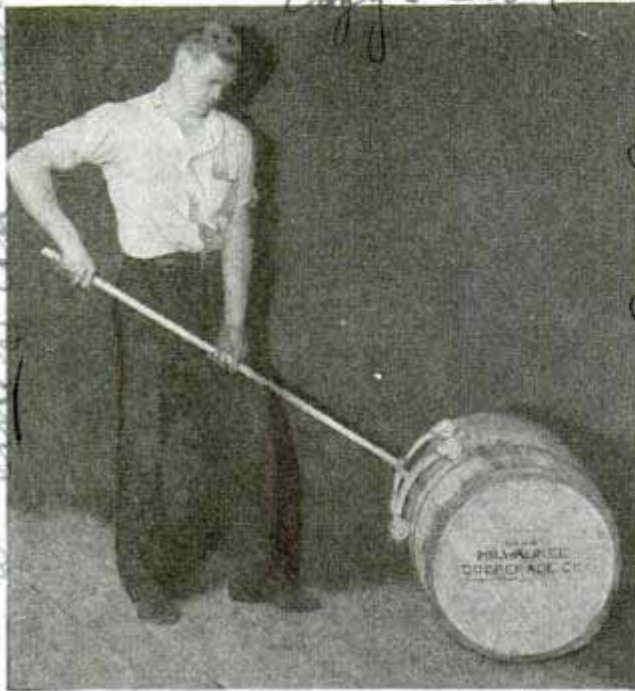
Barrel "goad" equipped with four rollers pushes and steers the heavy containers with minimum of effort
