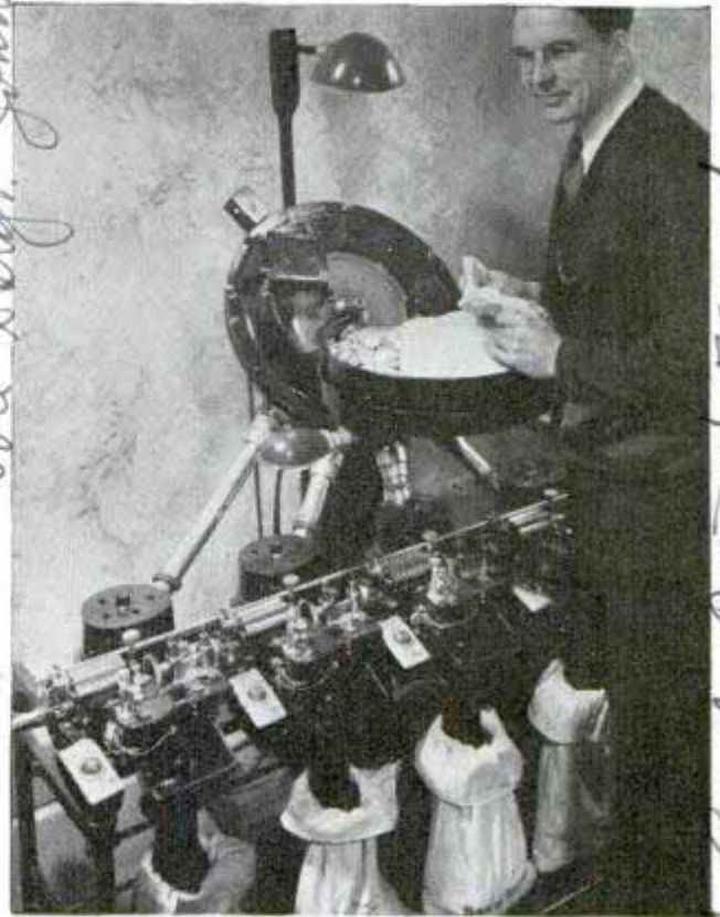
Coins poured into hopper are sorted and then counted as they clink along into the right money sack
