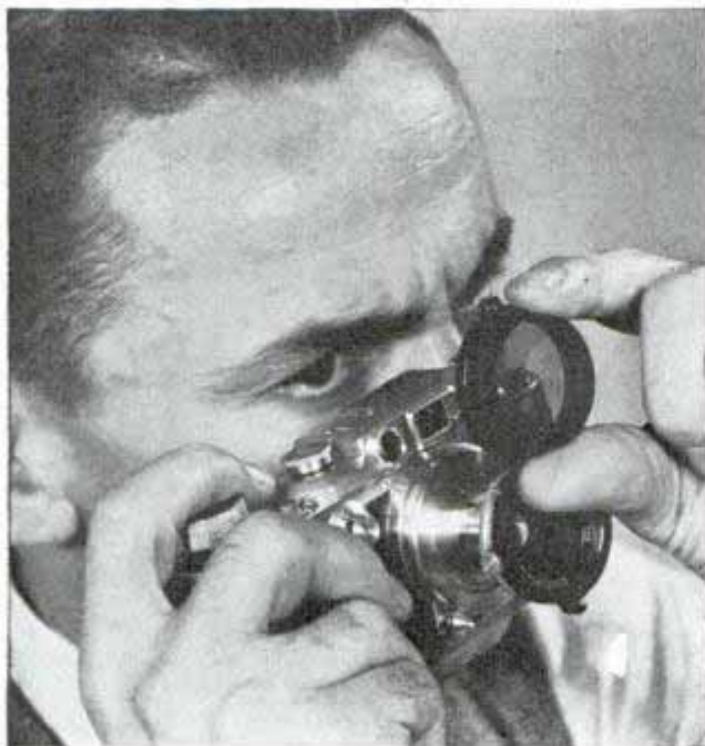
Photographer looks through polarizing filter to adjust it, then swings it in front of camera lens
