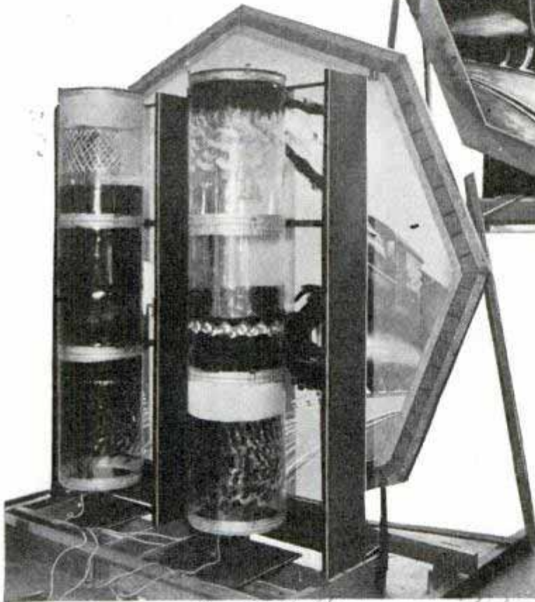
Left, light shining through rotating cylinders imparts backward motion to tracks, ballast, steam and smoke in train scene above
