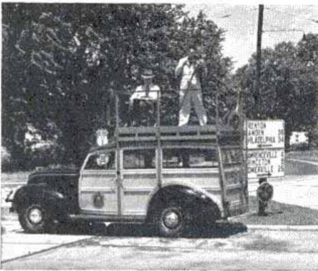
Camera car of accident laboratory films traffic movements while observer counts passing cars
