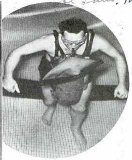
Two views of air tank which permits diver to remain under water for long periods. Left, ready to dive. Right, on bottom of pool
