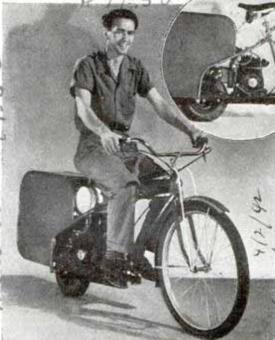
Motor scooter mounted in place of rear wheel has handlebar control and powers handy delivery bike
