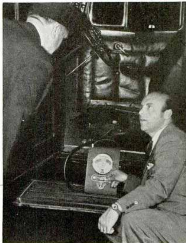
Ills of battery and car's electric system show up quickly on this tester that hooks to terminals
