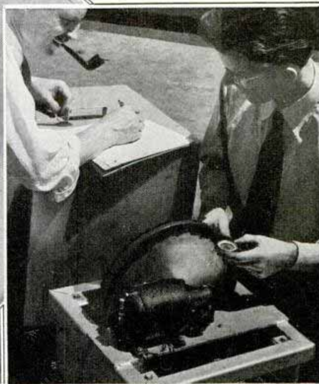
Left, lightning arrester that discharged lightning stroke captured by fifty-foot mast, center. Right, compass checks presence of magnetism in fulchronograph wheel
