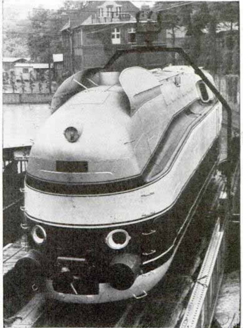
Smoke from streamliner is started upward and away from train by upturned fins that are worn on roof like a pair of earlaps
