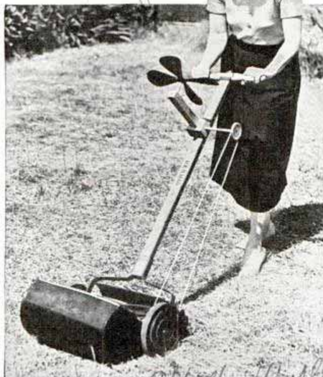
Fan blades on handle of lawn mower stir up breeze to cool worker while she pushes cutter under hot sun
