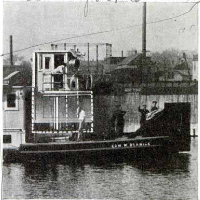
Pilot house, shown in "up" position for observation, can be brought down to clear low bridges by simply pressing button
