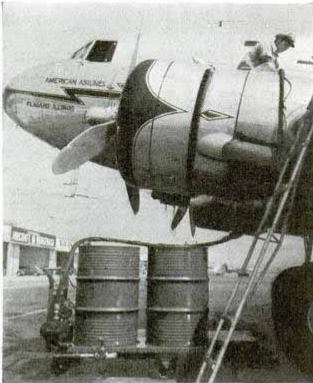
A mechanic rigged up this arrangement for pumping oil into the tanks of an air liner
