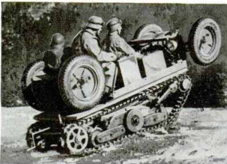
Here is the tank traveling over rough ground, with the tractor drive in contact with the surface
