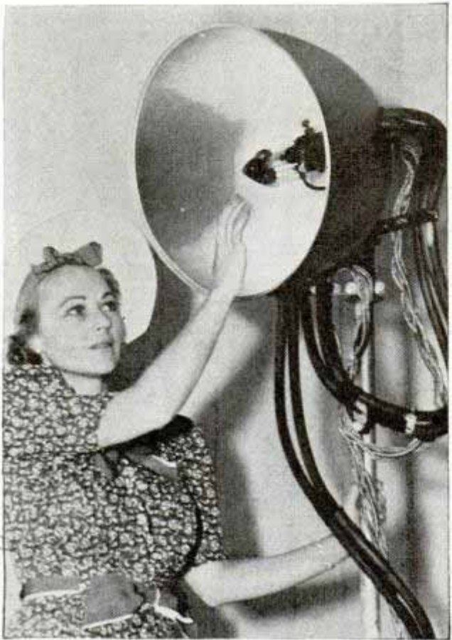
Water-cooled mercury arc lamp, small as cigarette, provides light with less heat for television studio
