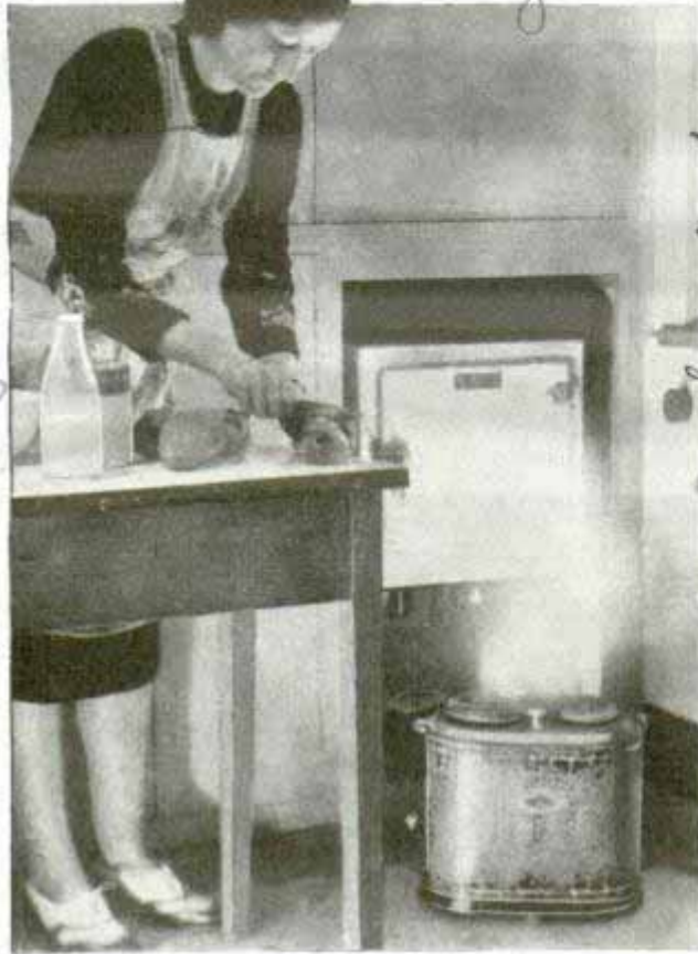
Dry mist from electric sterilizer floats in air, killing odors and bacteria, without leaving trace
