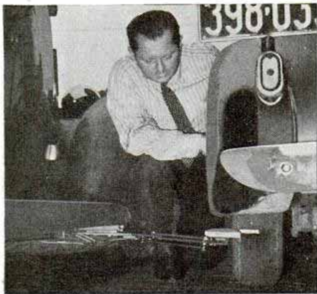
Milwaukee Journal photo Chalk stripe painted on tire by police car's automatic marker helps speed check of overtime parking
