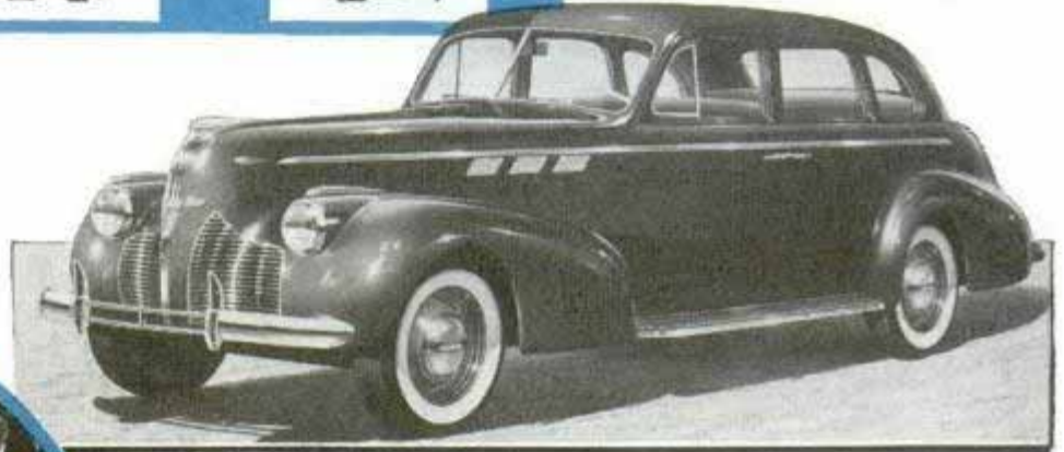
Left, seats in cars with Fisher bodies have foam rubber and cotton pads superimposed on spring base. Below, LaSalle "Special," with "torpedo" body. Note projectile-like appearance. The car has no running boards, due to being built low. It has an unusually wide front seat
