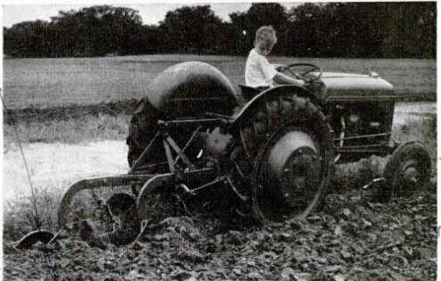
Top, tractor with "offset" seat made by International Harvester; and, below, Ford tractor has hydraulic controls for close-coupled implement
