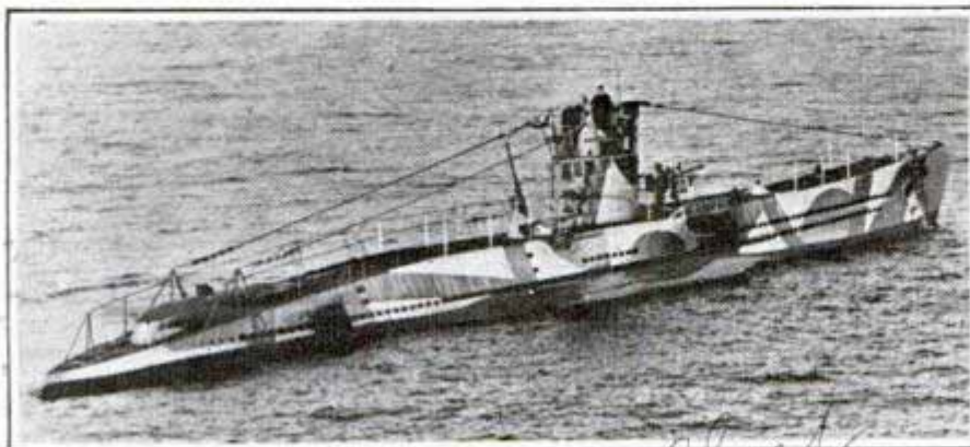
Difficult for enemy ships to see is this German submarine painted in war-time camouflage to blend its bulk with colors of surrounding waves
