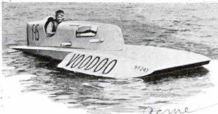
Sixteen-foot speedboat supported by pontoons draws only two inches of water. Pilot's seat is like the open cockpit of an airplane
