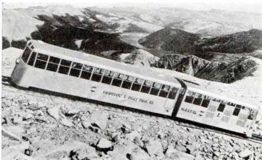
Pikes Peak's new Diesel train pushing up one of the twenty-five per cent grades. Three 160-horsepower engines furnish the motive power
