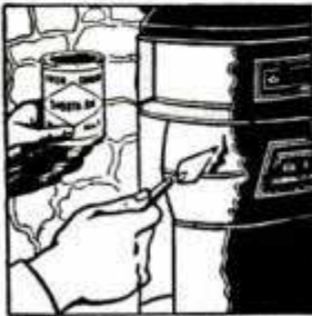
A—Sealing crack in a heater with Smooth-On
