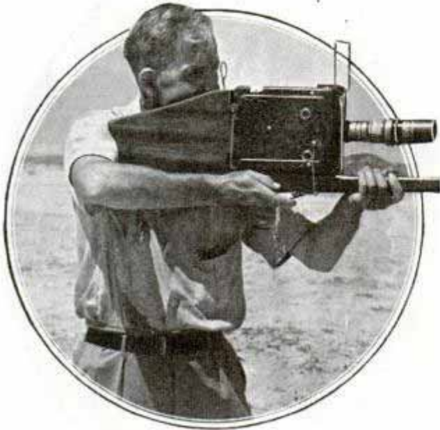
Taking steady aim with movie camera attached to gunstock for taking pictures from small boats
