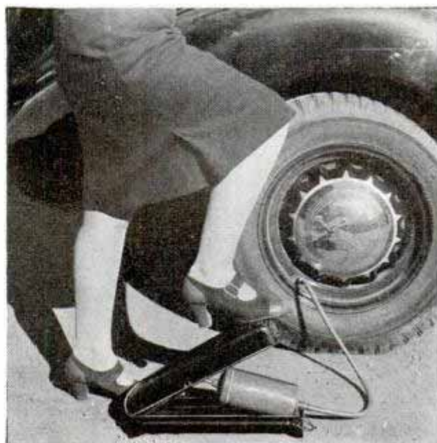
Pumping up the automobile tire is easy with this new foot-operated pump
