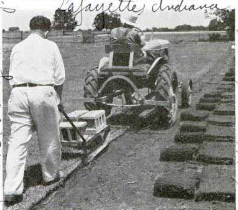
Shaving blocks of sod from a field with the tractor-drawn "harvester," which strips sod at any desired width or depth
