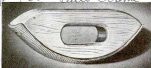
Convex file mounted on a half circle of hardwood is intended for filing protruding surfaces
