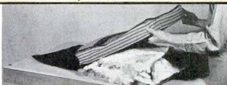
16 OPEN BOTTOM CASING FITTED IN PLACE OVER SPRING
