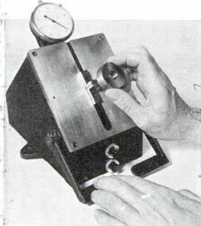
Needle dial gives instantly the inside or outside diameter of small objects within 1/10,000 inch
