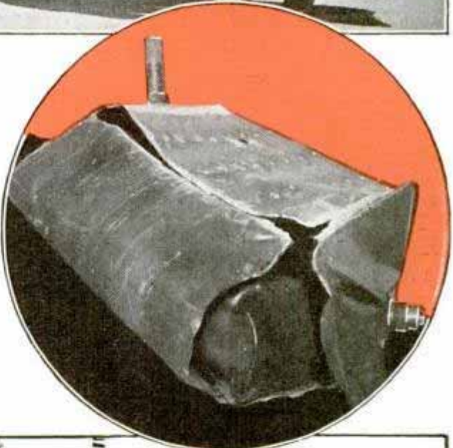
Above, "eyebrows" on wing edge give better control of plane. Circle, Thiokol-lined fuel tank after twenty-foot drop. The lining did not fail. Bottom, drawing is government's explanation of how pilot mistook southeast leg for the northeast leg of radio range, descended to land and crashed into mountain
