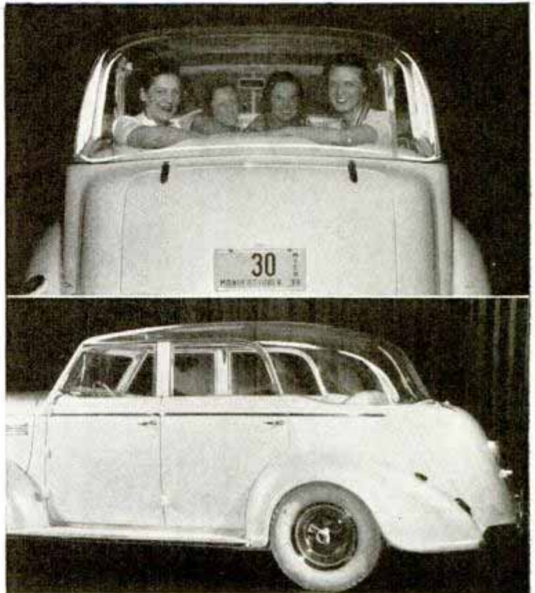
Two views of demonstration automobile fitted with a transparent top of plastic material. (Courtesy Briggs Body Co.)
