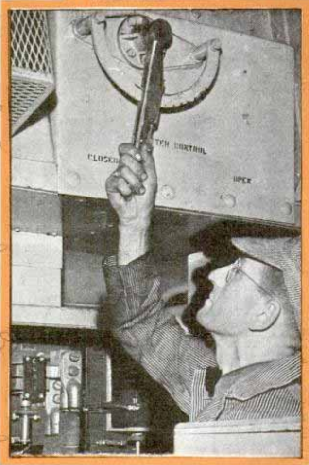
Top, "Super Chief" races through night. Below, opening shutters that send air to Diesel radiators
