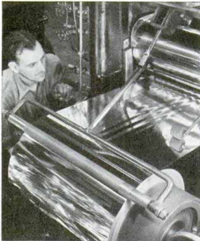
By careful rolling, aluminum foil as thin as .00025 inch can be produced. It has many industrial uses
