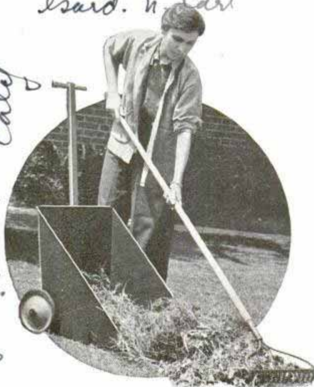
Rubber-tired metal cart for lawn work tilts forward to pick up a load from the rake.
