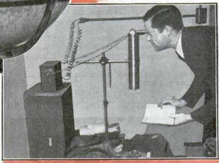
Left, finding epicenter of earthquake by plotting data from two seismological stations on globe. Pencil points to start of sharp quake on seismogram, above. Below, tilt meter testing Japanese theory that earth's surface tilts slightly before every temblor
