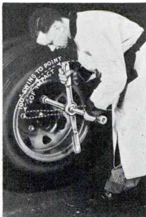
Dotted line shows how handle of wrench is swung to deliver blow to stubborn nut
