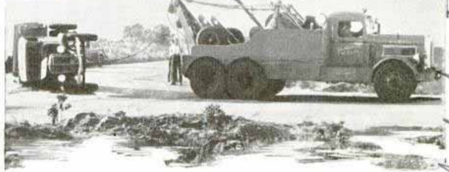
Goliath of wrecking cars, at right, can hoist 75,000-pound derelict up a cliff. At left, above, six levers behind the driver's seat control dual winches; right, view of the cab
