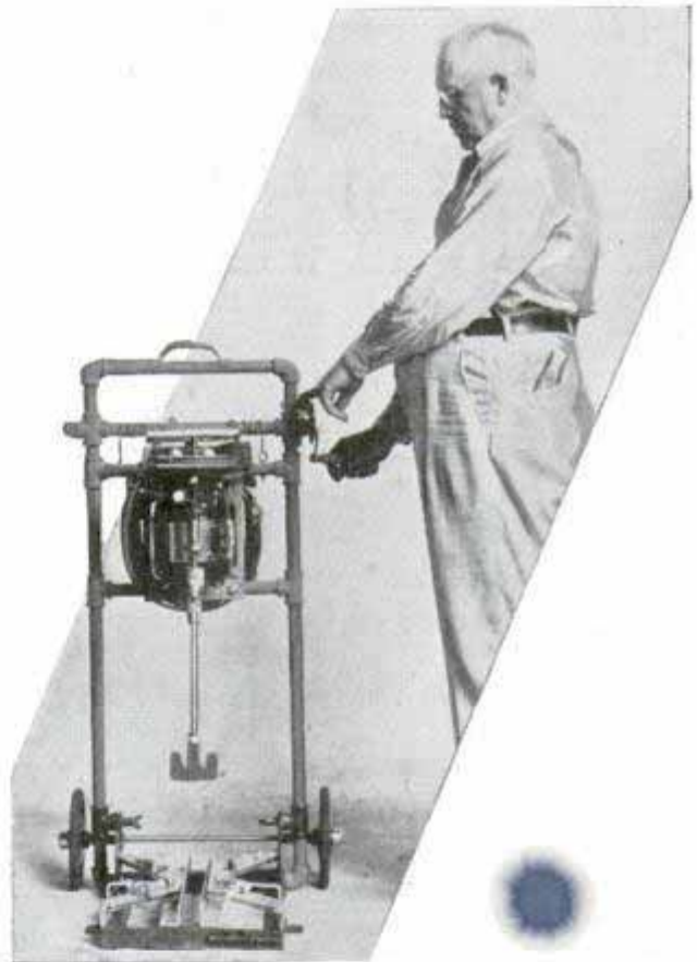
Paint mixer with power unit raised to top has its stirring blade adjusted for quart-size container
