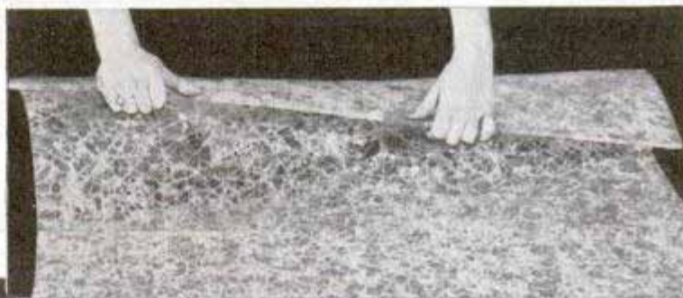
Notice distortion of sign through sheet-glass window, above, and clarity through plate glass, right. New plastic clings so tightly shattered glass can be rolled like rug. Below, reading test through glass
