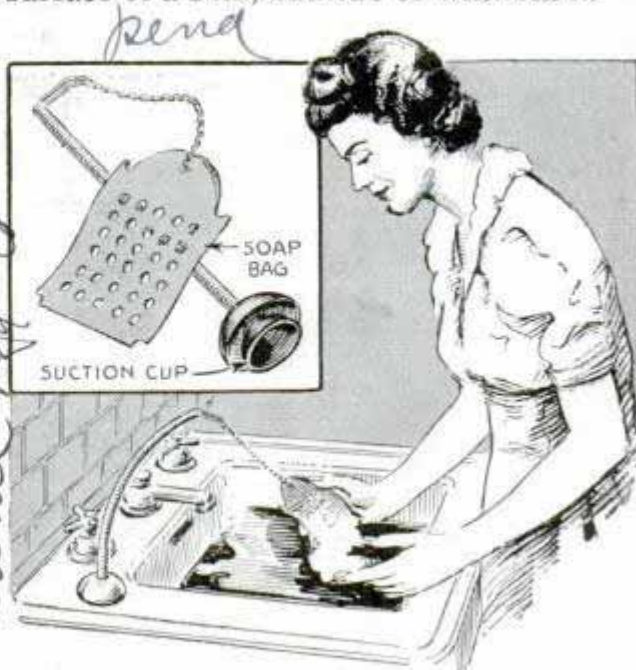
Soap holder mounted on flexible post eliminates untidy dish and conserves soap
