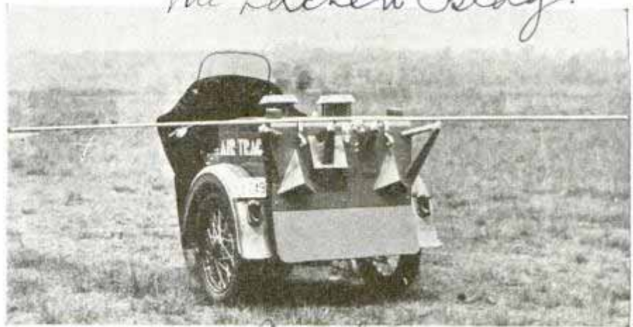
Radio station on motorcycle sends up fan-shaped signals which guide pilot to safe landing "on instruments." Horizontal pole is the antenna
