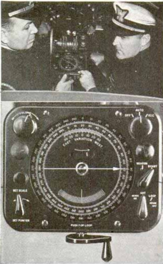
Arrow of automatic radio compass, shown at top in cockpit, points unerringly to station tuned in
