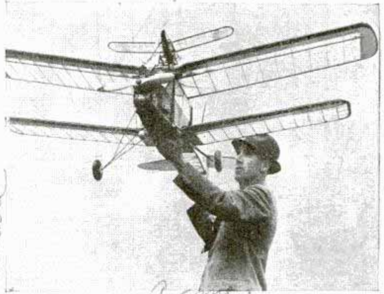
Launching "pickaback" composite plane at model aircraft meet in England. The carrier ship has a seven-foot wing spread
