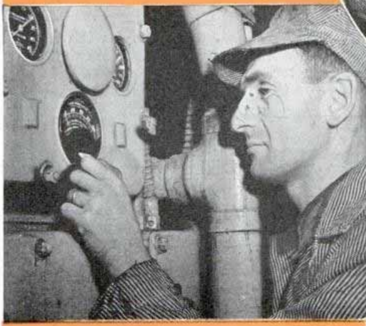
Top, engineer with hand on brake lever in sound-proofed cab. Center, making minor adjustments on one bank of twelve-cylinder Diesel. Bottom, checking engine conditions by exhaust temperatures
