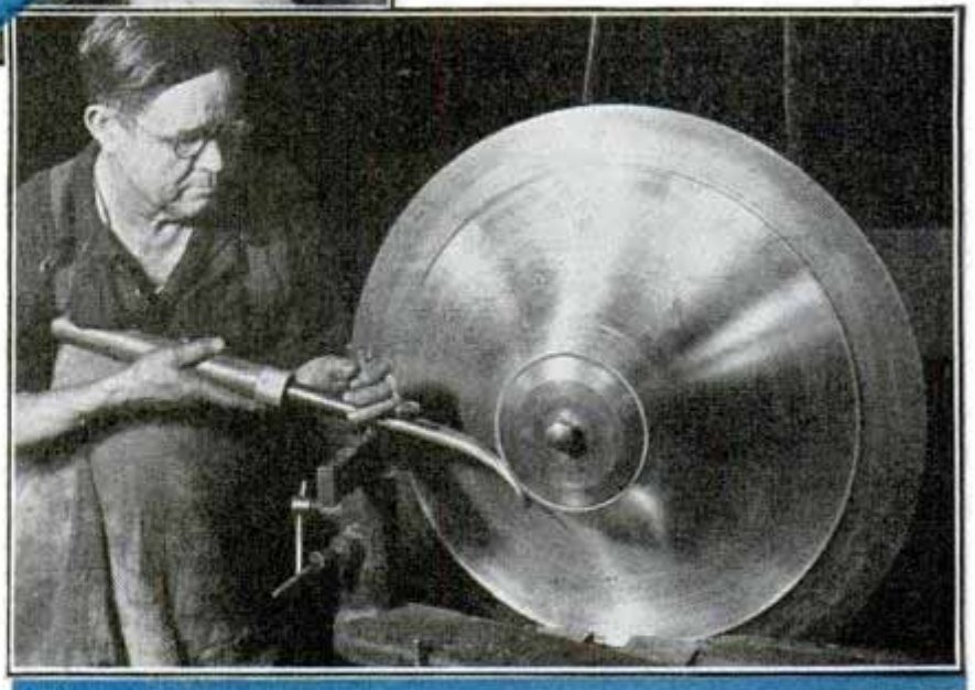
Top, typical test in Conn soundproof woodwind room. Center, delicate gauge which checks bore of clarinet to one-half-thousandth of an inch. Bottom shaping of a bell on a sousaphone as it is revolved at high speed. Applying pressure causes metal to flow in direction desired by operator
