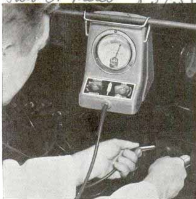
Testing valves of automobile engine for leakage with electric meter and compressed-air line
