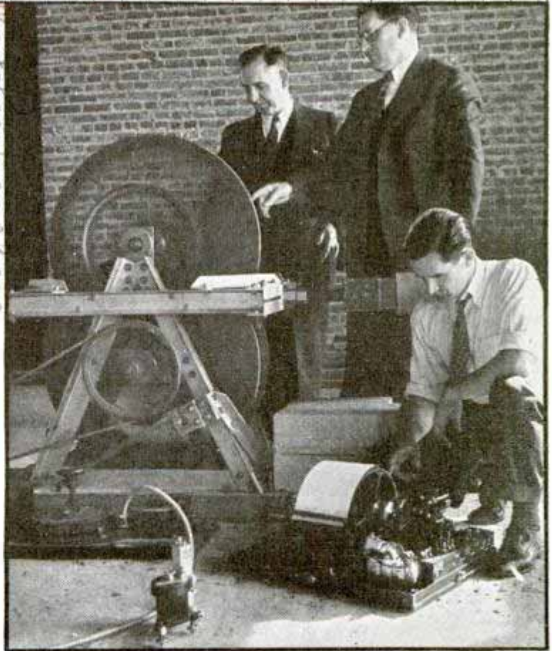
Areas in red on map at top of page indicate the earthquake belts of the world. Below, engineers test strength of a building with a vibrator. Scientific study has shown men how to make the largest buildings quakeproof
