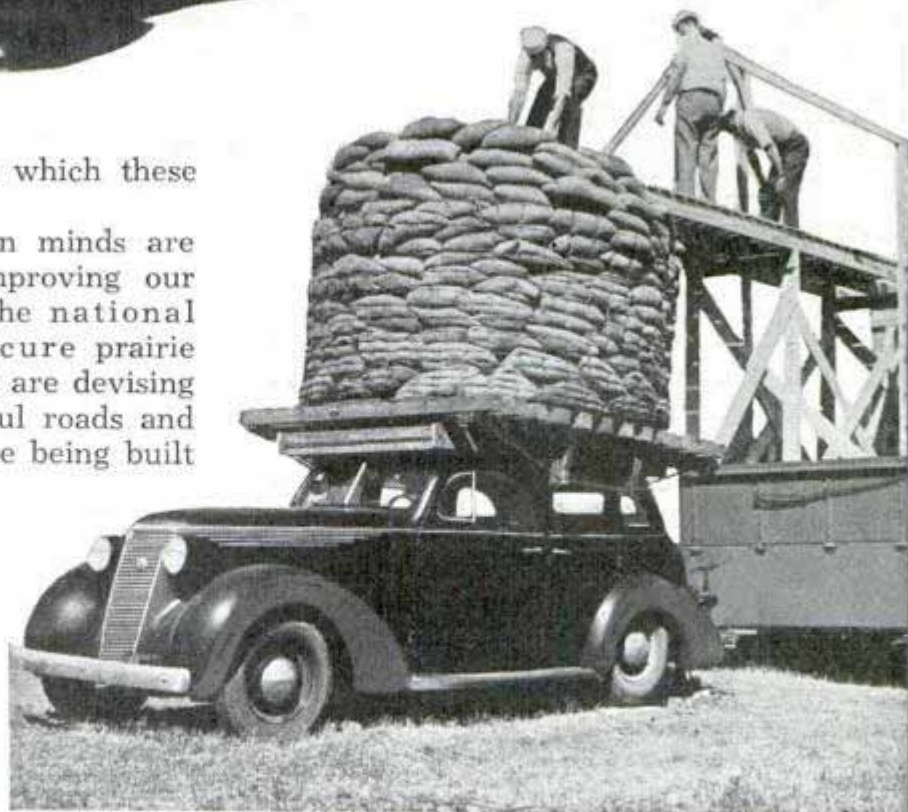
Top, left, eight-foot sign seen from 100 feet; right, to test brakes, one revolver fires when brakes are applied, the other when car stops. Bottom, 24,000 pounds of sandbags were piled on before steel roof gave way
