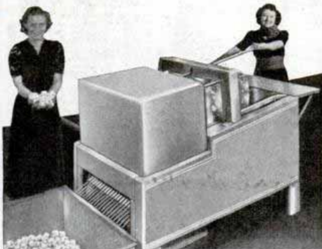
Large block of ice fed into steam cutter at right emerges at left as hundreds of small cubes
