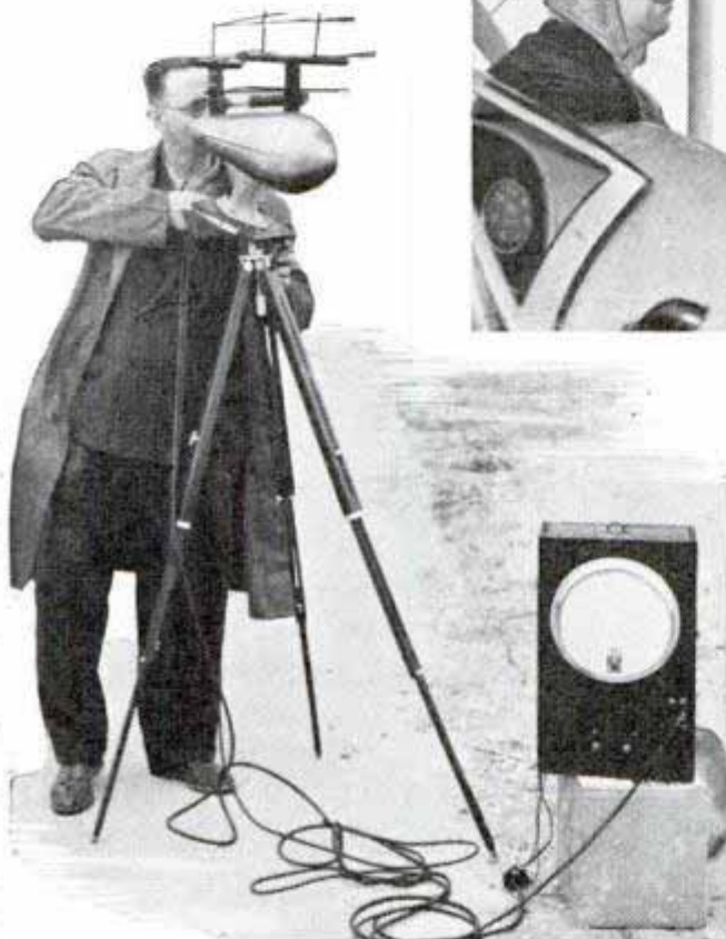
Using radio beam to detect hidden aircraft, left, and to indicate obstacle in path of plane, above
