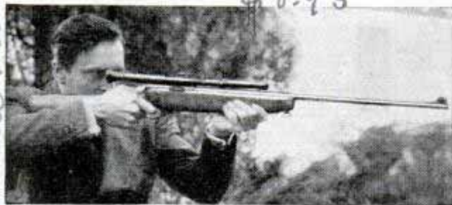
Using rifle sight which automatically gives the proper elevation for the shot
