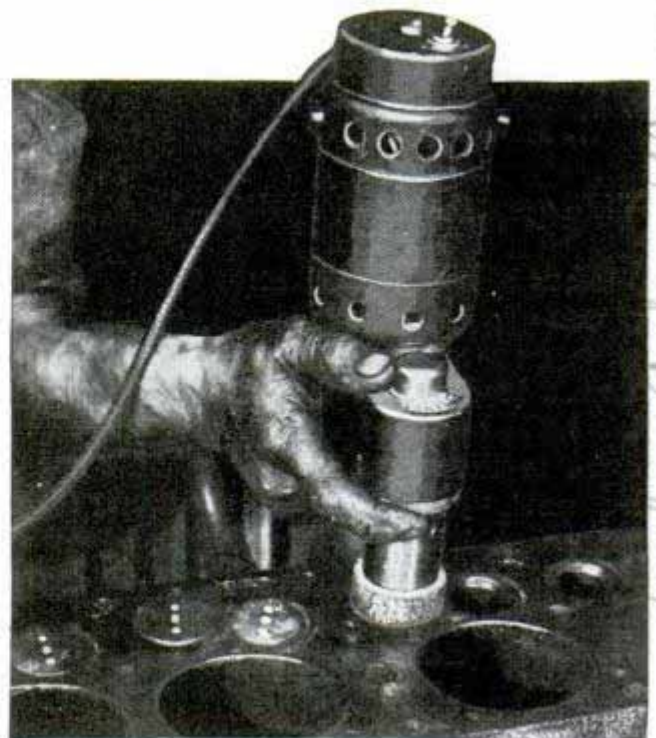
Electric valve grinder works efficiently in close quarters and can be held securely with one hand
