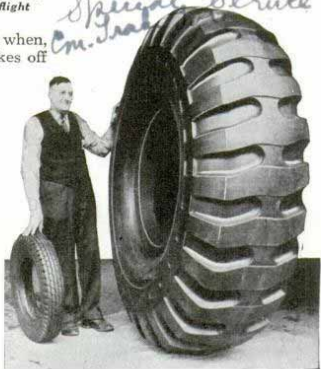
Inner tube of giant truck tire weighs 100 pounds, and the seven-foot tire itself weighs 1,500 pounds
