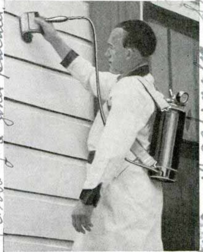
Paint is fed smoothly to bristles under control of valve in handle, eliminating dipping of brush
