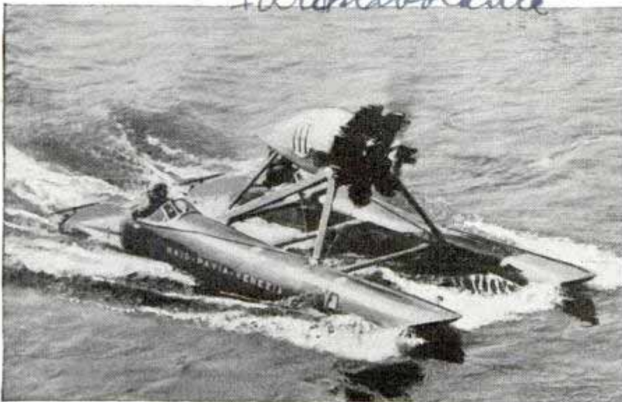
Driven by an "outrigger" engine with an air propeller, this Italian boat won race from Pavia to Venice. Driver sits in right of twin pontoons
