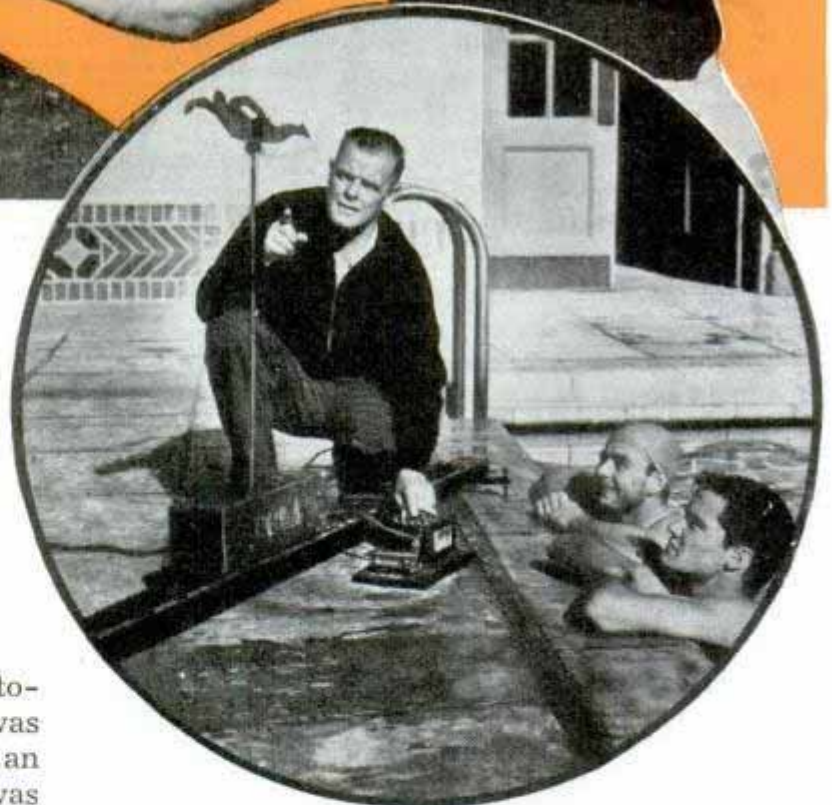
Athlete practicing with discus (left); javelin thrower in action (right), and electrical pacing device that runs along track beside pool to train swimmers to maintain certain pace (circle)
