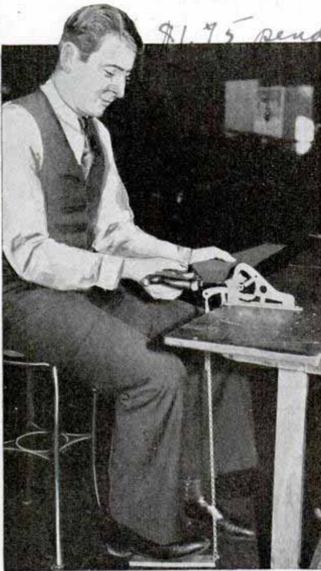
Every step on the treadle releases uniform blow of trip hammer for setting teeth of saw
