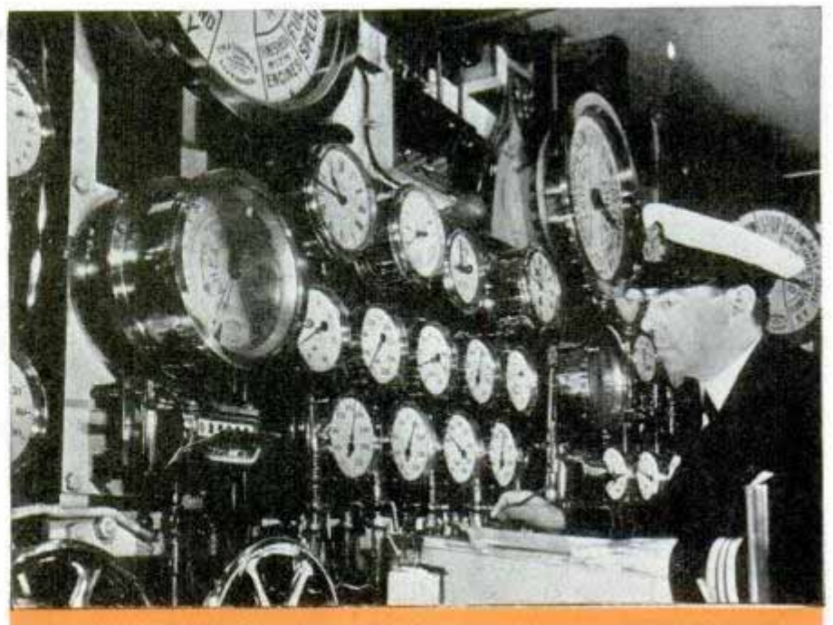
Top, left, playing deck tennis. Right, example of luxury afforded cabin-class passengers aboard the modern liner. Bottom, partial view of starting platform, with engineer making out log. Dials show engine performance.
