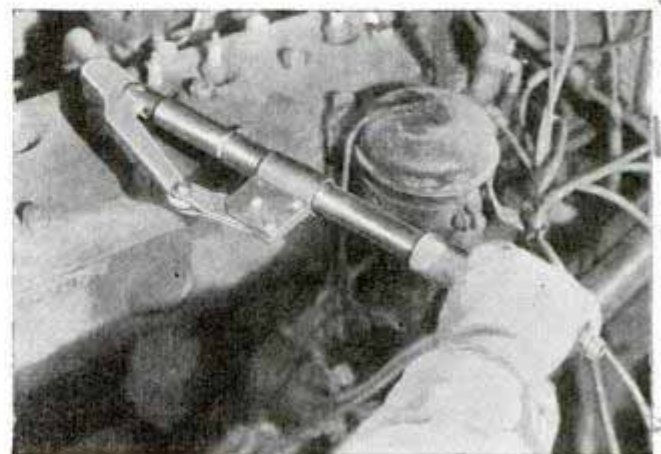
Pivoted lever will let go when predetermined pressure is applied to wrench
