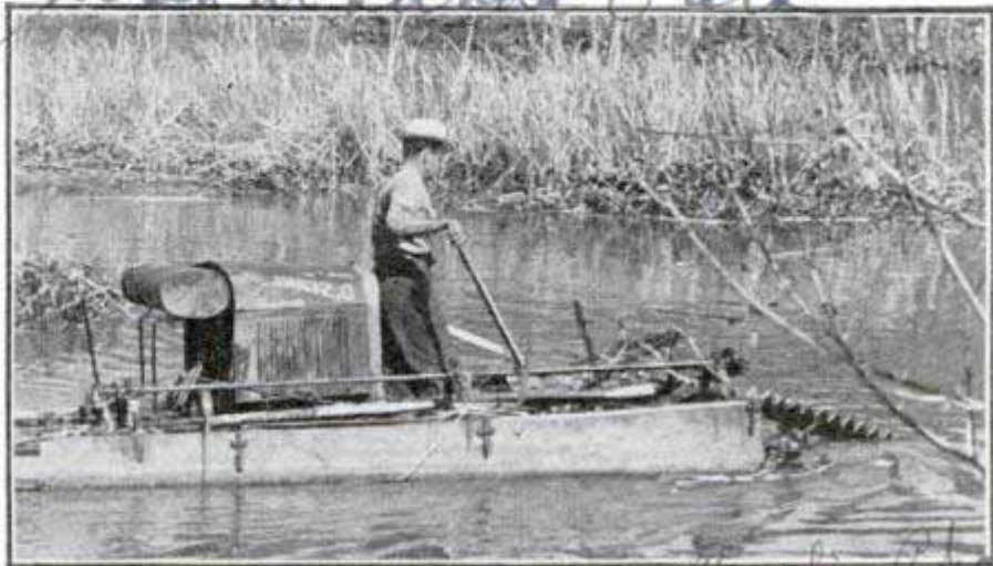
Blades mounted at the bow sever weeds as mower moves through the water
