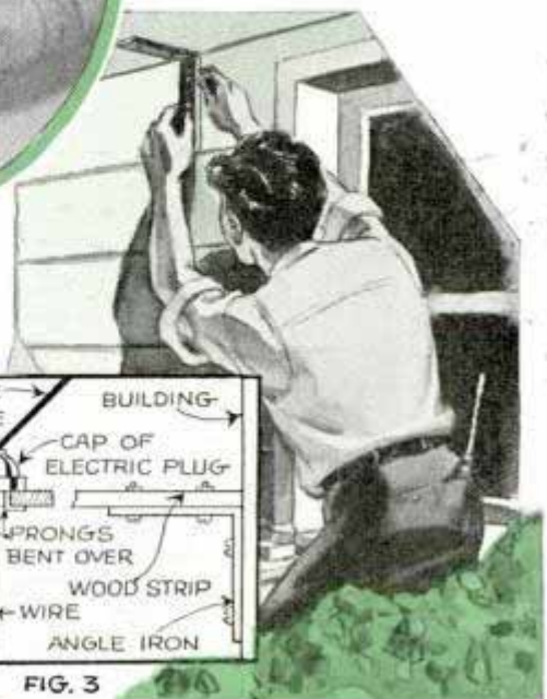
Fig. 3, insulating grommet, for antenna lead-in wire, made from electric plug cap; wood strip, mounted on angle iron, is fastened to building at any convenient point near window
