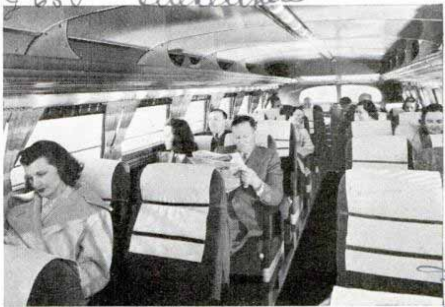
Air conditioning under driver's control, Venetian blinds and adjustable seats are comforts of Diesel buses operating from Chicago to Pacific
