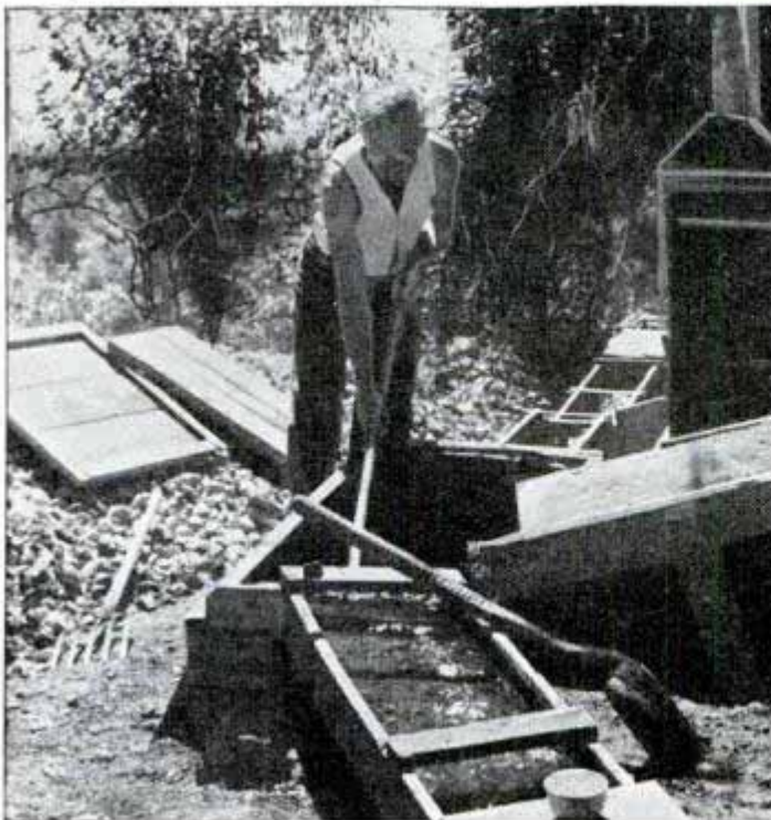
Top, resting place of early prospector; right, dry washer that separates gold dust from sand. Below, working sluice box in Mother Lode country
