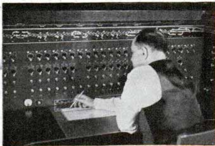
Dispatcher, top, talks to towerman by flicking switch; telegraph automatically reports passage of train. Below, Burlington operator at Brush, Colo., watching diagram showing train positions, controls 112 miles of line. Automatic log, right, records train movements, "R" indicating nonstop meet
