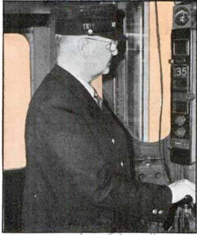
Top, old and new ways of switching; operator at right pushes two buttons lining up train route to San Francisco bay bridge. Center, governors on axle of bay bridge interurban hold train speed to limit shown on motorman's panel, below, according to track conditions ahead
