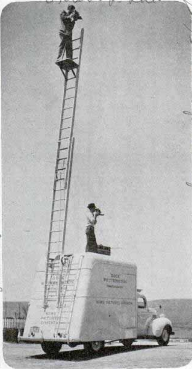
One feature of camera truck is this extension ladder for shots from above
