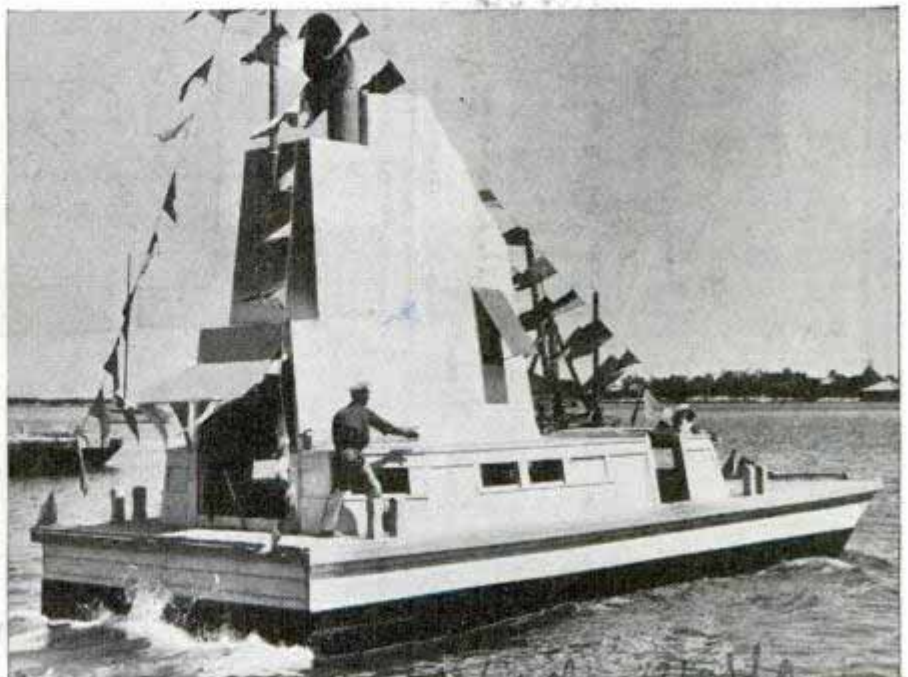
"Photosphere" for undersea observers is lowered from well inside barge
