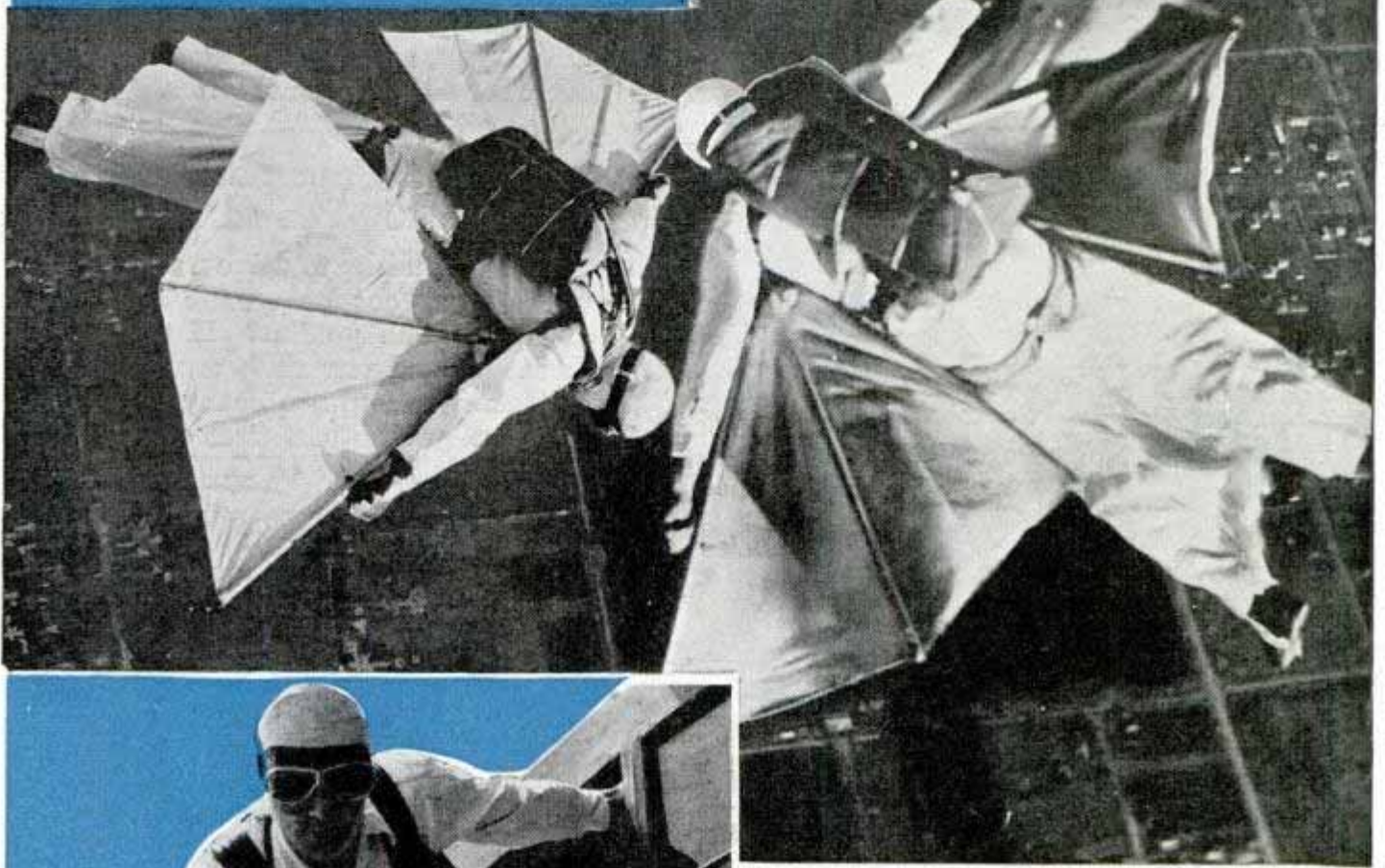
Above, the human glider in two positions simulating those in which he would appear shortly after leaping from the plane high in the air. Note the manner in which the wings are being used. The web between the legs aids in controlling the slow downward swoop. Left, at the moment of leaving the plane
