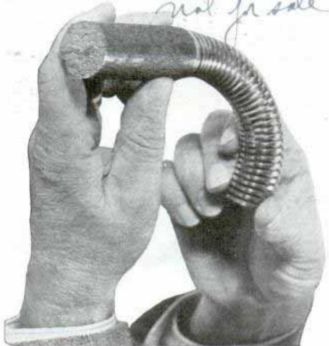
Coil spring of cast iron, bent "U"-shaped, returns to original shape without cracking or distortion
