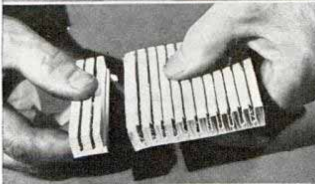
Slots in these sanding blocks permit bending them to fit a concave or convex surface
