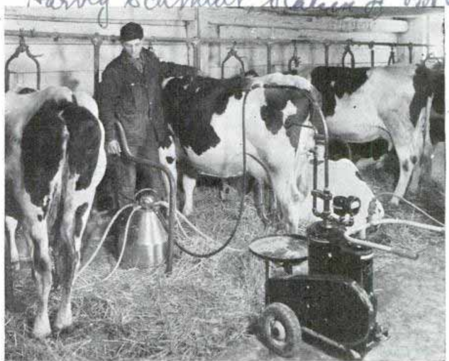
Portable milking machine delivers milk to covered pail under vacuum
