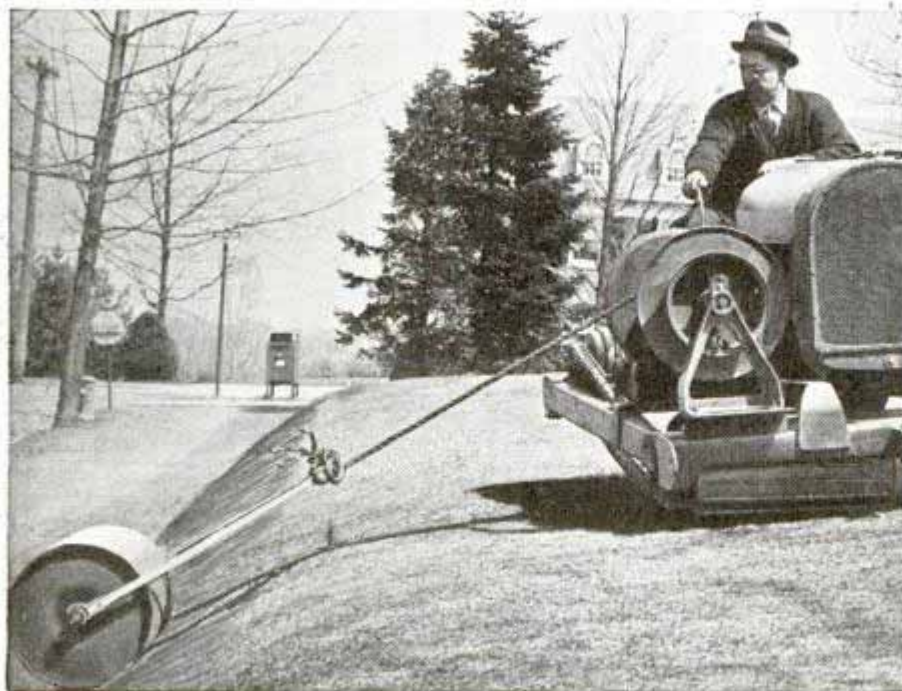
Demonstrating how power roller may be used in maintaining lawns on sloping ground. The machine rolls one acre per hour
