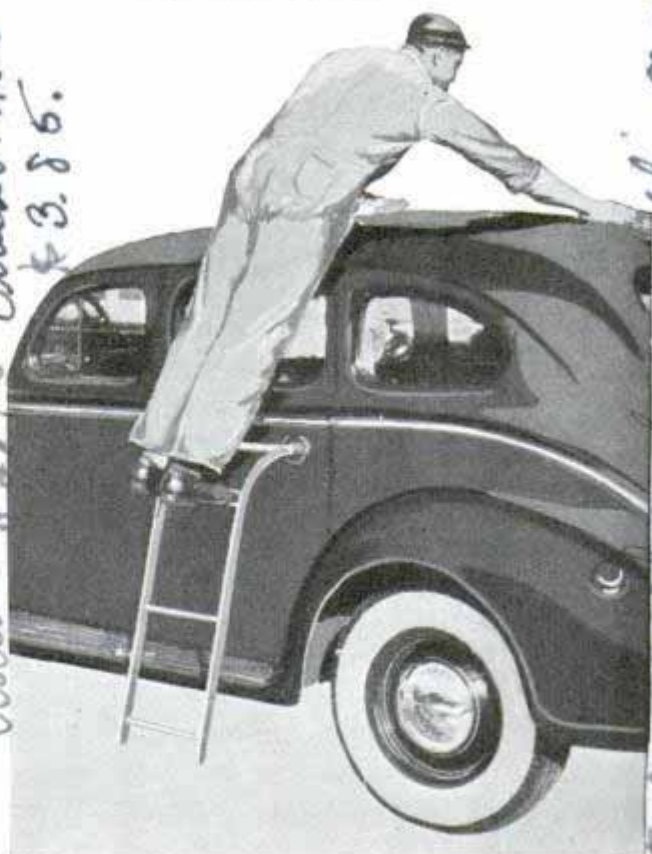
Rubber cups of strong ladder holding workman grip side of car and will not slip or mark car's finish
