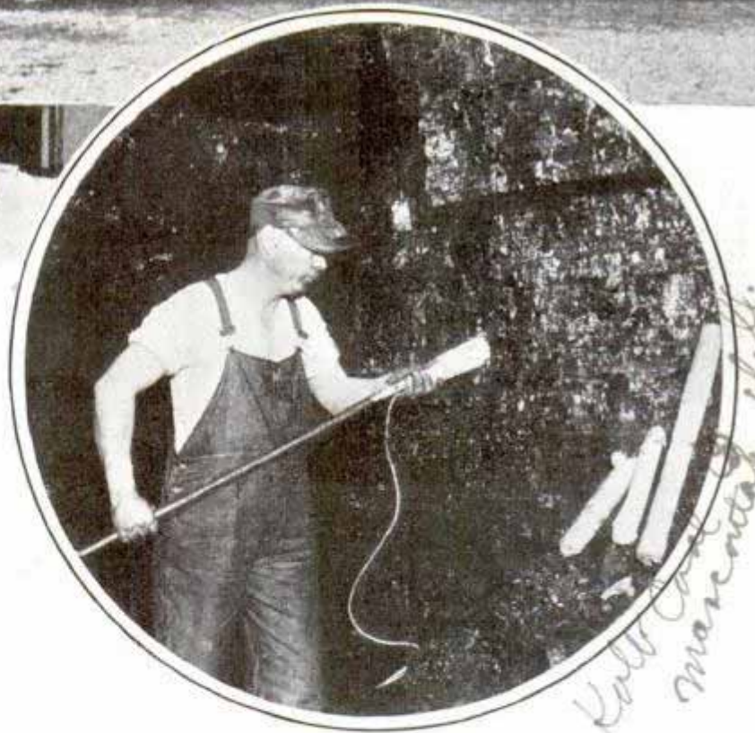
Ready to shoot (left), a blast that bears close resemblance to a forest (right) and ramming powder into face of coal mine (bottom)
