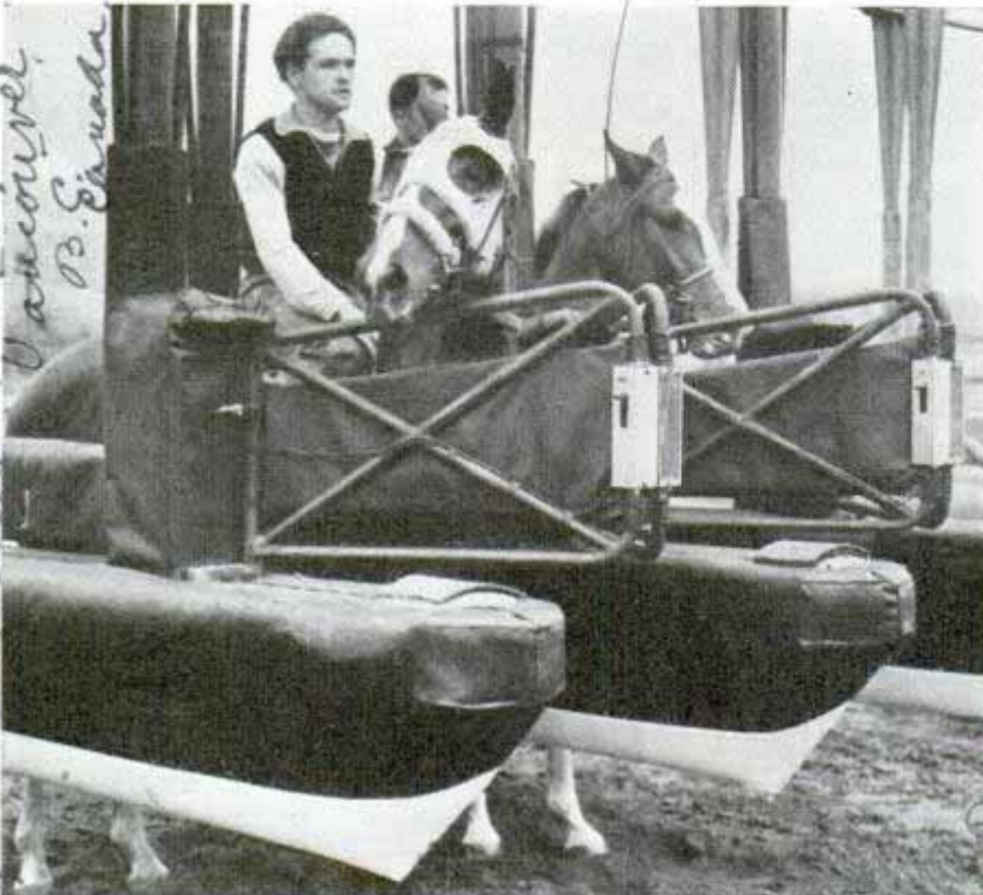
Led into these padded stalls with gate in front and bar in back, horses cannot back or break away until starter opens gates simultaneously
