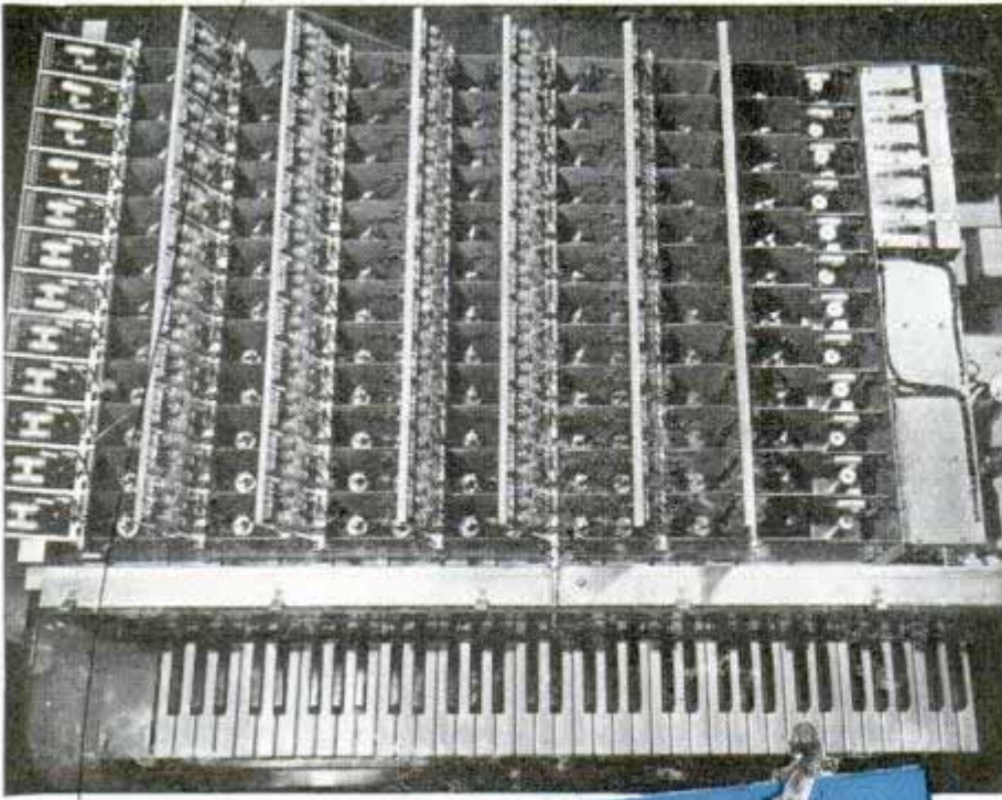
Tones of the Novachord (above) are produced by circuits of ordinary vacuum tubes. A new non-electric instrument (right), a cello-horn. Bottom, another new instrument, the vibra-harp, has the sound of a harp-but is played like a piano
