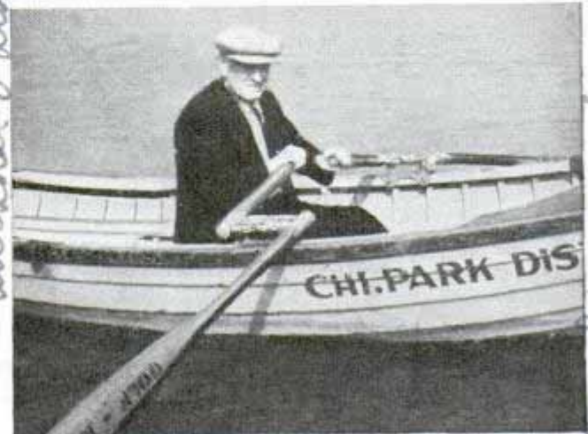
Top, oars folded. Note the gears. Bottom, oars in use with boatman facing forward
