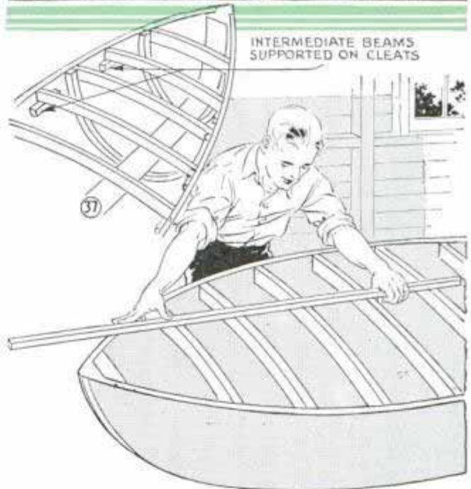
TESTING DECK BEAMS WITH A STRAIGHTEDGE
