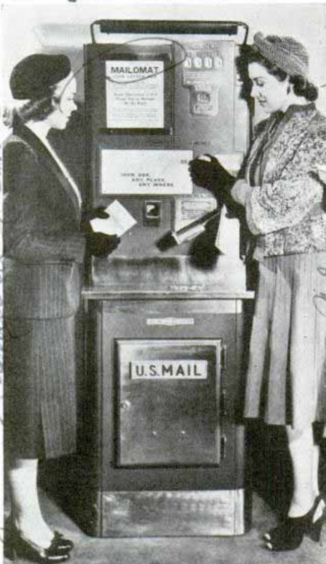
Slot-machine post office weighs letter, then stamps it and deposits it when proper coins are inserted
