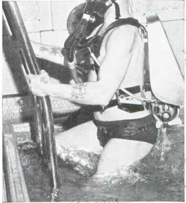
Diver leaving water after proving ability of gas helmet he is wearing to supply a man with air while working below surface
