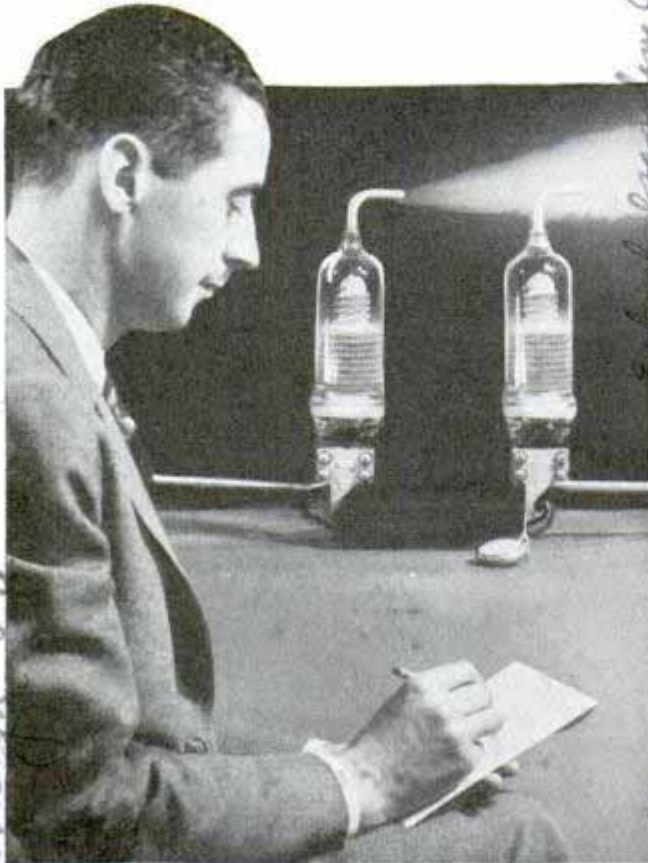
Jet of steam superheated to 350 degrees emerges from tip of "bottle" fifteen seconds after plugging in
