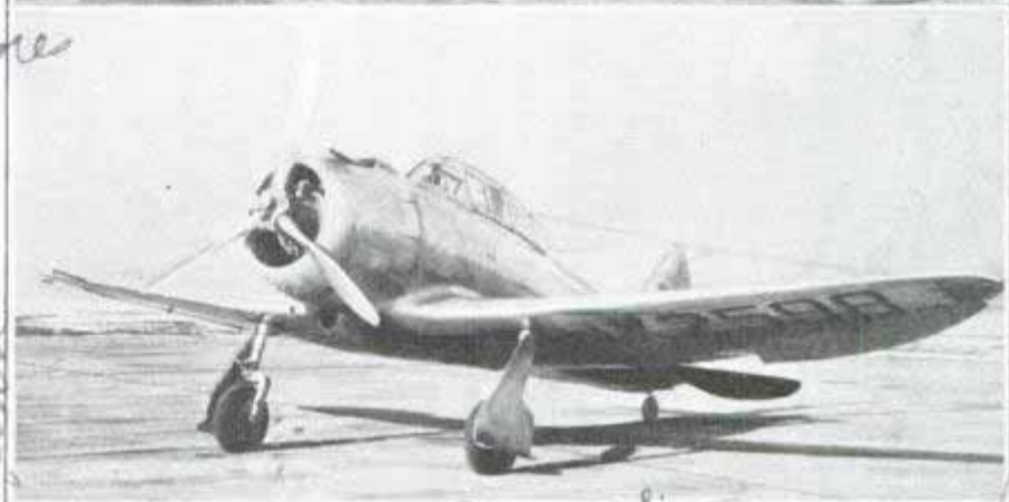
Top, the Bell "XP-39" pursuit plane with retractable tricycle landing gear; below, the Seversky "XP-41." Both are undergoing army trials
