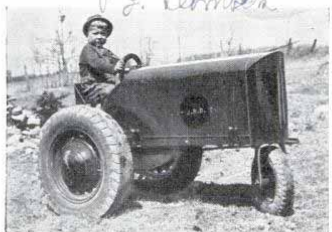
A washing-machine motor drives this midget tractor at a speed of one mile an hour
