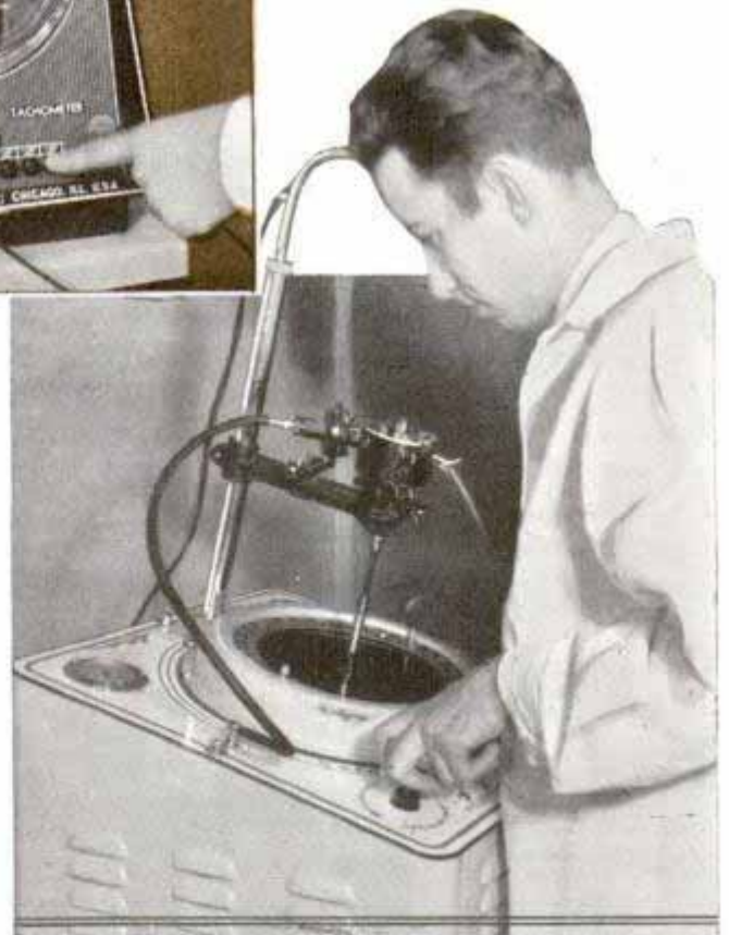
Top, locating trouble with modern tune-up equipment. Center, instrument for attaching to ignition distributor aids in tuning engine. Bottom, testing vacuum advance of distributor
