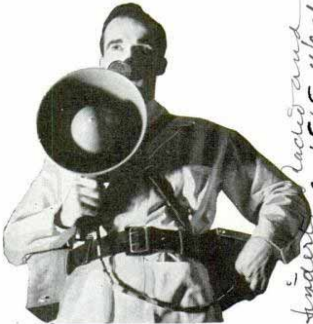
Guide's voice can be heard above machine noises by visitors when he speaks through portable amplifier
