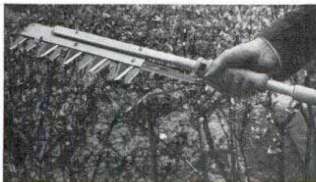
Cutting the shrubbery with the aid of hedge trimmer operated like a pump-action gun
