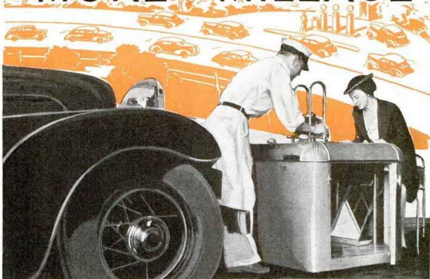
Wheel tester permits car owner to see if anything is wrong (above). Right, sketch of how tester works. Bottom, what car owner sees in small mirror on machine. Wheels at left are obviously out of alinement; those at right have been corrected. Note how images of front wheels are drawn together by the mirrors
