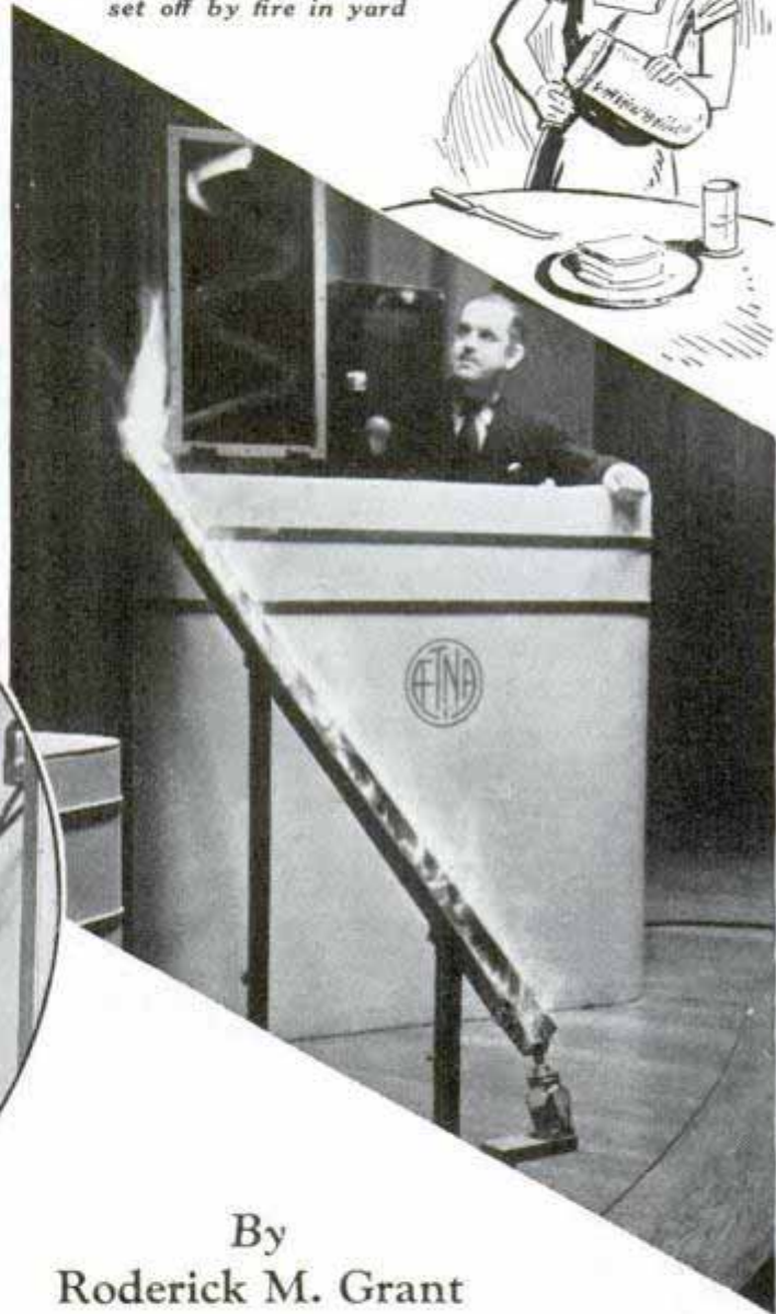
Touching light fixture and faucet invites electrocution, left. Below, keep electric cords from children and be sure they bear safety tag of Underwriters' Laboratories. Right, reproducing accident in which gasoline vapor flowed downstairs to be set off by fire in yard
