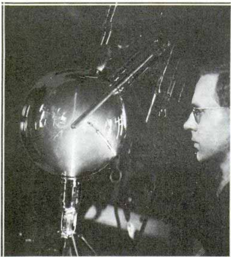
Luminous path of electrons in gas-filled tube is curved by magnet simulating creation of aurora borealis by magnetic pole
