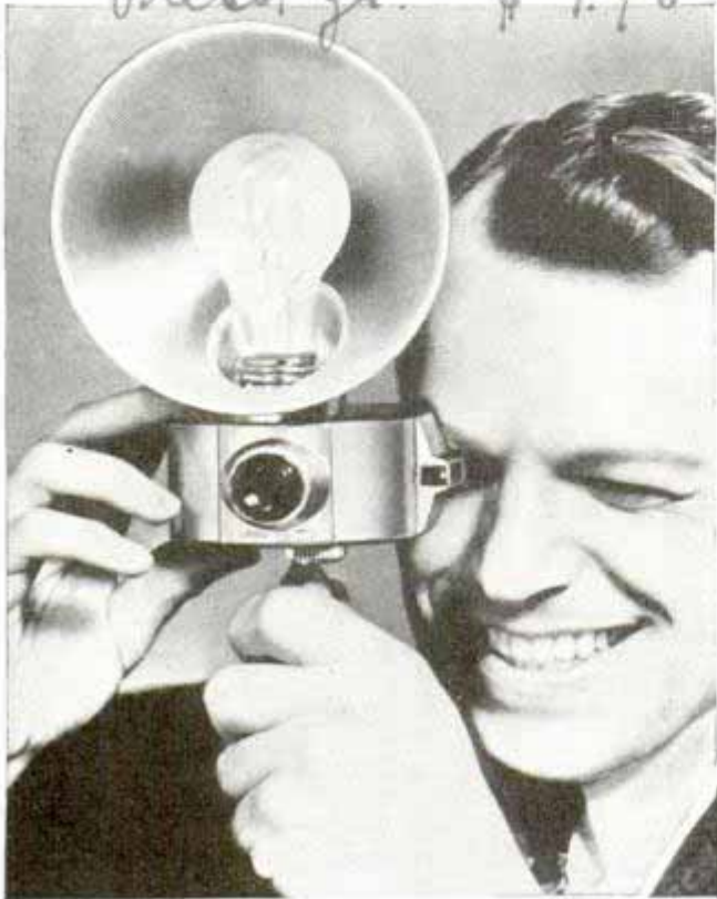
Battery-operated flash bulb fits in top of camera and is synchronized with shutter
