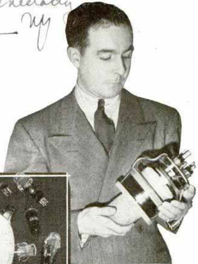
At left are some of the 648 tubes involved in the complicated task of broadcasting television. They range in size from the big camera tubes to the midget held between fingertips. Above, one of the costly water-cooled tubes which do the real work of transmitting
