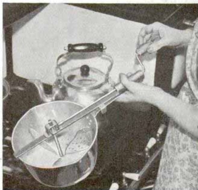
An occasional twist of the handle turns the mixing paddles, keeping food in motion so it will not burn
