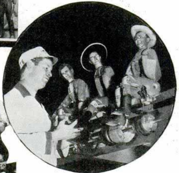
Circle, heads of cowboy figures were carved from photos of prize-winning riders. Left, intricate mechanism that animates the cowboy models makes each wave the right arm when each is introduced by name by the announcer. Action of the model is controlled by six motors and thirty-two solenoids
