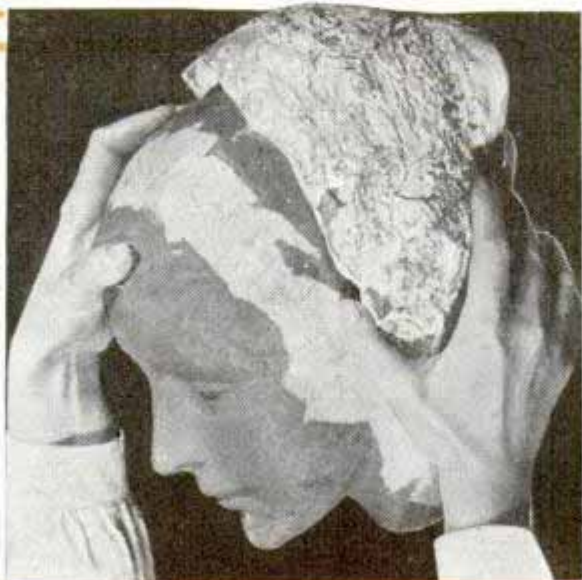
Above, installing the arm mechanism of a violin player. Right, head of dummy, made of paper in halves which are put together and the joint covered smoothly. Here the rear part of the head is being taken out of a plaster mold. Head motors operate the eyes and lips
