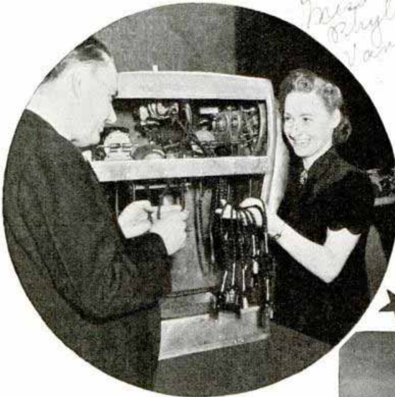
This is "Elektro," the seven-foot robot built by Westinghouse. Motors, relays and other mechanism enable him to perform thirty-six tricks
