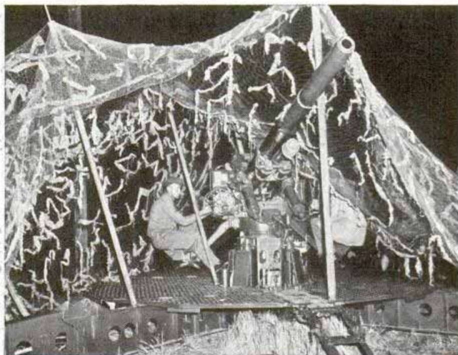
Anti-aircraft gun mounted on circular steel platform would easily be spotted from the air but for the camouflage net covering it
