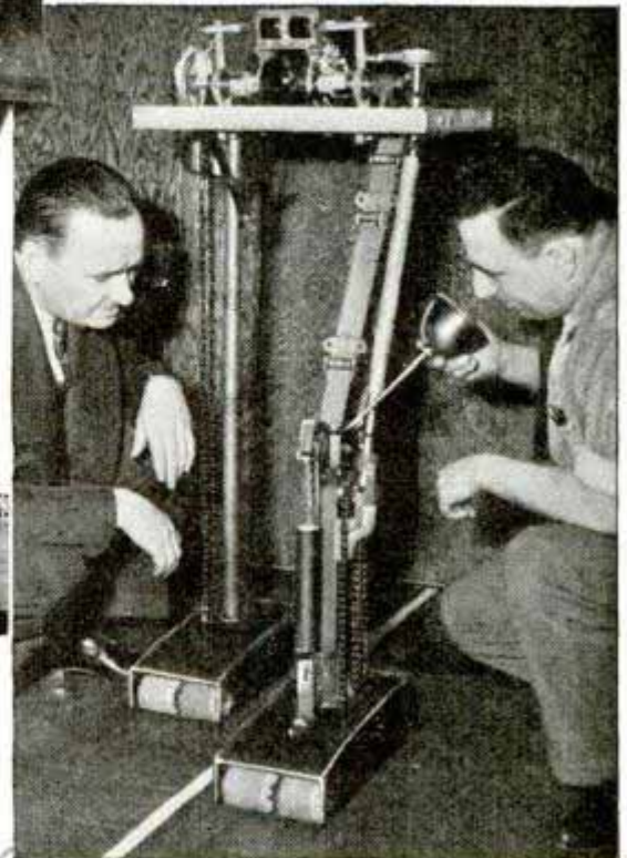
Top, left, showing some of the electrical cords used to control the moto-man. Right, the robot sings through his sound mechanism, his mouth waggling open and shut. The robot is made of 900 parts, the frame is steel and the covering is aluminum. His tricks include walking, talking, distinguishing colors, smoking and bowing
