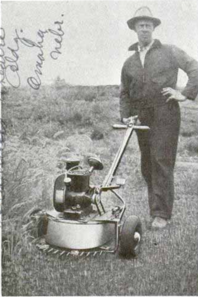
Cutters rotate at high speed in one direction, slashing off high grass and weeds gripped between tines
