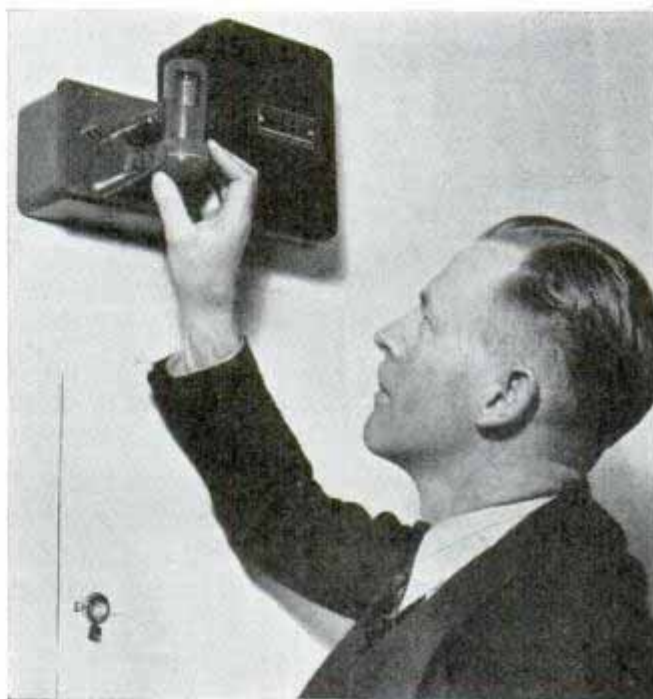
Adjusting sensitive eye of photoelectric relay that switches lights in room on or off as needed
