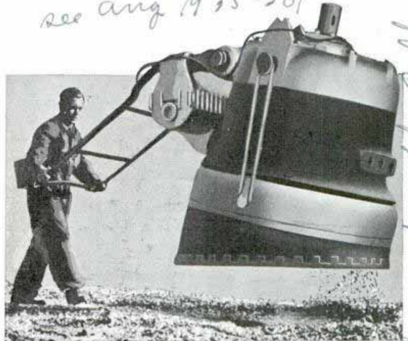
Benzol explosion controlled by operator makes tamper jump upward and forward, pounding road with 5,500-pound weight
