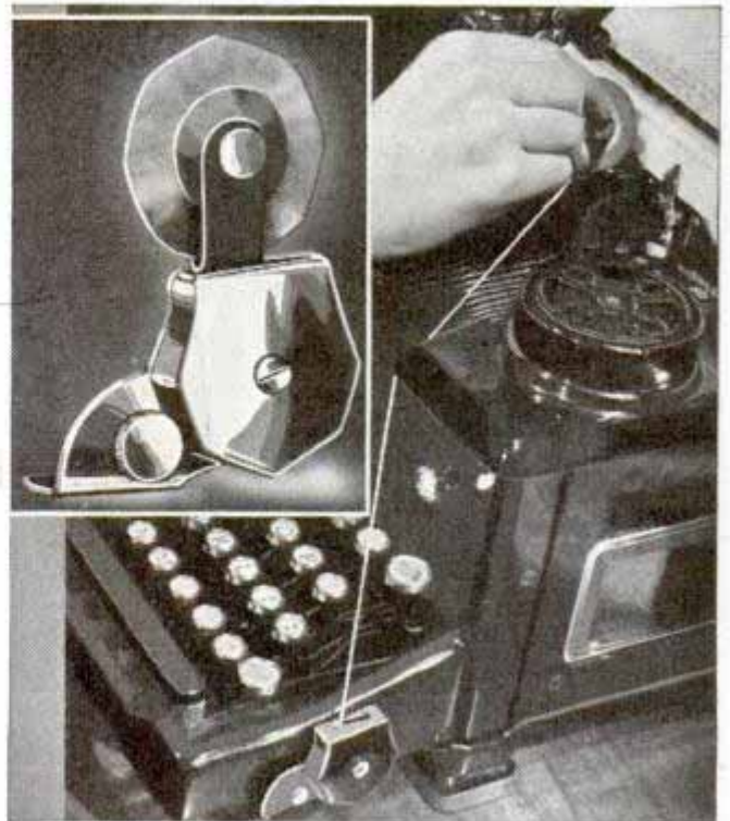
Spring draws eraser back to reel, shown in inset, when typist is through with it
