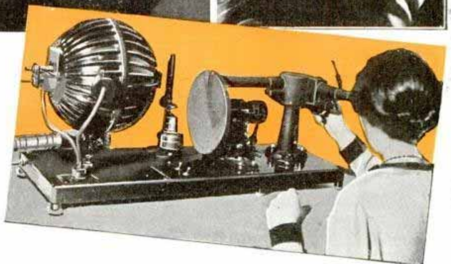
Top, bases for paint flowing through roller mill. Center strip, left to right, applying interior house finish; paint mixing and shading in fifty-gallon batch, and color test by spraying. Bottom, machine breaks color into its spectral components, making possible actual physical measurement of color values
