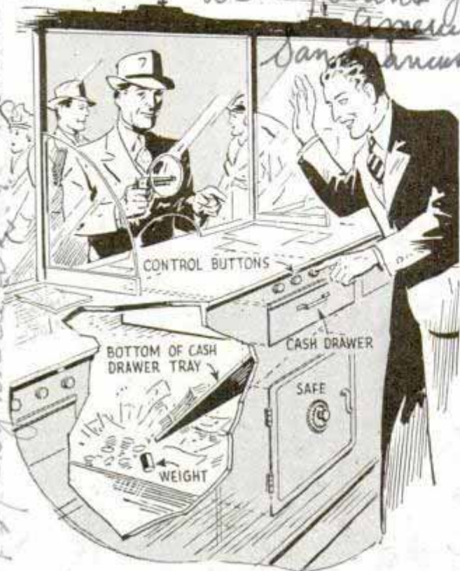
Pressing button throws money into the safe. Weight drops out, too, so tray can snap back
