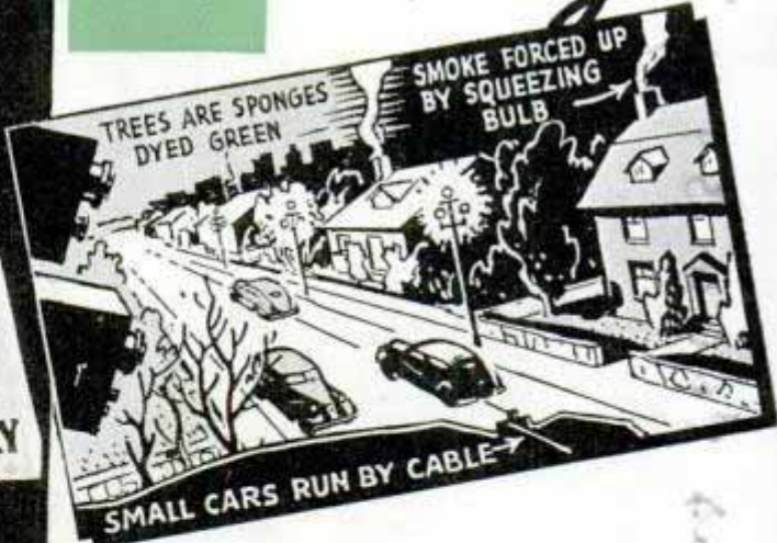
Sketches on this page, and the next, show how realistic scenes are created for television. Model villages with one-half candlepower lights, midget autos controlled by cable, dyed-sponge trees and shrubs and carefully constructed buildings are employed effectively. Lightning flashes are obtained for the village by opening and closing an electric switch
