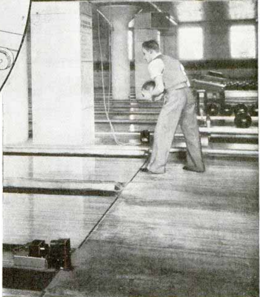
Left, some tasks performed by "electric brain." Right, pinhole detector for catching flaws in steel. Bottom, if player steps over foul line of bowling alley, the photoelectric detector immediately reveals the error
