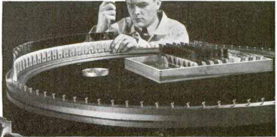
Left, installing one of two 2,500-watt lamps in twin-lens projector. Each of eleven projectors weighs 2,700 pounds. Water cells and near-freezing air blast are used for cooling. Below, the ingenious device which keeps film image centered in lens and rock-steady on screen even if slide is out of position; small plate of optical glass spins as film drum turns, refraction through glass centering the image. The natural-color transparencies used were made with cameras similar to your own
