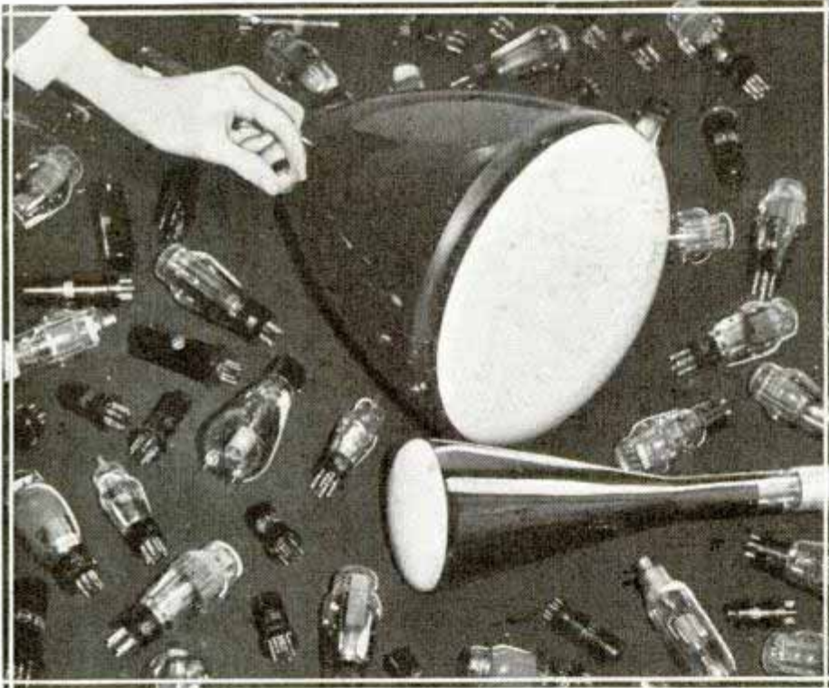
At left are some of the 648 tubes involved in the complicated task of broadcasting television. They range in size from the big camera tubes to the midget held between fingertips. Above, one of the costly water-cooled tubes which do the real work of transmitting
