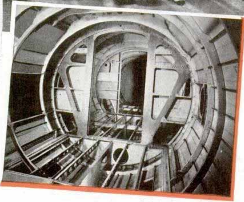
Top, loading a flying box car with heavy consignment of machinery. Left, interior construction of Douglas "DC-5," which is capable of carrying a three-ton load.
