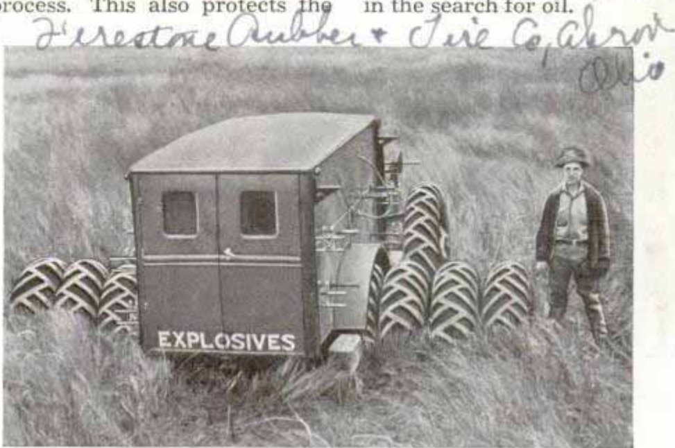
Here's how the big tires support truck as it travels through marshes
