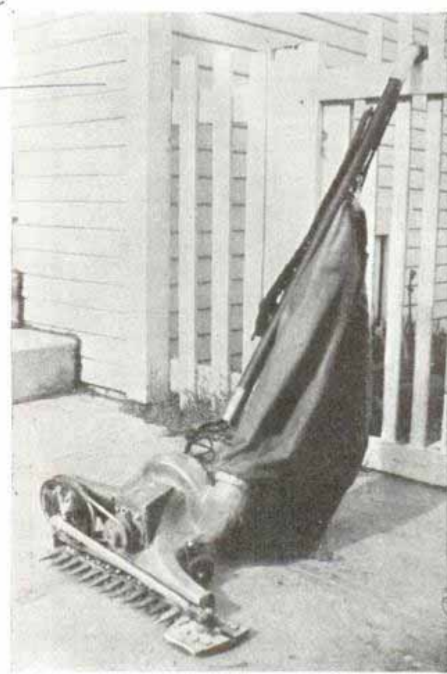
After cutting head clips the grass, the vacuum cleaner collects cuttings and weed seeds in bag
