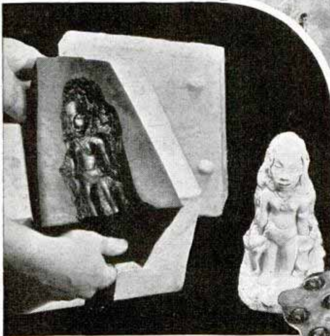
Above, coated textile roller after twenty months' use. Right, Koroseal-silk gown. Below, left, Koroseal mold for plaster casts. Right, trimming sheet of Koroseal hydraulic shock absorber gasket
