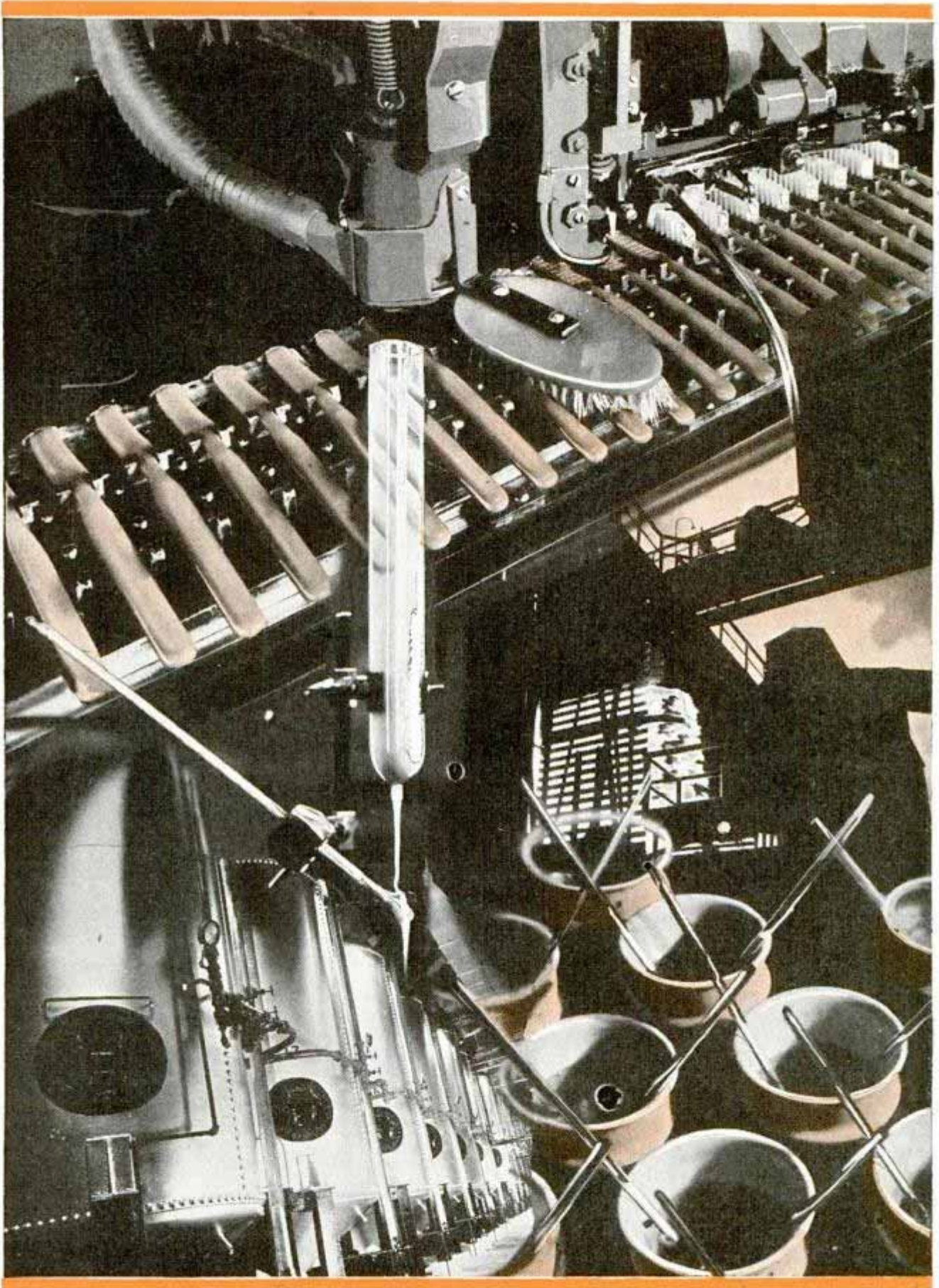
Leominster, Mass. Richmond, Va. Flashes from the world of chemistry. Top, machine drills holes in toothbrush handles, inserts bristles and anchors them automatically. Center, liquid viscose dripping from white tube. Right, incandescent coke being pushed out of ovens. Bottom, left, aging tanks used in manufacture of "Cellophane" cellulose film. Right, porcelain pots, glass rods and textile yarns in dye bath
