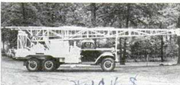
Oil drillers' rig mounted on truck whose all-wheel drive can negotiate hill country, swamp or desert
