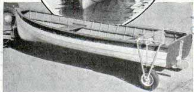
Boat as two-wheeled trailer towed by auto. Circle, wheels being flipped into boat after it is launched
