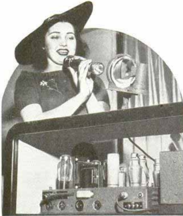
Speaker's voice is picked up by microphone in flashlight and varies beam reaching electric "eye"
