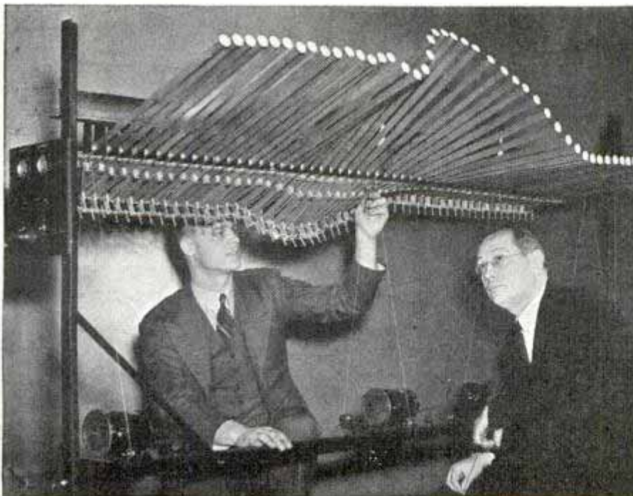
Aluminum bars trace in "slow motion" the wave surge of electric current while engineers simulate a short circuit on a power line
