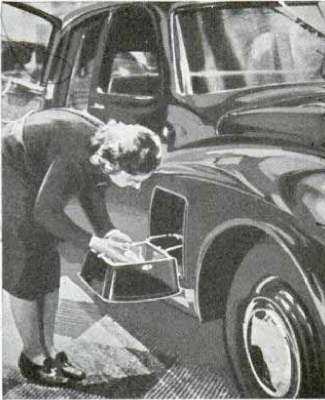
Washing up in the basin built into the waste space beneath the front fender of the car
