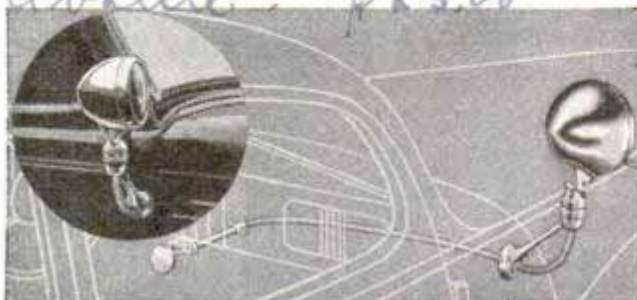
Driver controls spotlight on right-hand side by cable shown in diagram. Circle, lamp mounted on car
