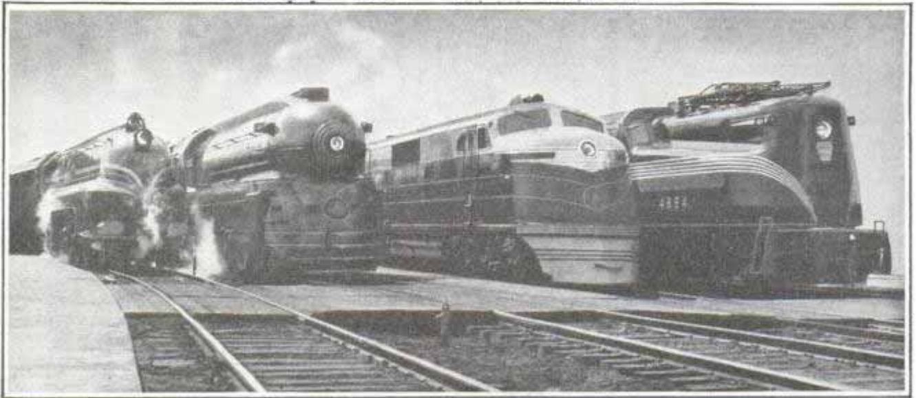
Here's a "four-horse" team representing the latest in steam, Diesel-electric and electric power. Left to right, British "Coronation Scot," two Baltimore and Ohio locomotives and a Pennsylvania electric engine
