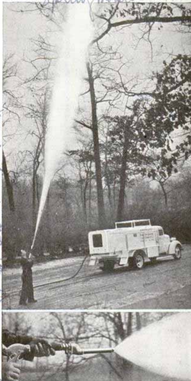
Top, sending fine stream into treetops. Below, operator's left hand grips the focusing control
