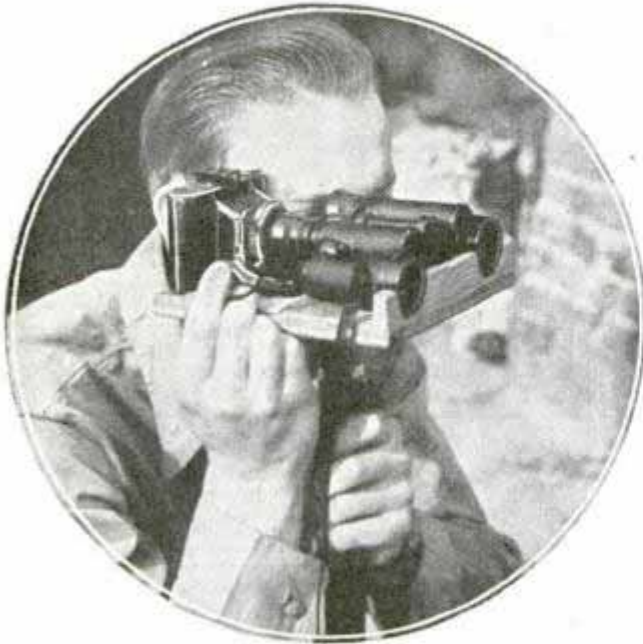
With camera mounted at right eyepiece of binoculars, distant view is brought into focus through left side
