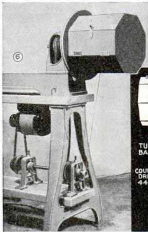
The speed of the barrel should be in a range from 40 to 90 revolutions per minute. Photo at left shows a simple cord drive for light work, while diagram below shows a suitable installation for regular work
