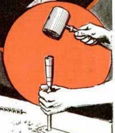
THE MORTISES ARE BORED—THEN SQUARED WITH CHISEL.
