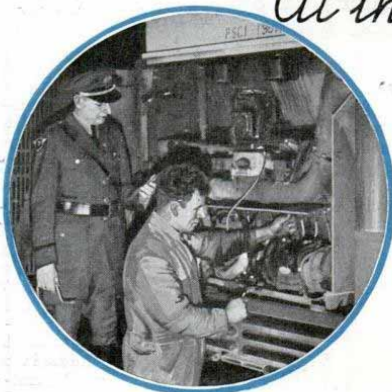
Top, driver examining ticket of a passenger. Center, a big coach on the road. Bottom, driver stands by while mechanic adjusts the huge 200-horsepower motor located at the rear of the bus. Experimental work with Diesel-powered coaches has been under way for some time to determine whether oil-burning power plants would be better for buses than the gasoline engines now in common use
