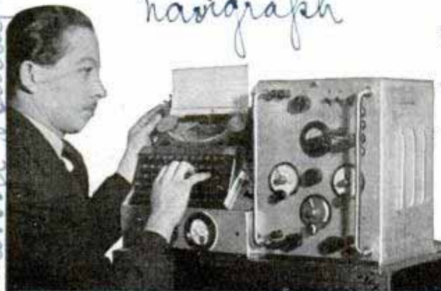
After dialing a distant receiving typewriter, the typist transmits his message by radio
