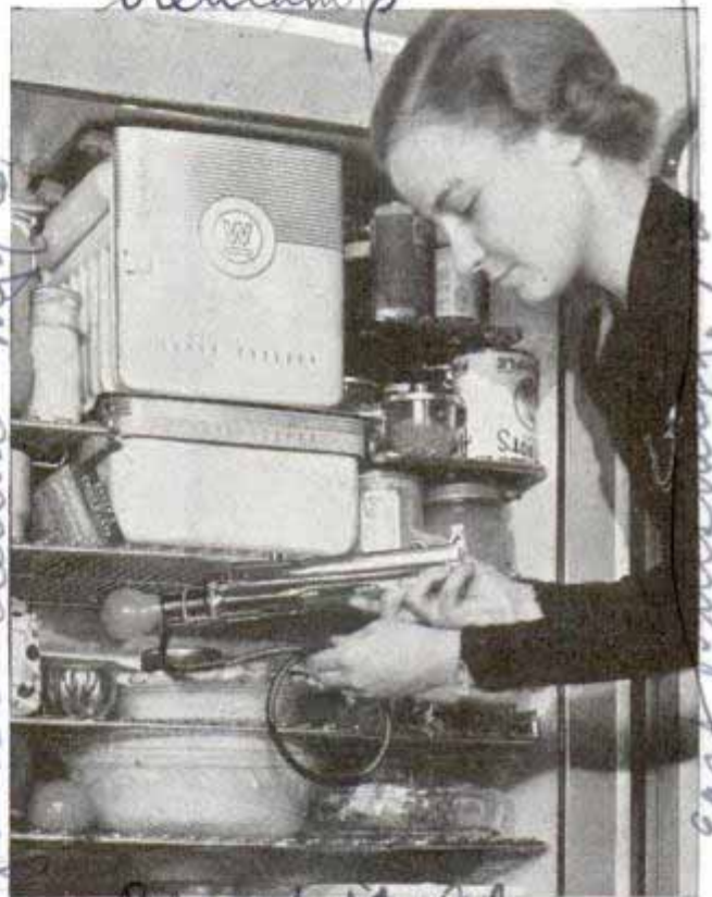
Tube lamp emits ultraviolet rays which kill bacteria floating in air within refrigerator
