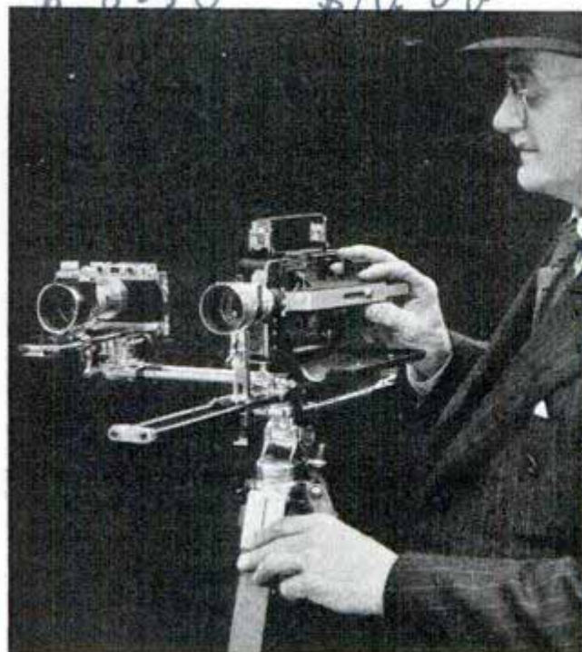
Without disturbing action of movie camera, still pictures can be snapped with camera on-twin mount
