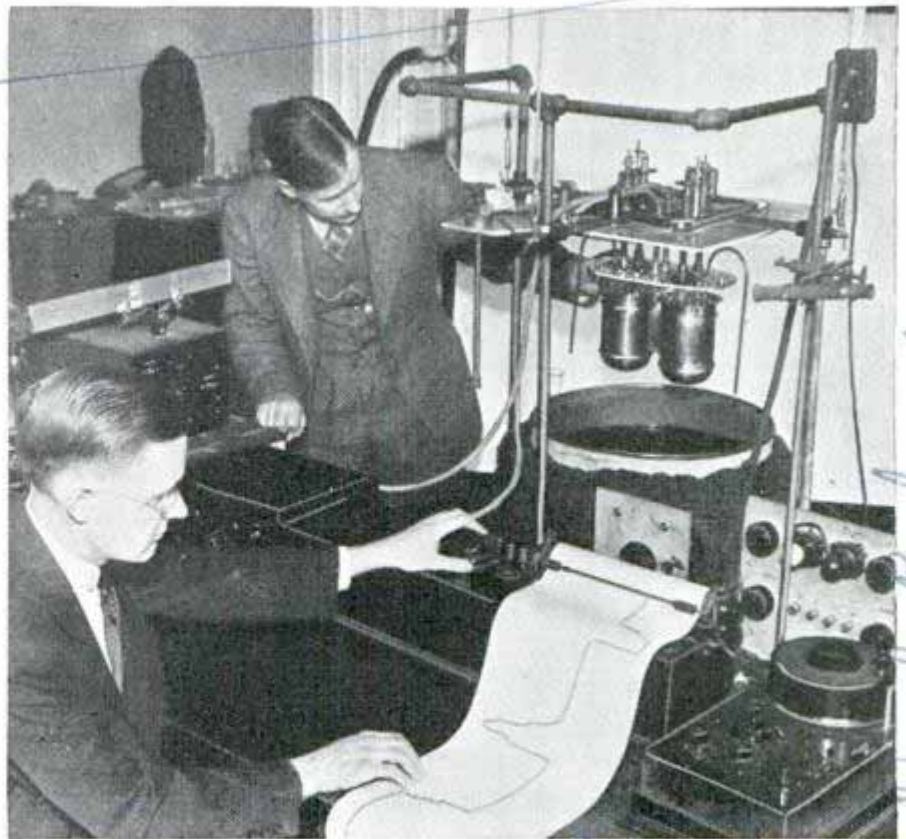
come Measuring minute temperature changes in a substance placed in one of the metal containers above vat. Heat graph is recorded on paper roll
