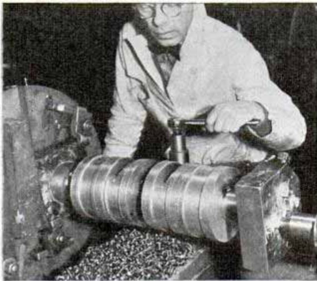
Turning solid billet of metal in lathe to create counterbalanced crankshaft for four-cylinder engine
