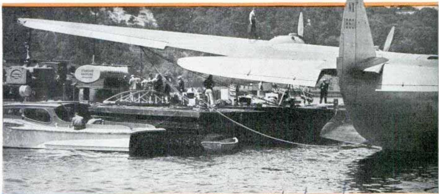
Sukorsky Top, another sky giant, the "Flying Dreadnaught," which was tested by Eddie Allen. Bottom, gasoline trucks go to sea on barges to service the mighty Boeing clipper during test flights
