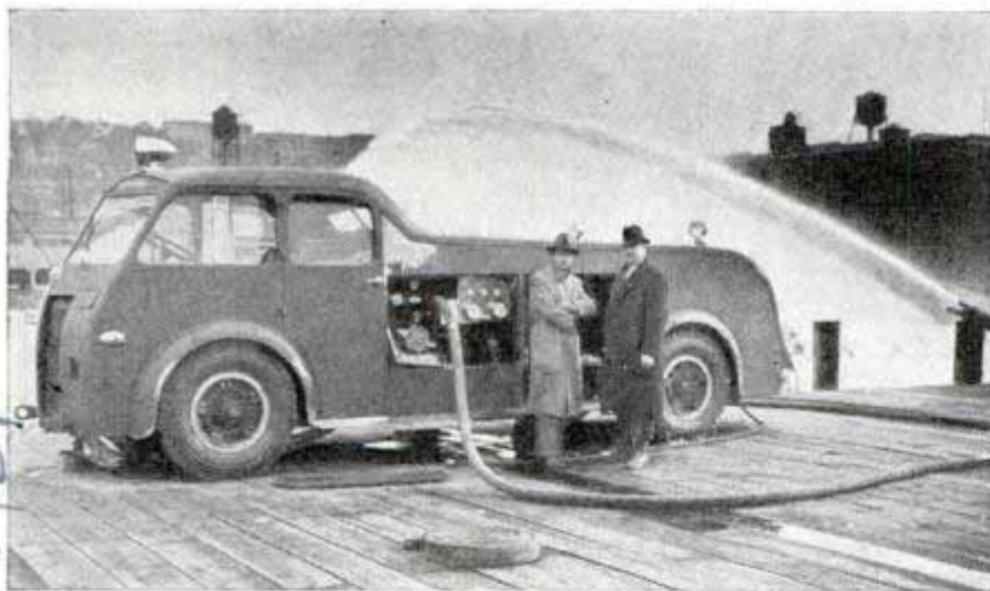
With low center of gravity and a wheelbase six feet shorter than the average fire truck, this pump and ladder car makes short turns at high speed
