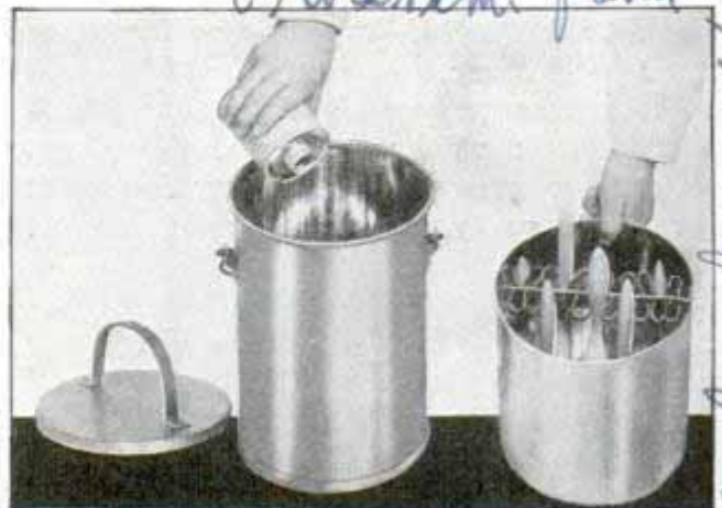
Pouring liquid into brush container, and, right, view of can with brushes suspended from holder at top
