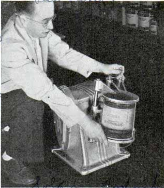
Clamped on the electric vibrator, the can of paint is given a vigorous shaking to prepare it for use
