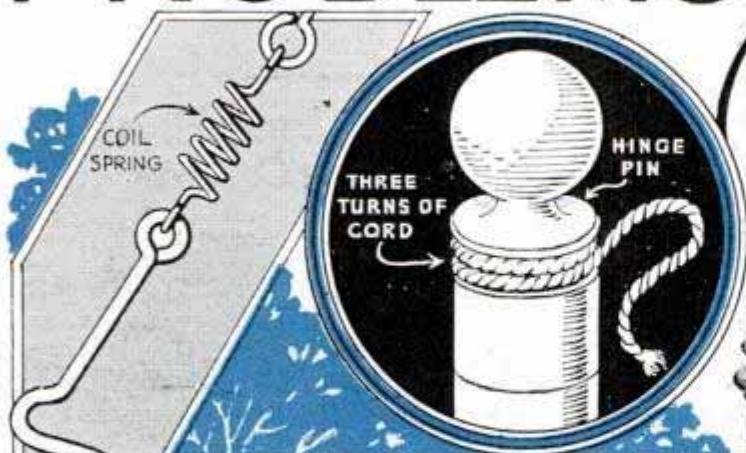
Right, two turns of cotton cord wrapped under hinge pin and kept oiled furnish lubrication and eliminate squeaks. Attach a screen-door hook with a small spring as above and it will hold the door snugly and allow enough flexibility to fasten the hook easily
