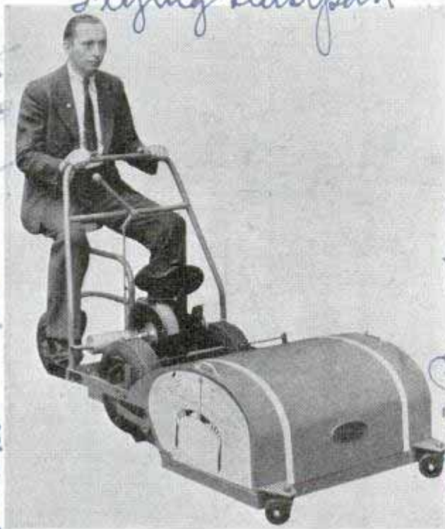
Operator rides along to steer dustpan. Pressure of broom on floor is fixed and always remains the same
