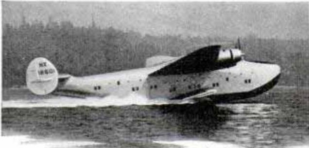
Pilot Allen lifting the Boeing clipper onto its planing step for a takeoff
