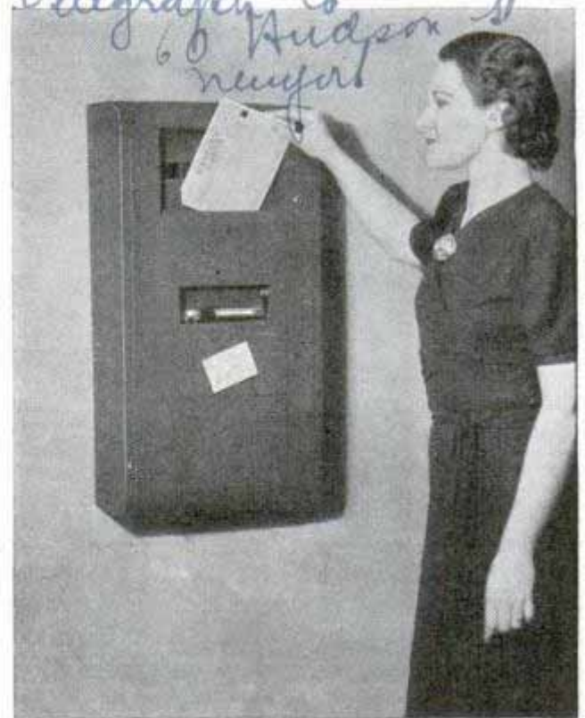
Dropping message in telegraph box, whence facsimile is automatically transmitted to the central office
