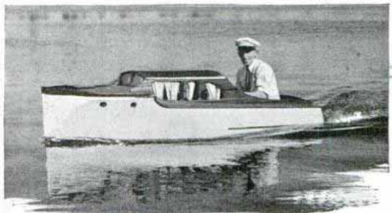
Undersized boat built to scale of three inches to the foot carries one man at ten miles per hour
