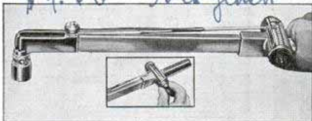
Turn of knob, as shown in inset, exposes scale and pointer is set to recommended tension
