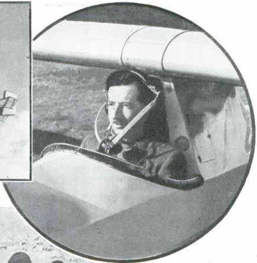
Above, pilot ready to be towed adjusts head-phone and mouthpiece. Left, two seated glider in air. Bottom, towing cable at back of car contains telephone wire
