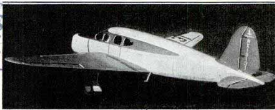
Five-seat plane with molded plywood fuselage cruises 200 miles an hour
