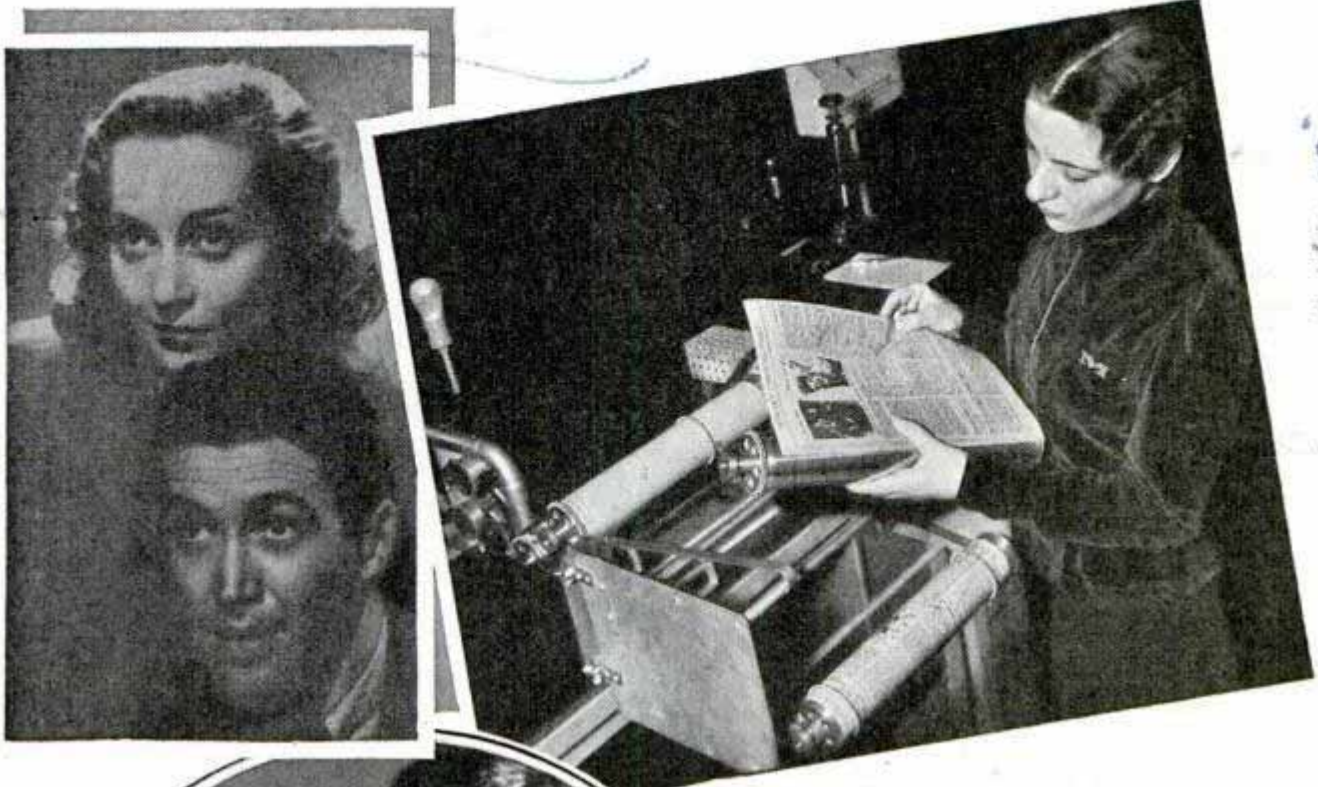
Right, page proof of magazine sent by facsimile method. Bottom, receiving a photograph transmitted by Western Union's new service. Upper left, reproduction of photo from a David O. Selznick movie, as sent by facsimile system
