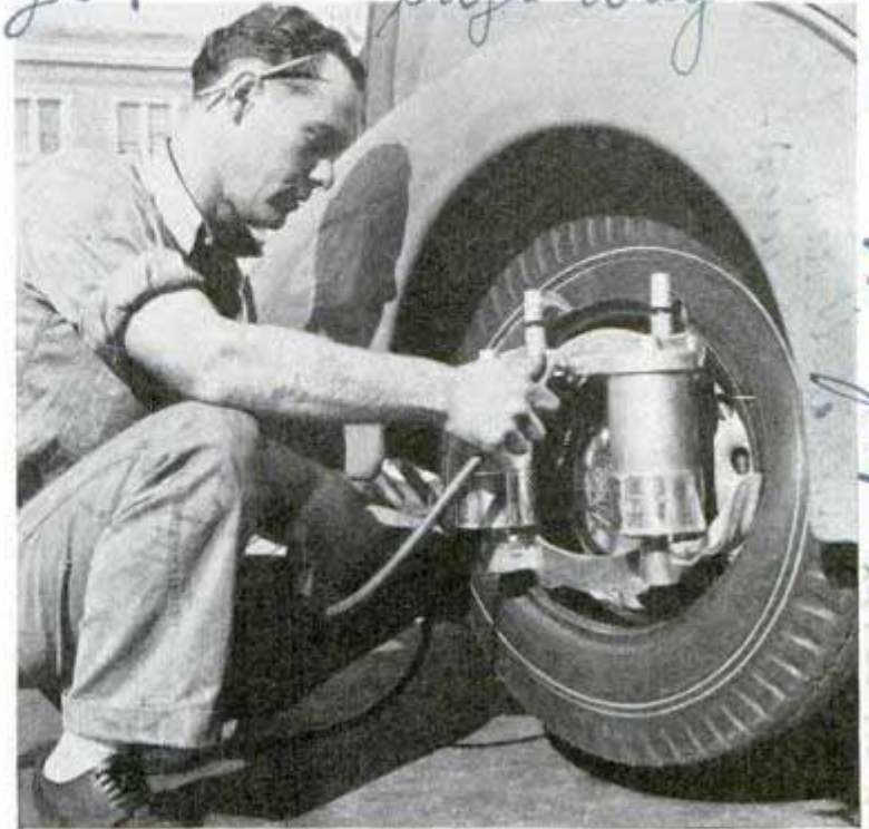
With tool hung from upper edge of rim, air pressure is applied and stretching arm snaps lower wall of tire in place on rim
