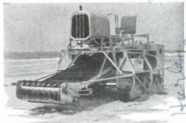
Sand scooped up by tractor is run through vacuum cleaner and then returned to beach minus all refuse
