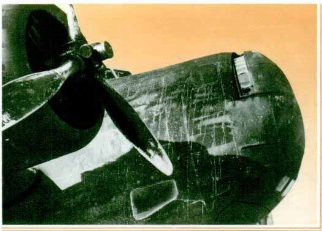
N OSE of bomber painted with lamp black. The dull surface reflects virtually no light, making the plane invisible from the ground at night, even in the rays of powerful searchlights. Bottom, New York from an altitude of 26,000 feet.
