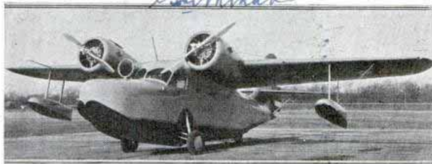
When army planes run into trouble at sea, this amphibian, now under test, can fly to the rescue at 140 miles an hour over a 500-mile range
