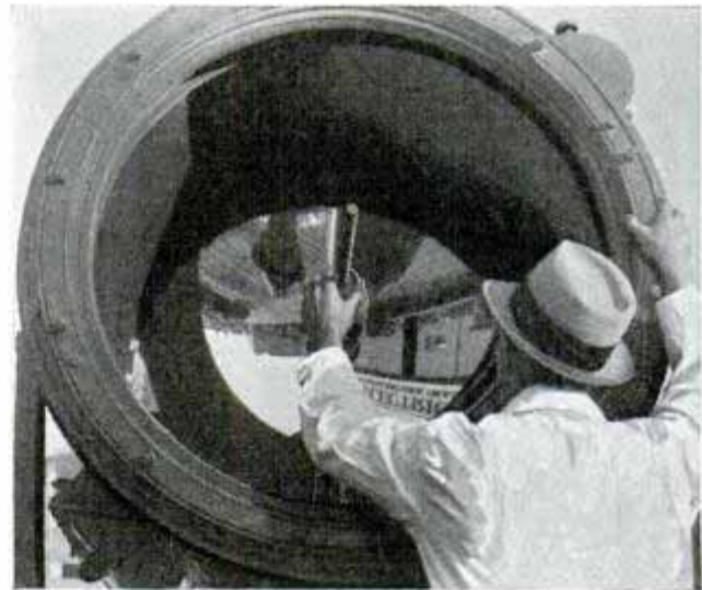
Adjusting carbons of a huge sun arc. Notice the perfect reflection in mirror behind the arc
