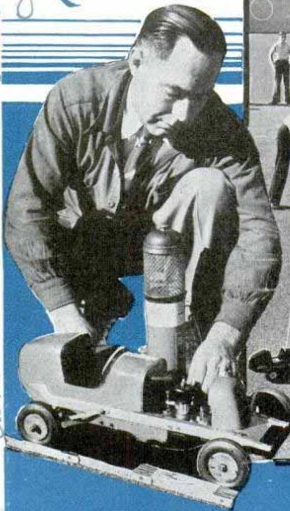
Above, Gordon A. Babb of Pasadena, designer, fills seventeen-inch racer's tank with two-ounce mixture of gasoline and oil. Right, "drivers" guide midgets in race on circular course by cords fastened to swivel joint on side of car. Below, underside of racer showing front-drive shaft and ignition batteries
