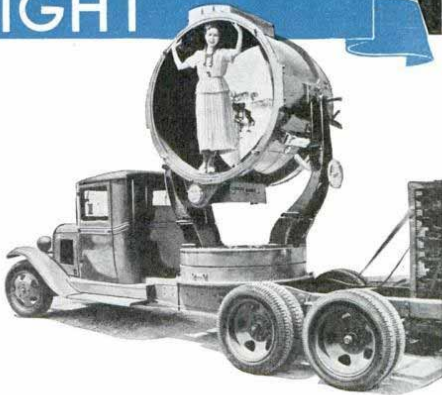
Top, battery of big sun arcs shines outside Hollywood theater where movie premiere is attracting celebrities. Below, head-high reflector cylinder of mobile 200-ampere arc projector which has a range of 100 miles
