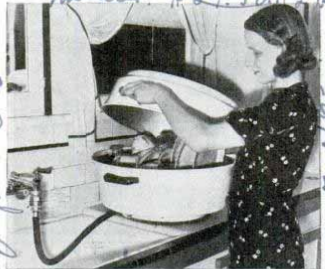
Placing cover on dishwasher before turning on hot water, which sprays dishes by means of rotating arms
