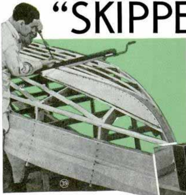
The garboard is the first plank to be fitted on the bottom. All bottom planks must be set in seam composition or similar adhesive in order to make watertight joints
