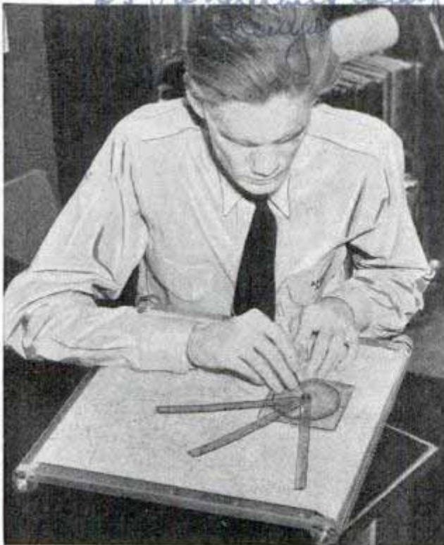
With protractor arms pointing to radio stations on which he has bearings, pilot finds his location
