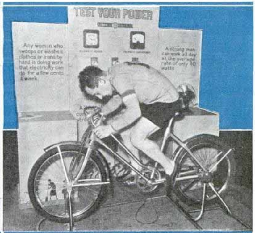
At left and above, old and modern methods of scrubbing and polishing floor. The bicyclist, pedaling a "bike" harnessed to watt meter, at his best could "pump" only 240 watts for an instant and in six full days could generate fifteen kilowatts
