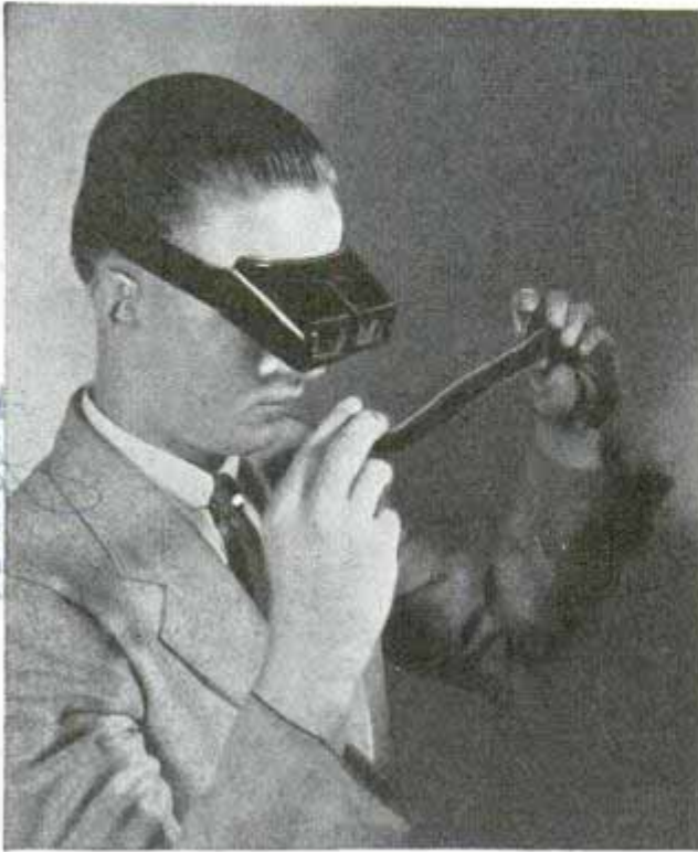
Both hands can be used for holding film before magnifier held on head by an adjustable band
