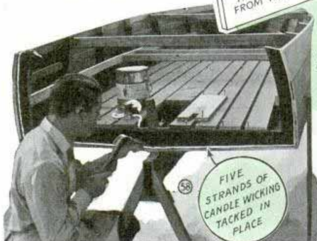
Drawings at right give details of transom and transom knees. Photo below shows joint being treated
