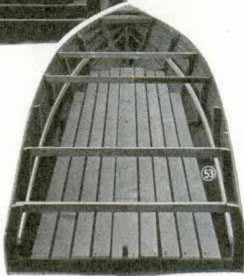
Above, seat risers and floor cleats in place. Photo at right shows flooring nailed in place
