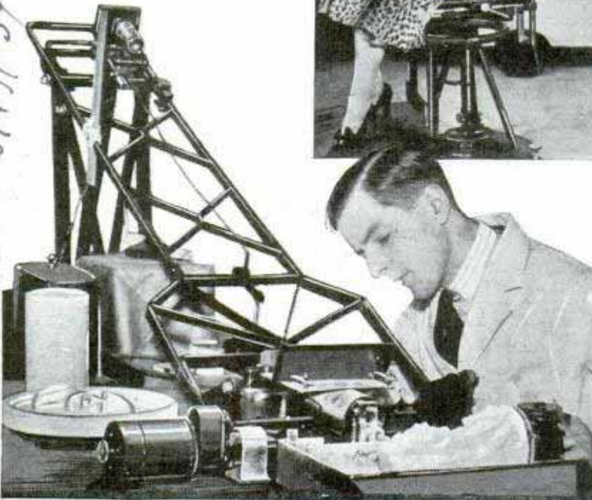
Above, S. T. Jeffreys, English originator of "photosculpture," with a mounted likeness of himself, and some of the busts and heads on his studio shelves. Right, vertical light beam scans face of the model as synchronized camera records contours. Below, automatic cutting tool, guided by film record of contours, carves out a bust from block of material
